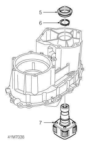
**5.** Using a flat bladed screwdriver free of rough edges, ease input shaft oil seal from front casing.
