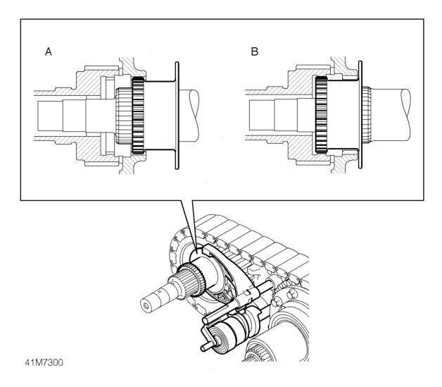
High and Low range are selected by the driver from a dashboard mounted switch on manual vehicles and via the selector lever on automatic vehicles. Transfer neutral is selected by inserting a 5 Amp fuse in position 11 of the driver's seat fuse box. Refer to Owner's Handbook.
