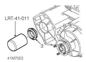
**3.** Position oil seal to transfer box front casing and fit oil seal using LRT-41-011.
