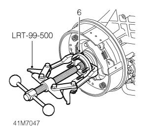
**6.** Using LRT-99-500 if necessary, remove flange from output shaft.
