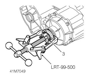
**3.** Using LRT-99-500 if necessary, remove drive flange from front output shaft.
