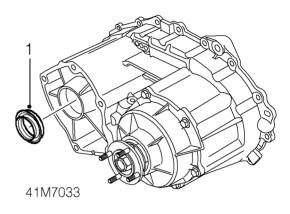
1. Using a flat bladed screwdriver free of rough edges, ease input shaft oil seal from transfer box front casing.
