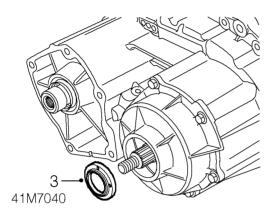
2. Using a flat bladed screwdriver free of rough edges, ease front output shaft oil seal from front casing.
