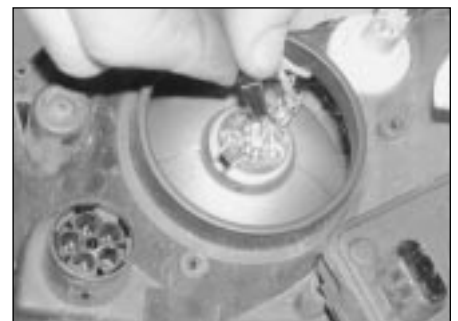
5.3 Disconnect the wiring plug from the bulb
