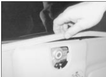
25.19 Release the sealing strip from the front of the console
