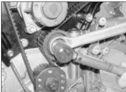
7.18b . . . then hold the pulley stationary and tighten its retaining bolt to the specified torque
