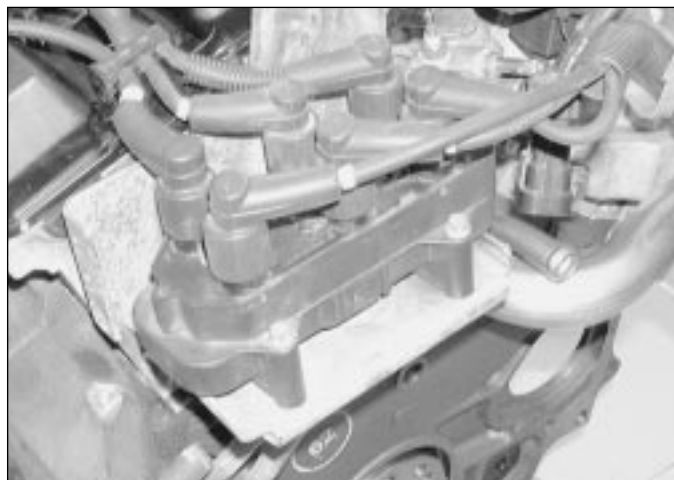
3.8 On 2.5 and 3.0 litre engines the DIS module is mounted on the rear of the left-hand cylinder head (later model shown with engine removed)
