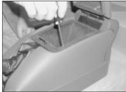
30.2a Open the lid of the storage box to the rear of the handbrake lever, then undo the four screws . . .
