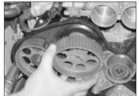
8.3b . . . and remove the sprocket from the camshaft
