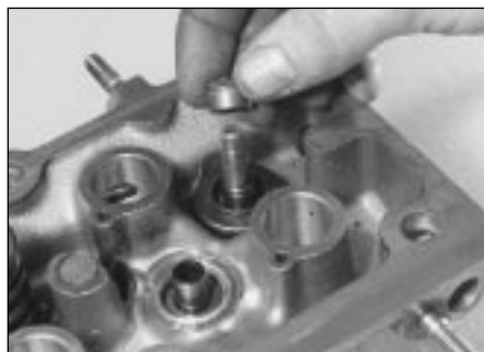
8.2c ... and install the valve stem oil seal
