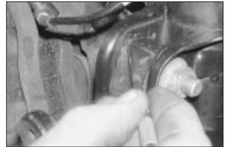
2.7a Mark the top of the steering knuckle in relation to the strut, to retain the camber setting . . .
