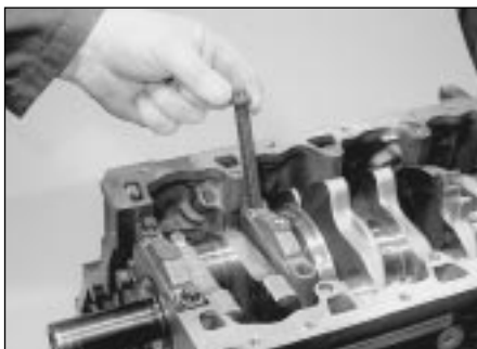
17.21 Lubricate the threads of the new main bearing cap bolts . . .
