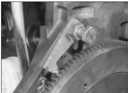
15.2 Lock the flywheel/driveplate ring gear with a tool similar to that shown
