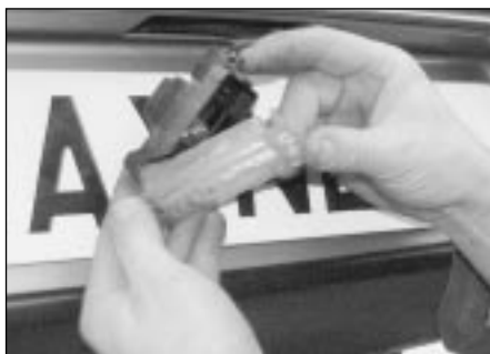
5.44a Unclip the lens from the light unit . . .
