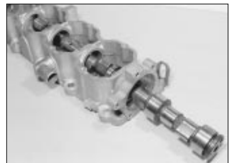
10.4 . . . and slide the camshaft out from the housing
