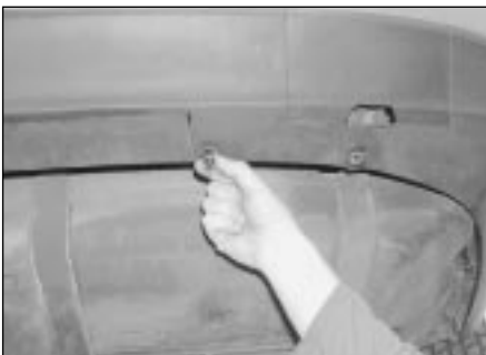
6.9b . . . then prise out the plastic rivets securing the lower edge of the bumper to the rear valance
