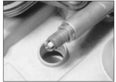
22.10 The multi-electrode plugs fitted as standard should not be adjusted
