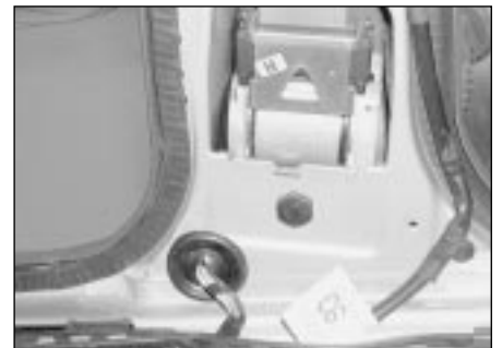
28.7 Inertia reel securing bolt
