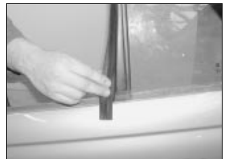
14.23 Peel the weather strip from the rear edge of the door window aperture
