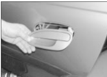
13.15 Withdraw the handle from the door
