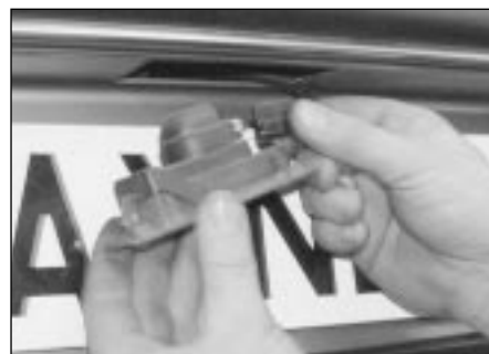
5.43 Depress the clip and remove the light unit from the bumper
