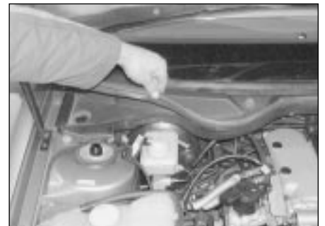
16.2 Release the rubber weatherstrip from the rear of the engine compartment bulkhead
