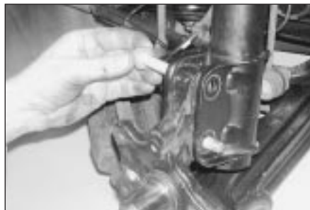
2.7c . . . and withdraw the strut lower securing bolts
