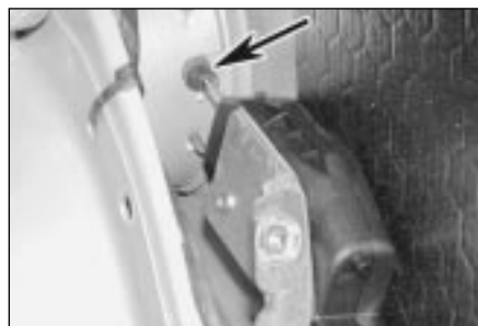
21.17a Ensure that the servo motor locking rod passes through the grommet in the bodywork . . .
