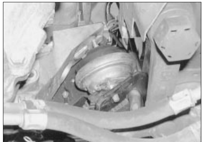
17.8b . . . then lift the engine slightly until there is sufficient clearance to manoeuvre the mounting out of position
