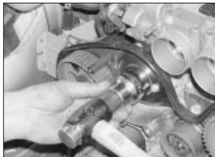
9.4 Tap the new seal into position using a socket which bears only on the seal outer edge as a drift
