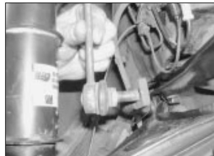
7.2c Detach the drop link from the anti-roll bar
