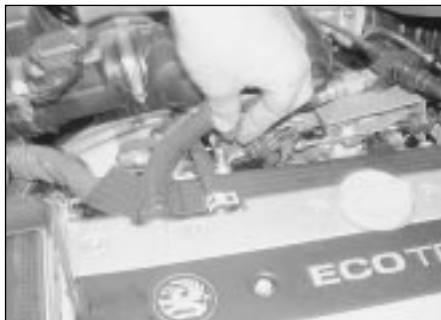
7.2a On 2.0 litre DOHC engines the fuel valve is located on the top of the fuel rail
