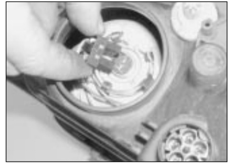
5.14 Unplug the wiring connector from the rear of the bulb
