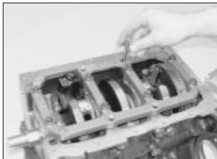
17.38b . . . then refit the bolts securing the casting to the cylinder block . . .
