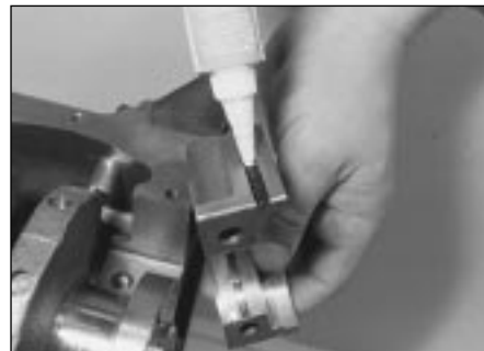
17.20 Fill the side grooves of the rear (number 5) bearing cap with sealant prior to refitting it to the engine
