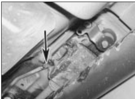
3.3a Release the retaining clips (arrowed) . . .
