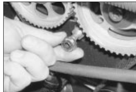
6.4 Ensure the inner rubber spacers are correctly fitted to the mountings before installing the outer cover . . .
