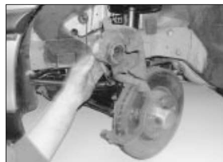
2.13 Pivot the caliper upwards to expose the brake pads
