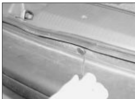
6.18a Prise off the protective caps . . .
