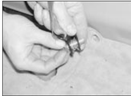
28.1b then slacken and withdraw the bolt and detach the seat belt lower anchor from the sill
