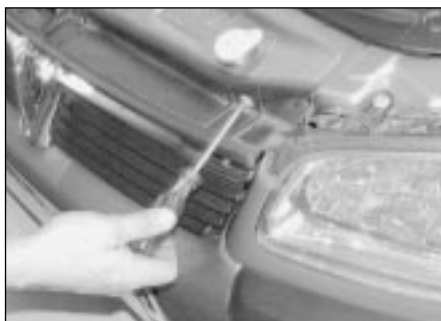
7.1 Slacken and withdraw the radiator grille upper mounting screws
