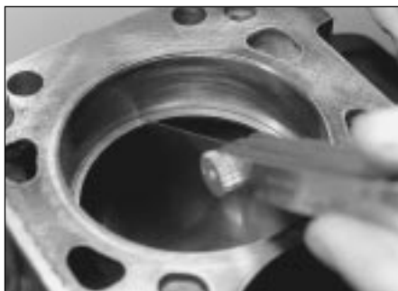
16.4 Measuring a piston ring end gap using a feeler gauge
