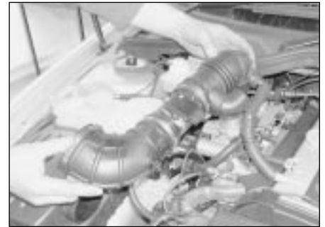
11.12b . . . then release the retaining clips and remove the intake duct assembly from the engine compartment
