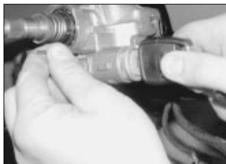
23.5a Depress the recessed locking button with a suitable tool . . .
