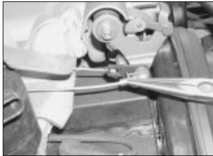
3.1 Remove the retaining clip and detach the inner cable from the throttle cam . . .
