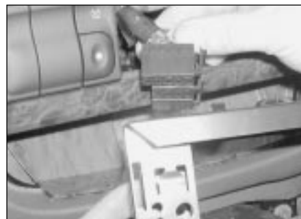
19.4b Disconnect the wiring and aerial connectors from the rear of the radio mounting frame
