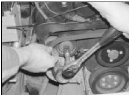
6.12 Lever the tensioner away from the belt then slip the belt off from its pulleys (2.5 litre engine shown)
