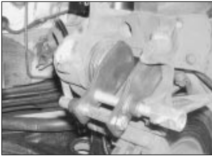
2.18 Using a retraction tool to push the piston back into the brake caliper
