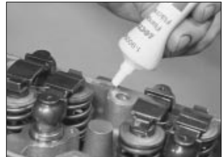
12.25 Apply sealant to the cylinder head upper mating surface then refit the camshaft housing
