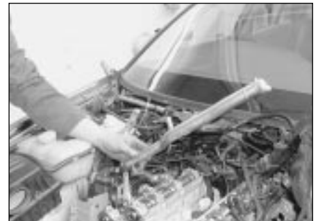
11.28c . . . then undo the retaining bolts and remove the pipe from the engine
