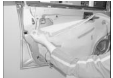
12.10 If necessary, carefully peel the protective plastic membrane from the door
