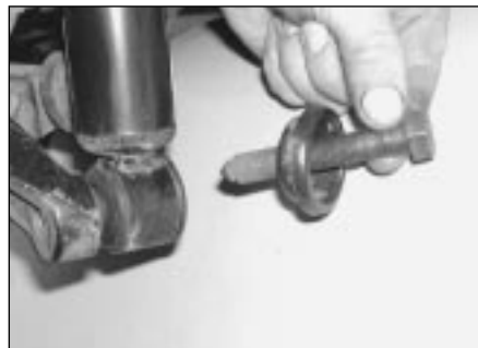
11.7a Unscrew the rear shock absorber lower mounting bolt and washer . . .
