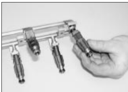
14.4d . . . then ease the injector out from the fuel rail
