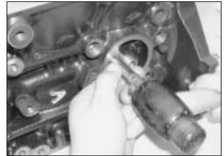
11.16b . . . and tap it fully into position using a hammer and socket
