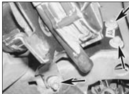
6.5 Undo the retaining nuts (arrowed) and remove the pump and filter assembly from the vehicle
