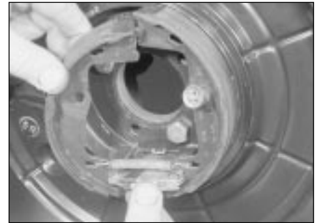
7.18b Engage the bottom of the shoe on the lever . . .
