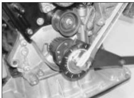
8.18b . . . then tighten it through the specified stage 2 and 3 angles
