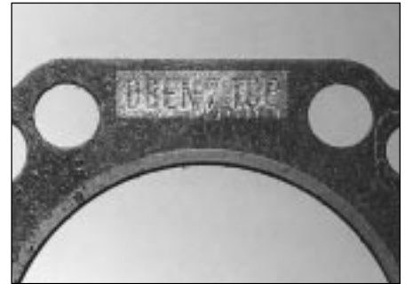
12.22 . . . making sure its OBEN/TOP marking is uppermost
