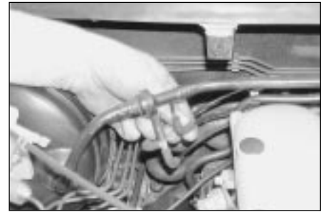
4.27c Disconnect the multi-ram intake system vacuum hoses from the servo unit pipe
