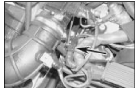
13.52 On later models the crankshaft sensor wiring connector (arrowed) is easily accessible
