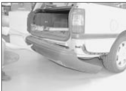
6.19 Carefully withdraw the rear bumper from the rear of the vehicle
