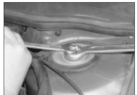
2.8d Counterhold the damper rod with a second spanner to prevent it from rotating
