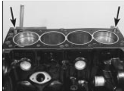
12.21 Fit the new gasket to the cylinder block, engaging it with the locating dowels (arrowed) . . .
