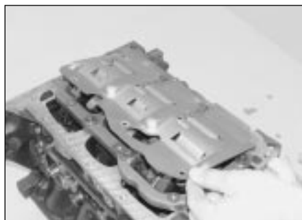
9.3 Removing the baffle plate - 2.5 and 3.0 litre engine
