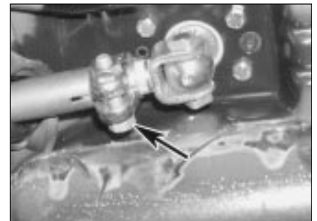
3.3c . . . to gain access to the gearchange linkage clamp bolt (arrowed)
