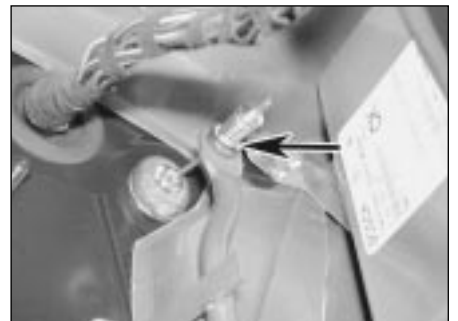
3.5 Unhook the accelerator cable (arrowed) from the upper end of the pedal
