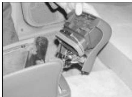
30.4b . . . and detach the rear passenger air vent module (where fitted) from the rear of the console
