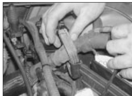
11.15c . . . and free the wiring harness from the relay box
