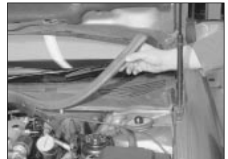
17.2 Carefully peel the rubber beading away from the bulkhead seam
