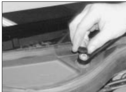
15.2 Prise the cover from the spindle end of the wiper arm
