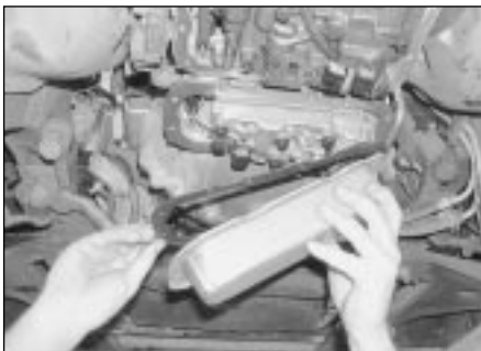
2.10 Refit the intermediate sump using a new gasket
