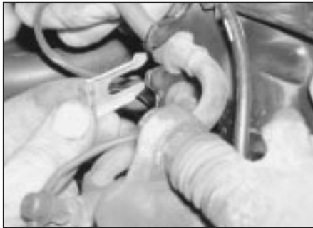
2.4a Pull out the retaining clip . . .
