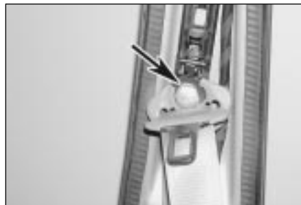
28.6 Slacken and withdraw the bolt (arrowed) and detach the seat belt upper anchor from the adjustment bar slider
