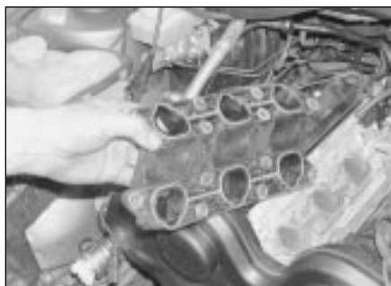
15.43 Removing the manifold flange
