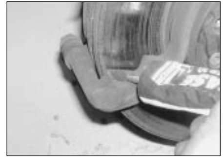
2.19b . . . and the brake pad contact points on the caliper mounting bracket
