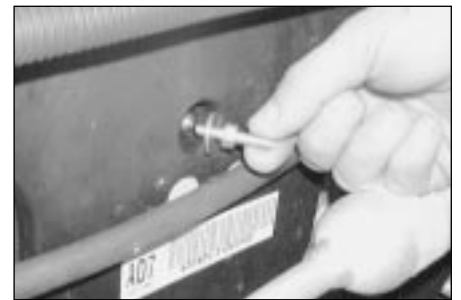
6.3a Slacken and remove the cover retaining bolts (upper bolt shown) and recover the outer rubber spacers . . .
