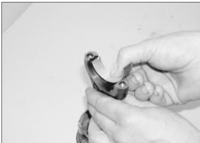
18.3 Fit the bearing shells to the connecting rod and cap making sure their tabs are correctly seated in the cutouts
