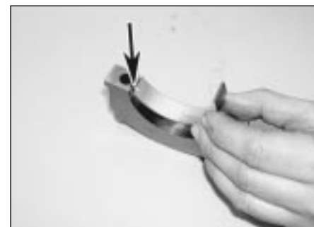
17.3 Fit each main bearing shell making sure its tab is correctly seated in the notch (arrowed)
