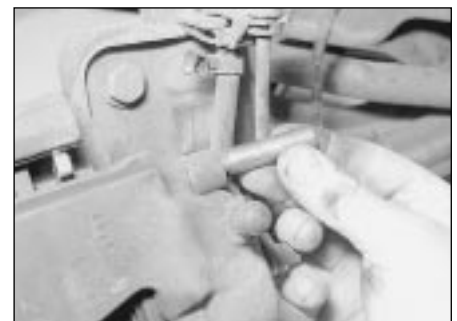
2.8b . . . then slacken and remove the two guide pin bolts
