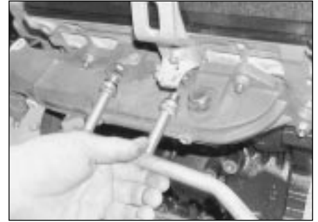
6.47 Removing the right-hand connecting pipe from the manifold
