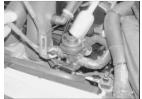
6.28b . . . then release the retaining clips and disconnect the hoses from the cut-off valve
