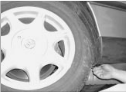
6.7 Unscrew the bolts securing the upper and lower leading edge of the bumper moulding to the bodywork
