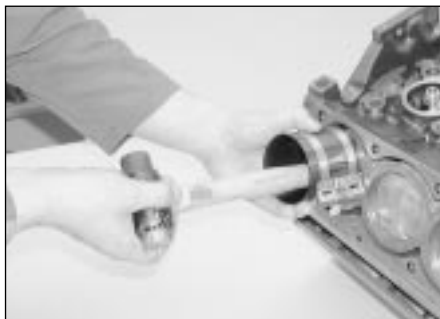
18.9 Insert the piston into the correct bore, tapping it gently into position with the handle of a hammer
