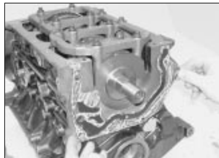
13.19a Locate the pump gasket on the dowels . . .
