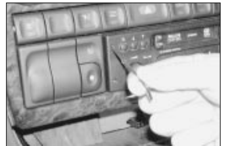
19.1 Using an Allen key, undo the grub screws from the four holes in each corner of the radio
