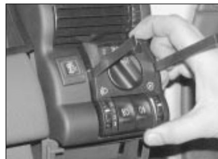
4.12a Depress the locking catches at the side of the switch unit . . .
