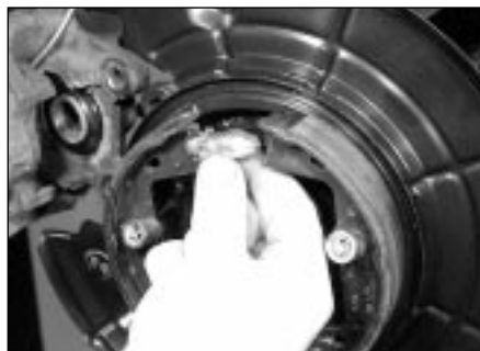
7.20 Refit the adjuster between the upper ends of the shoes
