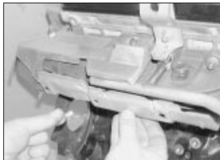
16.26a Undo the retaining bolts and remove the lower . . .
