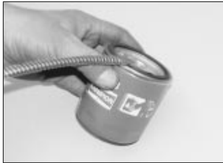
3.11a Lubricate the sealing ring of the new filter with a smear of engine oil . . .
