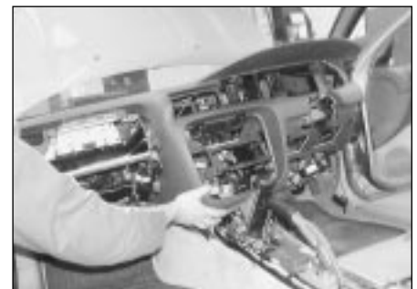
32.34 Carefully withdraw the facia from the bulkhead
