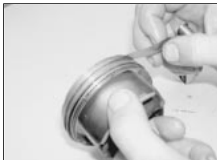
16.11a Checking the piston ring-to-groove clearance using a feeler gauge
