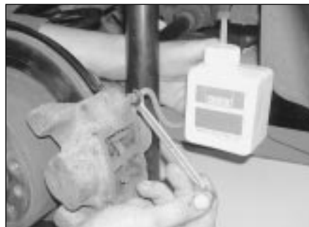
12.14b Fit the spanner over the bleed screw and push the tube onto the bleed screw nipple
