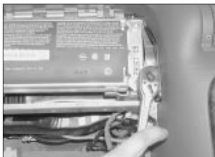
24.20 Slacken and remove the airbag unit securing bolts
