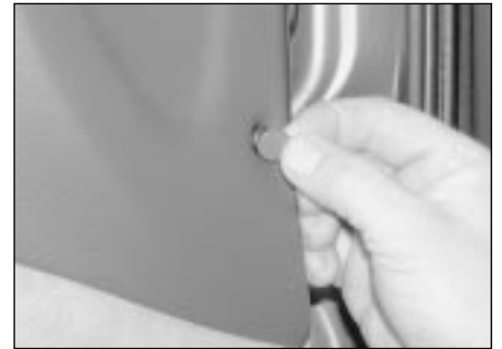
12.8a Prise off the protective caps . . .
