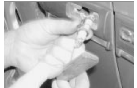
5.32 Hold the bulbholder, then twist the lens to remove it
