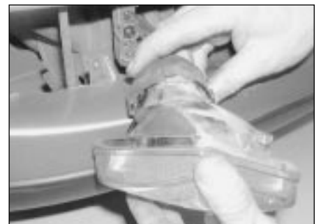
5.28 Rotate the protective cap and remove it from the rear of the foglight
