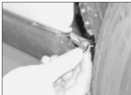
6.16 unscrew the bolts securing the leading edge of the bumper moulding to the bodywork
