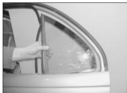
14.29b . . . then slide the glass towards the front of the door and remove it
