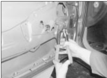
14.9 Use a pop-rivet gun to secure the regulator with new pop rivets
