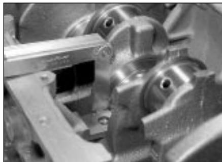
13.3 Using a feeler blade to measure crankshaft endfloat (2.0 litre engine shown)
