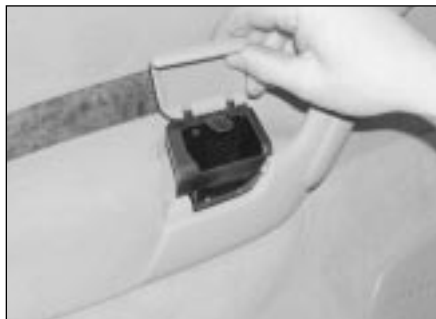
12.13 Use a small screwdriver to carefully prise off the ashtray unit from the armrest
