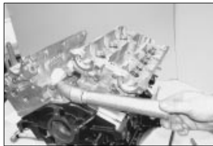
11.20b . . . then remove the coolant pipe from the thermostat housing (shown with engine removed)
