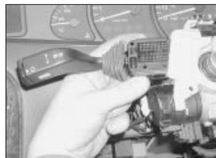
4.5a Depress the upper and lower locking tabs, then carefully slide the switch unit from the top of the housing . . .
