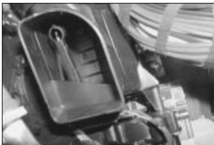
13.46 Location of the ECC right hand vent temperature sensor
