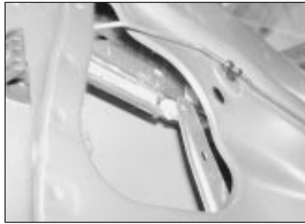
14.7b Slide the arm extensions from the channels at the bottom of the glass
