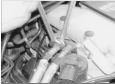
4.27a Slacken the union nuts and disconnect the fuel hoses from the fuel rail
