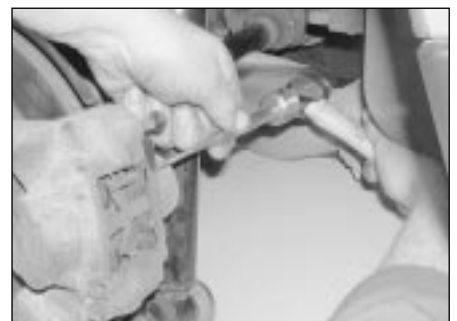
3.12 Drive the brake pad securing pins in from the inner surface of the caliper
