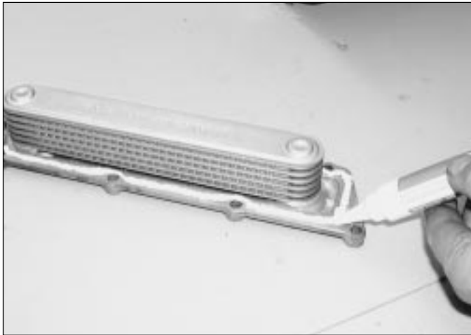
14.14 Apply a bead of sealant to the groove in the oil cooler cover
