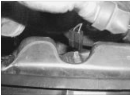
18.5 Disconnect the wiring from the top of the pump and position to one side
