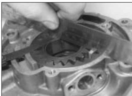
14.13b Using a straight edge and feeler blade to measure gear endfloat
