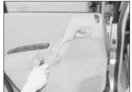
12.17a Unscrew and remove the door pull handle retaining screws . . .
