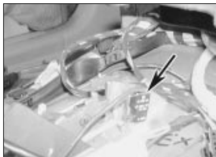
8.35 Selector lever pawl switch - later models
