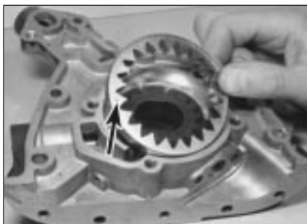
14.10 Lift the inner and outer gears (arrowed) out from the pump housing
