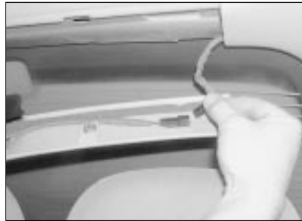
5.50 Unplug the wiring at the connector
