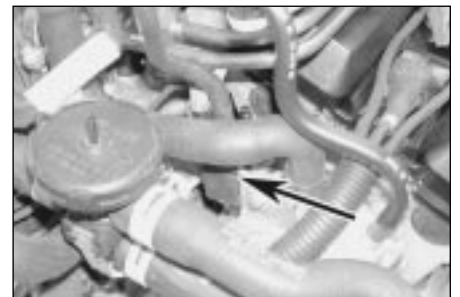
4.19 On 2.5 and 3.0 litre engines the purge valve (arrowed) is mounted on the rear of the right-hand cylinder head (shown with engine removed)
