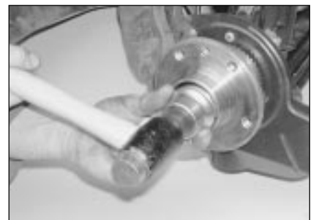
9.8 Carefully drive the hub onto the stub axle using a suitable socket
