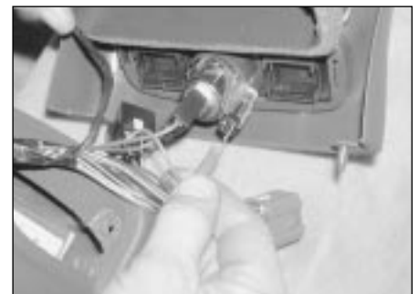
30.4c Unplug the wiring at the connector(s)
