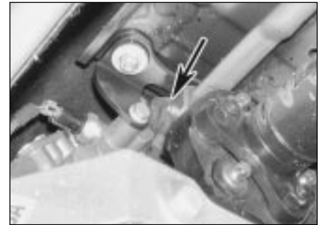
4.9 Slacken and remove the nut and pivot bolt (arrowed) securing the linkage rod to the transmission unit
