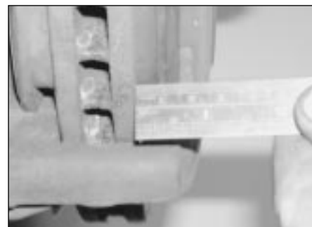
2.15 Measuring the thickness of a brake pad
