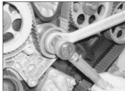
7.19 Remove all slack from the top run of the belt then hold the upper pulley stationary and tighten its retaining bolt to the specified torque
