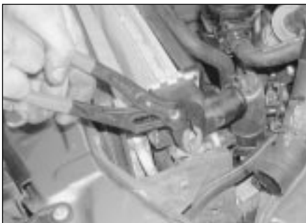
2.10a Release the spring clips at the top of the radiator ...
