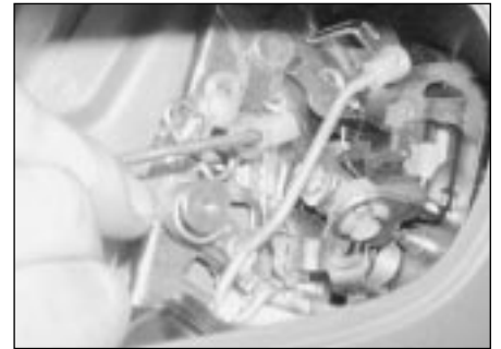
13.34 Disconnect the locking knob and interior handle link rods from the lock by releasing the plastic clips
