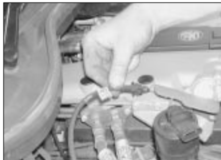
15.32c . . . and free the cruise control cable from the throttle cam and bracket
