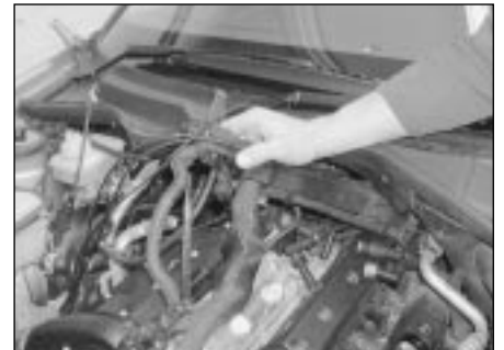
11.16d Once all the wiring has been disconnected, position the harness clear of the cylinder head
