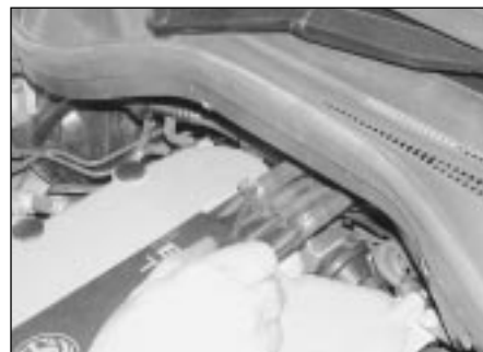
15.37 Release the retaining clips and disconnect the vacuum and breather hoses from the rear of the manifold
