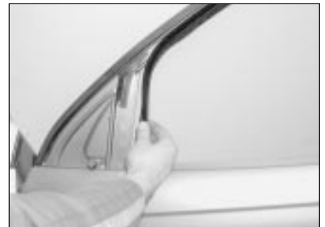
14.15 Peel the weather strip from the front edge of the door window aperture
