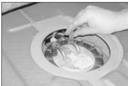
8.6 Release the retaining clips and disconnect the fuel hoses from the pump cover
