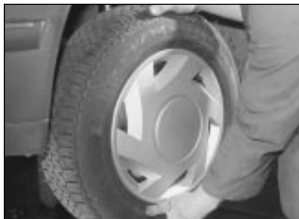
10.4 To check for play in the wheel bearing, grasp the roadwheel at the 12 o'clock and 6 o'clock positions, and try to rock it
