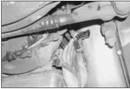
9.16 Disconnect the wiring connectors from the transmission unit and free the wiring from its retaining clips
