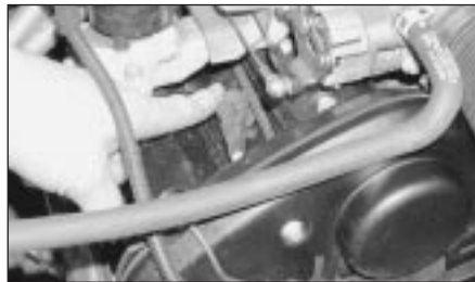
B Check that the spark plug HT leads are securely connected by pushing them onto the plugs (where accessible)
