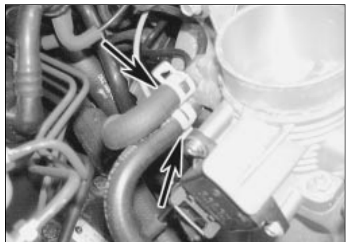
11.15 Release the retaining clips and disconnect the coolant hoses (arrowed) from the throttle housing
