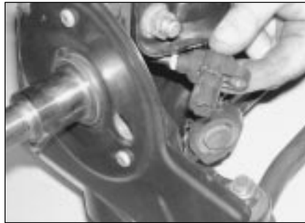
18.46b . . . and withdraw the ABS sensor
