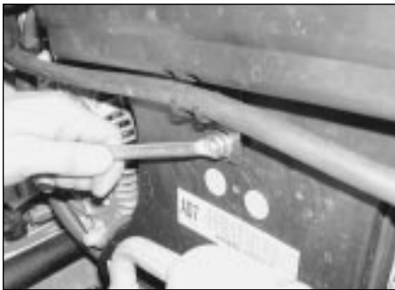
6.2a Undo the retaining nut and free the wiring tray from the outer cover . . .
