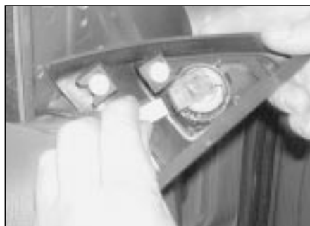
20.6 Unplug the wiring from the loudspeaker
