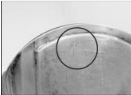
12.20a Ensure the piston and connecting rod are assembled so the arrow on the piston crown (circled) is pointing away from . . .
