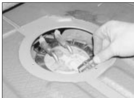
8.5 . . . then disconnect the wiring connector from the fuel pump cover
