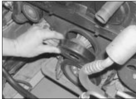
6.4b . . . and remove the pulley from the engine
