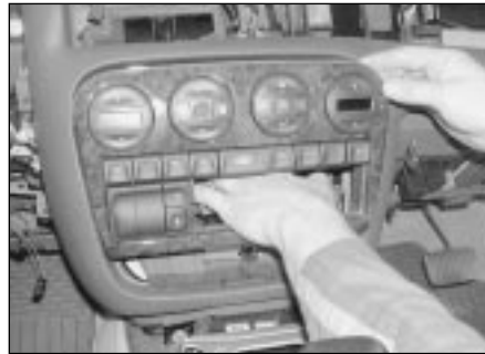
13.5a Reach through the radio aperture . . .
