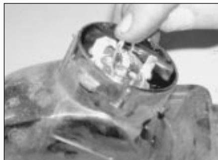
5.29b . . . then release the spring clip . . .
