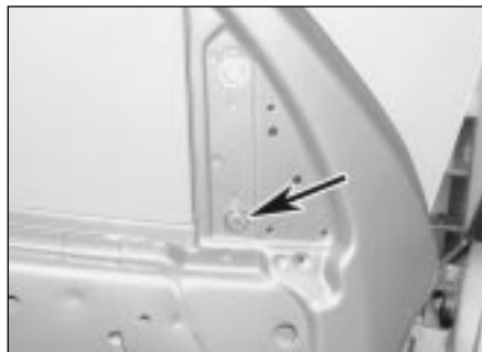
14.17a Slacken the window guide channel upper . . .
