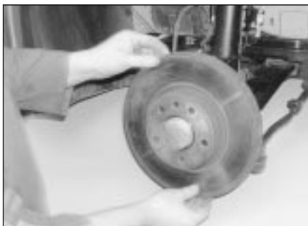
6.8b . . . then withdraw the front brake disc from the hub
