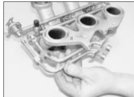
14.3c . . . and remove the fuel pipes from the manifold
