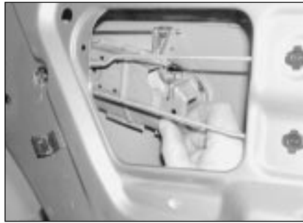
13.13b . . . and remove the mounting plate from the rear of the exterior door handle
