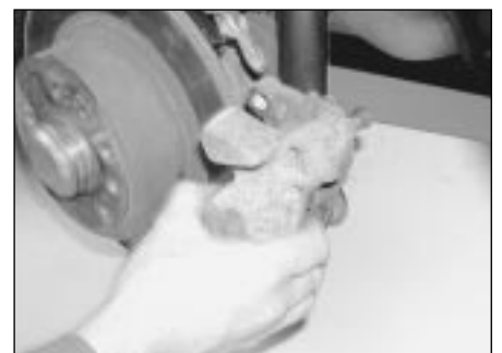
5.5b . . . and withdraw the caliper from the semi-trailing arm
