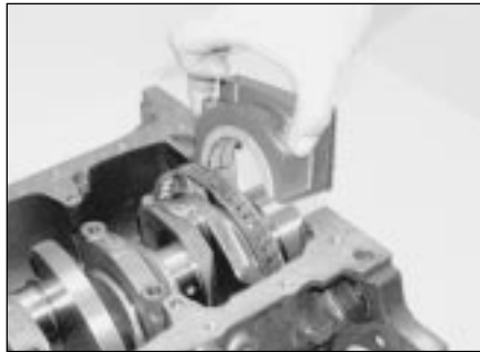
17.31b . . . then refitting it to the cylinder block
