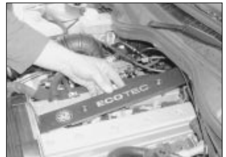
22.2 On 2.0 litre DOHC engine remove the spark plug cover to gain access to the plugs
