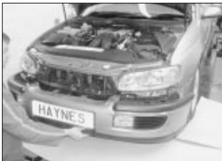
6.4b ... then carefully withdraw the front bumper from the front of the vehicle
