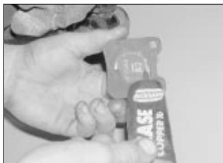
3.10 Apply a little high-melting point grease to the top and bottom edges of the backplates on the brake pads
