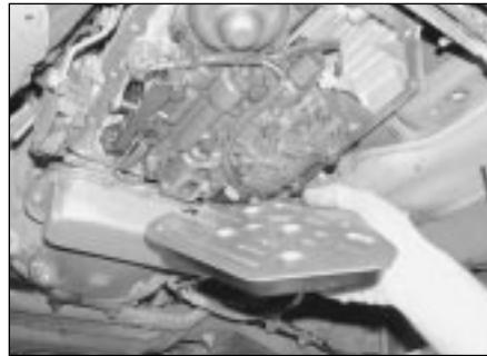
2.7b . . . and remove the fluid filter from the transmission unit
