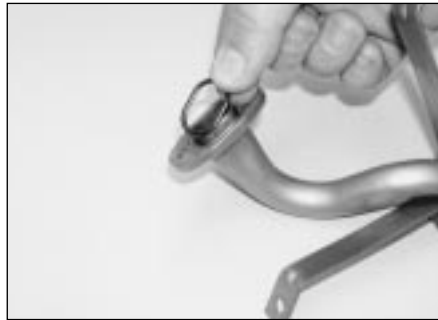
12.16 Fit a new sealing ring to the oil pump pick-up/strainer before refitting
