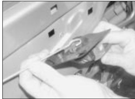
13.3 Twist the handle anticlockwise to unhook it from the link rod
