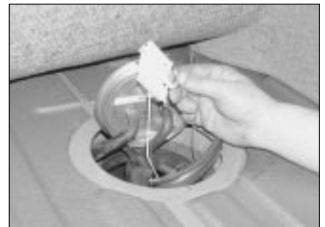
9.3 Removing the fuel gauge sender unit
