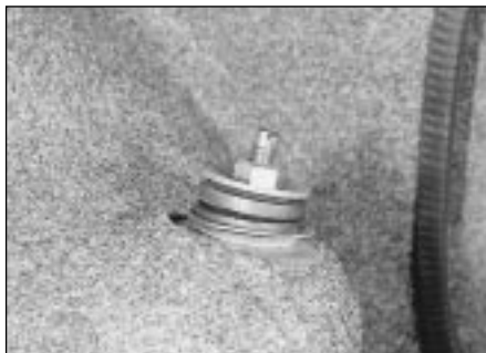
11.5 Unscrew the rear shock absorber upper mounting nut
