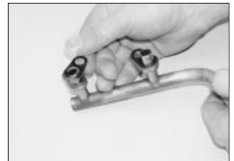
6.43 On refitting, ensure the mating surfaces are clean and dry and fit new gaskets to the connecting pipe
