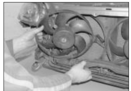
3.21b . . . then withdraw the fan and motor from its housing
