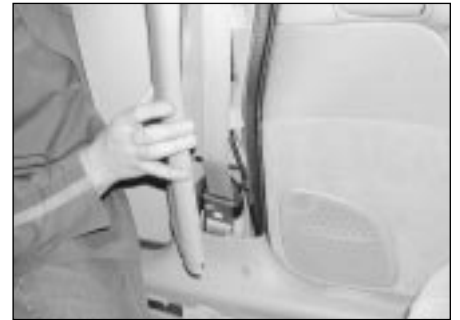
28.2 Unclip and remove the B-pillar lower trim panel
