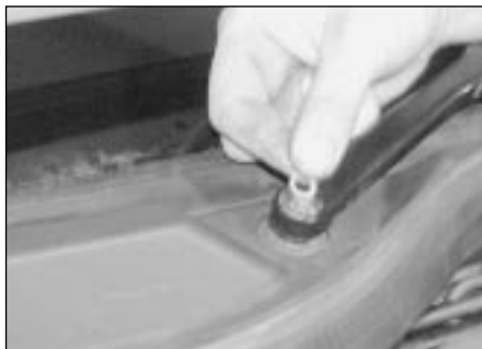
15.3b . . . and recover the small washer
