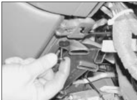
3.4b Prise out the centre pin then remove the fastener outer section . . .
