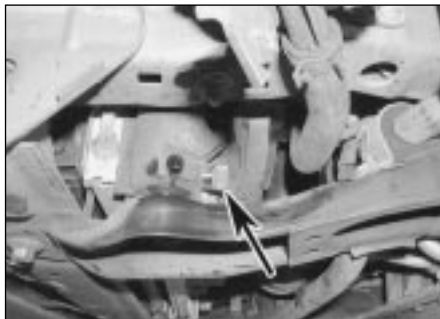
28.3 Open the drain plug at the base of the radiator (arrowed)
