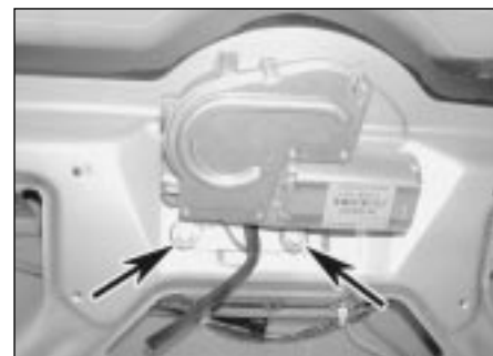
17.6 Unscrew the mounting bolts (arrowed) and withdraw the wiper motor
