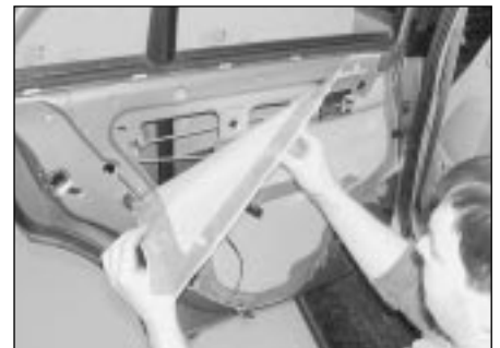
12.21 If necessary, carefully peel the protective plastic membrane from the door
