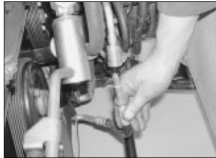
4.30c . . . and at the front of the engine (quick-release fitting pipes shown)
