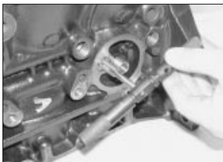
11.3a On 2.5 and 3.0 litre engines cut an M10 thread into the oil bypass valve . . .
