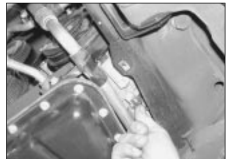
4.30a On models with air conditioning disconnect the wiring connector from the compressor . . .
