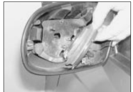
23.12b . . . and withdraw the servo motor from the mirror housing
