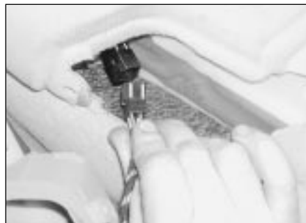
12.17c Where applicable, unplug the window switch wiring connector
