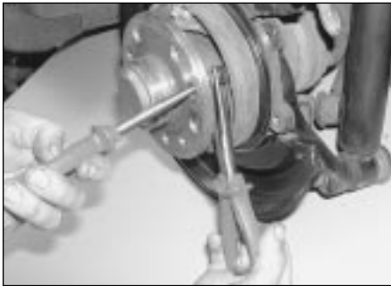
7.7 On later models, where the retaining pins are not cross-headed, depress the spring cups and turn them through 90° using two pairs of pliers
