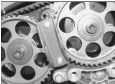
7.4d . . . making sure their TOP markings are uppermost
