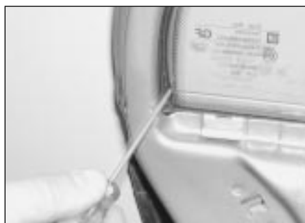
14.29a Carefully prise the rubber seal away from the window aperture . . .
