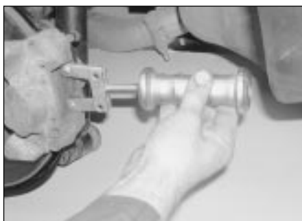
3.6b . . . or a pad extraction tool . . .
