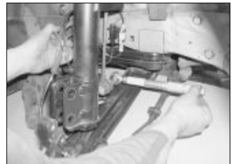
7.2d Counterhold the drop link stud using the flats provided
