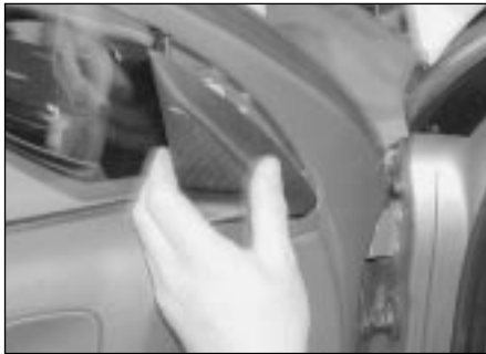
23.1a Carefully prise off the triangular plastic cover panel at the rear of the mirror mountings . . .
