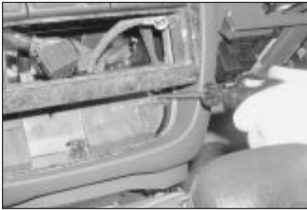
13.4 Slacken and remove the securing screws from the lower edge of the ECC panel
