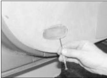
6.14 Carefully lever the light unit from the door trim panel
