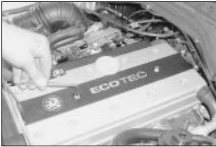
22.17 On 2.0 litre DOHC engines refit the spark plug cover and securely tighten its retaining screws
