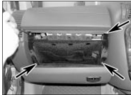
31.4 Undo the glovebox mounting screws (arrowed)
