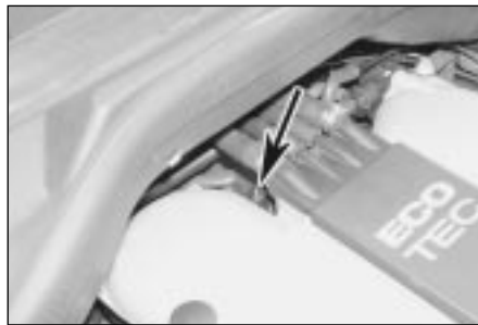
7.2b On 2.5 and 3.0 litre engines the fuel valve (arrowed) is located at the rear of the inlet manifold
