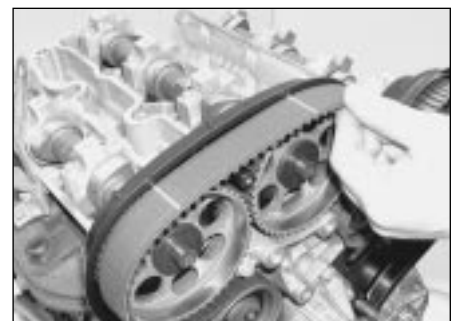
7.16a On engines with a modified tensioner, work around in a clockwise direction and engage the belt first with the right-hand cylinder head sprockets . . .
