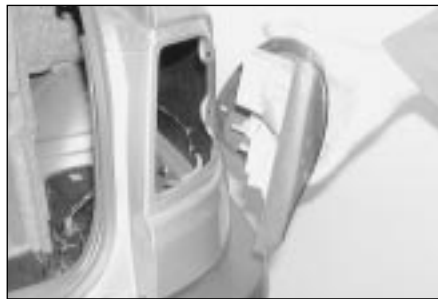
7.18c . . . and withdraw the light cluster from the rear of the vehicle (saloon models) . . .
