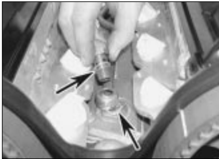
11.27b . . . then remove the union bolts and sealing washers (arrowed) and free the pipes from the oil cooler
