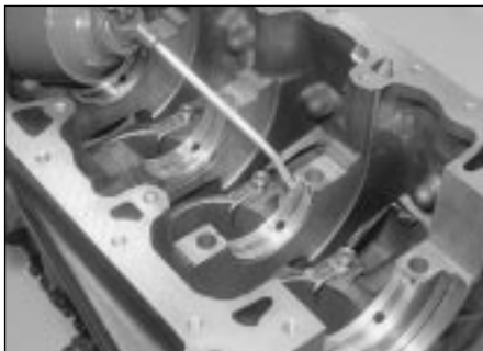
17.17 Lubricate the upper bearing shells with clean engine oil then lower the crankshaft into position
