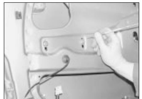
14.6 Mark the position of the regulator guide rail mounting bolts then unscrew and remove the bolts
