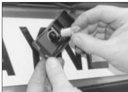
5.44b . . . then depress and twist the bulb from its contacts
