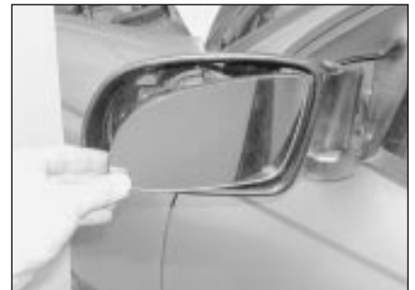
23.8 Unclip the mirror glass from its mountings
