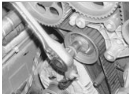
7.5a Slacken the tensioner pulley retaining nut . . .
