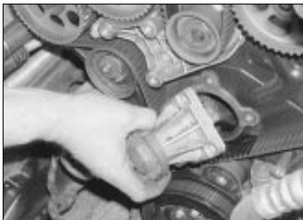
5.10a Lift the coolant pump away from the engine . . .
