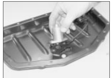
14.10 Removing the oil level sensor (2.5 litre engine shown)
