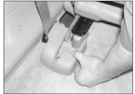
27.2b . . . and detach the plastic end cap from the outer seat runners
