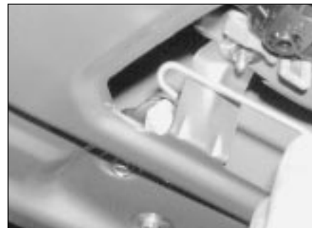
21.7 Disconnect the central locking link rod from the servo motor
