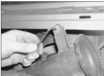
3.18 Undo the securing screws and detach the air intake duct from the crossmember
