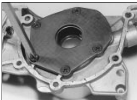
14.8 Undo the retaining screws and remove the oil pump cover
