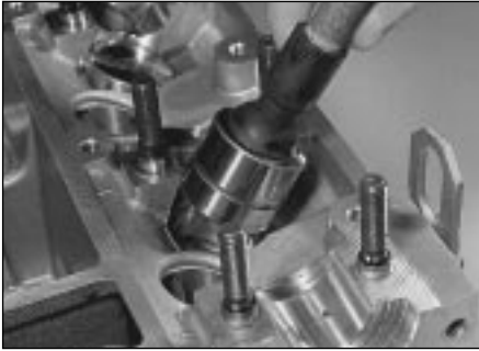
10.6 Using a rubber sucker to remove a camshaft follower
