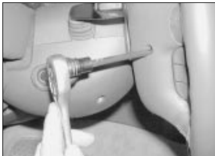
24.8a Unscrew and remove the two screws from the rear of the steering wheel . . .
