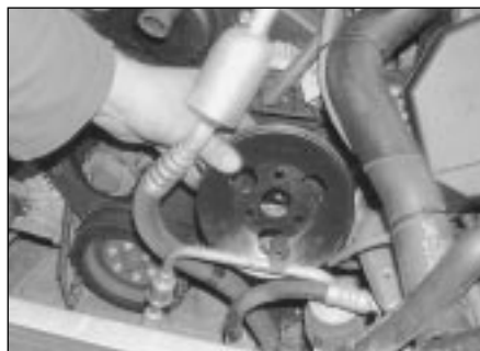
6.5b . . . and remove the pulley from the pump
