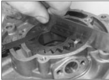
13.12b Using a straight edge and feeler blade to measure gear endfloat
