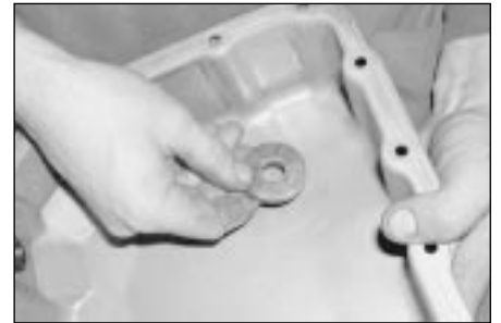
2.8 Clean all traces of metal fillings from magnet which is fitted inside the main sump
