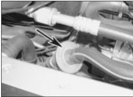
6.18 Release the retaining clip and disconnect the air hose from the non-return valve (arrowed)
