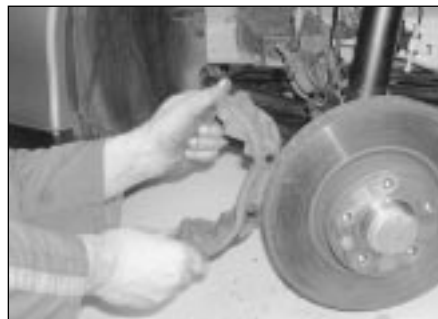
4.9b . . . then detach the caliper mounting bracket from the hub carrier
