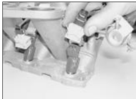
14.2a Disconnect the wiring connectors from the injectors . . .
