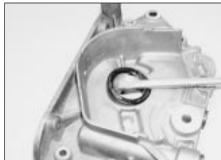
13.16a Lever out the oil seal out from the pump with a large flat-bladed screwdriver . . .
