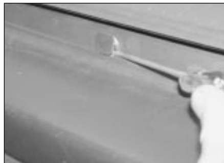
6.10 Prise off the protective caps and remove the screws securing the upper edge of the bumper moulding to the bodywork
