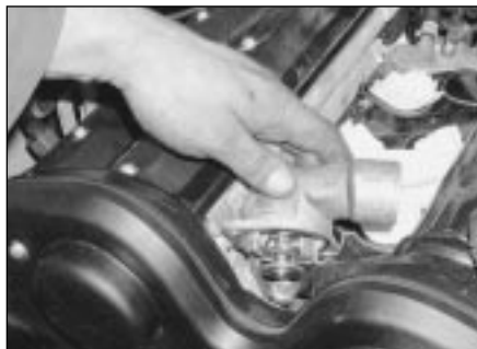
4.11 Unscrew the bolts, then remove the cover and integral thermostat
