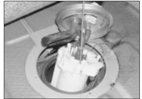
8.9a Release the retaining clips and withdraw the pump housing assembly from the tank with a piece of welding rod
