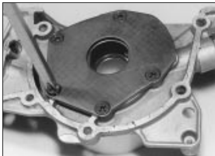
13.7 Undo the retaining screws and remove the oil pump cover
