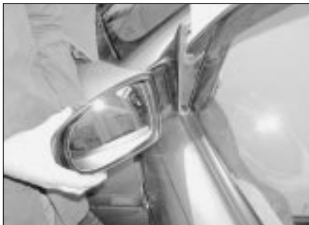
23.5b . . . and lift the mirror from the door
