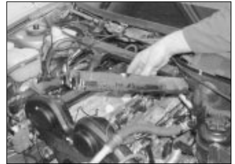
4.8 Removing the left-hand camshaft cover
