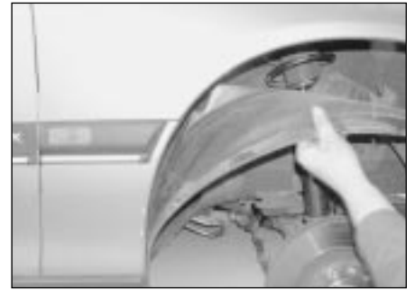
4.2c . . . and remove the right-hand front wheelarch liner
