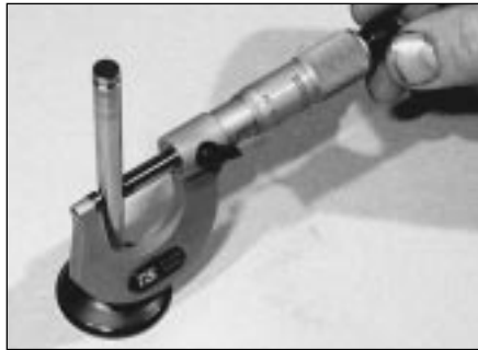
7.12 Using a micrometer to measure valve stem diameter
