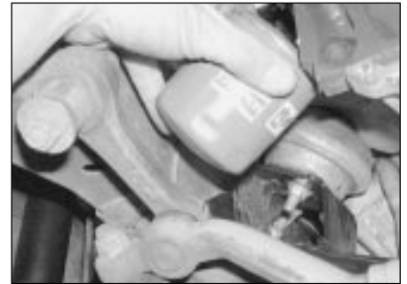
3.11b . . . then screw the filter on by hand only (2.5 litre engine shown)
