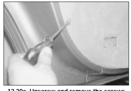
12.20a Unscrew and remove the screws from the rear and lower edges of the trim panel . . .
