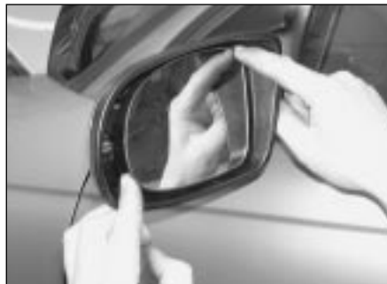
23.7 Gently press the upper inner corner of the glass inwards so that the lower outer corner protrudes from the mirror housing
