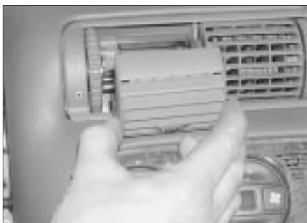
32.22a Carefully prise the two nozzles from the centre air vent housing . . .
