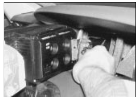
9.7 Disconnect the wiring from the rear of the multi-function display unit
