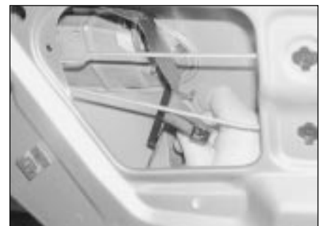
13.12b . . . and remove the plastic security panel from the door lock mechanism
