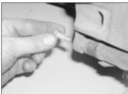
2.12b . . . and withdraw the guide pin bolt from the caliper
