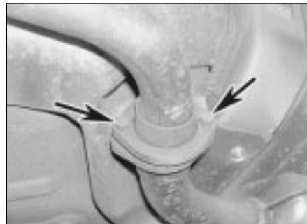
18.9 Front pipe-to-intermediate pipe bolts - 2.0 litre DOHC engine
