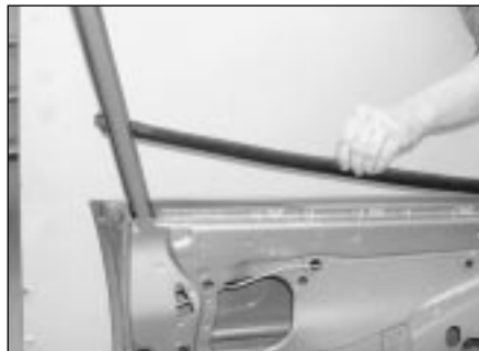
14.14 Remove the sealing strips from the inside and outside of the lower edge of the door window aperture
