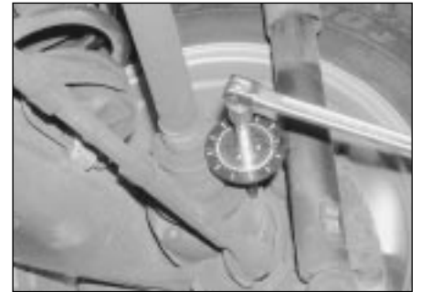
8.9b . . . then angle tighten to the specified second and third stages
