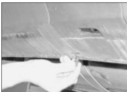
6.17b . . . then prise out the plastic rivets securing the lower edge of the bumper to the rear valance
