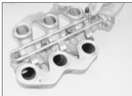
14.4b . . . and ease the fuel rail and injector assembly out of position
