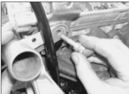
11.20a Slacken and remove the retaining bolt and spacer . . .
