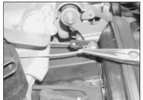
15.32a Remove the retaining clip and detach the accelerator inner cable from the throttle cam
