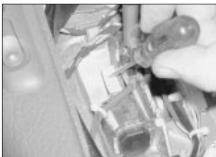
30.11 On automatic models, it may be necessary to release the gear selector from the PARK position, by depressing the yellow release lever, to allow the removal of the console from the floorpan
