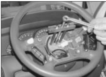
21.16b If necessary, use a proprietary steering wheel puller to assist removal
