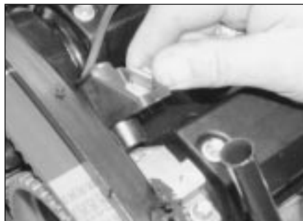
14.46 Removing the camshaft sensor
