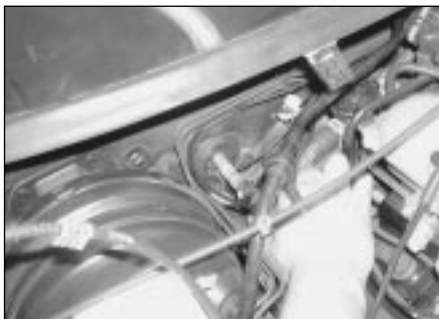
4.29a Pull back on the locking collars and detach the heater matrix coolant hoses from their unions on the bulkhead . . .
