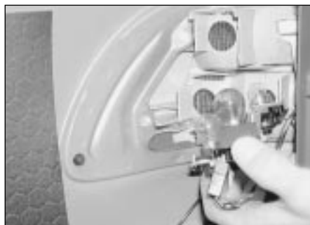
5.36 Withdraw the bulbholder from the rear light
