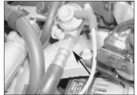
13.16b . . . and the fuel return pipe union nut
