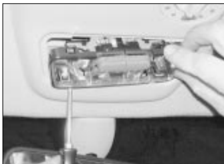
25.17a Remove the lens, then unclip the interior lamp unit from the console . . .
