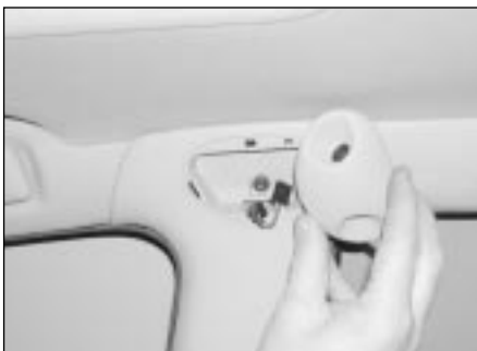
28.3 Unclip the alarm system interior sensor unit from the B-pillar upper trim panel . . .
