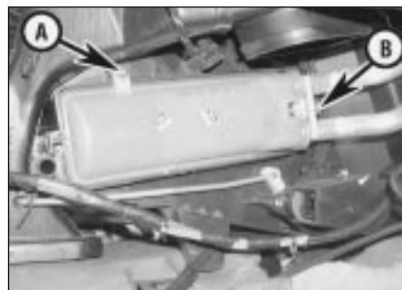
9.9 Heater matrix securing screw (A) and coolant pipe retaining plate bolt (B)
