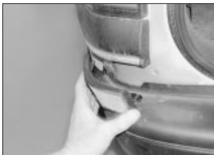
6.15 Unscrew the securing bolts and remove the reflectors from the underside of each rear light unit
