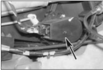
13.32 Unclip the cover panel to expose the right hand vent servo motor
