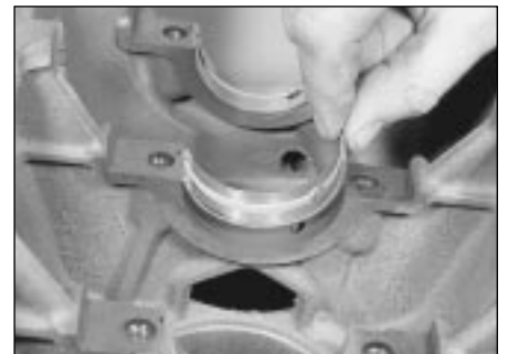
10.9 . . . and lift out the upper main bearing shells from the cylinder block
