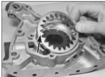
13.9 Lift the inner and outer gears (arrowed) out from the pump housing
