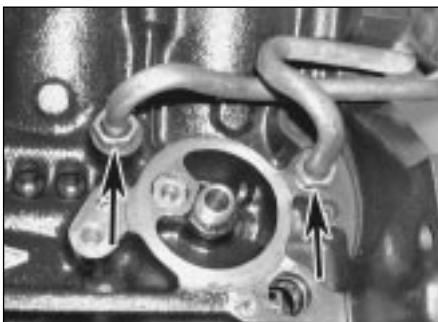
14.8a Slacken the union nuts (arrowed) securing the oil pipes to the block . . .
