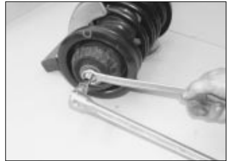
2.12a Hold the piston rod stationary with an Allen key . . .
