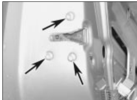
13.36a Unscrew the lock mechanism mounting screws (arrowed) . . .
