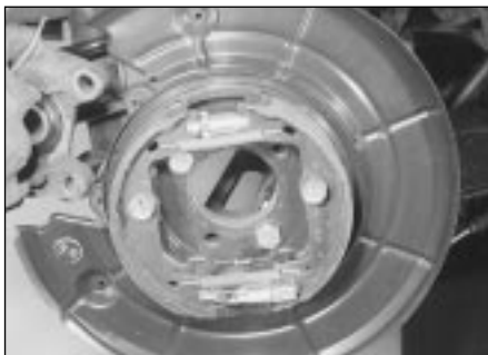
7.22 The handbrake shoes assembled ready for refitting of the rear hub
