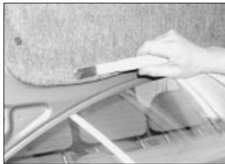
18.1a Prise carefully using a forked tool to release the press-stud fixings . . .
