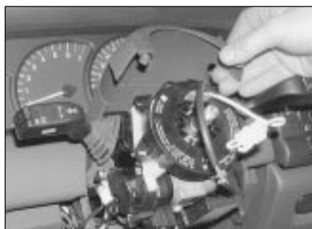
4.4e . . . and upper sections of the shroud panels from the steering column
