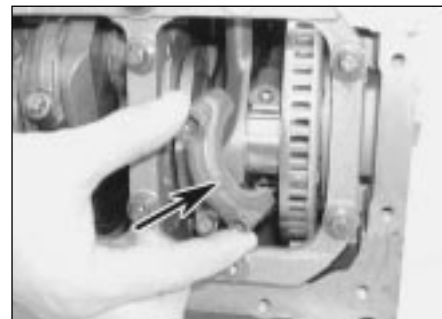
18.12a Refit the bearing cap making sure the lug is facing towards the flywheel/driveplate end of the engine . . .
