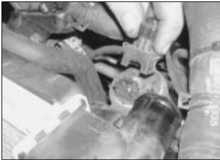
2.5c ... and auxiliary coolant pump
