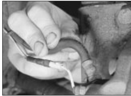
7.16 Inspecting the flexible hose connection to a front brake caliper
