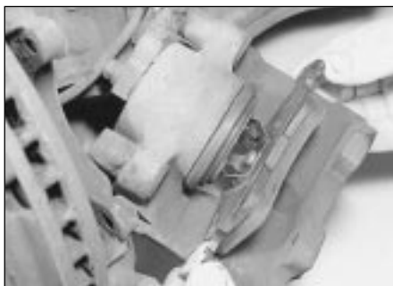
2.11 Carefully prise the inner pad from the caliper piston
