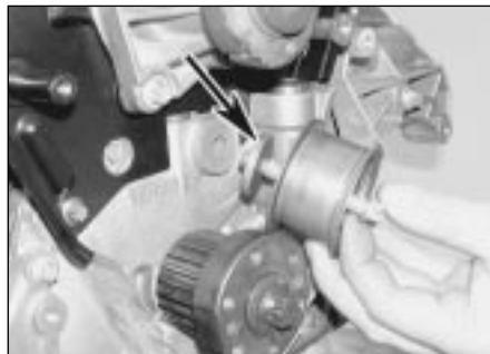
8.25 Unscrew the retaining bolt and remove the lower guide pulley and its spacer (arrowed) from the engine
