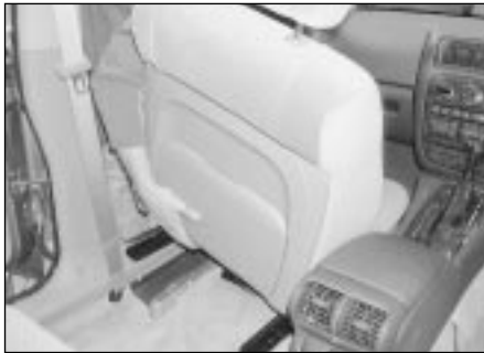
27.6b ... and remove the front seat from inside the vehicle
