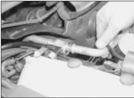
4.30b . . . and separate the air refrigerant pipes at the unions above the left-hand cylinder head . . .
