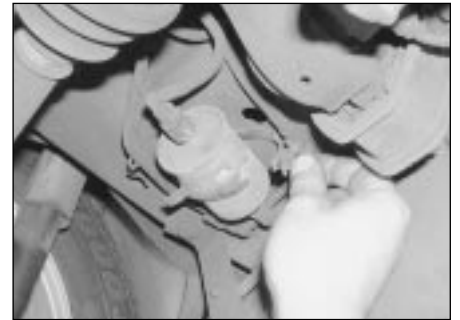
23.4 Release the retaining clip and free the fuel filter from the body
