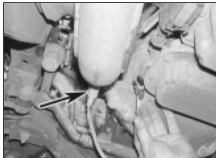
3.3 Disconnect the wiring connector then unscrew the oxygen sensor (arrowed) from the front pipe (2.5 litre engine shown)
