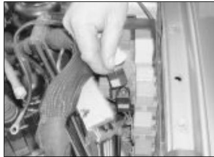
4.6b . . . and disconnect the engine wiring harness connector from the relay box
