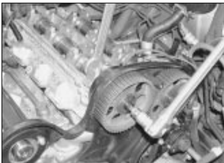
8.2b If the camshaft cover has been removed, the camshaft can be held with an open-ended spanner on the flats provided
