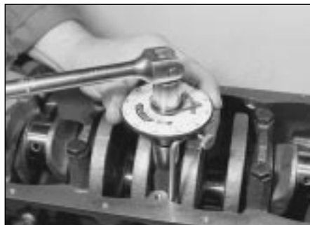
17.23 . . . and then through the specified stage 2 and 3 angles
