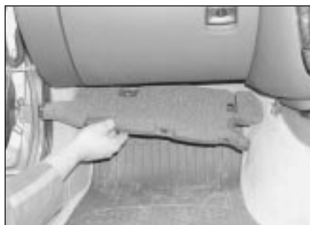
31.2 Release the press-stud clips and detach the trim panel from the underside of the fascia
