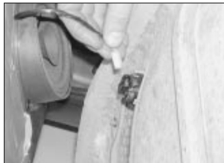
12.20c Unplug the speaker wiring as it becomes accessible
