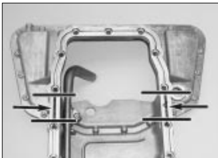
12.23 Apply a bead of sealant (arrowed) to the main casting seal groove in between the lines shown . . .
