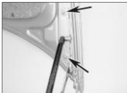
17.3 Unscrew the nuts (arrowed) that secure boot lid to the hinges
