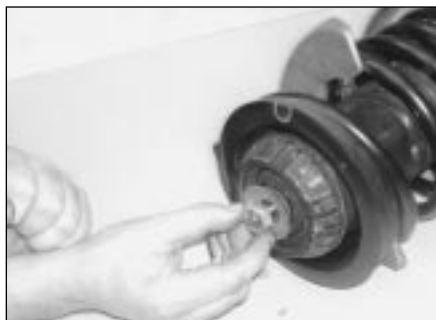
2.12b . . . then unscrew the damper rod nut . . .
