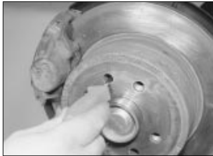
9.6 Adjusting the handbrake screws using a screwdriver through the hole in the disc/hub flange
