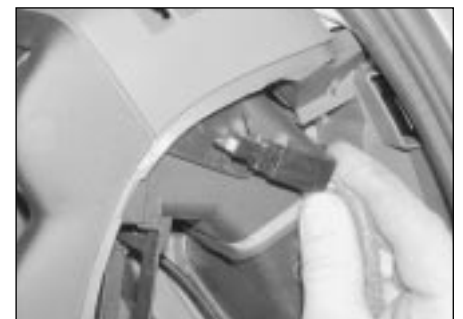
32.13 Unclip the bulb holder from the rear of the air vent housing
