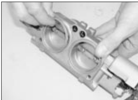
11.21 On refitting, fit new sealing rings to the throttle housing recesses
