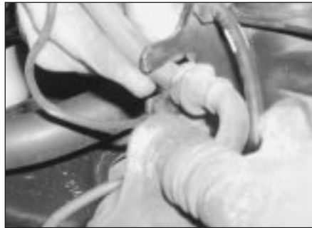
2.4b . . . and disconnect the hydraulic hose from the bracket on the strut
