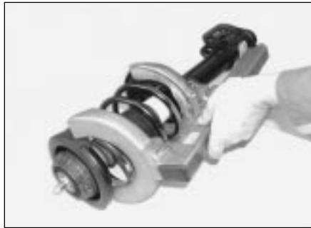
2.11 Fitting the spring compressor to the strut coil spring
