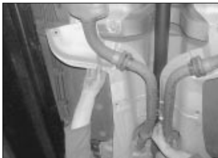
10.2 Remove the exhaust heat shields from the vehicle underbody
