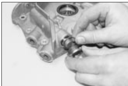
13.11a Slacken and remove the oil pressure relief valve bolt and sealing washer . . .
