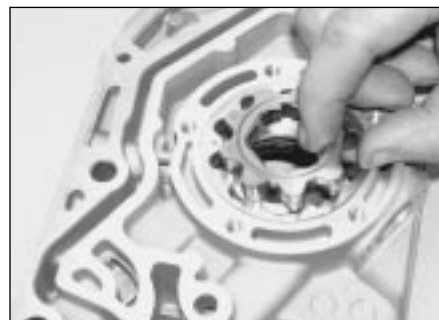
13.10 . . . then lift both rotors out of the housing
