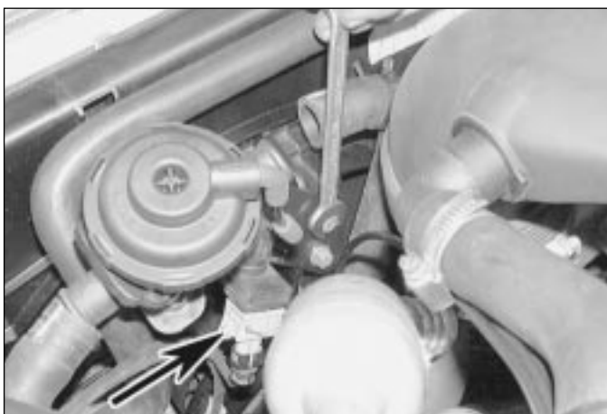
6.29 Undo the retaining bolts and disconnect the wiring connector (arrowed) then remove the bracket assembly from the vehicle
