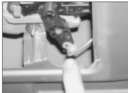
18.2 Disconnect the lock link rods from the rear of the lock assembly
