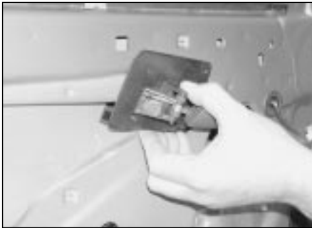
13.2 Press the interior handle forwards to release it from the elongated slots in the door panel
