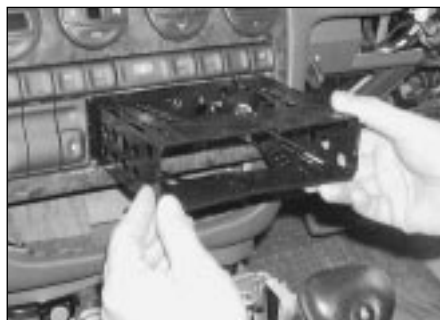
19.4a If required, bend back the securing tabs and release the mounting frame from the fascia
