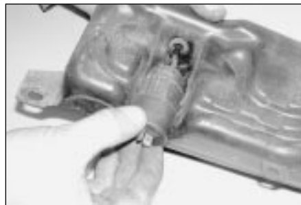
18.16 Pull the pump body to extract it from the reservoir grommet (shown with reservoir removed for clarity)
