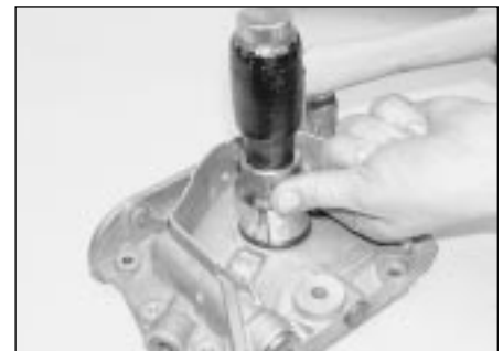
13.16b . . . and tap the new seal squarely into position, using a socket which bears only on the seal outer edge
