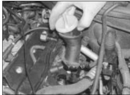
4.7b . . . and rotate the oil filler neck anti-clockwise to free it from the left-hand camshaft cover
