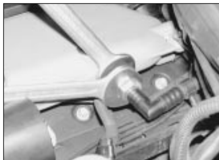
15.36 Unscrew the union nut and disconnect the braking system servo unit hose
