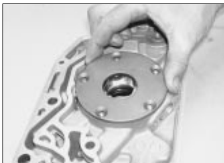
13.8 Undo the retaining screws and remove the cover from the oil pump
