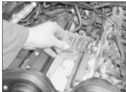
14.9b . . . then undo the retaining bolts and lift off the oil cooler cover
