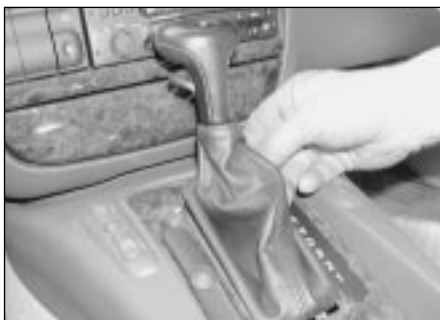
1.0a On later models, to release the selector lever from the P position with the battery disconnected, unclip the selector lever gaiter . . .
