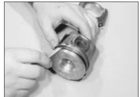
12.2 Using a feeler blade to remove a piston ring
