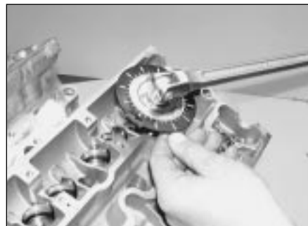
11.42 . . . and then through the specified stage 2 to 5 angles using an angle measuring gauge for accuracy
