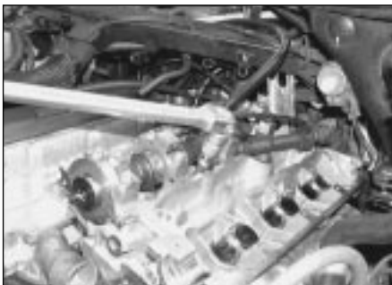
11.23 Evenly and progressively slacken and remove the cylinder head bolts . . .
