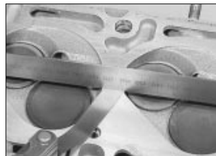
7.6 Checking the cylinder head surface for distortion
