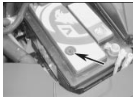
3.5 Standard Vauxhall battery with built-in charge indicator (arrowed)
