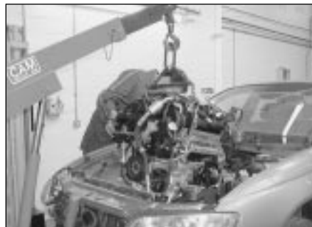
4.35 Lifting the engine unit out of position
