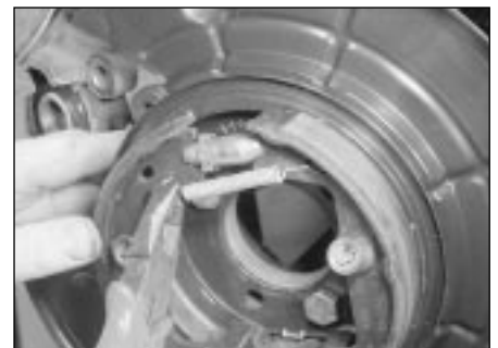
7.21 Hook the upper return spring on the shoes
