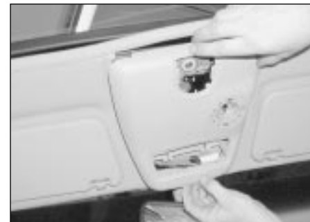
25.20b . . . then detach the console from the roof
