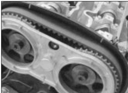
7.18a Remove all slack from the left-hand run of the belt by rotating the lower guide pulley whilst making sure the sprocket timing marks remain in alignment (timing gauge shown) . . .
