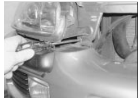
6.4a Unscrew and remove the upper mounting bolts ...
