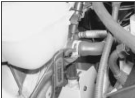
4.28a Disconnect the engine coolant hoses from the expansion tank . . .
