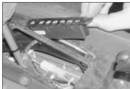
30.6a On automatic models, prise the gear position indicator module . . .
