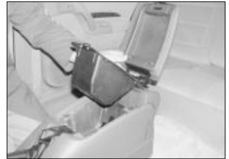
30.2b . . . and withdraw the storage box moulding from the console
