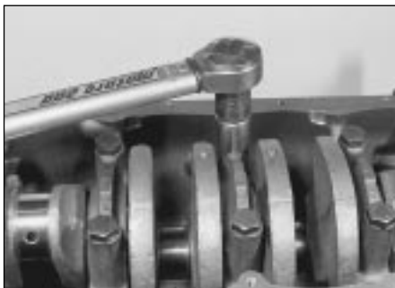
17.22 . . . then tighten the bolts to the specified stage 1 torque setting . . .
