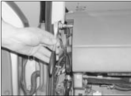
24.18a Using a long extension bar and a pair of long nosed pliers, slacken . . .
