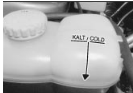
28.18 Slowly fill the system via the expansion tank filler neck, until the coolant level again reaches the KALT/COLD mark on the side of the expansion tank
