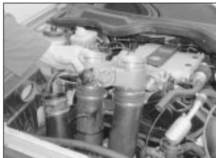
17.25 Removing the pre-volume chamber assembly
