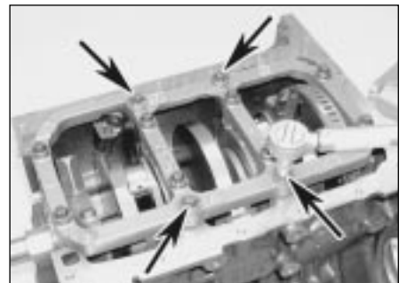
17.38c . . . and tighten them (arrowed) to their specified torque setting
