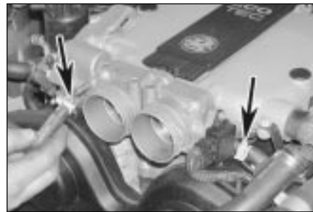
15.33 Release the retaining clips and detach the coolant hoses (arrowed) from the throttle housing
