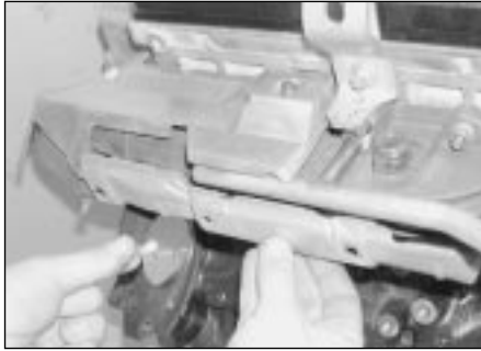
6.45a Undo the retaining bolts and remove the lower . . .
