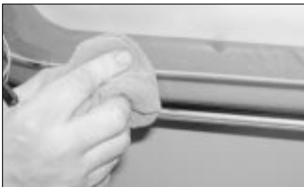
12.11 On models fitted with side airbags, it is important that the sealing strip around the edge of the membrane adheres to the door without gaps, to form an airtight seal
