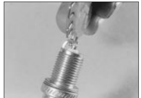
22.13 . . . and if necessary adjust the gap by bending the electrode
