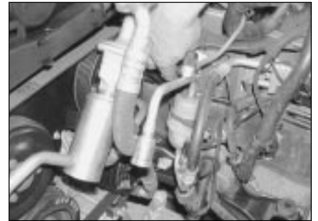
4.30d Release the receiver/drier damper mounting bracket and position the damper clear of the engine
