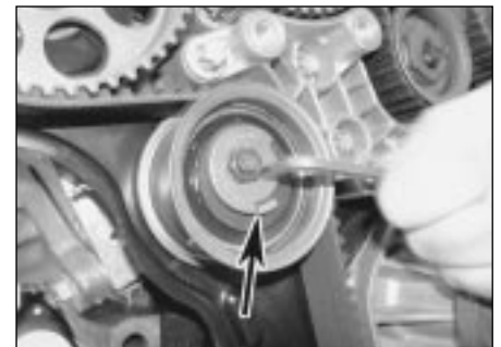
7.20 Rotate the tensioner pulley anti-clockwise until the gap (arrowed) is 0.5 to 1.5 mm then securely tighten its retaining nut
