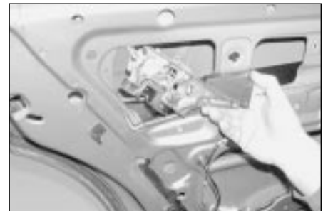
13.36b . . . and withdraw the lock mechanism through the exterior handle door aperture
