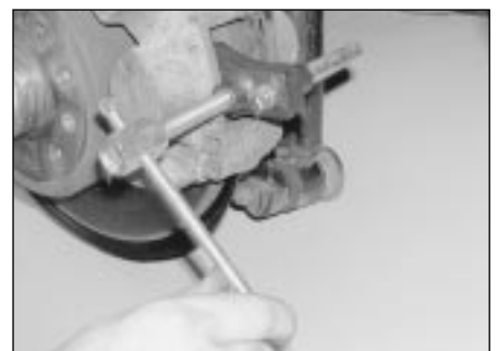
3.8 Using a retraction tool to press the pistons back into the caliper body
