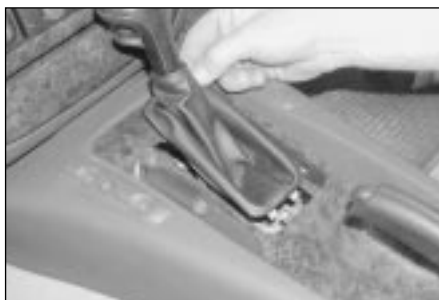
30.5 Unclip the gear lever gaiter from the console and fold it up over the gear lever knob
