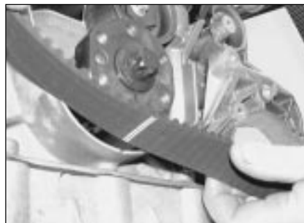
7.13a Align the double line on the timing belt with the crankshaft sprocket timing mark
