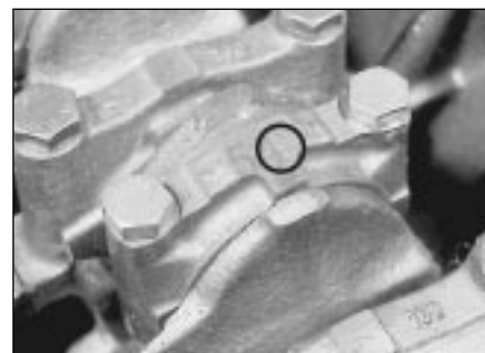
9.5 Make identification markings on the connecting rods and bearing caps (circled). Note that the lug on the bearing cap faces towards the flywheel/driveplate end of the engine
