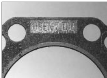
11.20 . . . making sure its OBEN/TOP marking is uppermost
