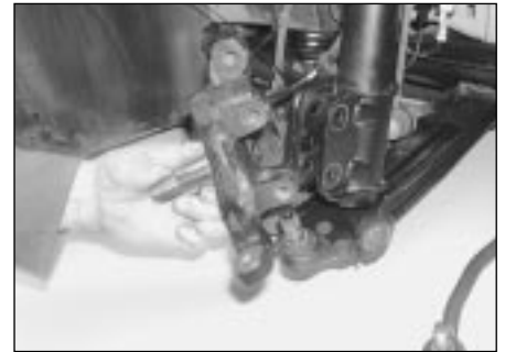
8.6b . . . and then lift the knuckle from the lower arm
