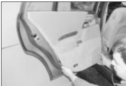
12.20b . . . lift the panel upwards to disengage it from the door, then remove it from the vehicle
