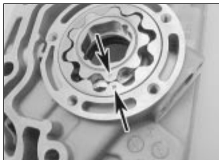
13.9 Note the identification markings (where present) on the pump rotors . . .
