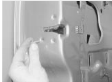
13.30 Unscrew and remove the front door lock retaining screws
