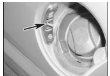
21.17b . . . and engages with the filler flap lock plate
