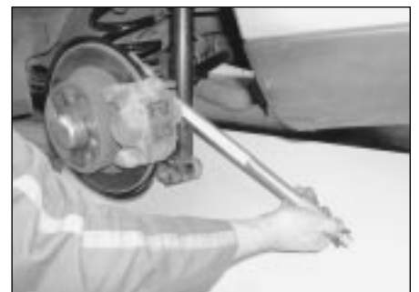
5.16 Tighten the caliper mounting bolts to the specified torque
