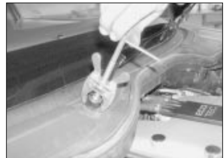
15.4b Using a proprietary puller to draw the wiper arm from its shaft
