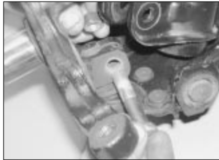
8.6a Unscrew and remove the pinch-bolt . . .
