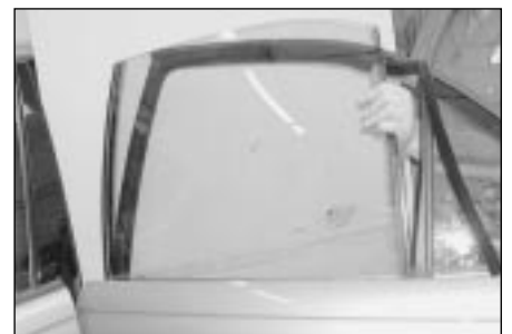
14.25 Slide the window glass to the top of the door, then tilt its upper corner forward to disengage it from the door and remove it
