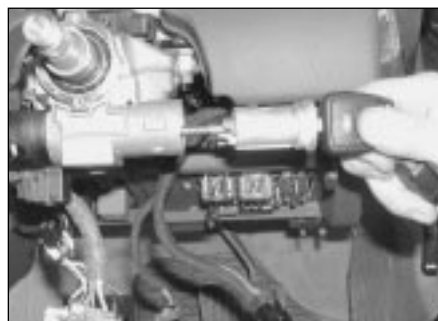
23.5b . . . and withdraw the lock cylinder, together with the key from, from the housing
