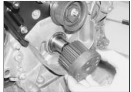
8.14b . . . then slide off the crankshaft sprocket . . .
