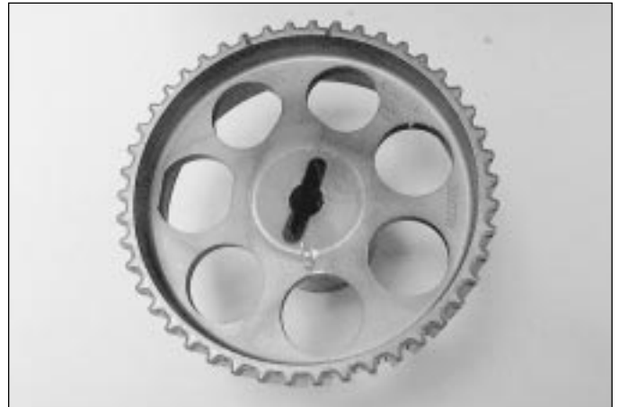
8.7b Left-hand cylinder head camshaft sprocket. Ensure timing mark and slot 3 are used on the inlet camshaft and 4 on the exhaust camshaft
