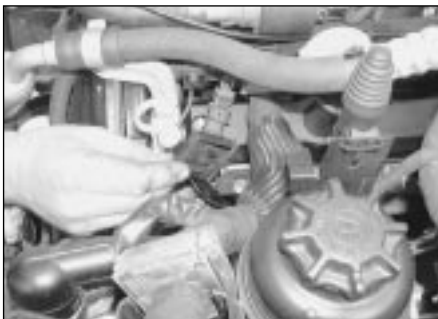
4.31 Remove the covers from the engine lifting brackets and attach the hoist
