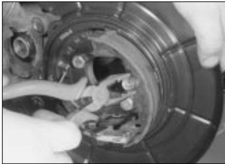
7.17c . . . and use a pair of pliers to depress and turn the cup
