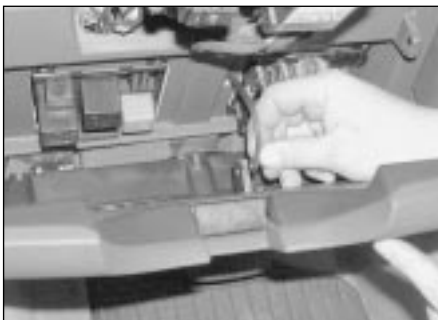
32.9a Open the fusebox cover and unhook the check strap from it
