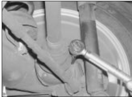
8.9a Tighten the driveshaft mounting bolts to the specified first stage torque . . .
