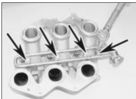
14.4a Undo the retaining bolts (arrowed) . . .
