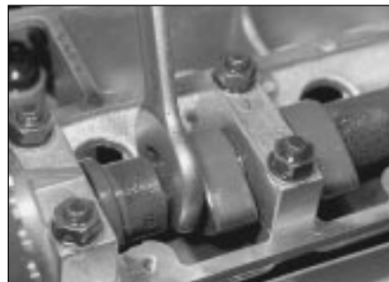
8.2 Using an open-ended spanner to retain the camshaft sprocket whilst the sprocket bolt is slackened
