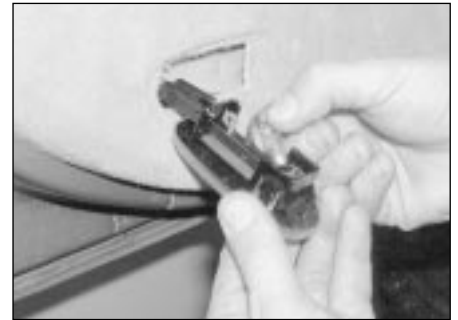
6.15b . . . then remove the bulb from the spring contacts
