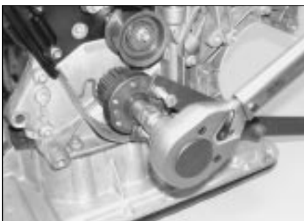
8.18a Tighten the crankshaft sprocket bolt to the specified stage 1 torque setting . . .
