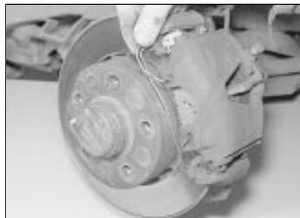
2.24 Refit the caliper spring, ensuring that its ends are firmly pressed into the holes in the side of the caliper body
