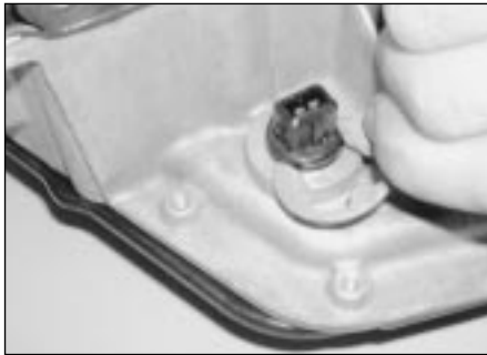
12.4 Slide off the retaining clip and push the oil level sensor wiring connector into the sump
