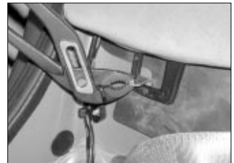
27.14 Bend up the metal securing tabs to release the seat back side cushions
