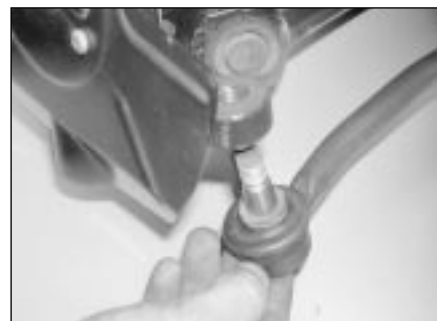
25.2c . . . to separate the tie rod from the steering knuckle
