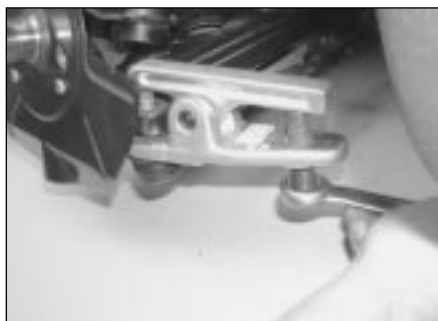
25.2b . . . and use a proprietary balljoint removal tool . . .
