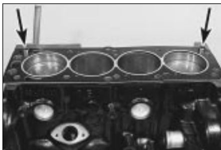
11.19 Fit the new gasket to the cylinder block, engaging it with the locating dowels (arrowed) . . .
