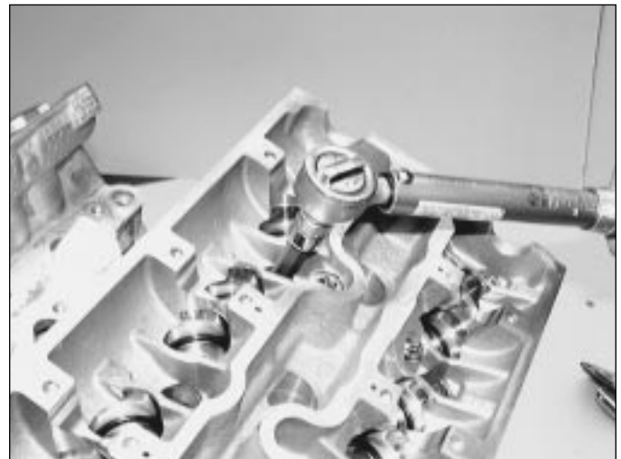
11.41b Working in the specified sequence, tighten the cylinder head bolts to the specified stage 1 torque . . .
