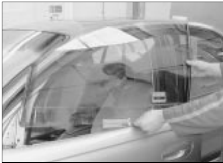
14.18 Tilt the window glass upper corner forward to disengage it, then remove it from the door
