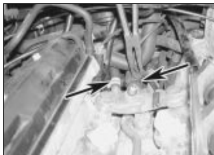
11.6 . . . then release the retaining clips and disconnect the coolant hoses from the outlet elbow
