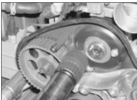
9.2a Carefully drill/punch holes in the oil seal . . .
