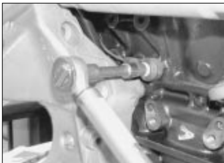
14.43 On refitting ensure the knock sensor is correctly positioned then tighten its retaining bolt to the specified torque
