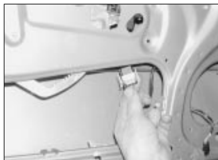
14.5 On models with electric windows, unplug the winder motor wiring at the connector
