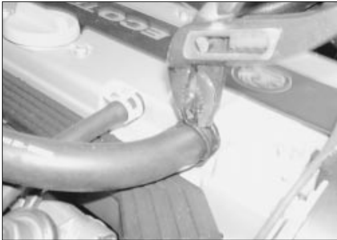
7.3a ... then disconnect the breather hose from the camshaft cover ...
