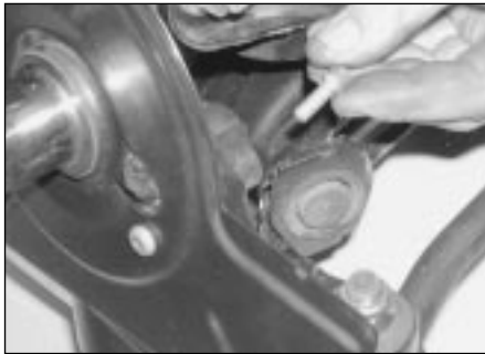
18.46a Unscrew the mounting bolt . . .
