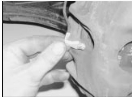
2.5 Unclip the pad wear sensor from the caliper aperture
