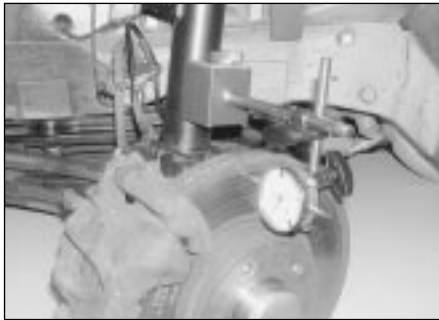
6.4 Checking the front brake disc runout
