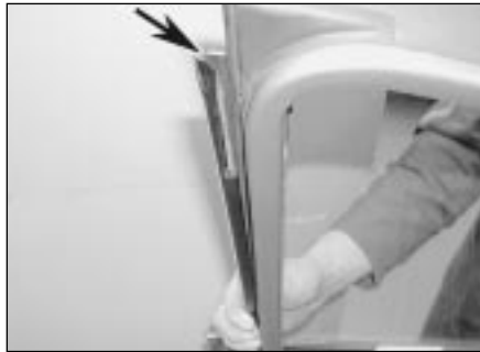
14.19a Ensure that the channel (arrowed) at the trailing edge of the glass engages with the rear edge of the door
