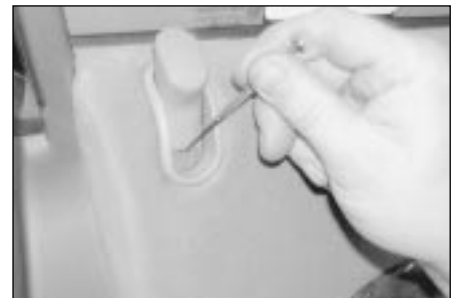
12.7a Prise the clip from the door locking knob and then detach the knob from the locking rod
