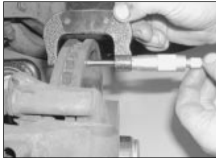
6.6 Checking the thickness of the front brake disc using a micrometer
