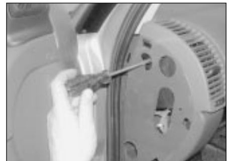
32.19a Slacken and withdraw the securing screws . . .
