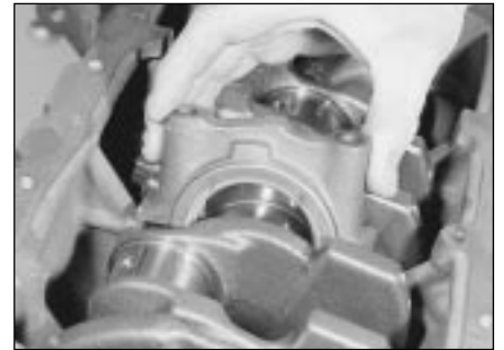
10.7 Removing the centre (No 3) main bearing cap. Note the thrust flanges incorporated into the bearing shell
