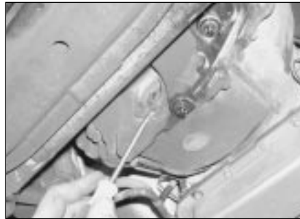
9.21a Prise out the cover from the sump flange . . .
