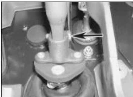
22.2 Unscrew and remove the upper clamp bolt (arrowed) to separate the inner section of the steering column from the flexible joint
