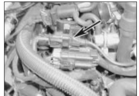
14.29 The crankshaft sensor wiring connector (arrowed) is clipped onto the engine rear lifting bracket (shown with engine removed)
