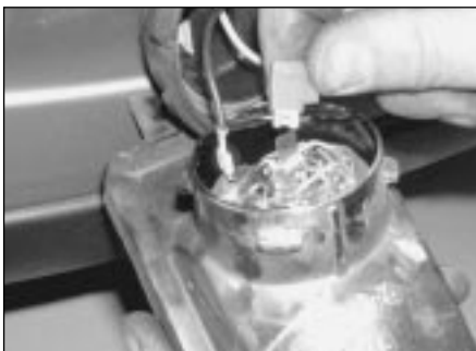
5.29a Disconnect the wiring . . .
