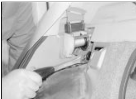
28.13 Unbolting the outer rear seat belt inertia reel from the C-pillar
