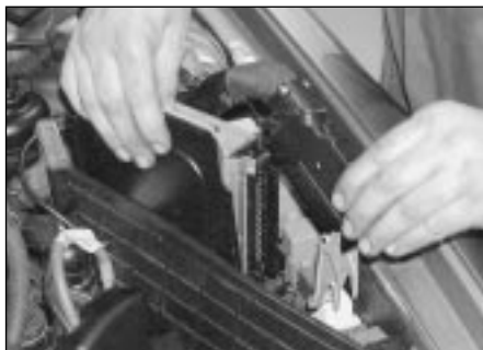
11.14 Disconnecting the wiring connector from the engine management ECU
