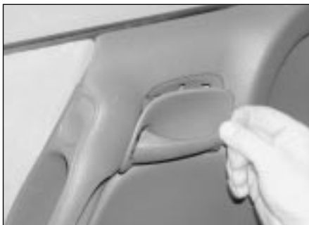
12.3 Prise the plastic cover from the inside of the interior door handle
