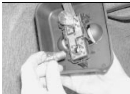
5.41 Depress and twist the relevant bulb to remove it
