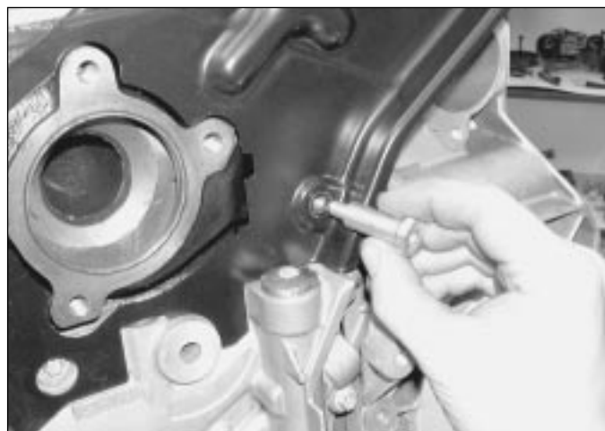
6.19 Ensure the threaded stud is correctly positioned when refitting the timing belt rear cover
