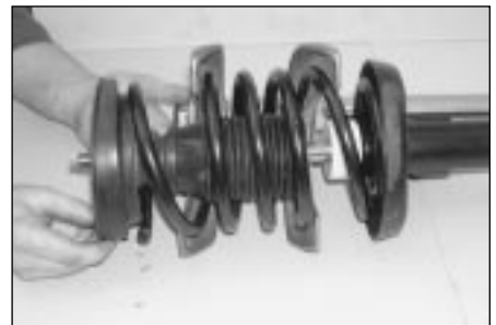
2.13c . . . then slide off the upper spring seat, upper rubber damper, bump stop rubber and dust cover
