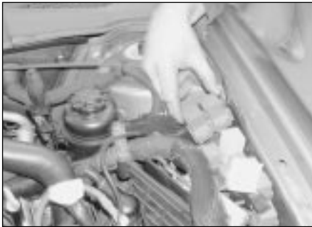
4.6a Unclip the injection system relays . . .
