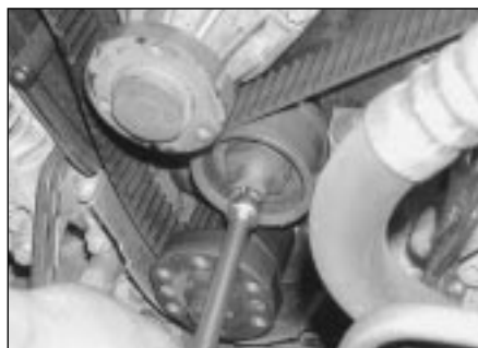
7.6b . . . and lower guide pulley in position then slide the belt off the sprockets
