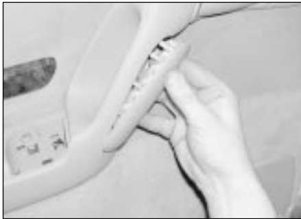
12.15 Carefully prise the grip from the underside of the door pull handle
