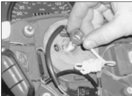
21.15c . . . and remove the steering wheel retaining nut . . .
