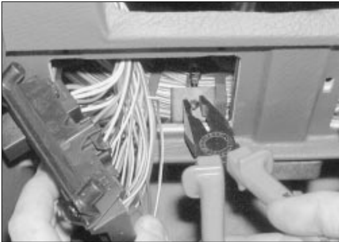
32.29a Release the main wiring harness from the mounting on the facia, behind the relay base plate, by compressing the press-stud clip with a pair of pliers . . .
