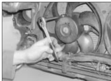
3.21a Slacken and remove the securing screws . . .
