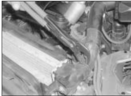
2.6a Disconnect the top hose from the radiator
