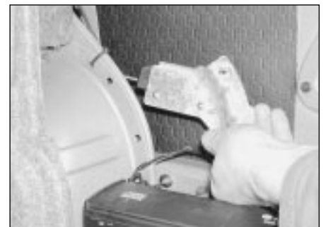
21.16b . . . and remove the servo motor and bracket from the bodywork
