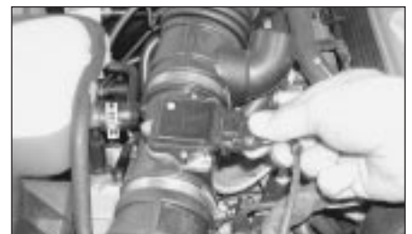
D Check that the engine management system wiring connectors are securely connected
