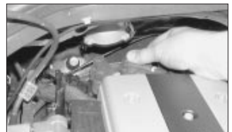
C Check that the spark plug HT leads are securely connected by pushing them onto the DIS module (where accessible)
