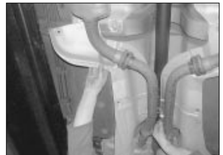
8.4 Unscrew the securing bolts and lower the exhaust system heatshields away from the underside of the vehicle
