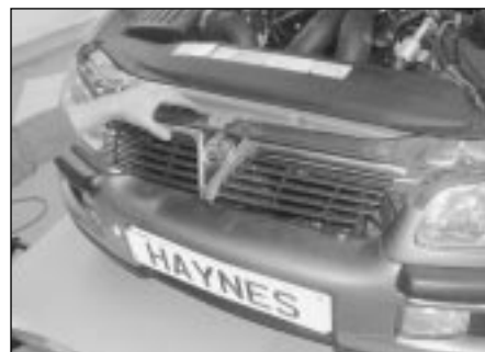
7.2b . . . then lift the radiator grille from the front bumper
