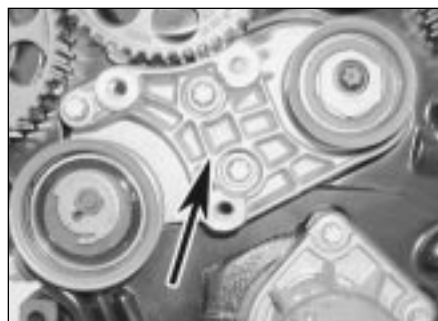
7.15 Checking the marking (location arrowed) on the tensioner/upper guide pulley backplate to identify which type of tensioner assembly is fitted to your engine - see text
