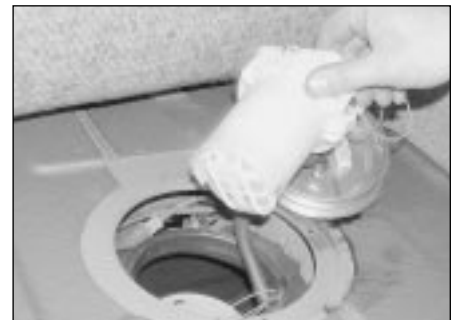
8.9b Ensure the pump filter is clean and undamaged
