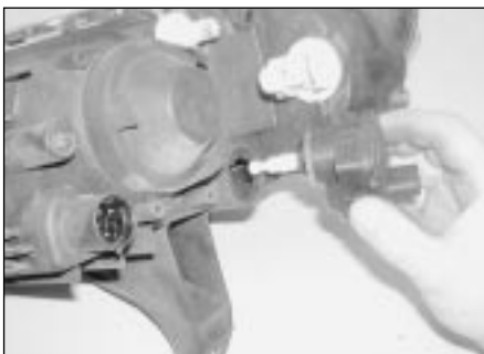
7.5 The headlight range control servo may be removed by twisting it anti-clockwise
