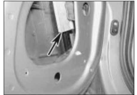
14.19b Ensure that the leading edge of the window glass engages with the guide channel (arrowed)
