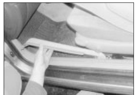
27.2c Unclip the trim panel from the side of the seat runner
