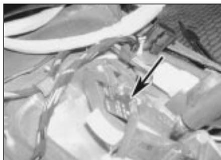
8.43 Ignition key release contact switch - later models
