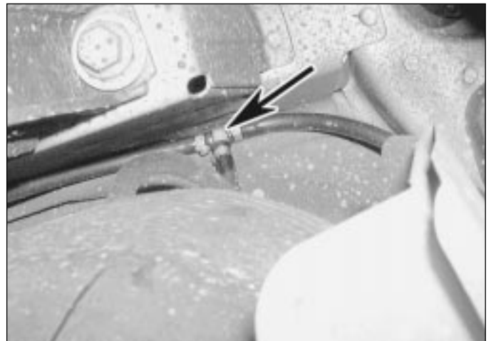
10.16 On Estate models locate the vent hose T-piece (arrowed) and disconnect the tank hoses
