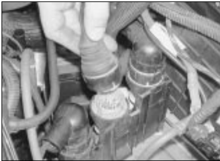
11.16a Disconnect the harness connectors located at the rear of the battery
