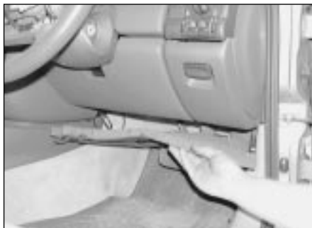
3.4a Release the retaining clips and remove the undercover panel from the driver's side of the fascia
