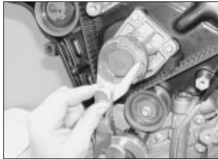
7.4b . . . and clamp its locking arm firmly around the coolant pump flange
