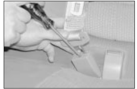
28.9c . . . and then depress the locking button to release the lower belt anchor from its buckle
