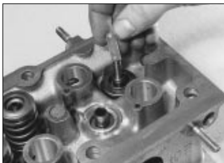
8.2b ... then fit the seal protector (where provided) ...
