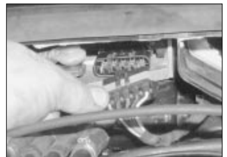
16.6 Disconnect the wiring at the wiper motor
