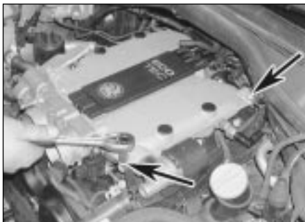
15.38 Undo the retaining bolts and free the hose/wiring brackets from the manifold
