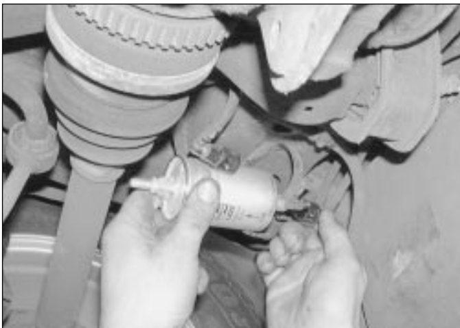
23.6 Depress the quick-release fitting tabs and detach the hoses from the fuel filter
