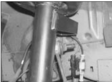
7.2b . . . and detach the drop link from the suspension strut
