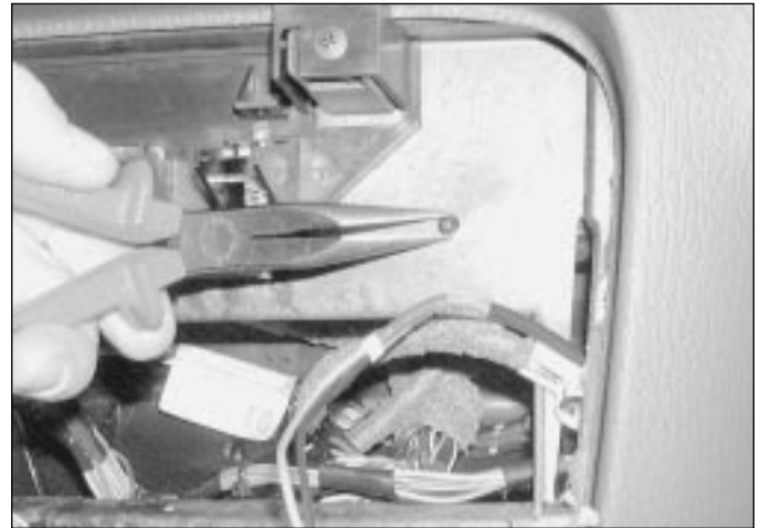
32.29b . . . release the three clips from the panel behind the heater/ECC control panel mounting aperture in a similar manner
