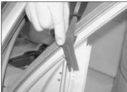
14.16 Remove the rubber seal from the window guide channel
