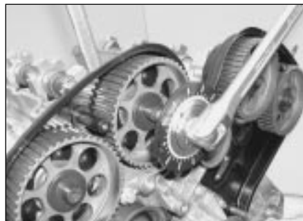
8.9b . . . and then through the specified stage 2 and 3 angles
