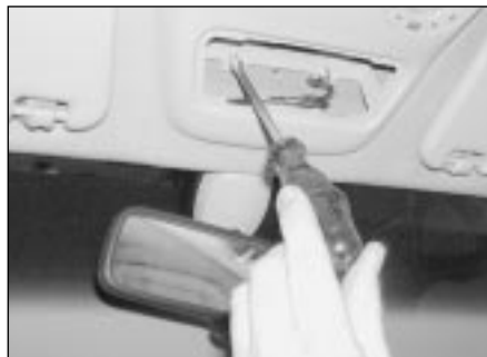
25.20a Undo the securing screws located inside the interior lamp recess . . .
