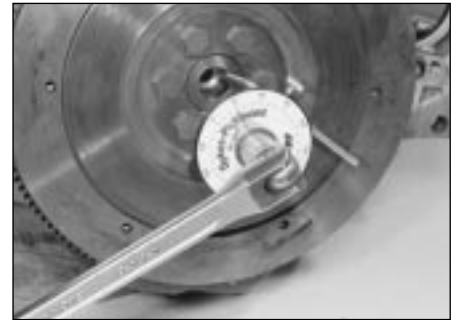
15.12b . . . then tighten them through the specified stage 2 and 3 angles
