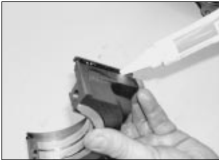
17.31a Fill the side grooves of the rear (number 4) bearing cap with sealant . . .
