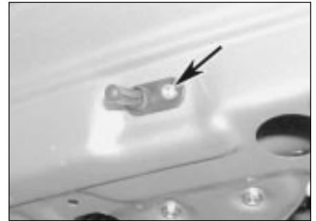
4.27 Undo the retaining screw (arrowed) and withdraw the switch - Estate model shown
