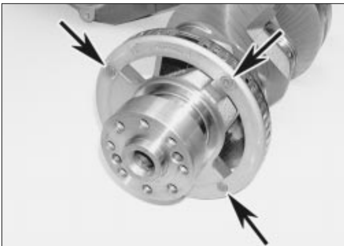
17.15 Crankshaft sensor rotor is secured to the crankshaft by four bolts (three arrowed)
