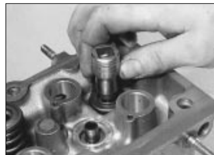
8.2d Press the oil seal fully onto the guide with a suitable socket
