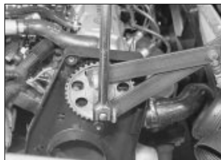
8.2 Using a home-made sprocket holding tool to retain the camshaft sprocket whilst the bolt is slackened
