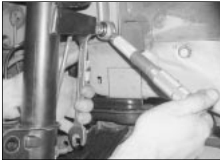
7.4 Tighten the anti-roll bar drop link securing nuts to the specified torque
