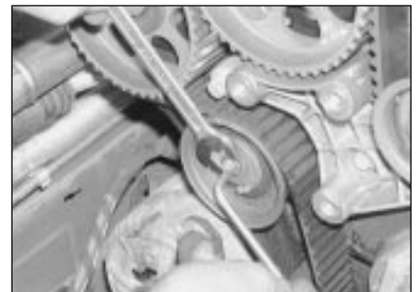
7.5b . . . then rotate the pulley clockwise, positioning it just before its stop, and secure it by retightening the nut
