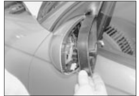
23.21b . . . and lift off the mirror housing frame
