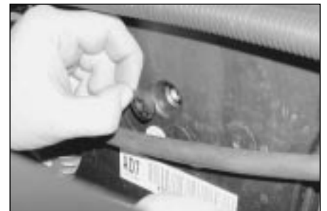
6.5 . . . and ensure the outer spacers are correctly positioned before refitting the retaining bolts
