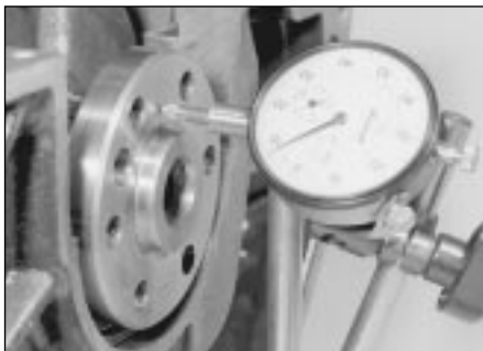
13.2 Checking crankshaft endfloat with a dial gauge
