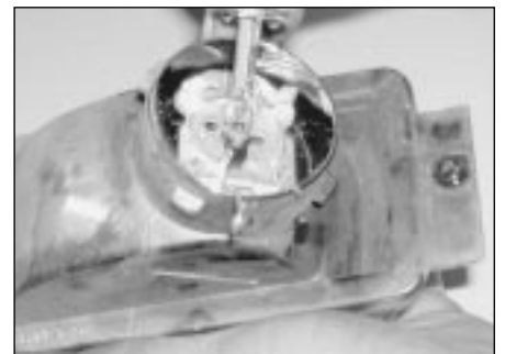
5.29c . . . and remove the bulb from the foglight
