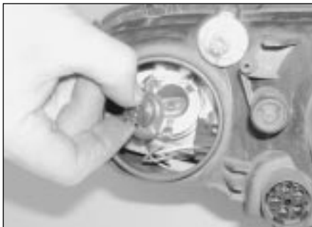
5.16 Press the bulb squarely into its housing until it is felt to engage with its retaining clips
