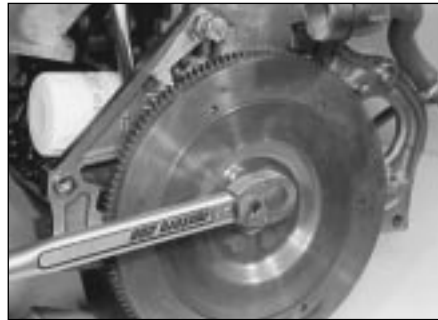
15.12a On manual transmission models, tighten the flywheel bolts to the specified stage 1 torque setting . . .
