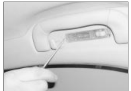
6.5 Carefully prise the rear interior light from the door upper trim panel
