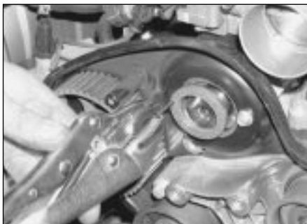
9.2b . . . then screw in a self-tapping screw and pull out the oil seal with pliers/grips
