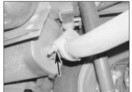
18.12 Tailpipe-to-intermediate pipe clamp - 2.0 litre DOHC engine
