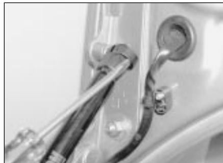
17.7 Using a small screwdriver, prise the spring clip from the top of the strut
