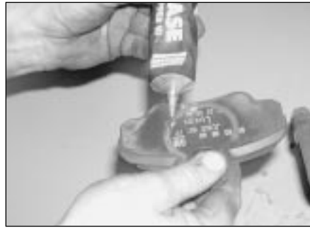
2.19a Apply a little high-melting-point copper brake grease to the brake pad backing plates . . .
