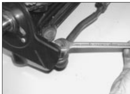
25.2a Unscrew the securing nut . . .
