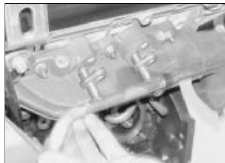
6.42 Removing the left-hand connecting pipe from the manifold (shown with engine removed)
