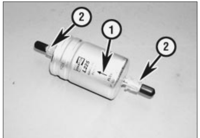
23.8 On refitting ensure the arrow (1) on the filter is pointing in the direction of fuel flow and the quick-release fitting clips (2) are correctly fitted
