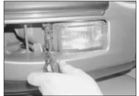
5.27 Undo the securing screws and pivot the fog light lens forwards
