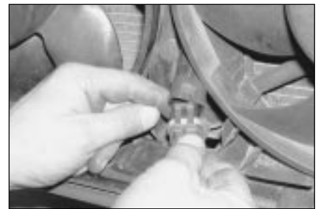
3.19b . . . then unplug the wiring harness from the auxiliary fan at the multi-way connector
