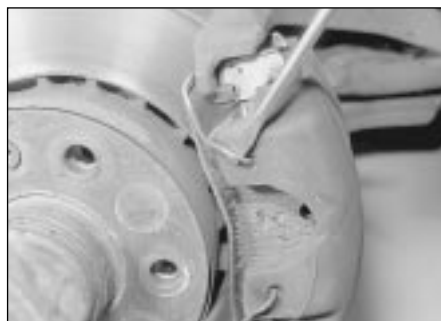
2.7 Remove the large spring clip from the side of the brake caliper
