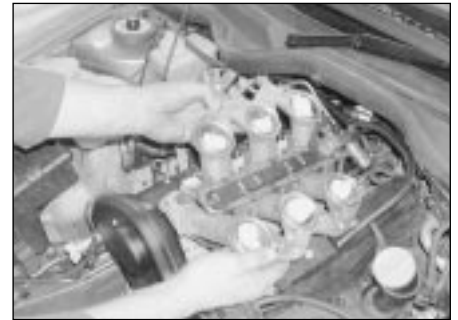
15.42a Remove the manifold lower section . . .
