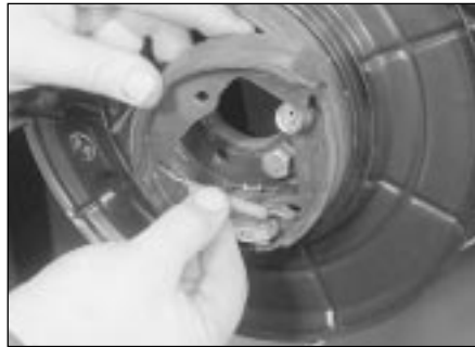
7.18a Refit the rear (leading) shoe and the lower return spring
