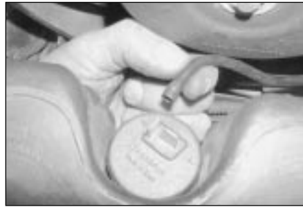
18.6 Disconnect the hose from the pump and allow the fluid to drain into the container
