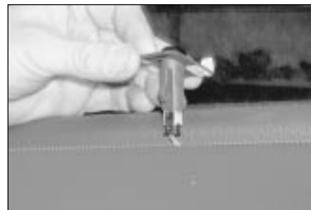
13.56 Carefully lever the sun sensor from the upper surface of the facia
