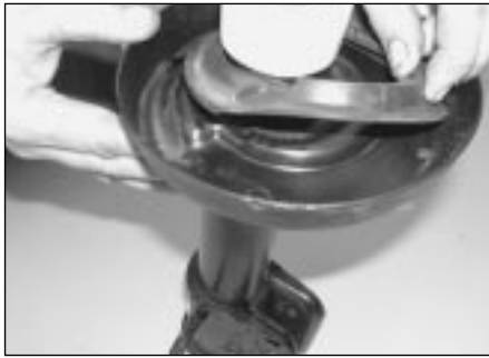
2.20a Refit the rubber damper to the lower spring seat
