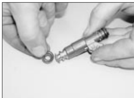
14.5 On refitting be sure to renew all injector sealing rings
