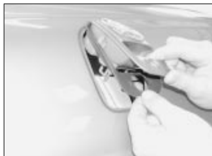
18.3c Remove the exterior handle and gasket from the outside of the bootlid
