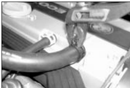
4.1 Release the retaining clips and disconnect the breather hoses from the camshaft cover
