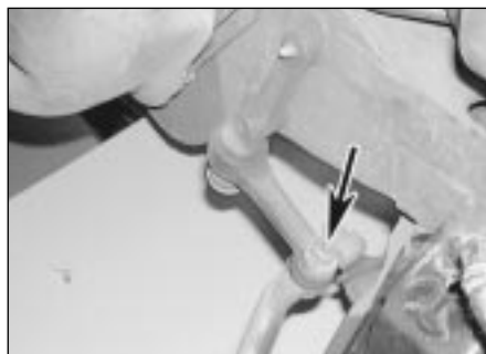
25.5b Centre tie-rod-to-idler balljoint nut (arrowed)
