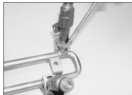
14.4c Slide off the relevant retaining clip . . .
