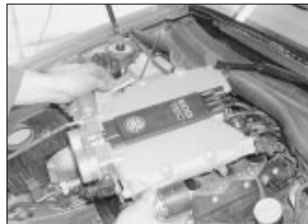
15.39b . . . and remove the manifold upper section
