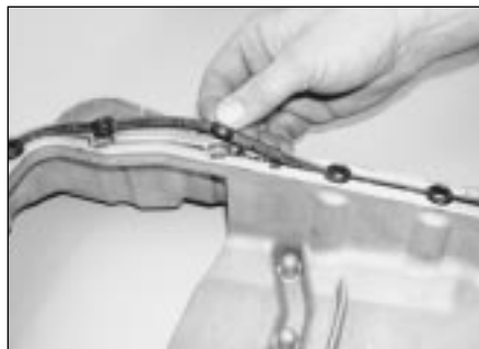
12.24a . . . then locate the new seal in the casting groove
