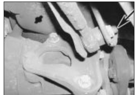
15.3 Track control arm-to-subframe bolt
