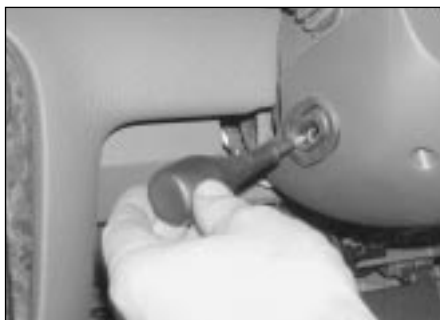
4.4a Unscrew the lever from the steering column tilt mechanism . . .
