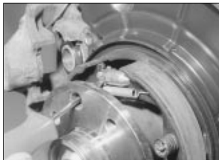
7.23 Using a screwdriver through the hole in the drive flange to turn the serrated nut on the adjuster
