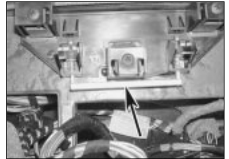
13.5b . . . and pull down on the aluminium locking bar at the rear of the upper edge of the control panel (shown with panel removed for clarity)
