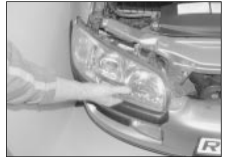
7.4c . . . and withdraw the headlight from the front of the vehicle
