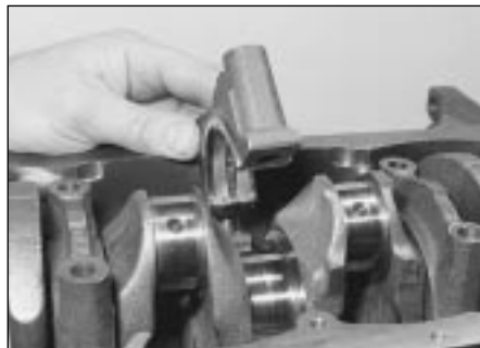
17.19 Refit the bearing caps number 1 to 4 ensuring each one is refitted in its original location
