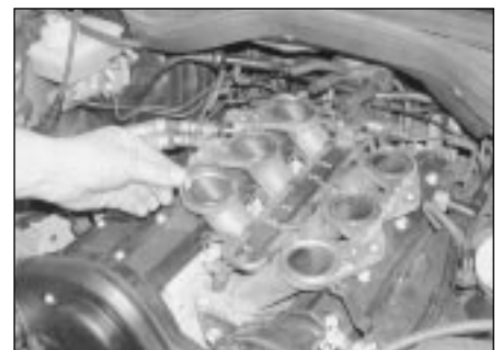
15.44 On refitting be sure to renew all manifold seals and sealing rings
