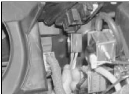
10.9 Unplug the wiring harness from the blower motor series resistor at the connector
