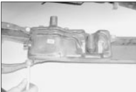
18.10 Unscrew the mounting bolts and withdraw the reservoir from the rear of the bumper inner section
