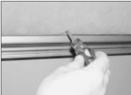
12.8b . . . then remove the screws from the lower and front edges of the trim panel
