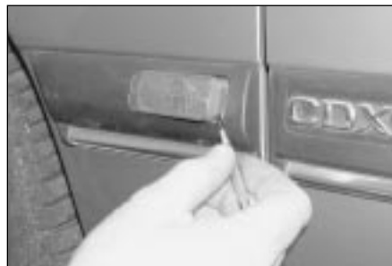
5.31 Carefully lever the side repeater light from the front wing moulding
