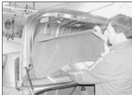
18.1b . . . and remove the trim panel from the inside of the bootlid
