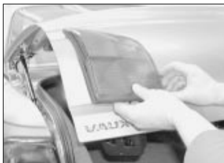
7.14b . . . and detach the light cluster from the bootlid
