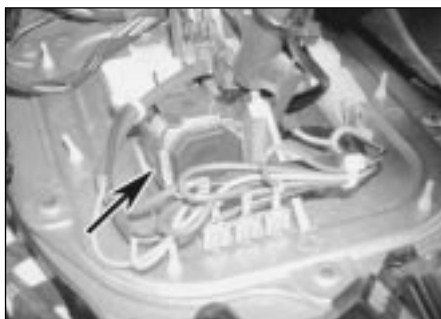
8.37 Selector lever pawl starter solenoid - later models
