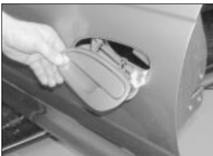
13.9c . . . and withdraw the handle from the door through handle aperture
