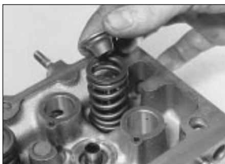
8.3 Fit the valve spring and spring retainer
