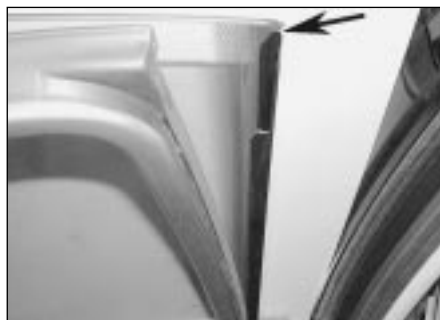
14.26b . . . and that the channel (arrowed) at the leading edge of the glass engages with the front edge of the door
