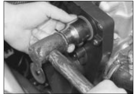
9.4 Fitting a new camshaft oil seal
