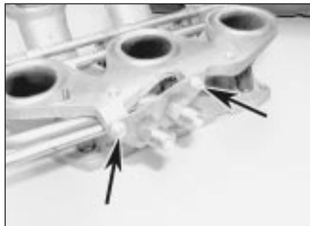
14.3b . . . then undo the retaining bolts (arrowed) . . .
