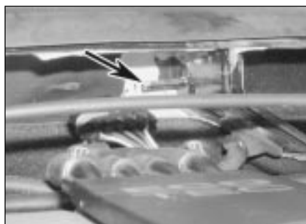
16.10 The grometed lug at the left hand end of the wiper assembly must engage with the corresponding peg (arrowed) on the bulkhead bracket
