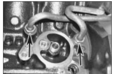
11.27a Unscrew the union nuts (arrowed) securing the oil pipes to the cylinder block . . .
