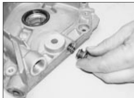
13.11c Slacken and remove the safety valve bolt and sealing washer . . .
