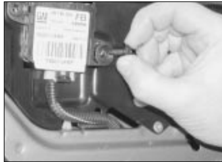
24.43a Unscrew the securing screws and remove the sensor from its mounting bracket
