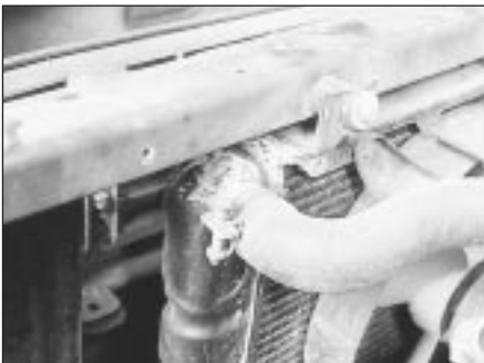
Leaking antifreeze often leaves a crystalline deposit like this.
