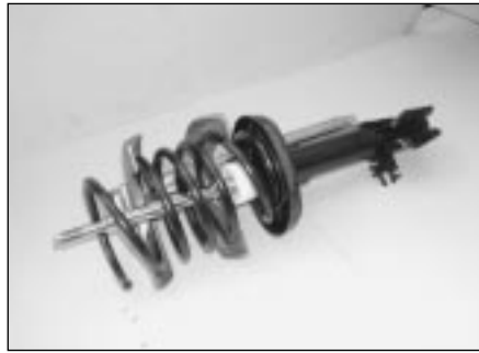
2.20b Lower the coil spring, together with the spring compressors, onto the lower spring seat
