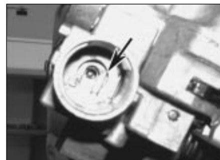
23.6 If necessary, press the locking button latch (arrowed) downwards, until the steering lock bolt disengages
