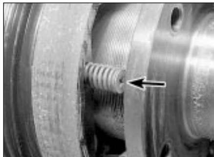
7.6 Handbrake shoe anti-rattle spring (arrowed) - early model
