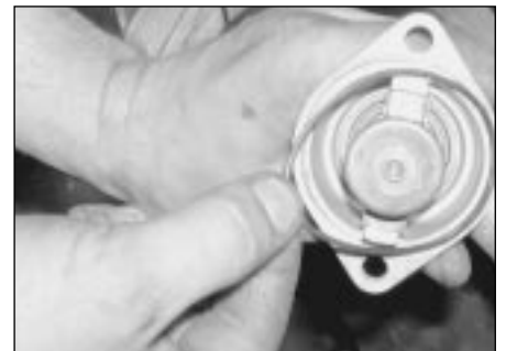
4.12 Fit a new sealing ring to the thermostat cover
