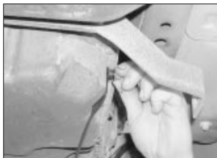
2.4 . . . and allow the transmission fluid to drain into a suitable container
