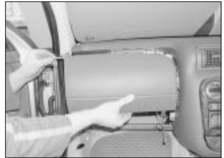
24.19 Remove the hinged cover to expose the airbag unit
