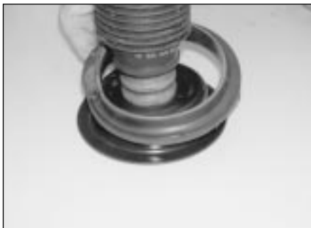
2.21 Locate the rubber damper in the upper spring seat
