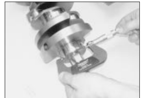
13.10 Using a micrometer to measure a main bearing journal
