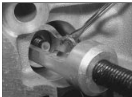
8.4 Compress the valve and locate the collets in the recess on the valve stem
