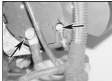
7.10 Slacken the retaining nuts (arrowed) and disconnect the wiring from the rear of the alternator (shown with engine removed)
