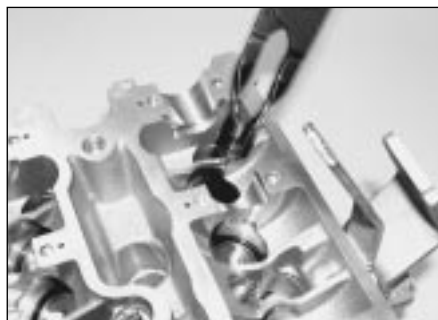
6.4b Pull off the valve stem seals using a pair of pliers
