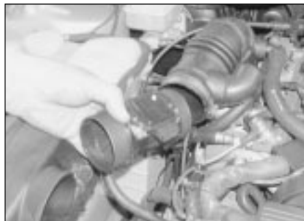
13.41 Removing the airflow meter
