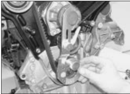
7.4a If the service tools are available, firmly attach the crankshaft locking tool to the sprocket . . .
