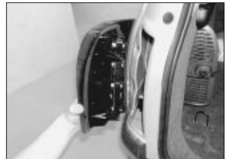
7.18d . . . and withdraw the light cluster from the rear of the vehicle (estate models)
