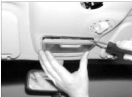
6.2 Carefully prise the lens from the front interior light using a screwdriver
