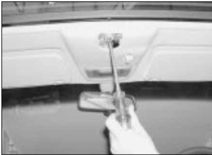
25.31 In an emergency, the sunroof glass can be operated by removing the cover panel and turning the manual drive shaft with a screwdriver
