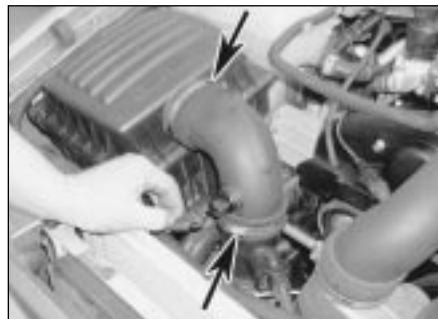
14.20 Disconnect the wiring connector from the intake air sensor then release the retaining clips (arrowed) and remove the intake duct
