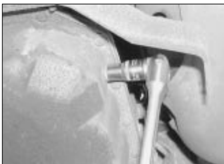
2.3 Slacken and remove the fluid level plug from the main sump . . .
