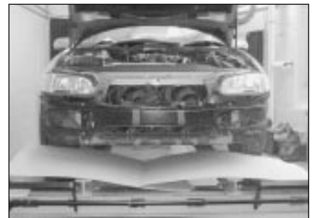
6.5b ... and then withdraw the bumper centre member from the front of the vehicle
