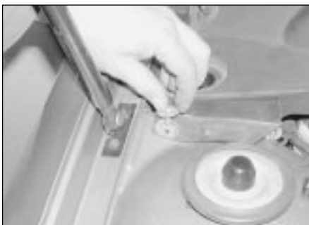
16.3 Slacken and withdraw the screws securing the ends of the water deflector panel to the bodywork
