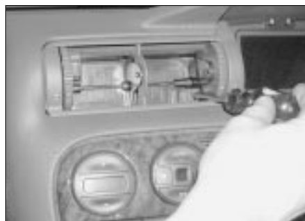
32.22b . . . then undo the securing screws . . .
