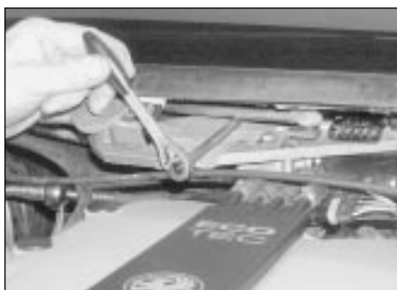
16.7c . . . and centre of the wiper motor assembly to the scuttle. Note that the centre securing bolt can only be accessed using an extension bar
