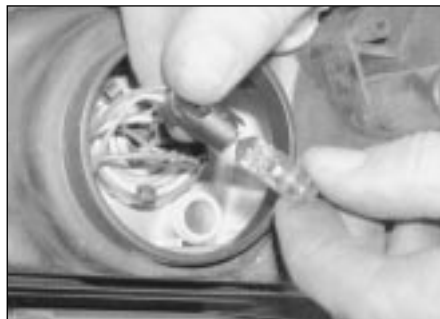
5.20 Remove the bulb from the holder
