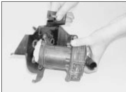
6.8b . . . and separate the pump from its mounting bracket
