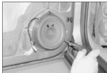
20.9 Undo the mounting screws and withdraw the loudspeaker from the door inner panel
