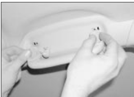
32.32a Unbolt and remove the driver and passenger grab handles . . .
