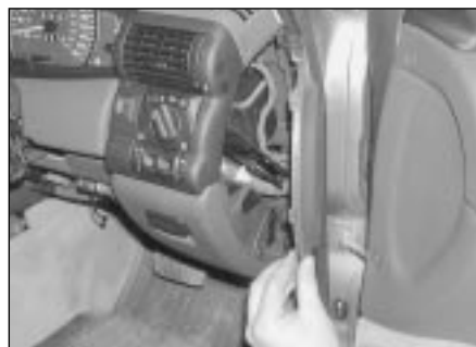
32.10 Lever the cover panel from the side of the right hand fascia end section
