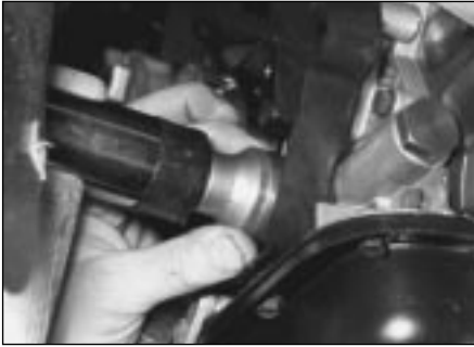
16.4 Fitting a new crankshaft front oil seal
