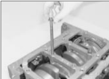
17.33 Lubricate the threads of the new main bearing cap bolts . . .
