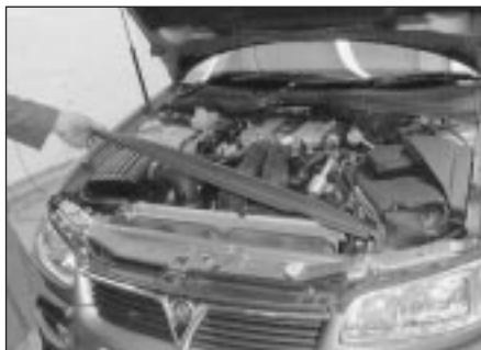
2.2 Lift out the radiator upper cover panel
