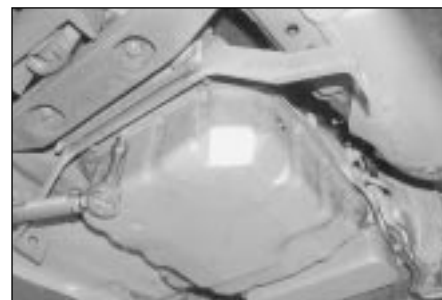
2.5 Unscrew the retaining bolts and remove the main sump from the transmission unit
