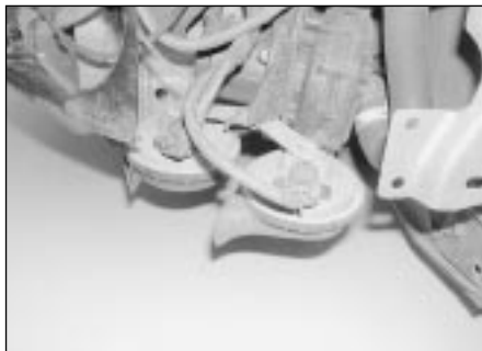
14.1 The horns are located behind the front bumper on the left-hand side of the vehicle
