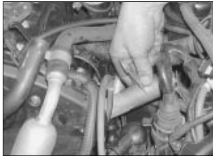
4.9a Carefully pull the coolant transfer pipe from the thermostat housing . . .
