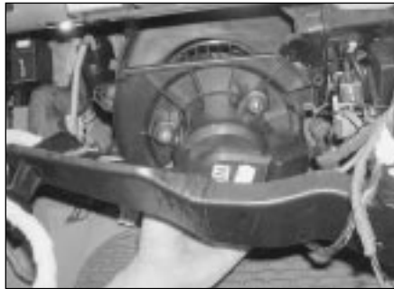
10.6b . . . then withdraw the blower motor and fan assembly from its housing
