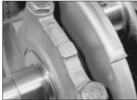
10.5 The main bearing caps should be numbered (No 1 cap shown)
