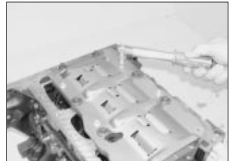
18.18 On 2.5 and 3.0 litre engines, refit the baffle plate and tighten its retaining bolts to the specified torque
