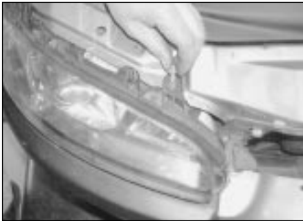
7.4a Unscrew the headlight mounting bolts located above . . .
