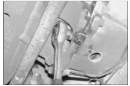
9.21b . . . then slacken and remove the torque converter to driveplate bolts as described in text
