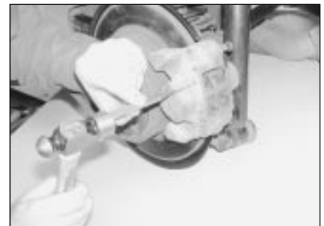
3.4 Driving out the upper rear brake pad pins using a thin punch
