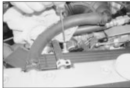
7.3 Place a wad of rag around the valve and depress the valve with a screwdriver to relieve the pressure in the fuel system
