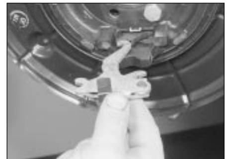
7.14c Refitting the lever assembly to the backplate
