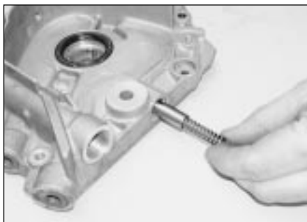
13.11d . . . and withdraw the spring and plunger from the pump
