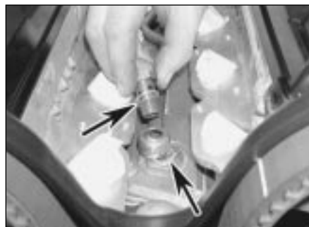
14.8b . . . then remove the union bolts and sealing washers (arrowed) and free the pipes from the oil cooler
