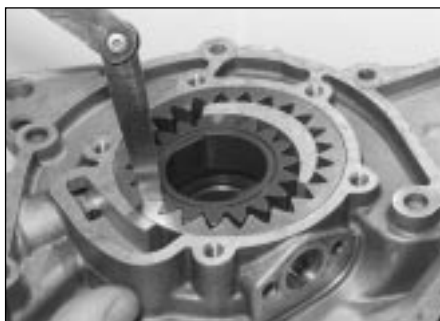
14.13a Using a feeler blade to check gear clearance
