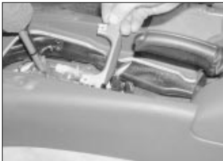
30.10b . . . remove the support bracket . . .
