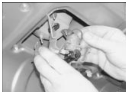
18.3b . . . then withdraw the lock from inside the bootlid
