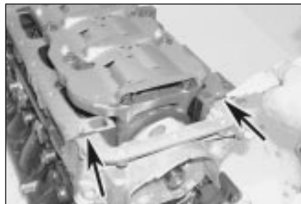
12.25a Apply a smear of sealant to the joints between the oil pump housing and cylinder block . . .
