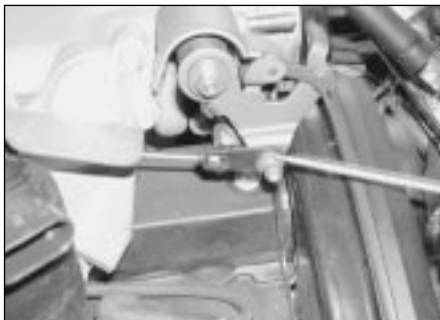
15.32b On models with cruise control praise off the second retaining clip . . .
