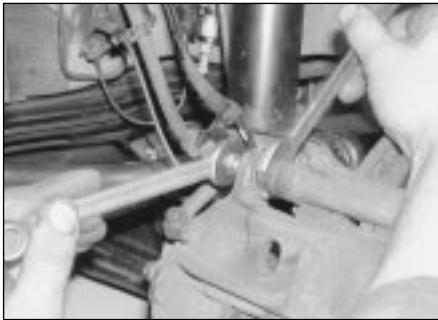
4.3a Slacken the upper guide pin bolt, counterholding the guide pin with a second spanner . . .
