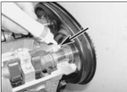
10.13 Apply sealant to the cylinder head surface on each side of the camshaft oil seal apertures (arrowed)
