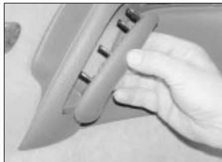
12.4 Carefully prise the grip from the underside of the door pull handle
