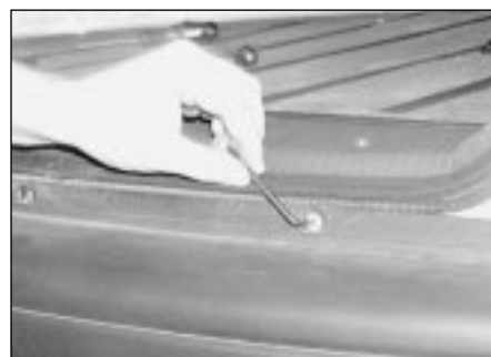
6.18b . . . then unscrew the screws securing the upper edge of the bumper moulding to the bodywork
