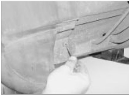
4.2a Unscrew the retaining nuts then press out the centre pins . . .
