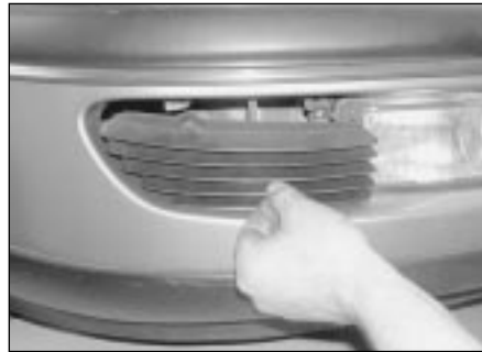
5.26 Remove the screws and detach the grille adjacent to the relevant fog light
