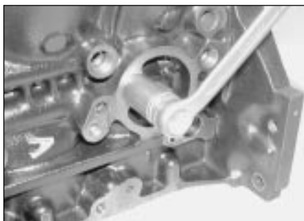
11.3b . . . then use an M10 bolt and washer and a suitable socket . . .
