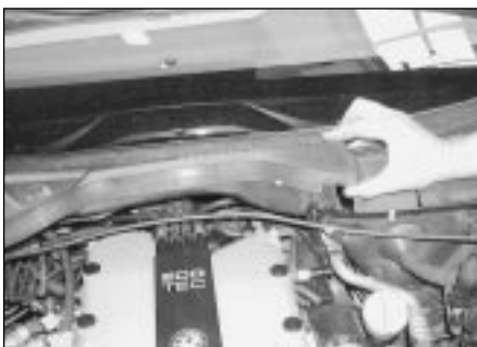
16.4c Unclip and remove the water deflector panel
