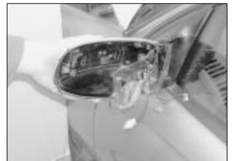
23.22b . . . and detach the cover from the front of the mirror housing
