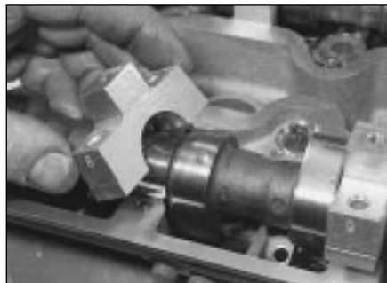
10.3 Removing a camshaft bearing cap
