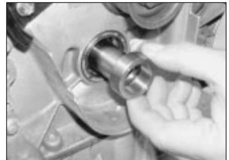
8.14c . . . and, if necessary, withdraw the spacer from the oil seal
