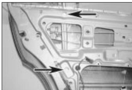
14.24b . . . centre and lower securing bolts (arrowed), then withdraw the guide channel from the door
