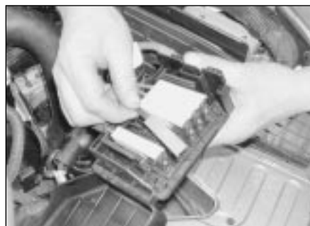
4.8b . . . and unclip the engine harness connector from the fusible link housing
