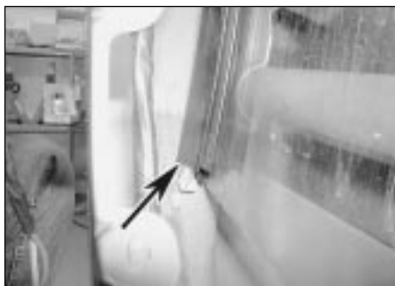
14.26a Ensure that the trailing edge of the window glass engages with the guide channel (arrowed) . . .
