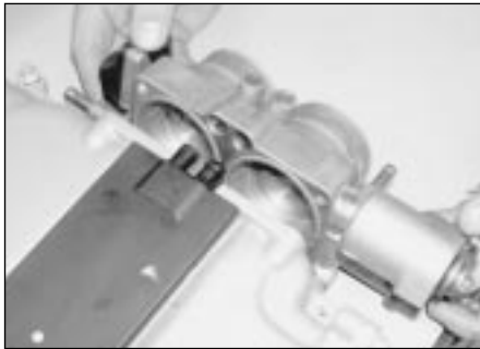
11.20 Removing the throttle housing - 2.5 and 3.0 litre engines
