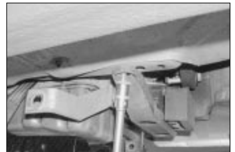
9.13 . . . then slacken and remove the bolts securing the transmission unit crossmember to the body
