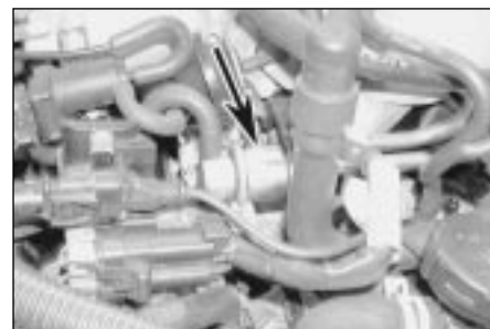
14.7 The fuel pressure regulator is located at the rear of the inlet manifold (shown with engine removed)
