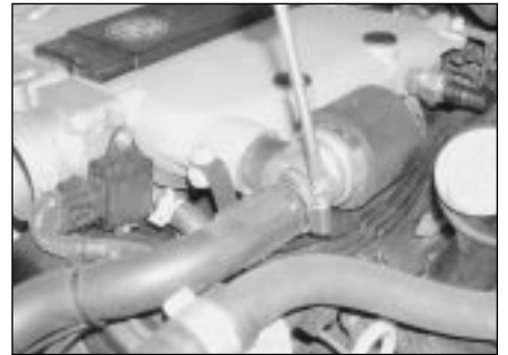
15.30 Slacken the retaining clip and detach the air hose from the idle speed adjuster valve
