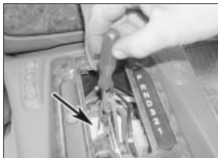
1.0b . . . then depress the yellow release lever (arrowed) on the selector lever mounting
