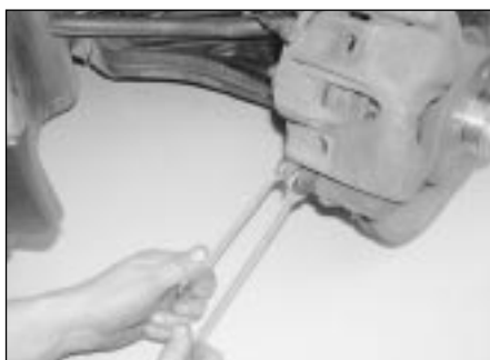
2.12a Slacken the lower guide pin bolt, counterholding the guide pin with a second spanner . . .
