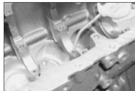
11.5 Use compressed air to blow out all the cylinder block internal drillings and oilways
