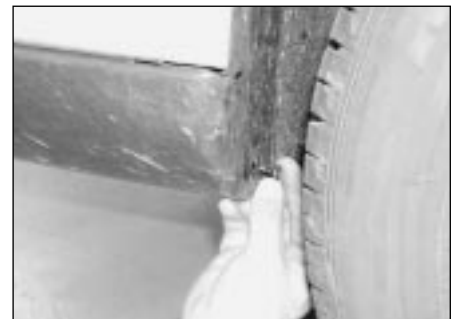
6.14 Remove the securing screws and detach the lower edges of the plastic liners from both rear wheel arches
