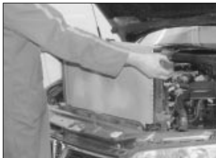
2.10b ... then withdraw radiator complete with the cooling fan from engine compartment
