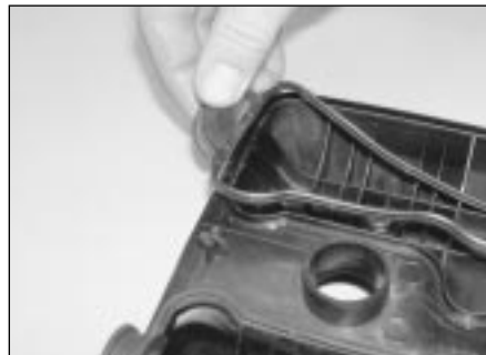
4.9a Fit the new seals securely to the cover grooves . . .
