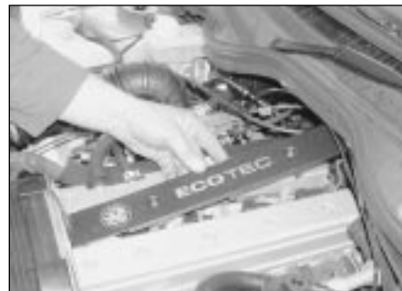
4.2a Remove the spark plug cover . . .
