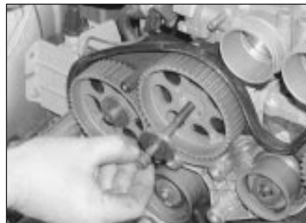
8.3a Unscrew the retaining bolt and washer . . .
