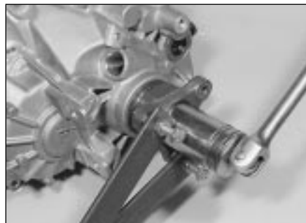
5.2 Slacken and remove the retaining nut whilst retaining the propeller shaft flange with a home-made tool . . .
