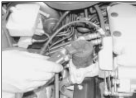
5.7 On 2.5 and 3.0 litre engines, disconnect the wiring connector . . .
