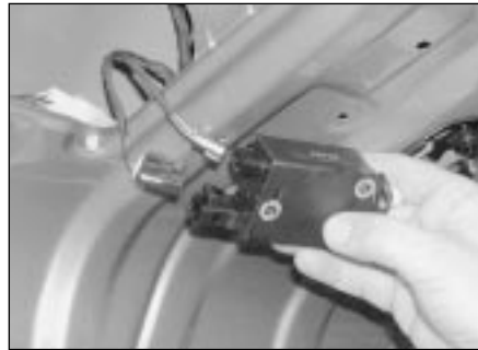
21.8b and remove the servo motor from the bootlid
