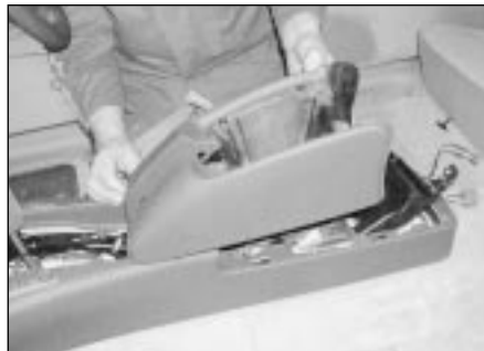
30.9b . . . and lift off the centre arm rest (where fitted)
