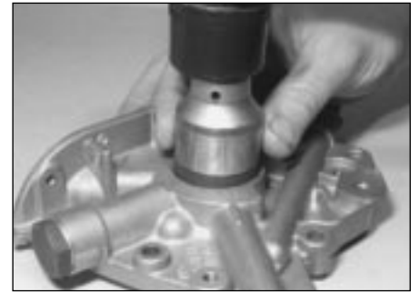
13.14 Fitting a new crankshaft oil seal to the oil pump housing
