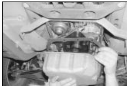
2.11 Ensure the mating surfaces are clean and dry then refit the main sump complete with a new gasket
