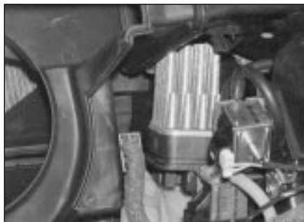
10.10 Withdraw the resistor from the fan/motor housing
