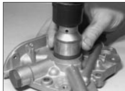
14.15 Fitting a new crankshaft oil seal to the oil pump housing
