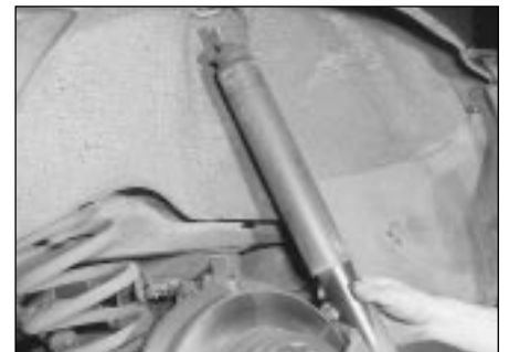
11.7b . . . then remove the shock absorber from the wheel arch
