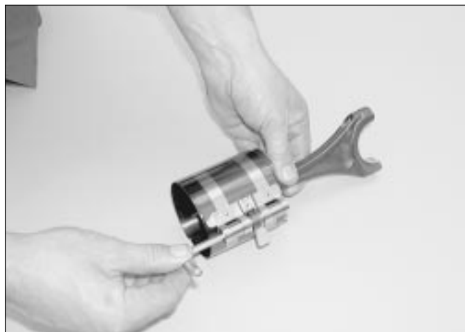
18.8 Ensure the piston ring end gaps are correctly positioned then clamp them in position with a ring compressor
