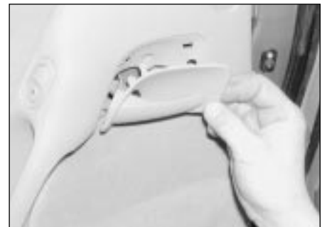
12.14 Unclip the trim panel from behind the door lock release handle
