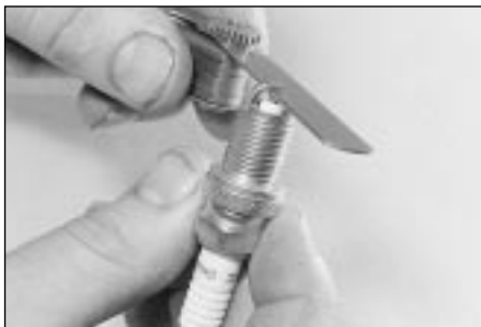
22.12a If single electrode plugs are being fitted, check the electrode gap using a feeler gauge . . .
