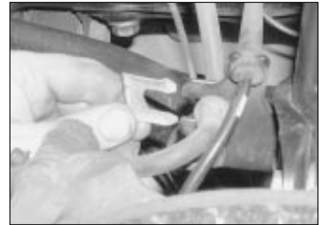
2.6 Slide out the metal retaining clip and release the brake hose from the suspension strut
