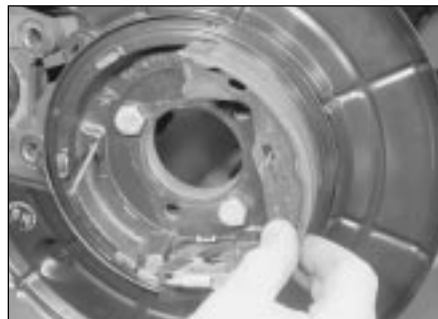
7.17a Locate the front (trailing) shoe on the backplate . . .
