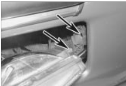
5.30 When refitting the light ensure that the lug (arrowed) at the inner edge engages correctly with the recess in the front bumper valence
