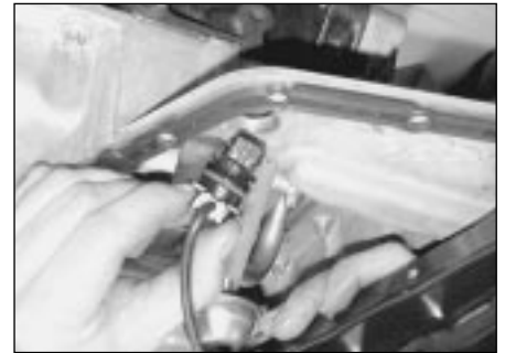
12.18 On refitting, locate the oil level sensor wiring connector in the main casting before bolting the sump pan in position
