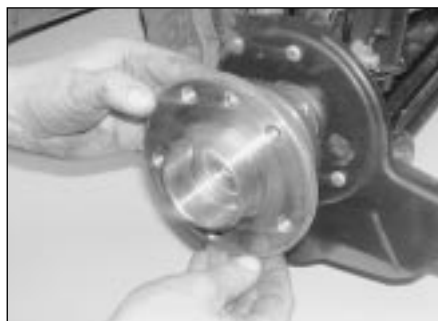
9.6c . . . and pull the hub from the stub axle
