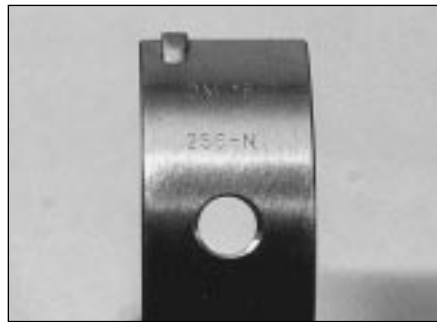
14.1 Typical main bearing shell identification marking
