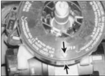
24.29 Airbag contact unit alignment markings (arrowed) - refer to text
