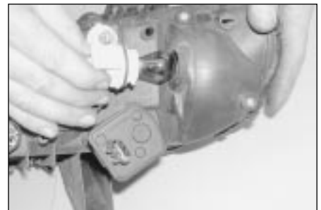
5.23 Rotate the indicator bulbholder anticlockwise to release it from the rear of the light unit
