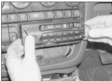
19.3 Using the DIN removal tools carefully withdraw the radio/cassette/CD player from the fascia
