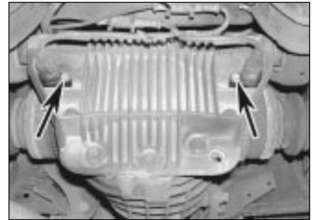
18.51 ABS rear wheel speed sensors (arrowed)
