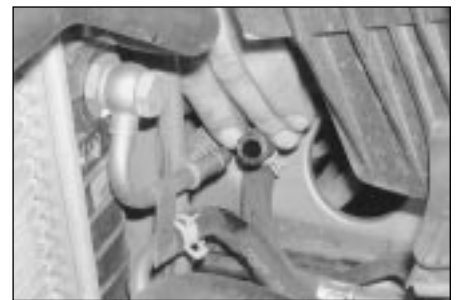
2.9 Disconnect the narrow bore transmission fluid cooler hoses from the radiator
