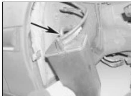
4.3b . . . then free the charcoal canister from its mounting and disconnect it from its hoses
