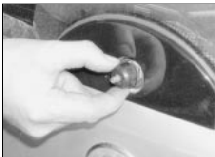
17.2 Remove the plastic cap and unscrew the wiper spindle nut
