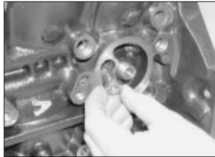
11.16a On 2.5 and 3.0 litre engines, insert the new bypass valve into the cylinder block . . .
