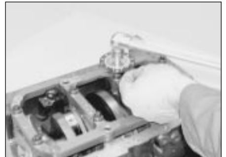
17.35 . . . and then through the specified stage 2 and 3 angles
