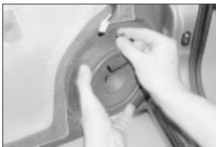
20.2 Undo the mounting screws and withdraw the loudspeaker from the door inner panel
