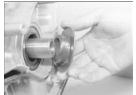
8.12 Remove the flanged spacer if necessary
