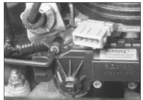
11.16 Unscrewing an idle speed control motor securing screw
