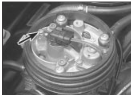
12.5 Fuel injector retaining plate securing screw (arrowed)
