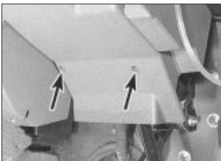
14.2 Steering column lower trim panel screws (arrowed)
