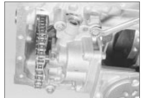
13.2 The oil pump is retained by three bolts
