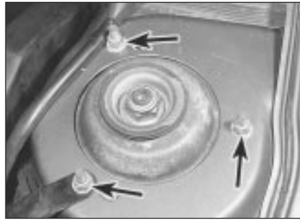
4.2 Front suspension top mounting nuts
