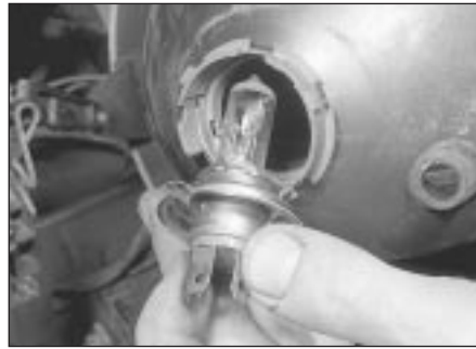
8.7b ... and withdraw the headlight bulb
