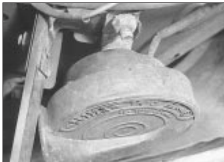
20.3 Horn and mounting nut
