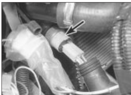
5.4a Disconnect the thermo-switch (arrowed) . . .
