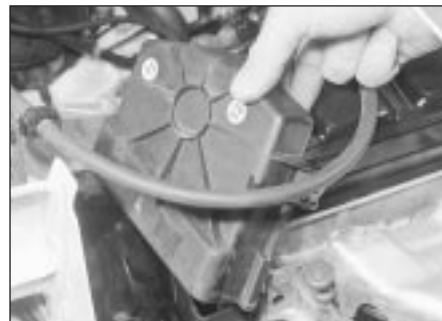
6.1b . . . and remove the timing belt upper cover
