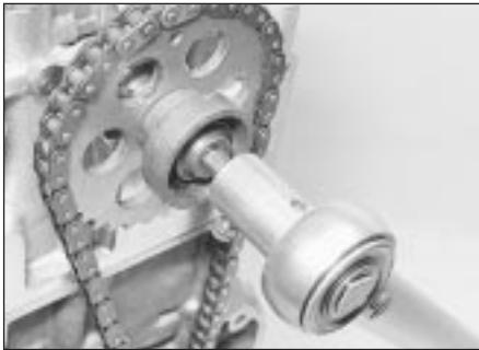
4.23 Tightening the camshaft sprocket retaining bolt
