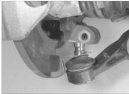
2.4b . . . and pull the suspension arm down from the hub carrier
