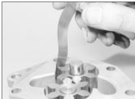
5.6 Checking oil pump gear to body clearance
