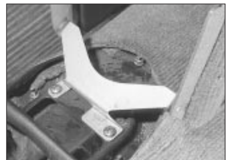
26.12 Facia central lower panels and bracket
