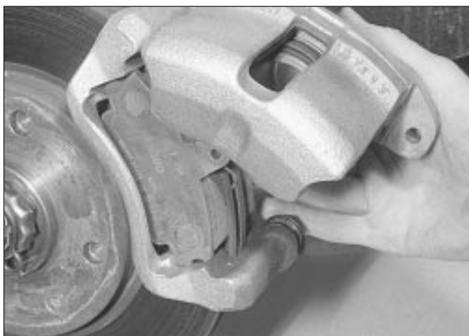
4.20a Swivel the caliper upwards . . .
