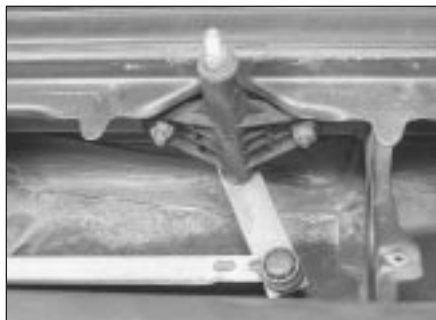
15.4 Wiper spindle body
