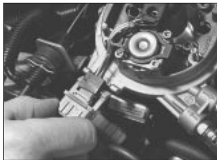
11.12a Separate the two halves of fuel injector wiring connector . . .
