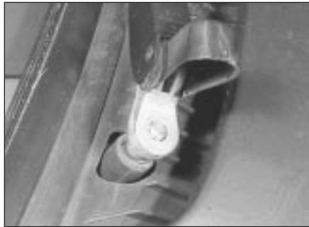
14.2b . . . and remove the wiper arm
