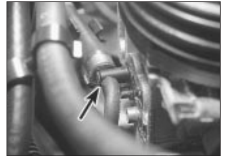
11.25 Vacuum hose connection to throttle body (arrowed)
