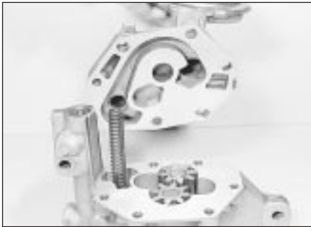
10.5a Lift off the pump strainer cover . . .
