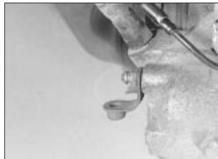
2.14 Bleed screw and dust cap on front brake caliper
