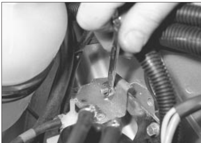
8.7a Unscrew the securing nut . . .
