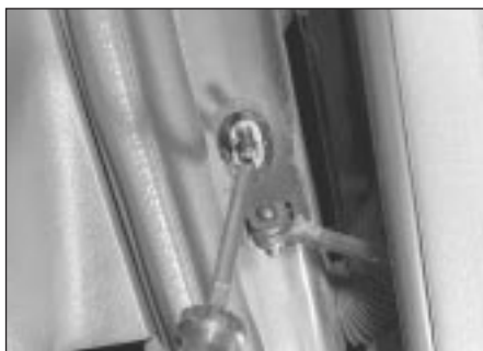
4.21 Removing a courtesy light switch
