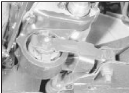
8.3 Engine lower mounting
