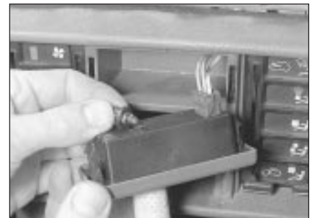
9.11 Removing digital clock illumination light bulb
