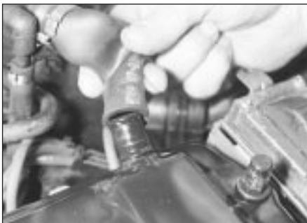
4.3 Disconnect the breather hose from the cylinder head cover . . .
