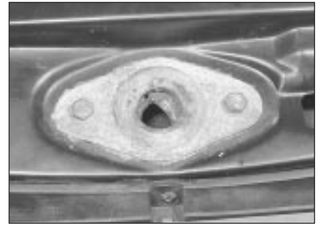
7.2 Bonnet lock retaining bolts
