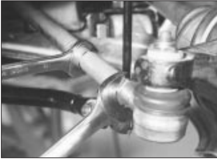
21.11 Adjusting the front wheel toe setting
