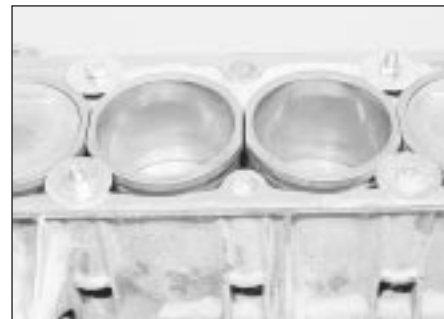
8.17 Cylinder liners clamped with washers and bolts
