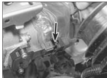
4.15 Disconnect the distributor wiring connector on TU series engines
