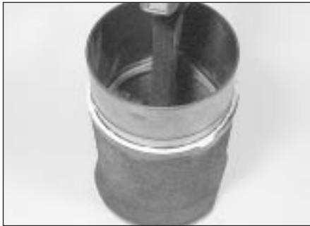
9.11 Cylinder liner with paper base seal
