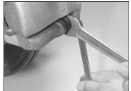
4.19 Unscrewing the lower caliper guide pin bolt (1.9 GTI)
