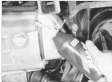
21.4 Topping-up the transmission oil level
