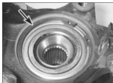
3.3 Front hub bearing retaining circlip (arrowed)
