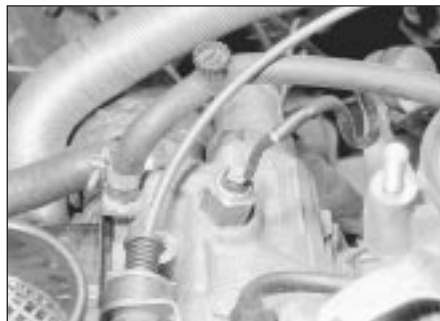
7.5 Coolant temperature sensor location on XV, XW and XY series engines
