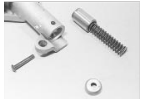
5.8 Oil pump pressure relief valve components
