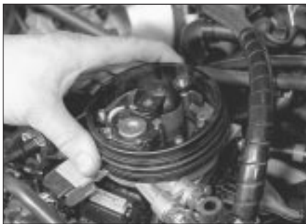
11.11a Remove the sealing ring . . .
