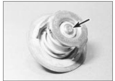
4.9 Thermostat temperature rating (arrowed) stamped on base
