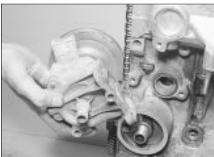
8.3b . . . withdraw the pump from the cylinder block . . .
