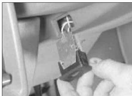
4.16 Instrument illumination rheostat
