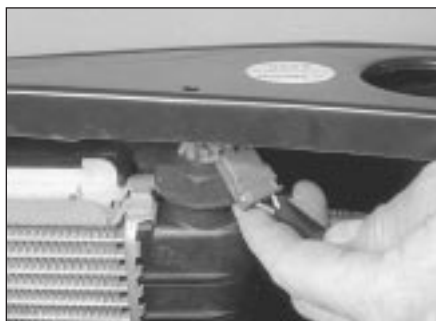
5.4b . . . and low coolant level sensor wiring
