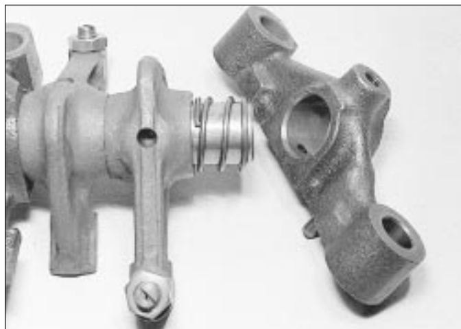
6.4b . . . and slide the components off the shaft
