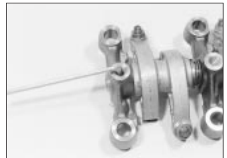
10.5b . . . then remove the grub screw
