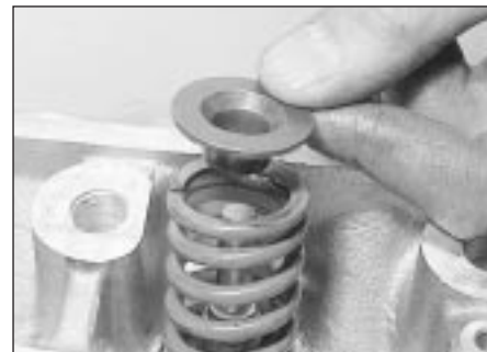
6.4b . . . Release the compressor and remove the spring retainer . . .
