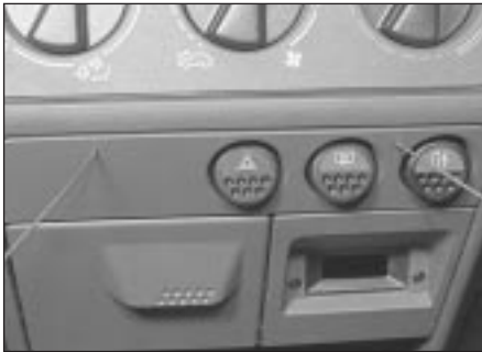
26.27a Method of releasing the switch surround upper clips
