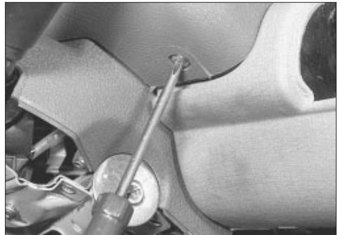
5.4 ... and lower retaining screws
