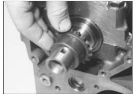
8.12a Slide off the oil pump drive sprocket . . .
