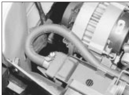
5.3 Expansion tank vent hose connection on the radiator
