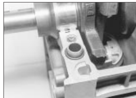
13.41 Crankcase flange O-ring seal
