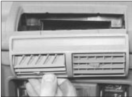
26.4 Removing the central air vents
