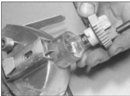
8.10 Remove the front direction indicator light bulbholder ...
