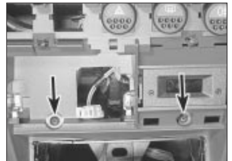
26.36 Front fascia panel screws (arrowed)
