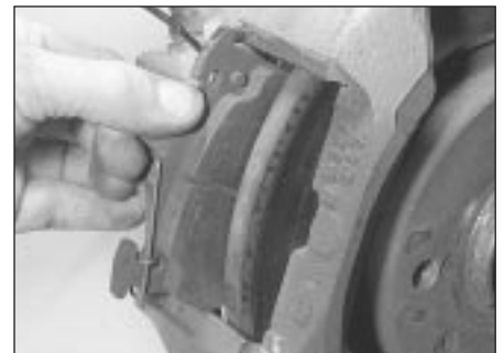
4.6 Removing the inner pad (DBA Bendix caliper)
