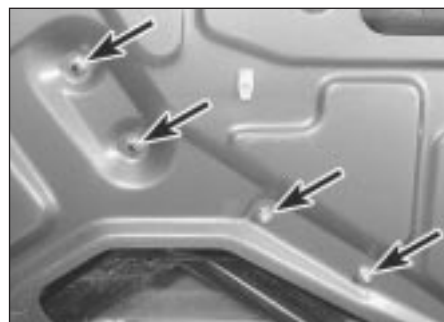
12.2a Window regulator mounting nuts (arrowed)
