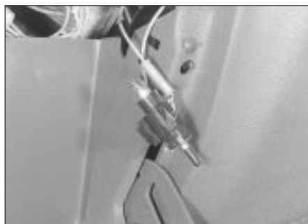
4.26 Glovebox illumination switch
