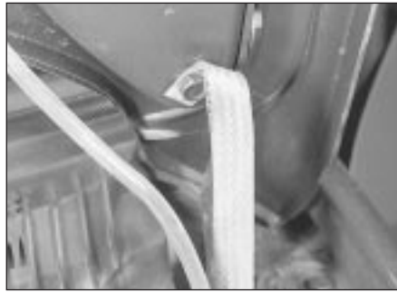
6.3 Braided lead fitted to the bonnet
