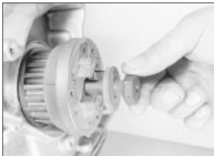
8.11a Remove the crankshaft sprocket bolt . . .
