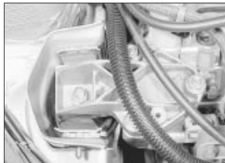
8.6 Right-hand engine mounting and cylinder head bracket
