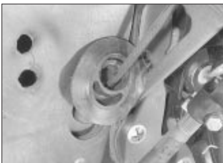
7.3b Speedometer cable grommet on the bulkhead
