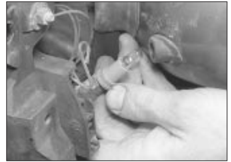
8.9 Removing the front parking light bulbholder
