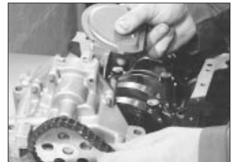
10.3 Removing the oil pump
