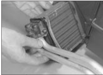
9.6b . . . then withdraw the matrix from the heater casing
