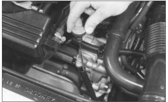
5.1 Withdrawing the automatic transmission fluid dipstick
