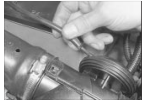
2.9 Disconnect the hose from the vacuum motor
