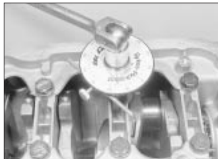
13.75b . . . then angle-tighten them through the specified Stage 2 angle
