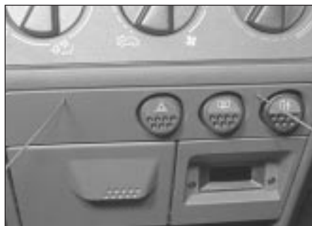
4.13b Insert lengths of rod into the special holes . . .
