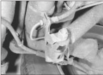
10.2 Rear shock absorber bottom mounting
