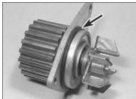
8.18b . . . then recover the O-ring seal (arrowed)
