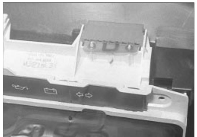
5.6b Instrument panel right-hand upper multiplug
