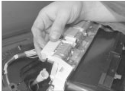
5.17 . . . and disconnecting the wiring plugs
