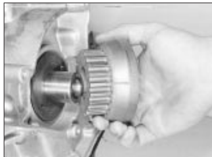
8.11b . . . then slide off the sprocket
