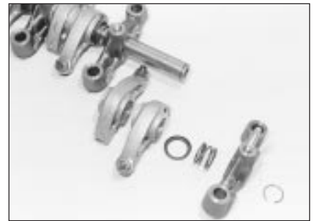
10.4 Remove the circlip, and slide the components off the end of the rocker shaft
