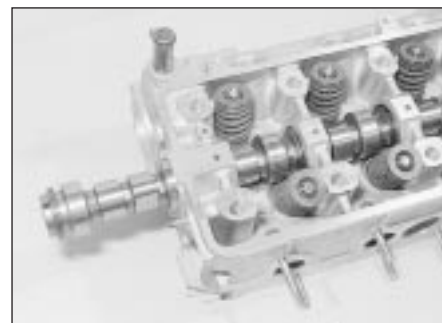
6.8 Removing the camshaft
