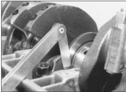
8.7 Checking crankshaft endfloat using feeler blades
