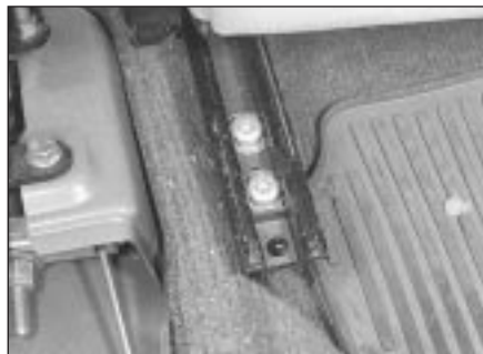
21.1 Front seat rear inner mounting bolts
