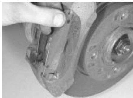
4.5 Removing the outer pad (DBA Bendix caliper)
