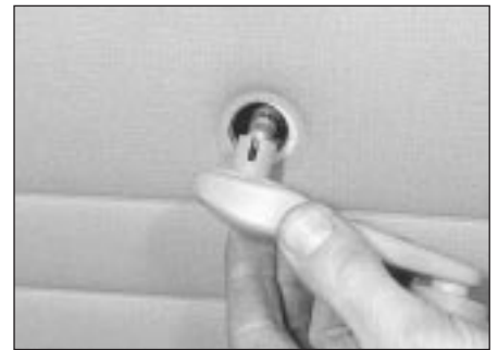
11.4 Removing the window regulator handle
