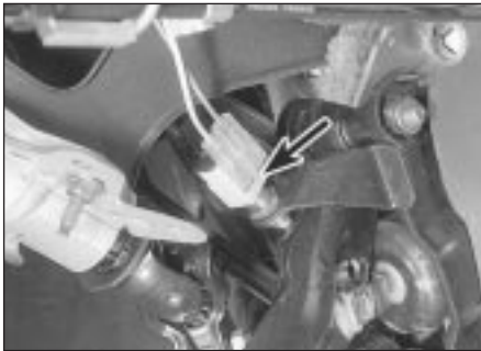
4.35 Brake stop light switch wiring connector (arrowed)
