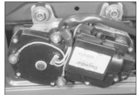
16.6 Tailgate wiper motor and mounting bolts
