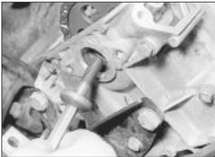
7.23 Unscrew and remove the camshaft sprocket bolt
