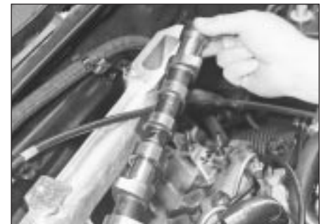
7.9 Lift the camshaft from the cylinder head
