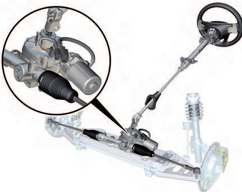
Electric power steering EPS
