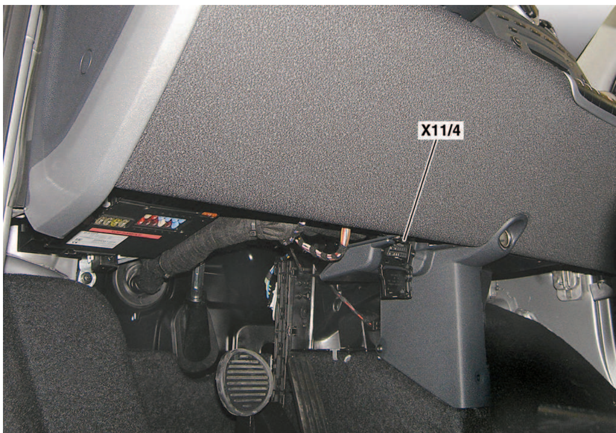
Location of data link connector (X11/4)
