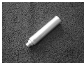
Lower casing cover barrel bearing installer,
