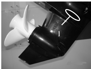
1. Oil level plug screw
