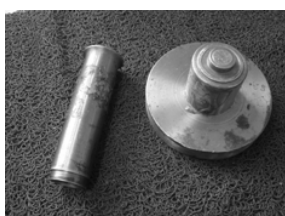
Forward gear bearing installer
