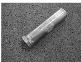
Housing oil seal installer
