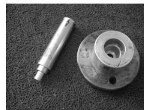
Bearing block copper sleeve installer
