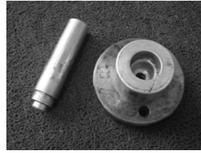
Bearing block oil seal installer
