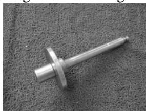
Rolling needle bearing installer
