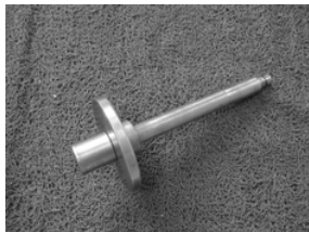
Rolling needle bearing installer
