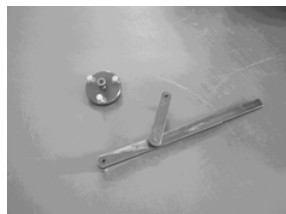
Flywheel gripper and flywheel puller
