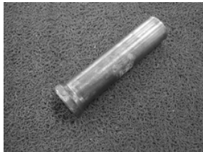
Housing oil seal installer
