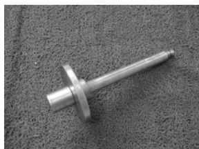
Needle bearing installer
