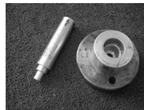
Bearing block copper sleeve installer
