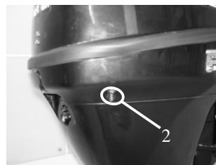
2. Cooling water checking hole
