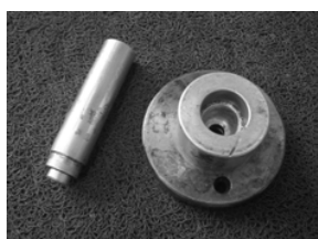
Bearing block oil seal installer
