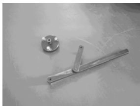
Flywheel gripper and puller
