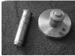
Forward gear bearing installer
