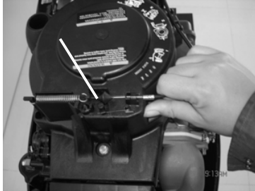
1. Start-in-gear protection device cable
