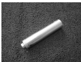
Lower casing cover oil seal installer
