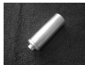
Lower casing cover bearing installer
