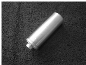
Lower casing cover bearing installer
