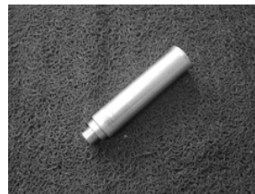
Lower casing cover barrel bearing installer
