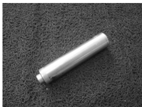
Lower casing cover oil seal installer
