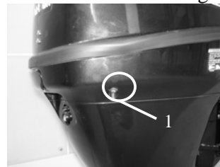
1. Cooling water checking hole
