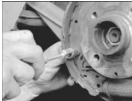
6.6a Remove the front shoe hold-down spring . . .
