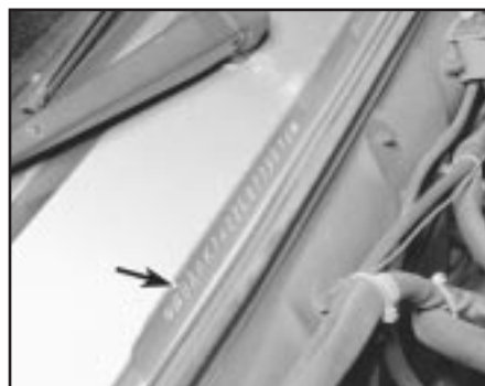
The VIN (arrowed) is stamped on the bulkhead
