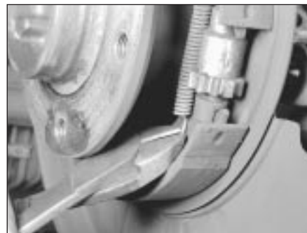
12.7a Remove the lower shoe return spring (diagonal cutting pliers are being used here because they grip the spring well, but care must be taken not to cut or nick the spring)
