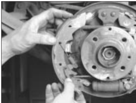
6.7 Remove the front shoe, automatic adjuster lever and spring as an assembly, then remove the lever and spring, and set them aside for attachment to the new shoe
