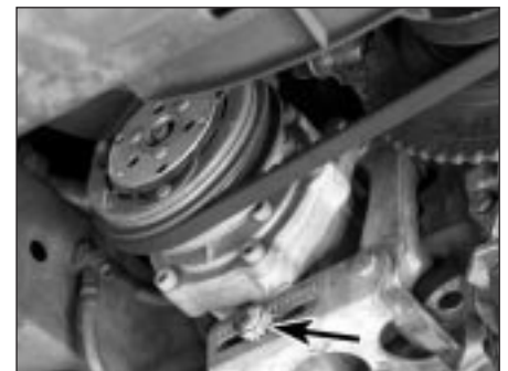
11.6 Loosen the nut on the other end of the adjuster bolt (arrowed) and turn the bolt to increase or decrease tension on the drivebelt
