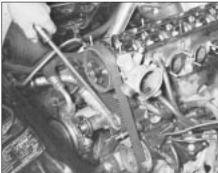
10.21 On the M20 engine, after the belt has been installed correctly around all sprockets and the tensioner pulley, lightly apply pressure to the tensioner, to be sure the tensioner isn't stuck and has full movement against the timing belt
