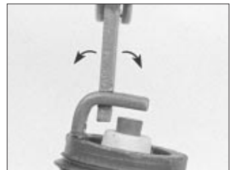
14.4b To change the gap, bend the earth electrode only, as indicated by the arrows, and be very careful not to crack or chip the porcelain insulator surrounding the centre electrode
