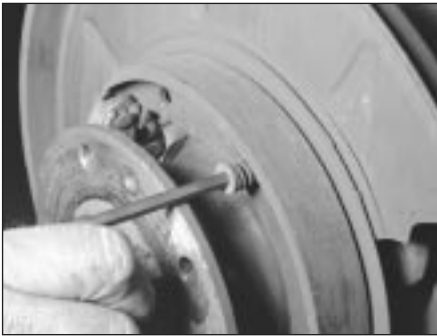
12.7c Remove the shoe hold-down springs
