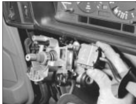
6.6 Squeeze the wiper/washer switch tabs and pull it directly out of the mounting
