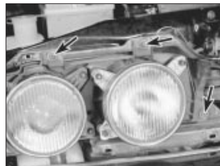
14.4 Remove the screws (arrowed) and detach the headlight housing
