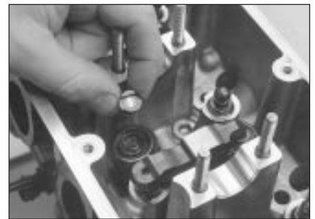
8.20b . . . and thrust discs . . .
