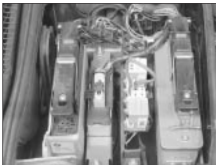
3.6d . . . then, use a jumper wire to bridge the terminals on the connector that correspond to fuel pump relay pins 30 and 87
