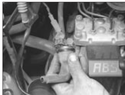
6.8 When the ignition is switched on, there should be a distinct "click" from the purge valve
