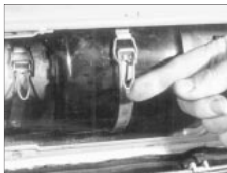
9.5a Unclip the retaining strap to remove the blower housing . . .
