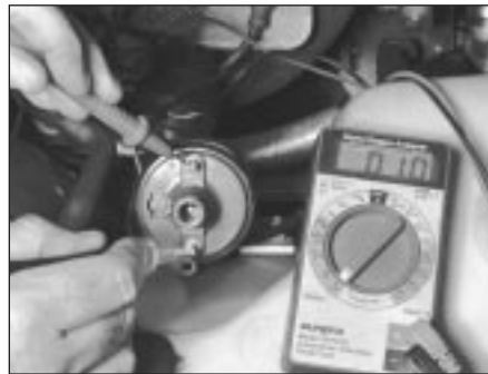
9.4a Using an ohmmeter, measure the resistance between the primary terminals of the ignition coil (TCI system shown)
