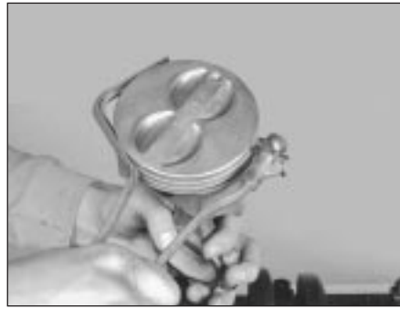
18.4 The piston ring grooves can be cleaned with a special tool, as shown here
