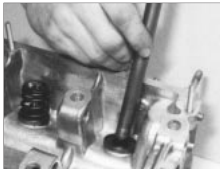
11.4b . . .then lightly drive on the seal with a socket or piece of tubing
