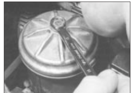
6.17a Unscrew the bolt . . .
