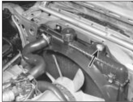
4.8 The radiator is bolted to the front panel at either the sides or the top of the radiator
