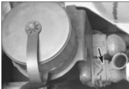
12.7a On later 3-Series models, the pulse sensor connector (arrowed) is located next to the 20-pin diagnostic connector
