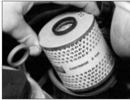
6.17c ... and lift out the cartridge
