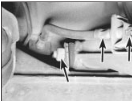
13.3 Disconnect the rear brake hose (middle arrow) from the metal brake line fitting (right arrow) at this bracket on the trailing arm, then plug the line and hose immediately; the other arrow points to the nut for the inner pivot bolt
