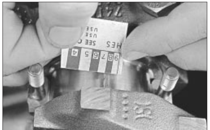
26.17 Measuring the width of the crushed Plastigage to determine the big-end bearing oil clearance (be sure to use the correct scale - standard and metric ones are included)
