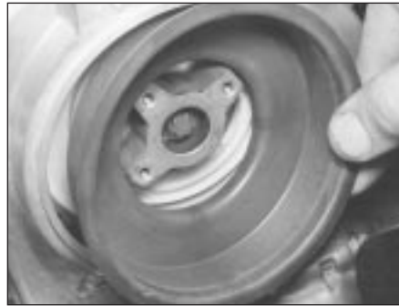
9.6c ... and remove the black plastic cover
