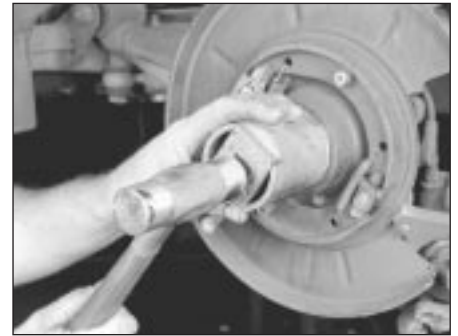
15.14a To refit the new bearing, use a large socket or a piece of pipe with an outside diameter the same diameter as the outer race of the bearing - don't apply force to the inner race - and make sure the bearing is fully seated against the back of its bore
