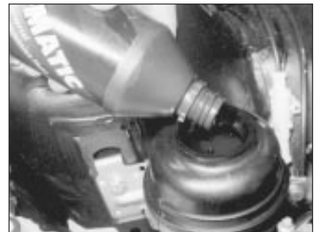
7.6 Adding fluid to the power steering reservoir
