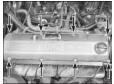
4.6b Valve cover bolt locations (arrowed) on M20 six-cylinder engines
