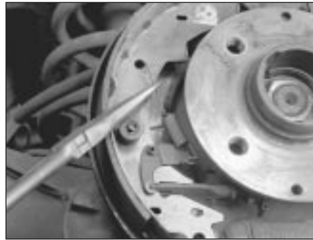
6.13b . . . then hook the lower end of the spring onto the lever as shown; stretch the spring, and hook the upper end into its hole in the handbrake shoe
