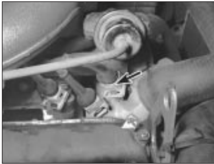
4.1 The coolant temperature sensor (arrowed) is usually located next to the temperature sender unit, near the fuel pressure regulator
