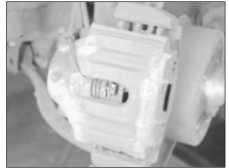
26.11 Look through the caliper inspection window to inspect the brake pads - the pad lining which rubs against the disc can also be inspected by looking through each end of the caliper
