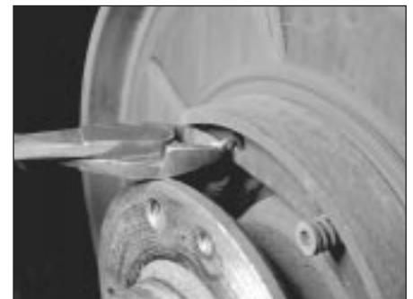
12.7b Remove the upper shoe return spring
