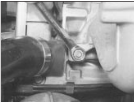
5.14b Removing the lower intake manifold nuts (M40 engine)
