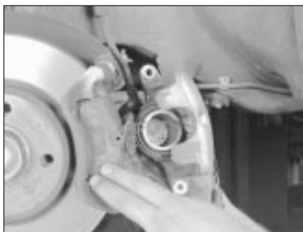
3.5d Remove the caliper, brake pad wear sensor and inner pad all at the same time (3-Series), then refit the inner pad on the piston and press the piston fully into the bore with a C-clamp
