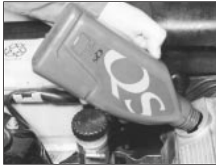
4.6b Topping-up the engine oil
