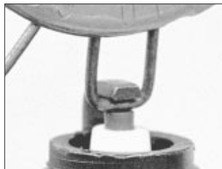
14.4a Spark plug manufacturers recommend using a wire-type gauge when checking the gap - if the wire does not slide between the electrodes with a slight drag, adjustment is required
