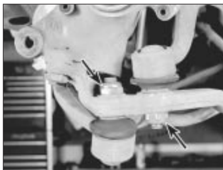
4.7a Remove the self-locking nut (control arm nut, left arrow; thrust arm nut, right arrow) from the balljoint, then support the steering arm, and press or knock the balljoint out of the steering arm
