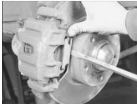
3.5h Prise off the anti-rattle spring (5-Series)
