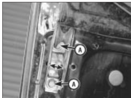
10.18 Loosen the bolts (A) and adjust the roller guide from side to side until it engages securely in the catch
