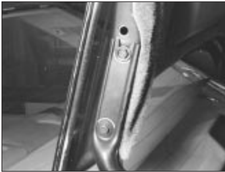
14.3 Mark around the hinge bolts so you can refit the boot lid in its original location - unscrew or loosen the boot lid-to-hinge bolts to remove or adjust it
