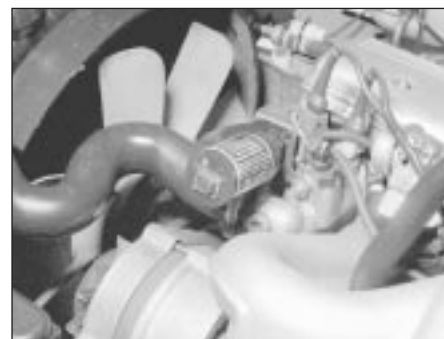
34.2b An aftermarket service light resetting tool such as this one can be plugged into the service connector and used to reset the service lights
