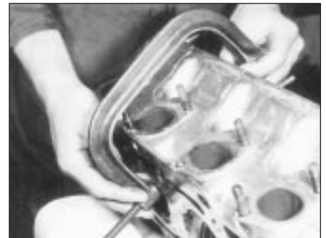
8.22 Using a valve spring compressor to compress a valve spring
