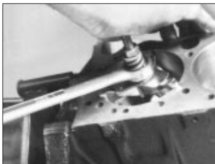
12.1 A ridge reamer is required to remove the ridge from the top of each cylinder - do this before removing the pistons!
