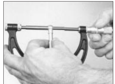
16.4c The gauge is then measured with a micrometer to determine the bore size
