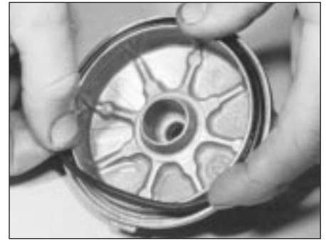
6.19 Renewing the rubber O-ring in the cover
