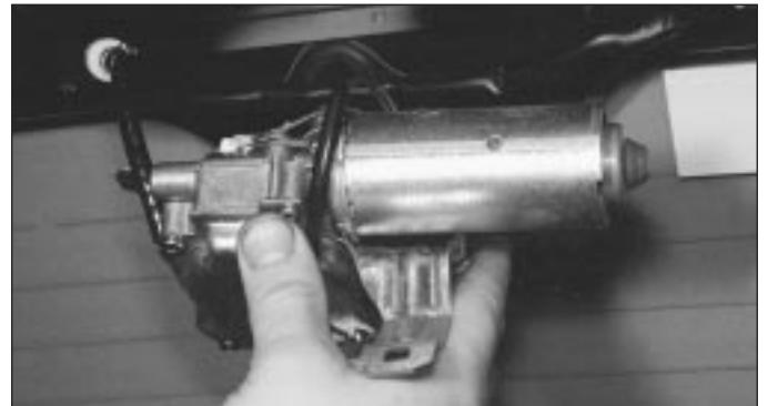
16.11a Removing the tailgate wiper motor (3-Series)
