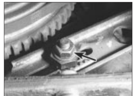
22.6a Typical 3-Series power steering pump adjusting bolt (arrowed) . . .
