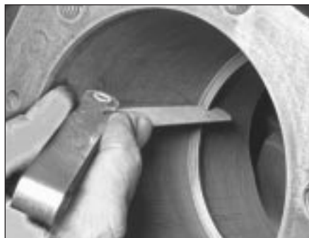
22.4 With the ring square in the cylinder, measure the end gap with a feeler gauge
