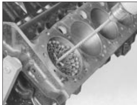
17.4 A “bottle brush” hone will produce better results if you’ve never honed cylinders before
