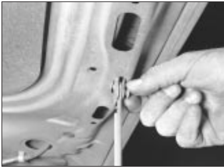
10.3b . . . and pull the hinge pin out while supporting the bonnet
