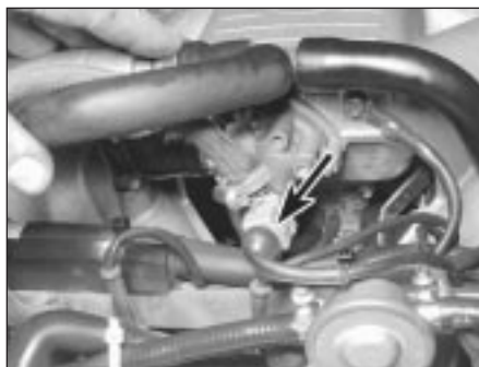
19.1 Cold start injector electrical connector (arrowed) on the M10 engine. Most cold start injectors are mounted in the intake manifold
