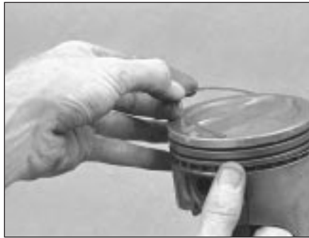
22.9b DO NOT use a piston ring refitting tool when refitting the oil ring side rails
