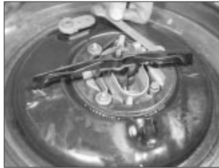
8.6a Unscrew the four air cleaner-to-carburettor nuts . . .
