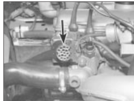
34.2a The earlier 15-pin connector (arrowed) is mounted near the front of the engine. The 20-pin connector used on later models is located in the left rear corner of the engine compartment
