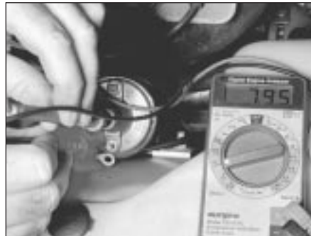
9.5a Using an ohmmeter, measure the secondary resistance of the coil (TCI system)
