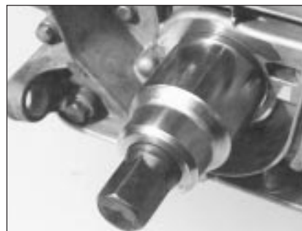
14.32 Using a large socket and the crankshaft pulley bolt to pull the oil seal into the housing (M40 engine)
