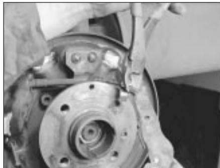
6.9 To disconnect the handbrake cable from the handbrake lever, pull on the plug at the end of the cable, and detach the cable from the bracket on the upper end of the lever (diagonal cutting pliers are being used here because they grip the cable well, but care must be taken not to nick the cable)
