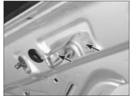
14.7b Adjust the boot lid lock striker after loosening the bolts (arrowed)
