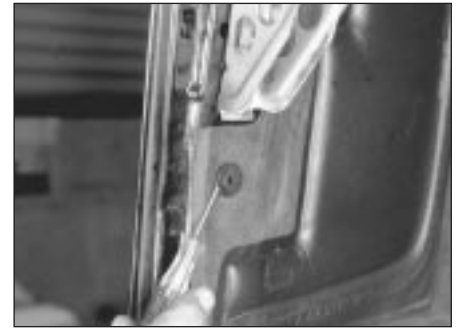
10.8b . . . prise the retainer out
