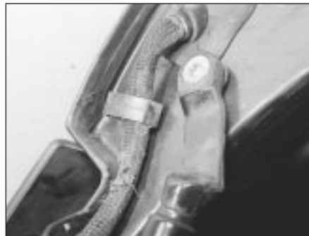
14.12b Strut mounting on the tailgate (5-Series)
