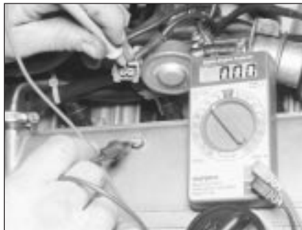
19.3 Check for a voltage signal (about 12 volts) at the cold start injector connector when the starter motor is operated
