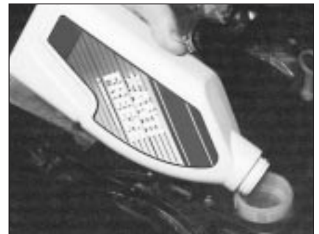
4.9d Adding antifreeze mixture
