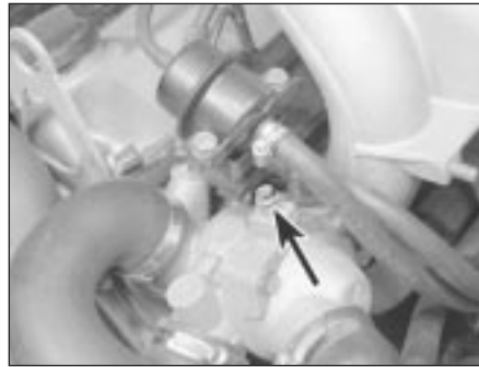
29.16 The bleed screw (arrowed) is located on the thermostat housing (six-cylinder models)
