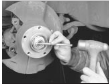
8.3 Using a chisel, knock out the staked portion of the hub nut
