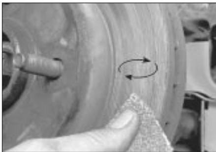
5.4b Using a swirling motion, remove the glaze from the disc surface with sandpaper or emery cloth
