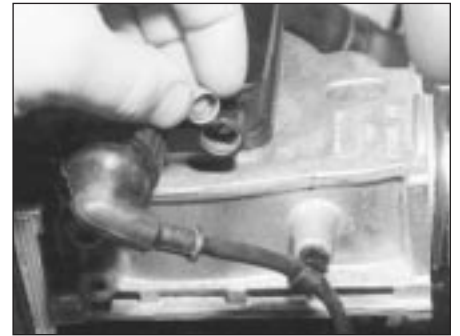
12.12a Removing the tamperproof plug from the airflow meter
