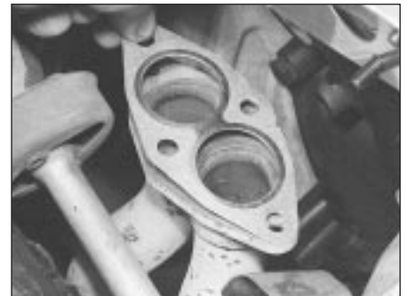
6.7c Removing the exhaust manifold-to-downpipe gasket (M40 engine)
