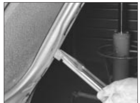
10.3a Use needle-nose pliers to pull off the hinge pin clip . . .
