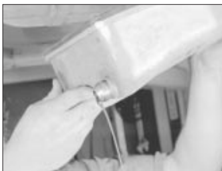
28.7 Lower the sump from the transmission
