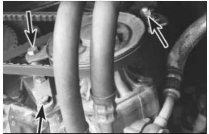
22.6c Typical 5-Series power steering pump mounting bolts (arrowed)
