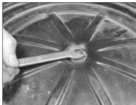
8.2b . . . then remove the air cleaner cover centre nut, and lift off the cover
