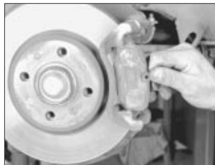
3.5e Remove the outer brake pad (3-Series) - to fit the new pads, reverse the removal procedure
