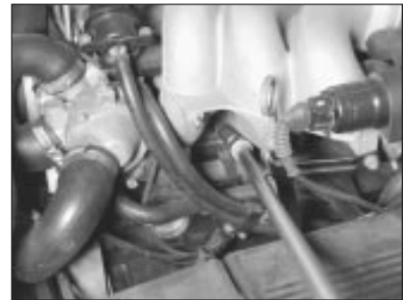
5.14a Remove the intake manifold nuts with a socket, ratchet and long extension (M20 engine)
