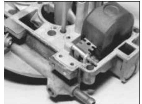
12.12a Tap out the float pivot pins, and remove the floats . . .
