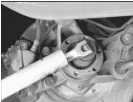
15.8 Lower the vehicle and loosen the drive flange nut
