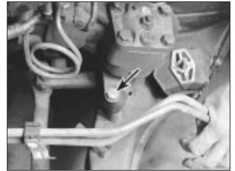
21.10a This bolt (arrowed) secures the steering box to the subframe crossmember. The nut, not visible in this photo, is accessed through a hole in the crossmember (engine removed for clarity, left-hand-drive shown)
