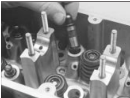
8.20c . . . then lift out the hydraulic tappets
