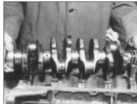
13.6 Remove the crankshaft by lifting straight up. Be very careful when removing the crankshaft - it is very heavy
