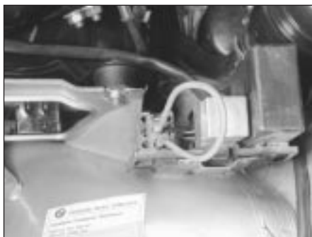
3.6a On L-Jetronic systems, use a jumper wire to bridge the terminals on the connector that correspond to the fuel pump relay pins 30 and 87b
