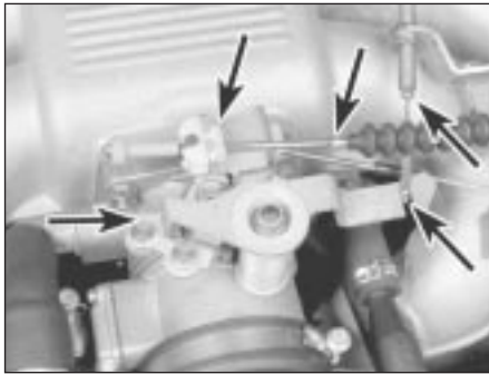
19.3 Check and lubricate the throttle linkage at the points shown (arrowed) - fuel injection engine shown
