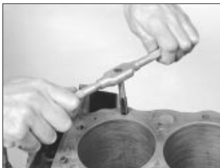
12.24 The cylinder head bolt holes should be cleaned and restored with a tap (be sure to remove debris from the holes after this is done)
