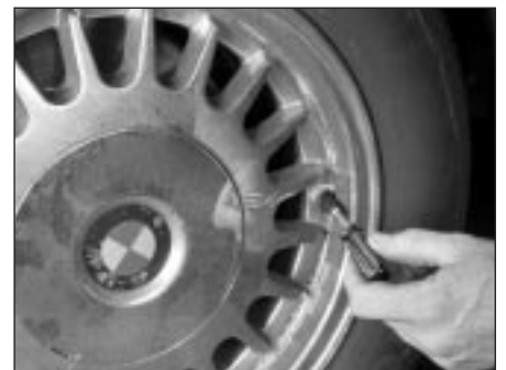
5.4a If a slow puncture is suspected, check the valve core first to make sure it's tight
