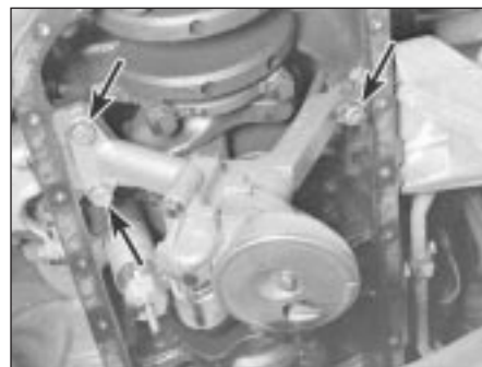
14.3a On M20 engines, the oil pump is bolted across the engine block from side to side, towards the front of the engine
