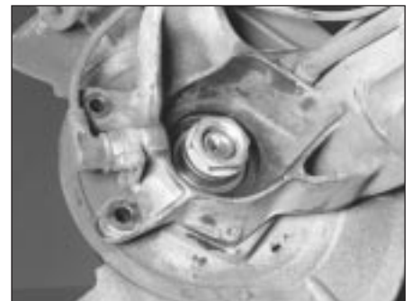
15.14d When you refit the spacer, make sure it's centred on the inner race of the bearing before tightening the nut
