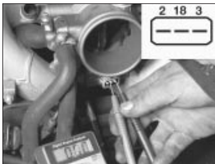
4.28c ... then check for continuity between terminals 3 and 18 as the throttle is opened
