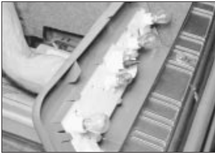
15.4a On 3-Series models, the entire tail light housing assembly is self-earthing through the mounting screw - loosen the plastic screw and pull the housing back . . .
