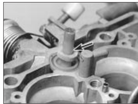
12.15c Accelerator pump seal (arrowed)
