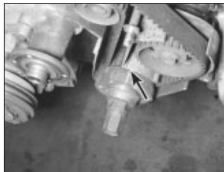
10.5a Align the groove in the hub on the end of the crankshaft with the notch in the front inner cover (arrowed) and mark them for assembly reference later on
