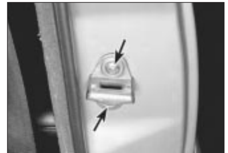
13.7 The door lock striker position can be adjusted after loosening the screws (arrowed)
