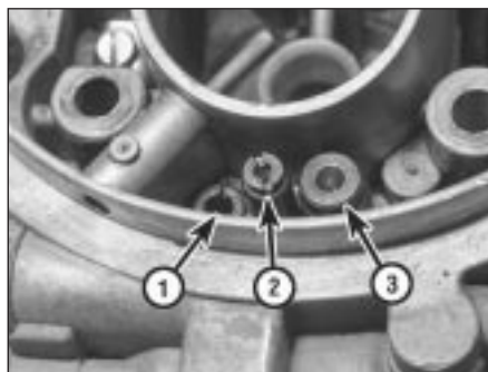
12.13d Secondary bypass air jet (1), TM air jet (2), and air correction jet (3)
