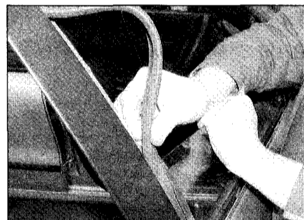
18.5c ... then pull up the rear window glass moulding from the rear guide channel
