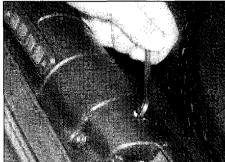
8.8b ... and loosen the striker bolts with an Allen key
