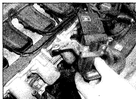
8.7 Move the oil filler tube clear of the inlet manifold
