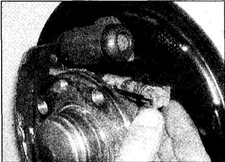
5.27 Removing the self-adjuster mechanism from the trailing shoe
