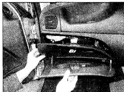
23.20c ... and withdraw the glovebox from the fascia
