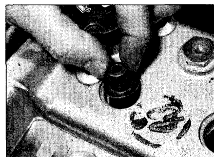
4.21b ... place a suitable washer or similar into the recess to keep the dowel rod vertical ...
