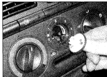
23.13a Pull off the heater ventilation centre control knob ...
