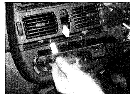
23.15b ... and withdraw the switch panel from the front of the fascia ...
