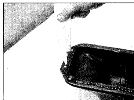
12.4 Applying sealant to the sump flange
