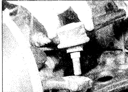
23.2b Separate the track-rod end from the steering arm
