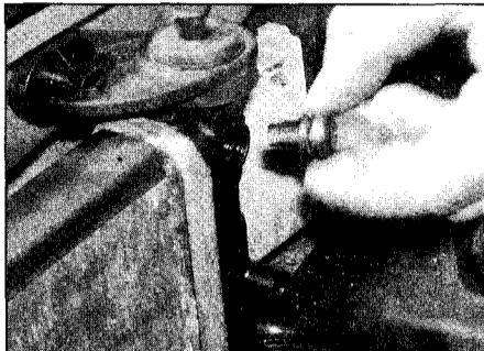
31.3a Opening the radiator bleed screw on a 1.4 litre engine . . .
