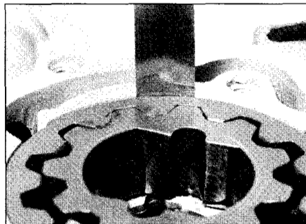
13.9a Measuring oil pump outer gear-to-pump housing clearance
