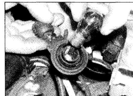
4.14 . . . then depress and twist the bulb to remove it
