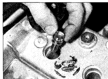
4.21a Screw the spark plug bodies of the home-made piston positioning tools into each spark plug hole ...
