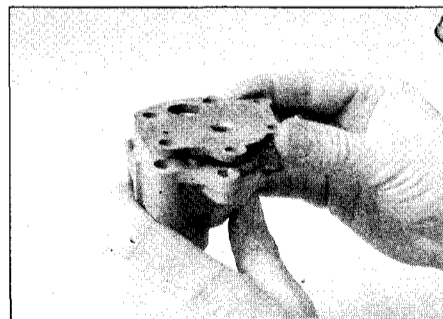
15.8 Remove the adaptor plate from the oil pump body
