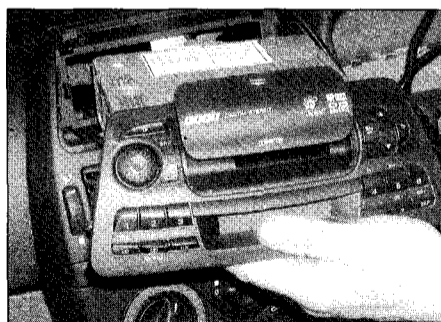
12.3 Removing the radio/cassette from the fascia
