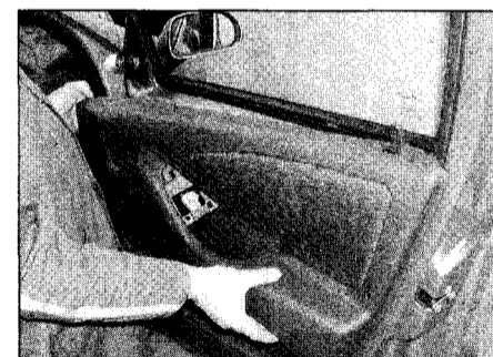
14.5b Lifting the inner trim panel from the door
