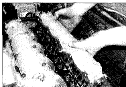
6.14a When removing the housings, tip them over, to prevent the tappets falling out . . .
