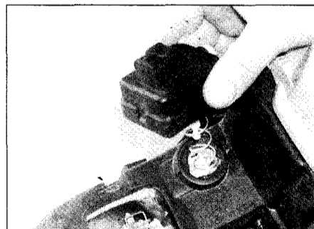
8.3 Removing the headlight beam adjuster from the headlight unit
