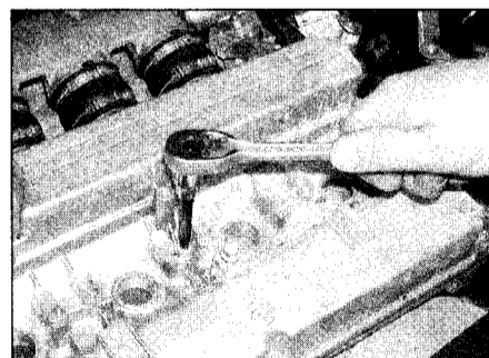
6.10 Removing the camshaft cover bolts
