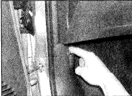
5.40 The inertia switch can be reset without removing the sill trim panel, if required
