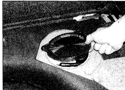
5.3b . . . and take off the dust cover for access to the sender unit
