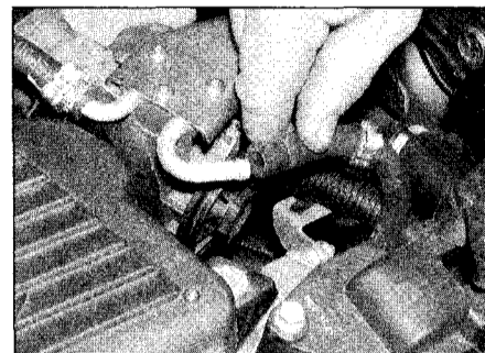
4.6b . . . then disconnect the coolant hoses from the throttle body
