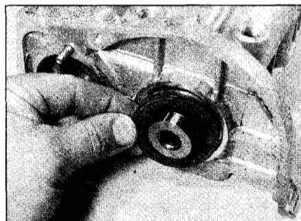
9.16 Fit a new exhaust camshaft oil seal
