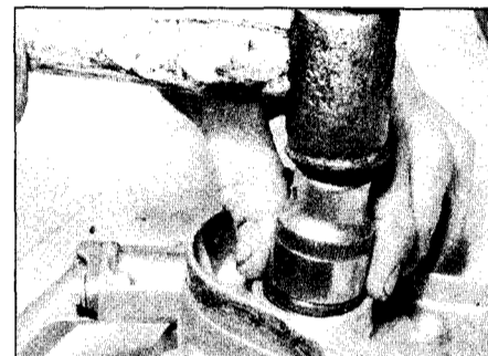
13.13 Using a socket to fit a new oil seal to the oil pump
