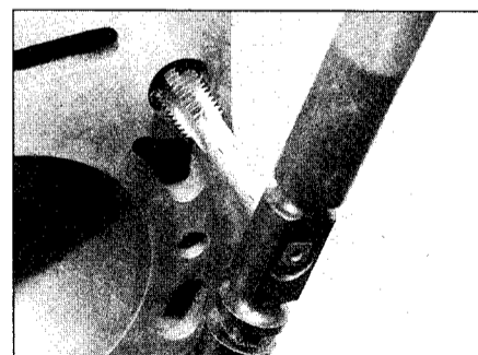
8.8 To clean the cylinder block bolt threads, run a correct-size tap into the holes
