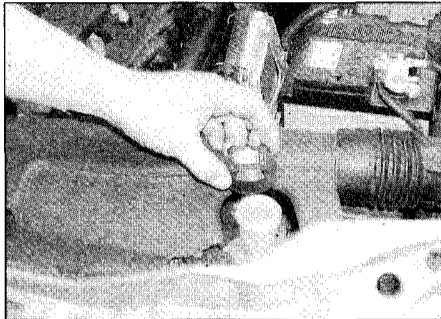
31.24a Remove the expansion tank cap . . .
