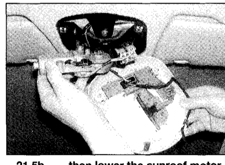
21.5b ... then lower the sunroof motor and interior light/roof switch from the headlining
