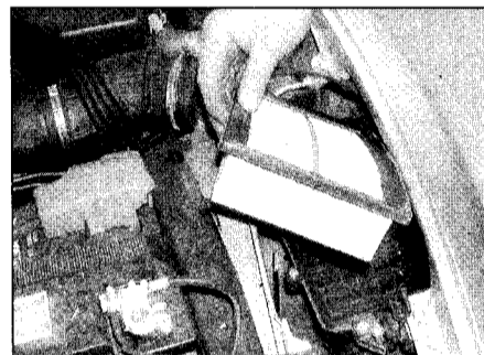
19.3 Lift out the air filter element, noting which way round it fits
