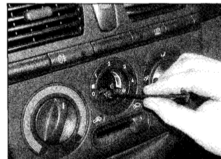
23.13b ... and undo the screw located beneath it
