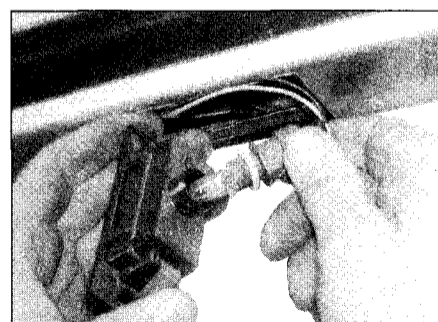
4.39a Twist the bulbholder from the light unit . . .
