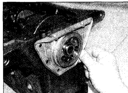
10.27b . . . fit the flange and seal over the end of the crankshaft . . .
