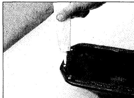
14.7a Run a bead of sealant around the sump flange . . .
