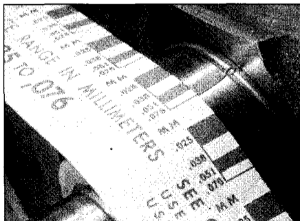
11.15 Measure the width of the crushed Plastigauge, using the scale provided
