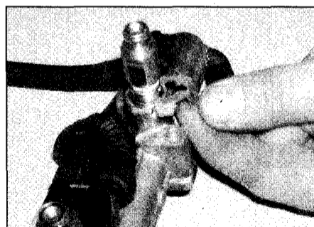
4.18b . . . slide out the locking clip (where fitted) . . .
