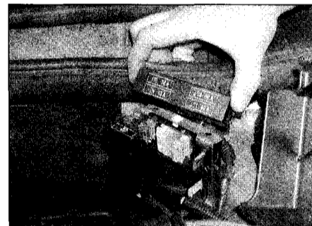
4.64a Remove the fusebox lid at the rear of the engine compartment ...
