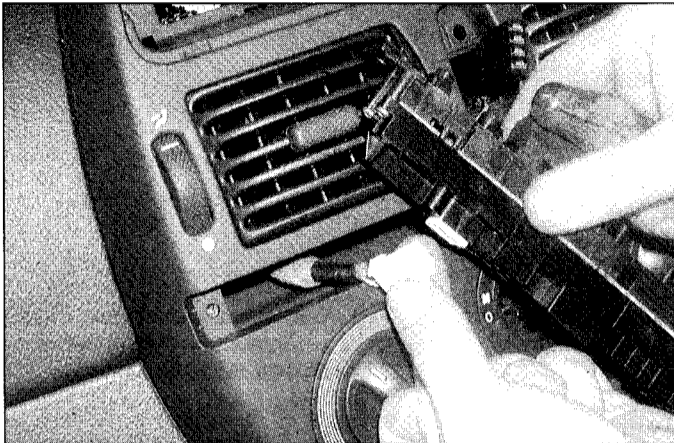
23.15c ... then disconnect the wiring
