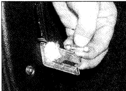
5.14 ... and extract the festoon-type bulb from the spring contacts
