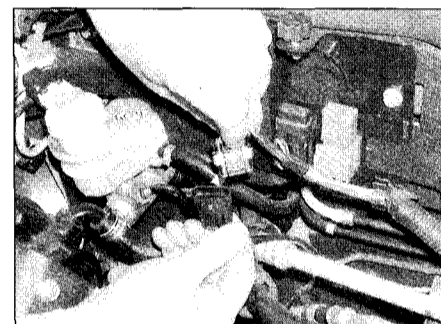
11.11b . . . then locate and disconnect the wiring plug for the oxygen sensor
