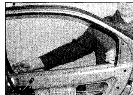
18.17 Removing the rear door window glass
