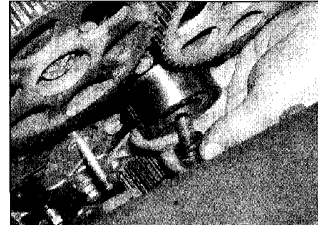
5.33 Removing the fixed guide pulley
