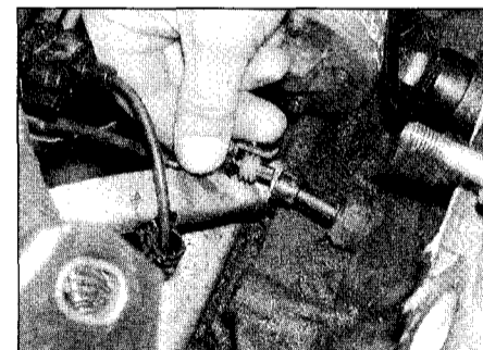
14.2 Disconnect the switch wiring connector
