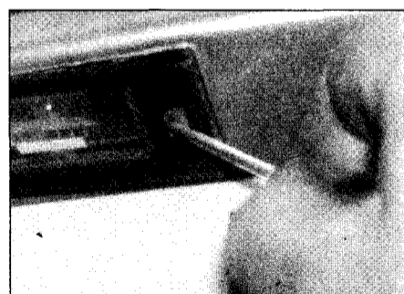
4.38 Use a screwdriver to depress the plastic retainer on the rear number plate light
