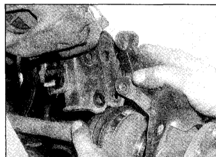
2.9b . . . separate the hub carrier from the bottom of the strut . . .
