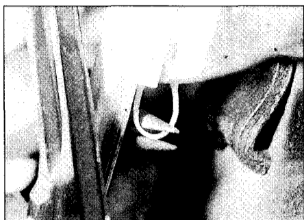
18.3a Using a pair of pliers to unclip the plastic fastener that secures the front window glass to the regulator mechanism
