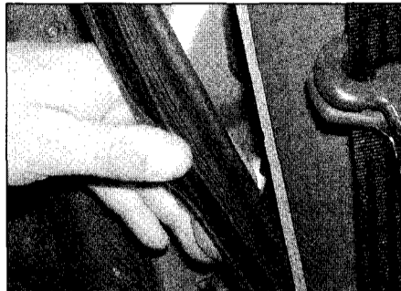
20.12 Pull the door weatherstrips away from the B-pillar
