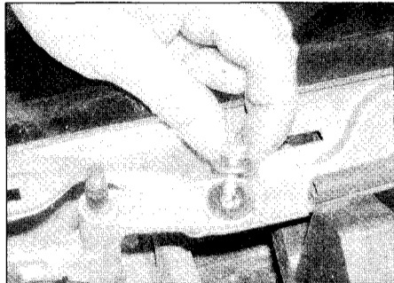
18.6b Wiper mounting bolt located on the linkage frame
