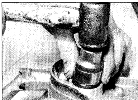
13.13 Using a socket to fit a new oil seal to the oil pump
