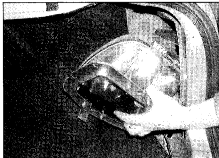
6.18b . . . then withdraw the rear light cluster from inside the loadspace
