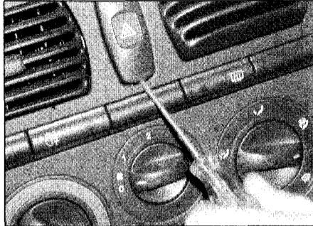
14.33a Use a screwdriver to prise the hazard warning switch . . .
