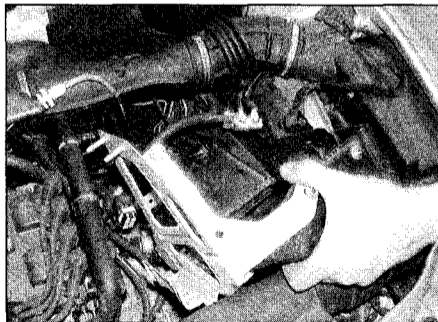
2.8 Removing the battery tray
