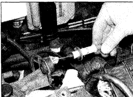
4.4b . . . and release the cable from the mounting bracket
