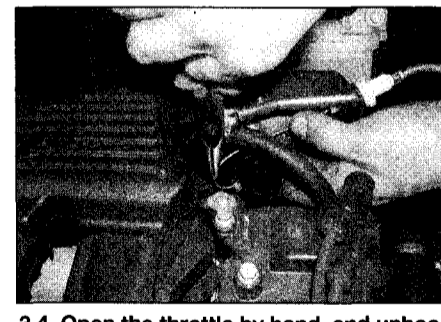
3.4 Open the throttle by hand, and unhook the cable end fitting from the throttle quadrant
