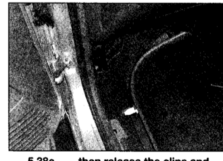
5.38c ... then release the clips and remove the sill trim panel
