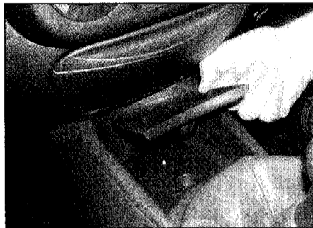
23.4a Remove the covering from the odds tray in the centre console . . .
