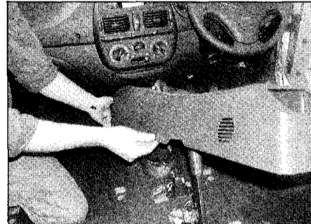
23.7e ... then withdraw the centre console over the handbrake lever
