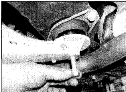
13.14 Removing the engine rear mounting through-bolt
