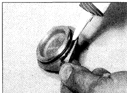
9.22b . . . then apply RTV gasket sealant to the cover plate contact face
