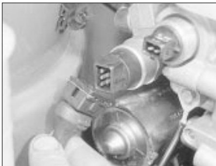
15.3d Disconnecting the pressure switch multi-plug
