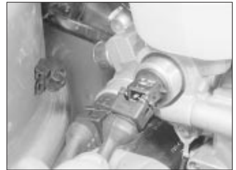
15.3c Disconnecting the main valve plug
