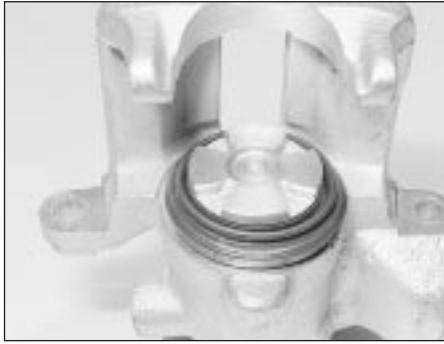
12.21 Dust boot fitted to caliper and piston
