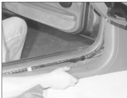
41.30 Removing the passenger side lower kick panel
