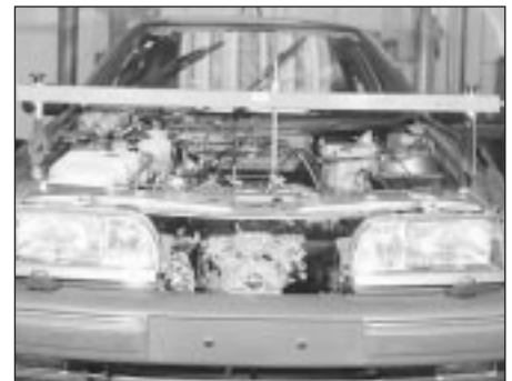
10.28a Using an engine support bar to support the engine
