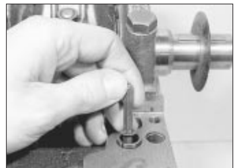
19.4 Removing the oil pump driveshaft
