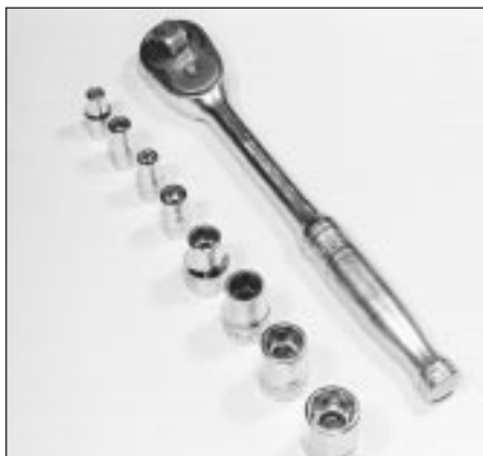
Sockets and reversible ratchet drive
