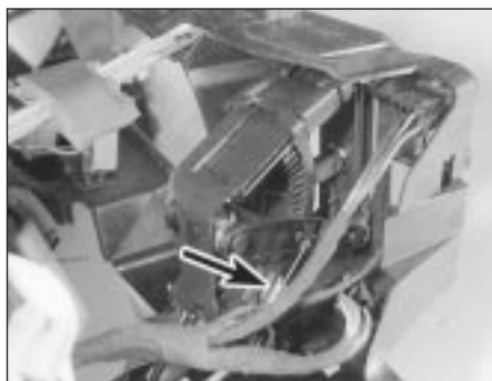
17.4 Heater control cable clip (arrowed) viewed through windscreen
