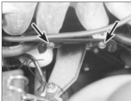
40.35 Two bolts (arrowed) secure the bracket to the manifold; the bolts securing it to the block are hidden
