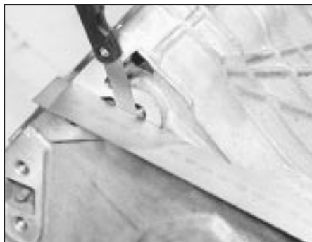
25.15 Measuring the clearance between the cylinder block and sump end faces
