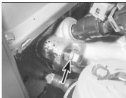
40.40b Use two nuts locked together (arrowed) to remove the stud
