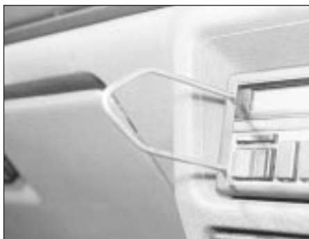
30.9 A DIN extraction tool fitted to a radio/cassette unit
