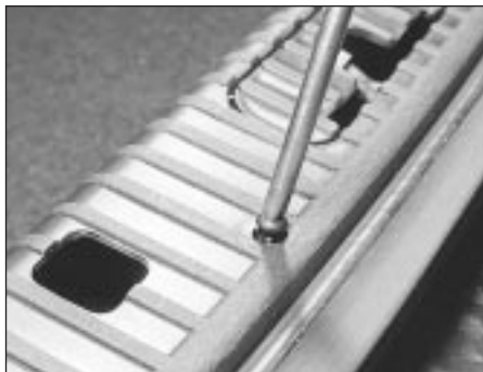
7.4a On early models it will be necessary to remove the luggage compartment rear trim panel to gain access to the fuel cut-off inertia switch . . .
