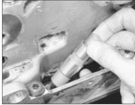
18.11 Lifting the chain tensioner plunger assembly from the cylinder head
