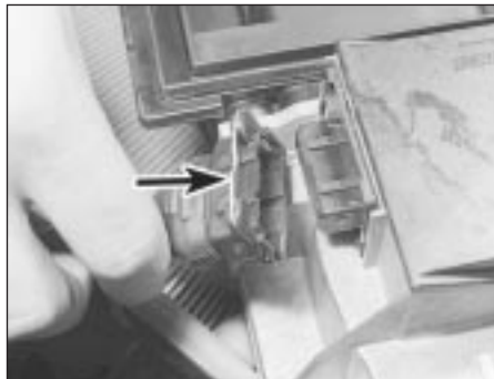
35.2 Disconnecting the airflow meter multi-plug. Meter is inverted to show locking clip (arrowed)
