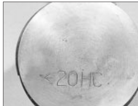
37.4b Piston crown markings Arrow points to front of engine
