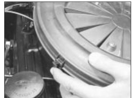
38.2 Releasing an air cleaner cover clip (carburettor model)
