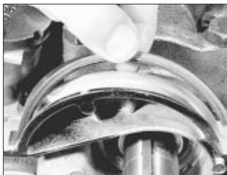
39.1b Fitting the rubber strip into its groove
