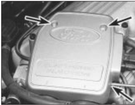
9.5a Three screws (arrowed) secure the throttle linkage cover
