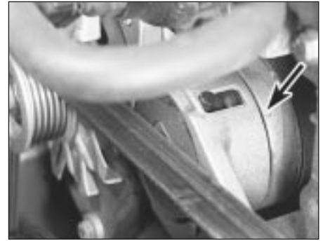
21.14b Water pump/alternator drivebelt tensioner wear indicator location (arrowed) - DOHC engine
