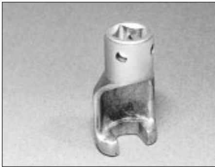
23.11 Cutaway socket spanner
