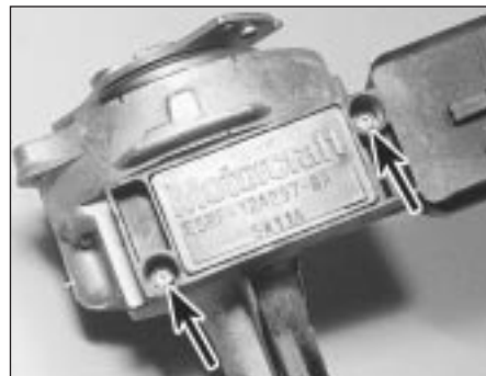
15.4 Two screws (arrowed) which secure the ignition module
