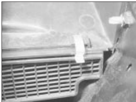
29.4 One of the plenum chamber cover clips
