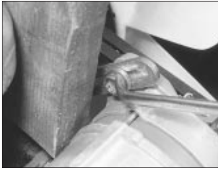
21.8 Tightening the alternator strap bolt
