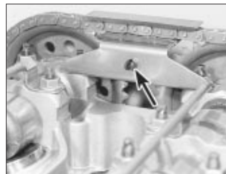
18.7 Upper timing chain guide securing lugs (arrowed)
