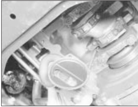
12.6 Removing the oil pump and driveshaft
