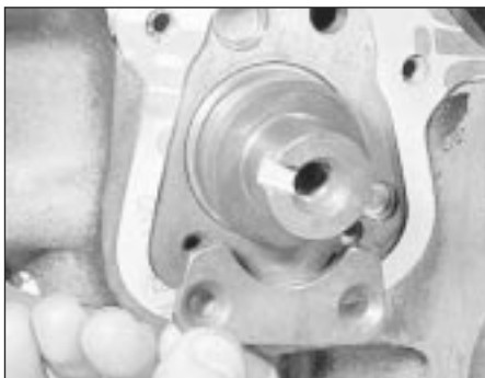
14.5a Removing the auxiliary shaft thrust plate
