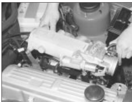
40.40a Removing the inlet manifold
