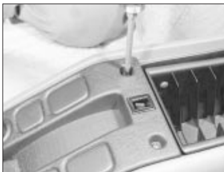
42.7 Removing a switch panel screw (high series)
