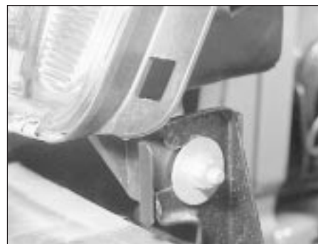
4.6c Headlight side mounting nut
