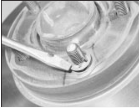
5.3 Disc-securing spring clip
