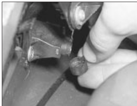
31.18 Remove the cover from the mixture adjustment potentiometer
