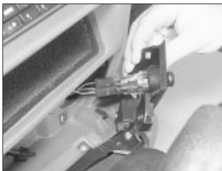
41.25 Withdraw the cigarette lighter and disconnect the wiring plugs
