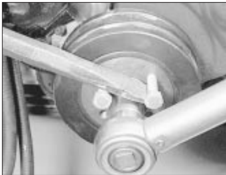
45.16 Holding the crankshaft pulley with two bolts and a lever while tightening the central bolt
