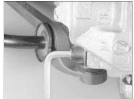
7.4 Undoing a caliper slide bolt
