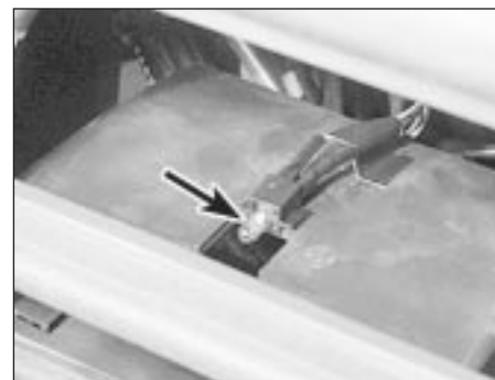
6.26 Ashtray light bulb seen through radio aperture
