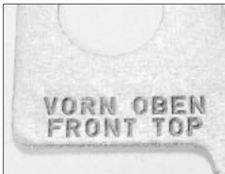
38.3 Cylinder head gasket markings
