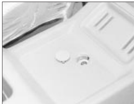
42.3 The central console securing screw (low series)
