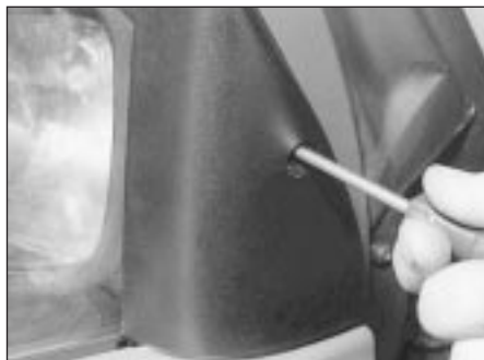
22.6 Removing the mirror mounting trim screw
