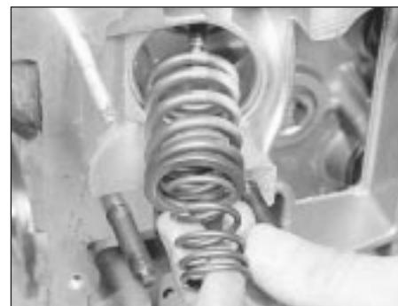
19.1 Withdrawing the double valve springs from the cylinder head
