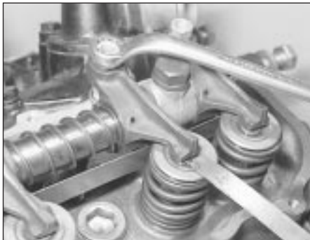
23.20 Adjusting a valve clearance - V6 engine
