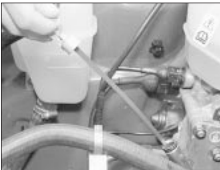
17.3 The automatic transmission dipstick
