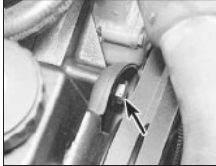
11.4 Steering pump pivot bolt (arrowed) - V6 model shown
