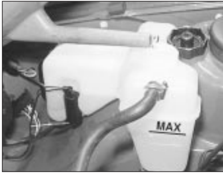
3.9 Topping up the cooling system
