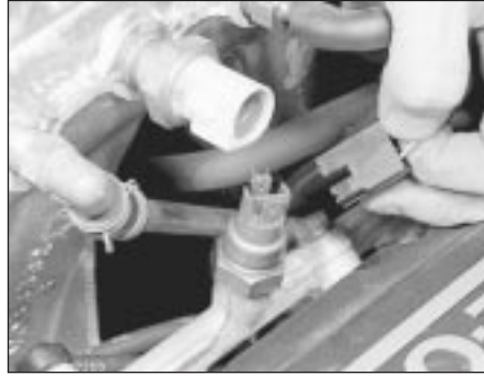
26.3 Disconnecting the fuel temperature sensor wiring plug
