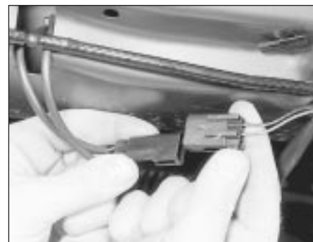
6.8 On later models disconnect the washer nozzle heater wiring plugs before removing the bonnet
