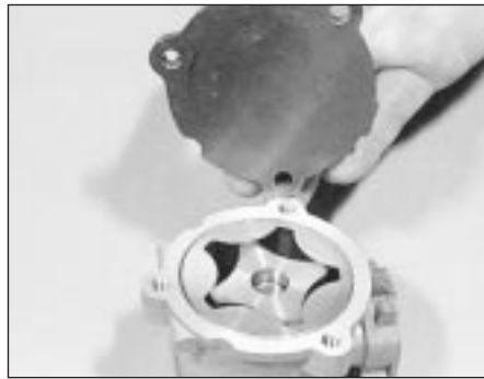
26.1 Removing the oil pump cover
