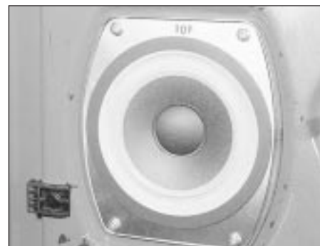
31.4 Front door loudspeaker - note TOP marking
