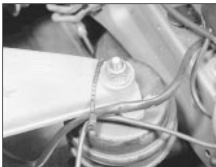
10.28b Engine mounting top nut
