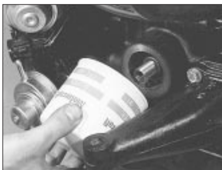
8.6 Fitting an oil filter
