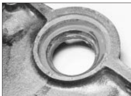
36.1 Timing cover oil seal
