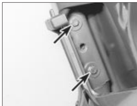
9.3 Boot lid retaining bolts (arrowed) - Saloon models
