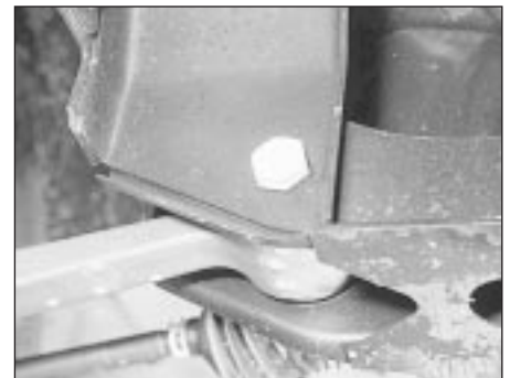
15.3 Front suspension lower arm pivot bolt
