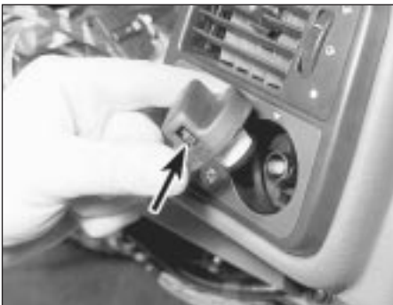
41.20 Depress the tang (arrowed) and pull off the light switch control knob
