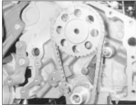
36.18 Fitting timing chain and sprockets
