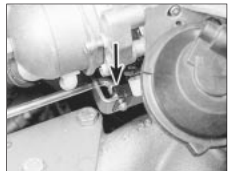
12.4 Throttle arm-to-lever clip (arrowed)
