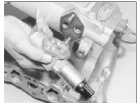
34.3 Removing the idle speed control valve
