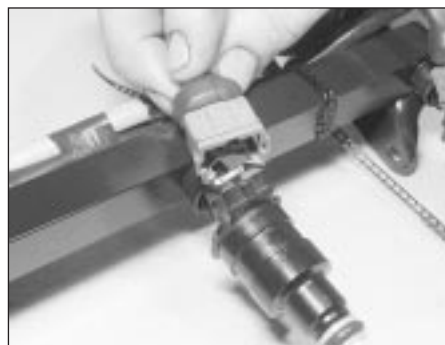
36.11 Disconnecting a fuel injector multi-plug
