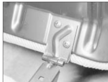
49.1 Rear seat hinge-to-cushion screws
