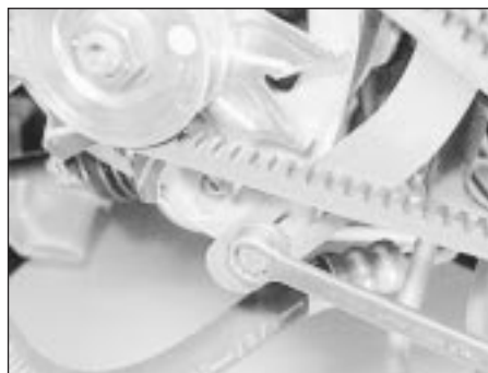
36.39a Alternator drivebelt tensioner strap bolt
