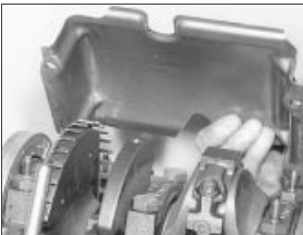
29.3 Withdrawing the oil baffle
