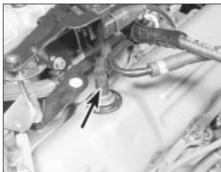
8.23 Rocker cover breather hose (arrowed)
