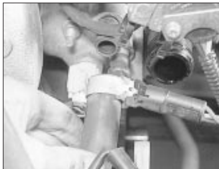
17.5 Disconnecting the heater coolant hose from the inlet manifold
