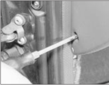
41.34a Facia left-hand mounting screw
