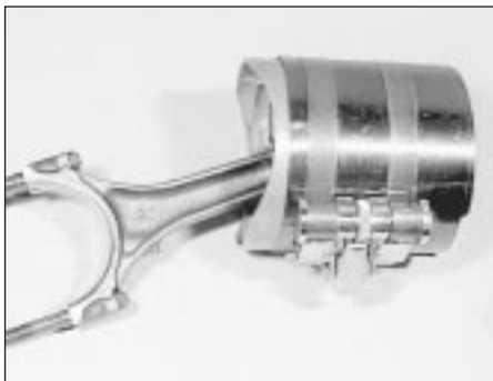
33.6a Piston with ring compressor fitted
