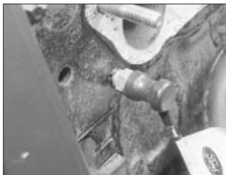
15.1a Temperature gauge sender (manifold removed)
