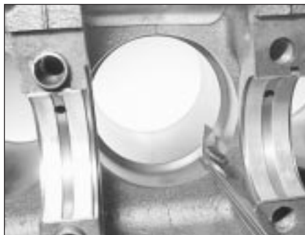
29.4b Checking a ring gap at the bottom of the cylinder
