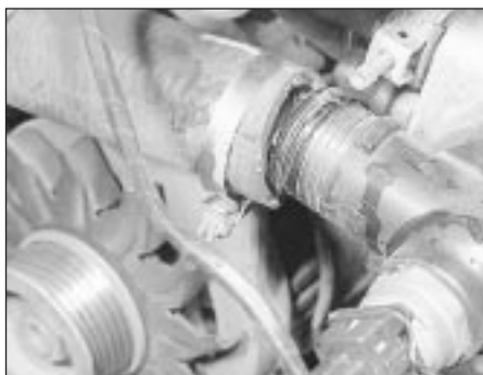
7.12b . . . from the thermostat housing
