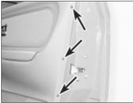
22.1 Three screws (arrowed) secure the rear edge of the front door trim panel
