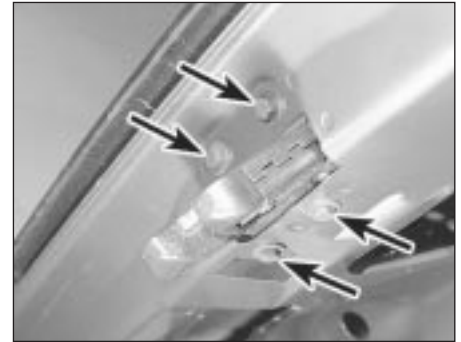
18.4 Boot lid lock retaining bolts (arrowed) - Saloon models
