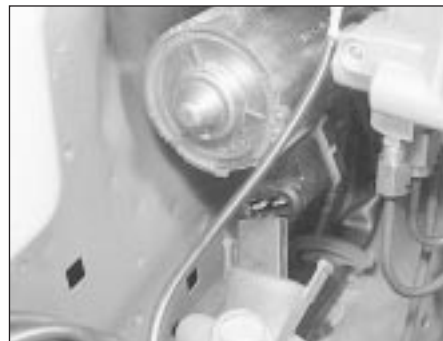
15.3e Disconnecting the pump motor plug
