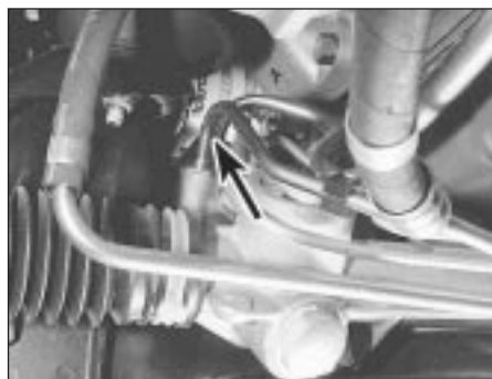
3.17 Clamp plate bolt (arrowed) is located between two fluid pipes
