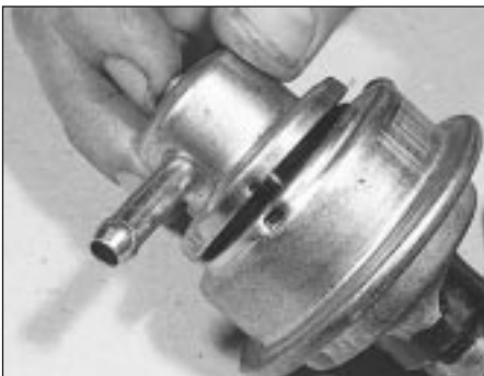
4.8a Removing the fuel pump cover - note alignment indentations
