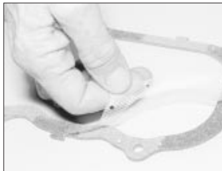
38.21 Peeling off rocker cover gasket protective shield
