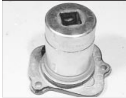
41.3b Fitting a new oil seal in the auxiliary shaft cover
