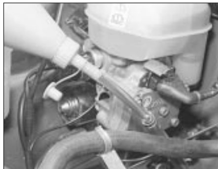
17.4 Topping up the transmission fluid
