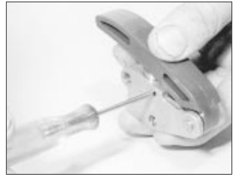
36.20 Releasing timing chain tensioner pawl
