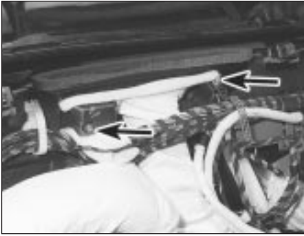
19.19 Release the facia wiring loom from the bulkhead to gain access to the demister nozzle retaining nut and screw (arrowed)
