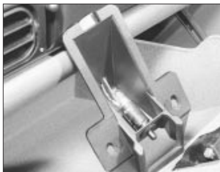
6.23 The glovebox light unit
