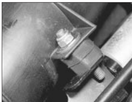
38.17 Air intake tube retaining nut (fuel-injection DOHC)
