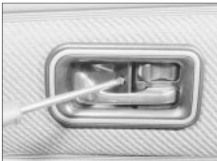
22.5 Removing the door handle surround screw
