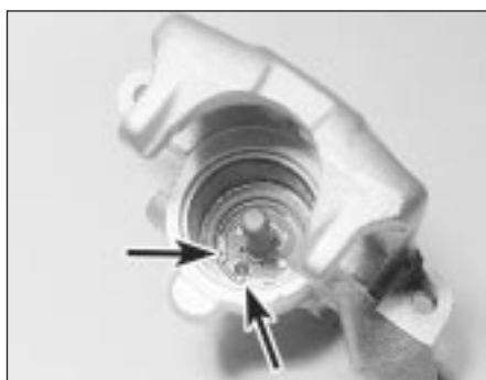
12.8 Remove the circlip (ends arrowed) to release the pushrod and key plate
