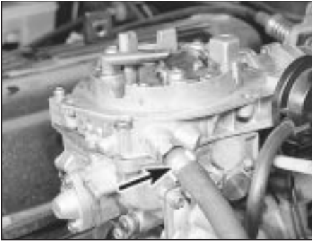
12.5 Crimped hose clip (arrowed) must be renewed
