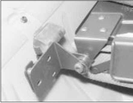
49.3 Rear seat backrest hinges. One of the backrests has been removed
