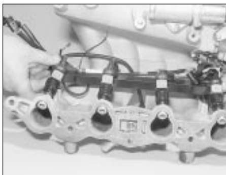
40.42a Removing the fuel rail and injectors from the manifold
