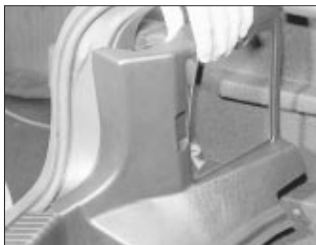
4.16 Remove the trim panel for access to the rear light cluster retaining nuts
