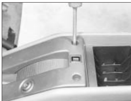
42.19a Slacken and remove the two switch panel retaining screws . . .
