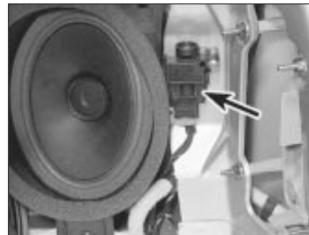
7.3 Fuel cut-off inertia switch location - Estate models
