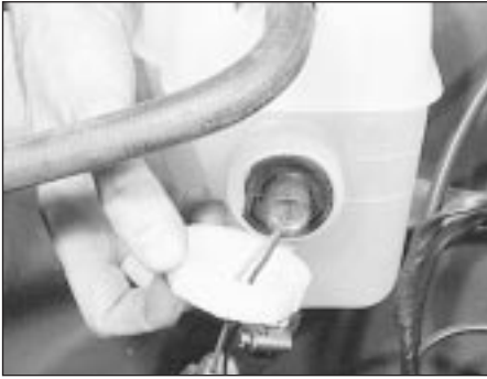
27.16 Removing the coolant level switch
