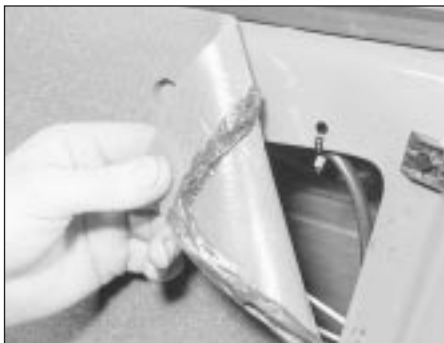
22.8a Peeling back the rubber sheet
