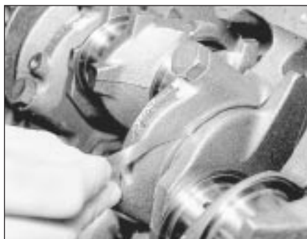
31.13 Checking crankshaft endfloat
