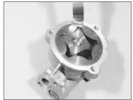
26.2a Checking the outer rotor-to-housing clearance
