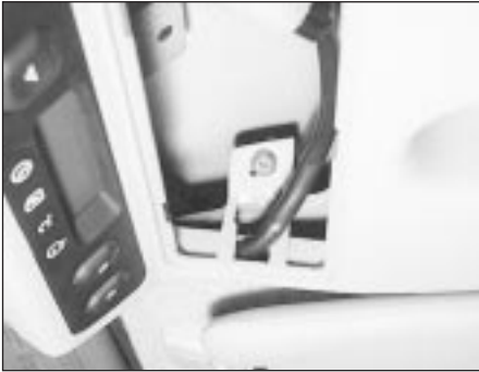
43.4a One of the overhead console retaining screws
