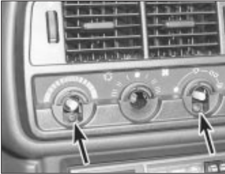
41.18a Remove the control knobs to gain access to the two hidden central vent panel retaining screws (arrowed)
