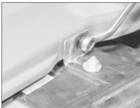
4.6a Headlight top mounting screw
