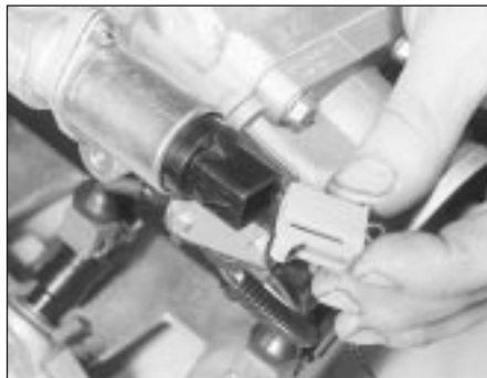
34.2 Disconnecting the idle speed control valve
