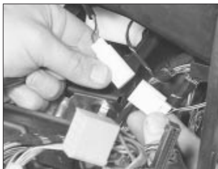
41.32 Disconnect the alarm warning LED wiring connector
