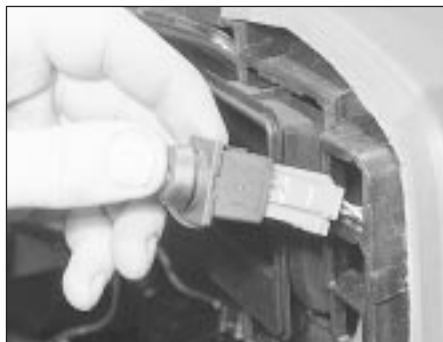
15.54 Removing a foglight switch
