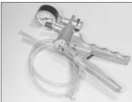
Vacuum pump and gauge
