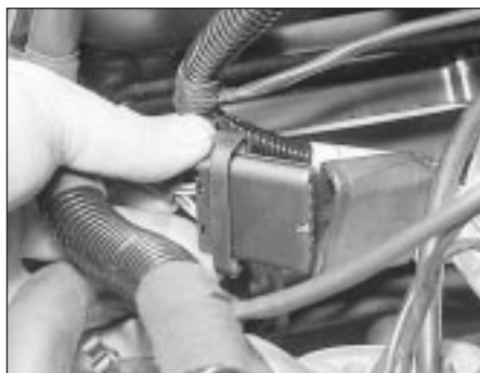
8.19a Disconnecting the distributor wiring plug
