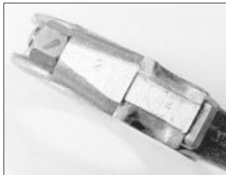
33.6b Connecting rod and cap carry cylinder numbers
