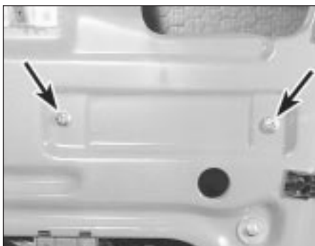
24.5a The two regulator slide screws (arrowed)
