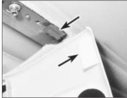
43.4b Slide the console rearwards to release the clips (arrowed)
