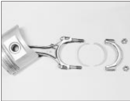
33.1 Piston, connecting rod and shells ready for assembly
