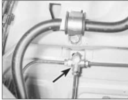
21.7 Brake pipe union T-piece (arrowed)
