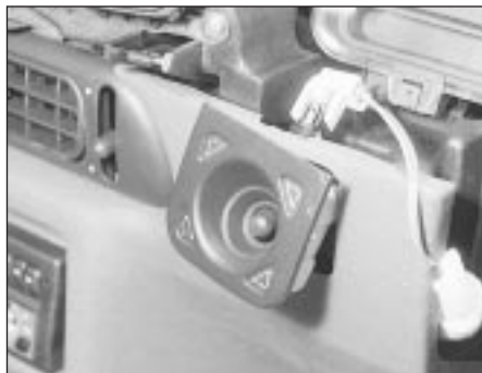
33.3 Removing the joystick fader
