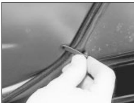
6.10 On refitting ensure the wiring and hoses are correctly routed and secured by all necessary retaining clips
