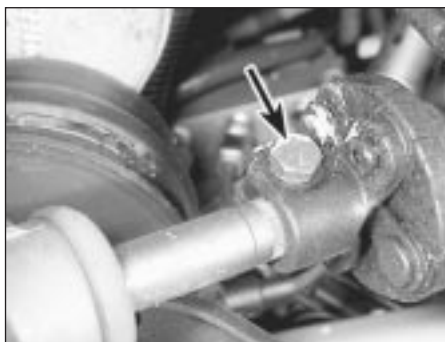
5.29 Intermediate shaft lower clamp bolt (arrowed)
