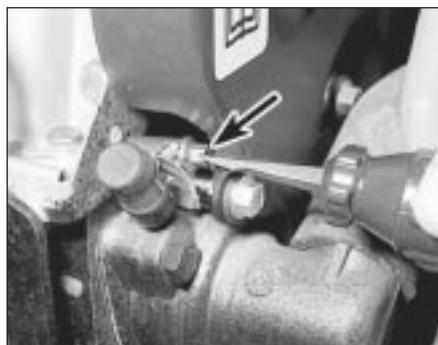
46.4b Releasing the bleed spigot cap - OHC engine
