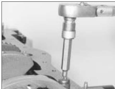
30.4 Unscrewing a sump mounting plate securing bolt
