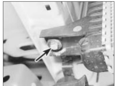
5.8 One of the radiator bottom mounting bolts (arrowed)
