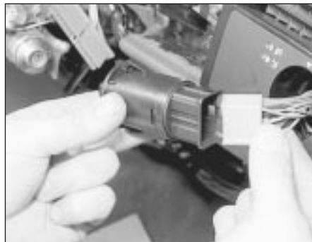
41.21 Withdraw the light switch and disconnect the wiring plug
