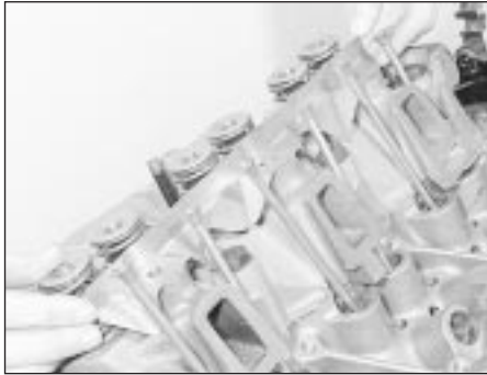
38.7a Fitting the pushrods and oil splash shields
