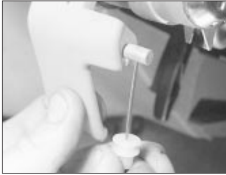
11.3 Unhooking the cable inner from the release lever
