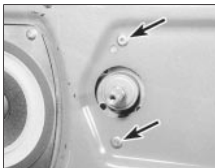
24.5b Two of the rivets (arrowed) which secure the regulator
