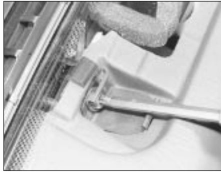
41.34b Facia upper mounting screw
