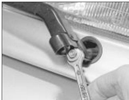
27.7 Removing a headlamp wiper arm
