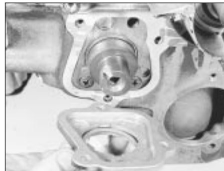
14.4 Removing the auxiliary shaft front cover
