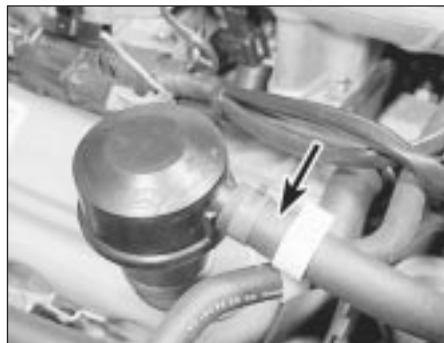
8.15 Oil filler breather hose (arrowed)
