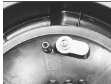
3.2b Air cleaner heat sensor
