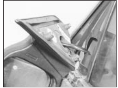
39.3 Removing a mirror from the door
