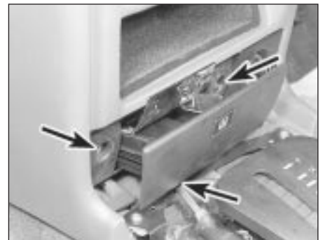
41.24 Ashtray retaining screw locations (arrowed)
