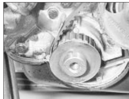
13.8 Remove the guide washer from in front of the crankshaft sprocket
