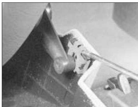
41.29a Lift the glovebox hinge retaining clips and disconnect the hinge arms
