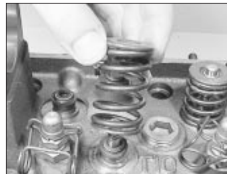
12.2b Removing a valve spring and cap
