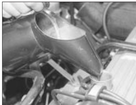
3.3 Topping up the engine oil
