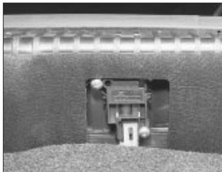
7.4b . . . on later models an access cover in the trim panel is provided
