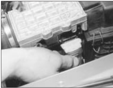
8.14a Front airflow sensor wiring plug
