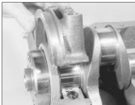
22.7 Removing the rear main bearing cap
