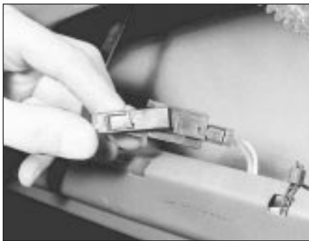
24.4 Window motor multi-plug
