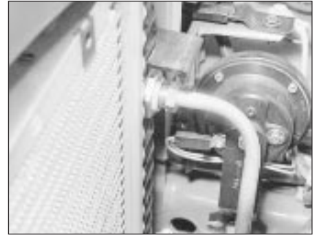
5.4 Transmission fluid cooler upper union
