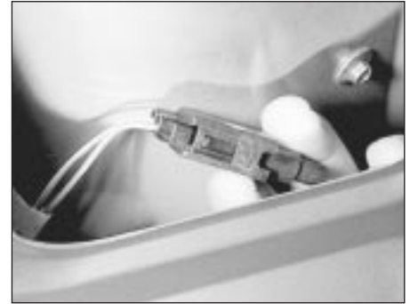
9.2 On Saloon models remove the trim panel to gain access to the lock and warning switch wiring connectors
