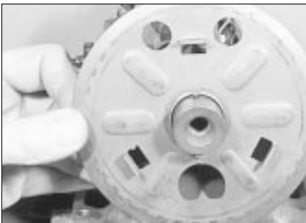
11.3 Removing the camshaft sprocket backplate
