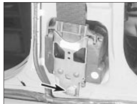
47.5 Seat belt retractor mechanism - securing the bolt arrowed
