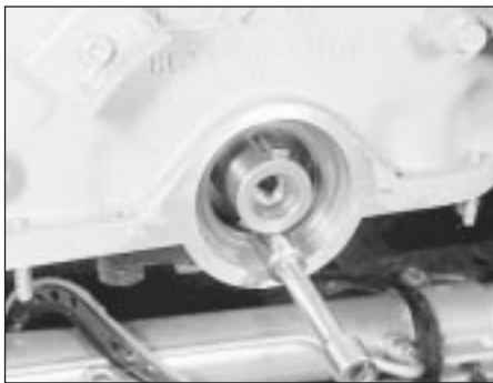
36.26b Using a socket to check the crankshaft to timing cover gap
