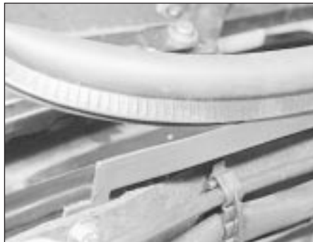
29.2 Pulling off the rubber sealing strip
