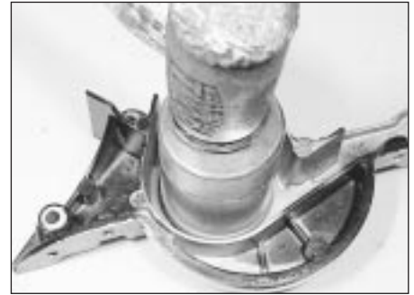
17.4 Using a socket and a hammer to seat the new seal
