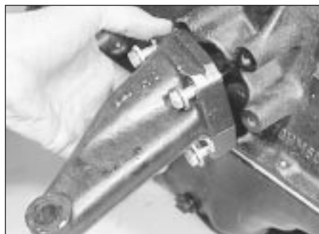
9.1b Removing an engine bearer arm
