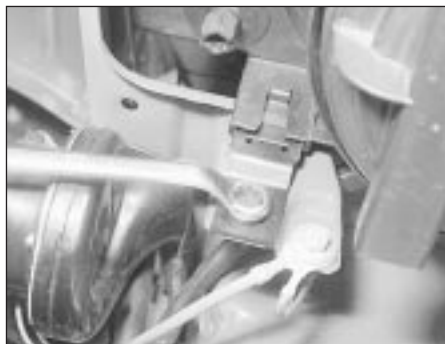
4.6b Headlight bottom mounting screw
