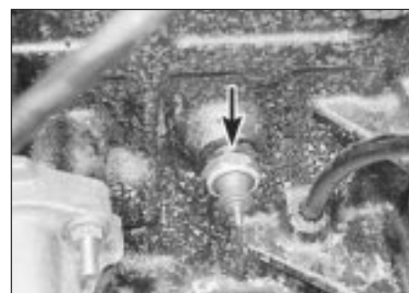
9.1a Engine oil pressure switch (arrowed)
