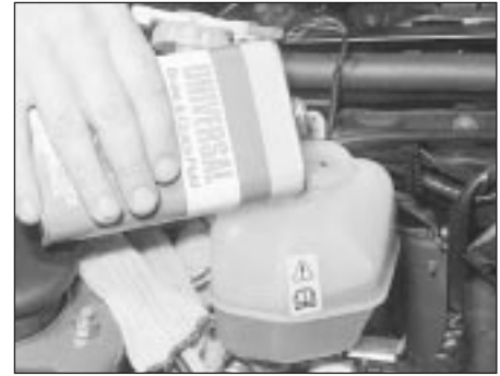
3.15 Topping up the brake fluid reservoir
