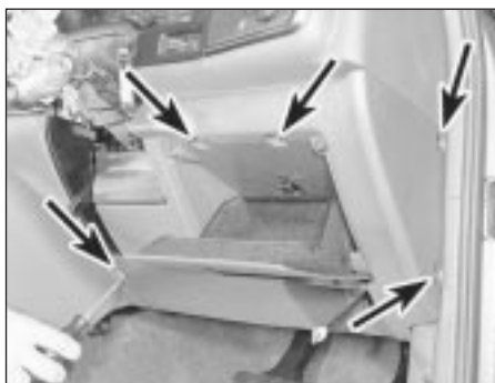
41.28 Undo the five right-hand lower fascia panel retaining screws (arrowed)
