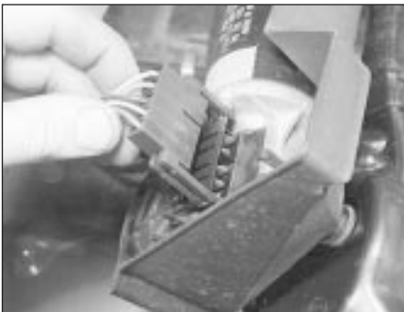
23.3 Disconnecting the wiper motor multi-plug
