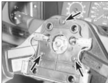
12.3 Three screws (arrowed) secure the horn switch plate
