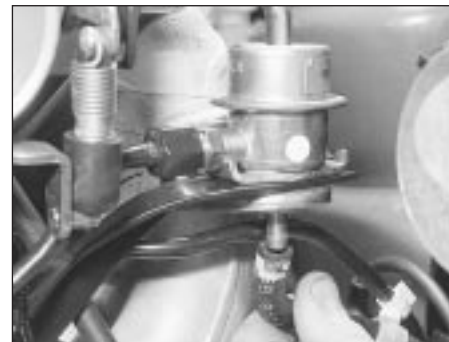
37.3 Disconnecting the fuel return pipe from the fuel pressure regulator
