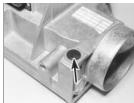
31.7 Tamperproof plug (arrowed) covering mixture adjusting screw
