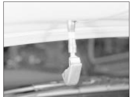
25.1 A windscreen washer jet prised out of its location in the bonnet
