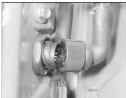
7.1 Door wiring multi-plug
