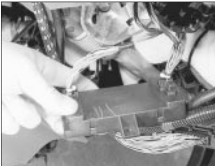
27.27 Removing the auxiliary warning system control module
