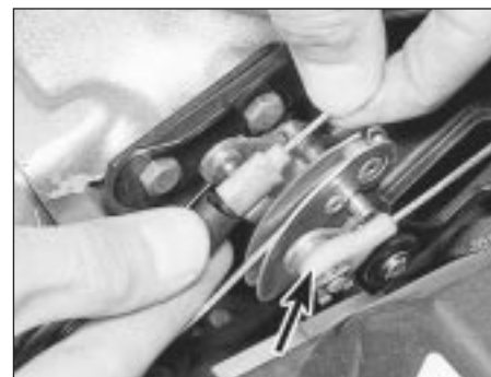
40.52 Disconnect the throttle cable from the linkage. Speed control cable (arrowed)
