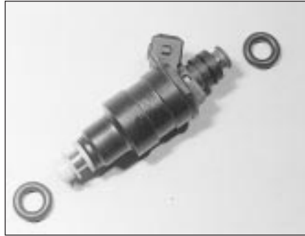
36.13 Injector with seals removed
