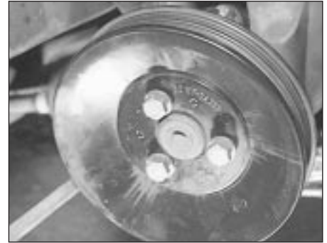
11.10 Unbolt the power steering pump pulley . . .
