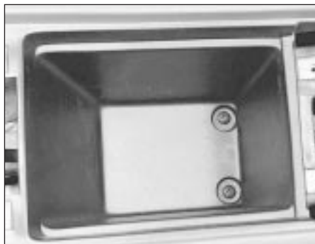
42.8 Cassette box, showing securing screws (high series)
