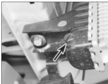
46.4a Radiator drain plug (arrowed) - OHC engine
