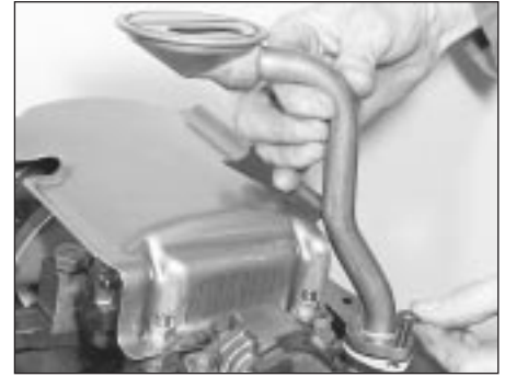
29.2 Removing the oil pick-up pipe
