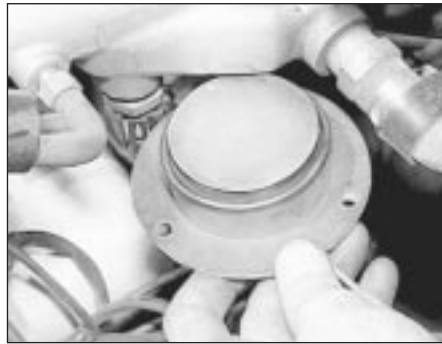
21.5 Removing the manifold heater
