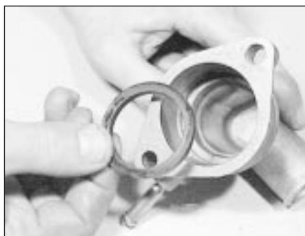
7.5c . . . and the sealing ring
