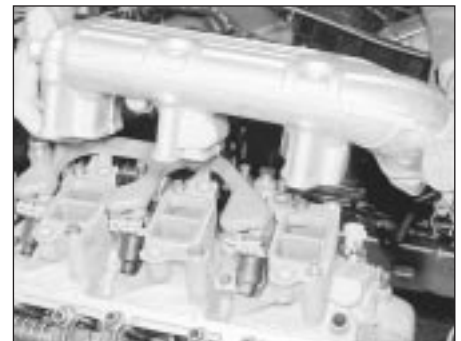
38.22 Lowering the plenum chamber into position
