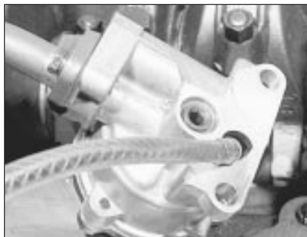
38.2 Priming the oil pump
