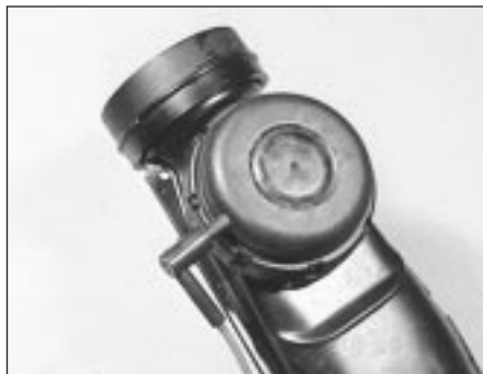
3.2a Air cleaner vacuum diaphragm unit
