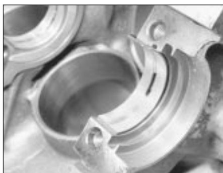
31.1 Rear main bearing shell in the crankcase
