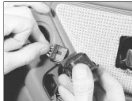
15.15 Removing a mirror control switch
