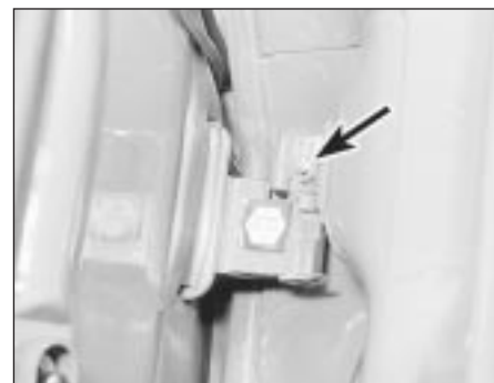
7.3 One of the hinge cotter pins (arrowed)
