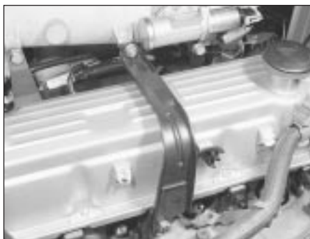
40.34 Inlet manifold-to-cylinder head bracing strut
