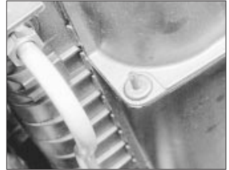
10.22a Radiator upper shroud plastic clip and centre pin
