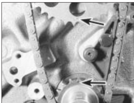
10.37 Timing sprocket alignment marks (arrowed)
