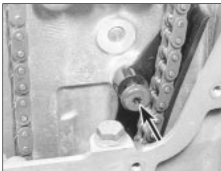
15.11a Lower timing chain guide upper securing bolt (arrowed)
