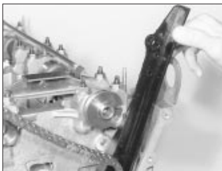
15.11c Withdrawing the lower timing chain guide
