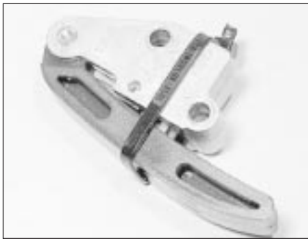
36.21 Timing chain tensioner retracted using a cable-tie
