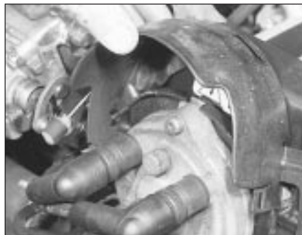
39.21b . . . and the upper section of the distributor shield - DOHC engine
