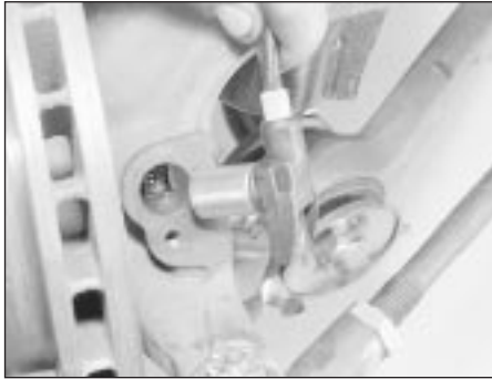
26.3 Removing a front sensor
