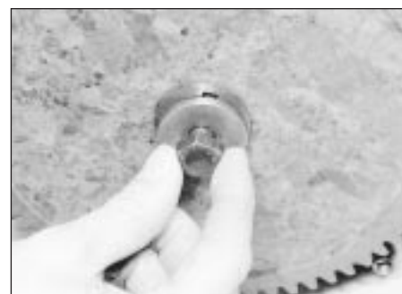
36.5 Camshaft gear washer and bolt
