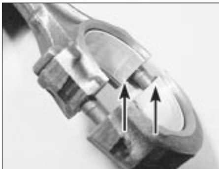
37.2 Big-end bearing shell lugs (arrowed) are adjacent
