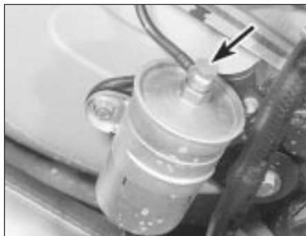
41.4 Fuel filter outlet union (arrowed) - OHC engine
