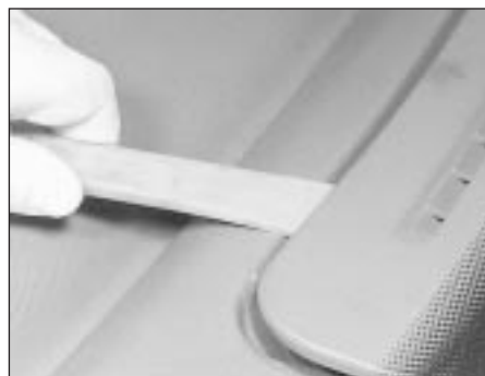
41.33 Removing the windscreen vent panel (viewed through the windscreen)
