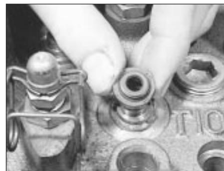
12.4 Removing a valve stem oil seal
