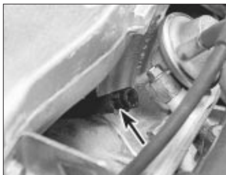
37.13 Disconnect the fuel return hose (arrowed) from the fuel pressure regulator
