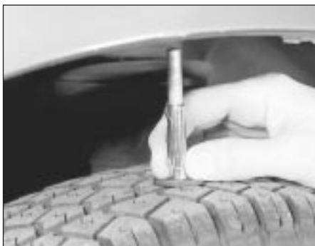
4.1 Checking the tyre tread depth
