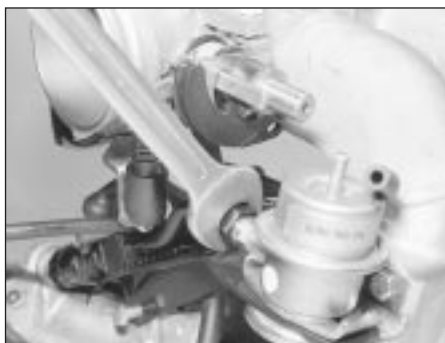
37.5 Slackening the fuel pressure regulator feed union nut
