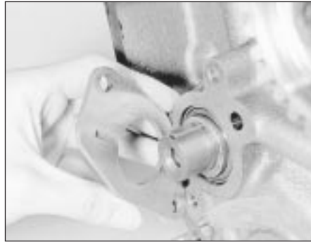
32.3b Fitting the camshaft thrust plate
