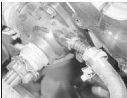
7.12a Disconnecting the coolant hoses . . .
