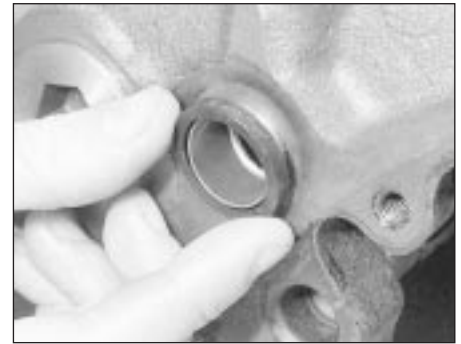
32.4 Timing cover dowel and seal
