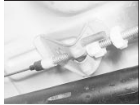
22.3 Handbrake cable adjuster Locknut previously backed off adjuster nut
