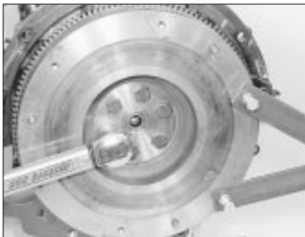
22.1 Improvised tool used to hold flywheel when tightening securing bolts
