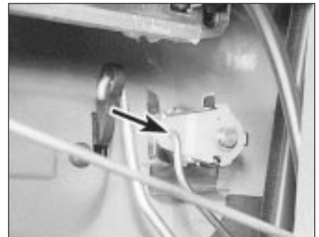
14.2 Unhook the operating rod (arrowed) from the lock barrel lever
