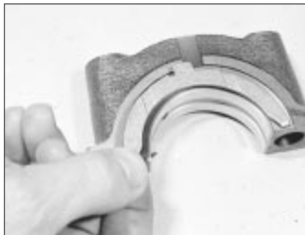
36.14 Fitting a thrust washer to the centre main bearing cap
