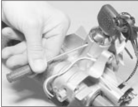
8.3 Depress the column lock locking button
