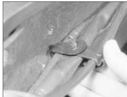
29.3 Pulling out a wiring harness clip
