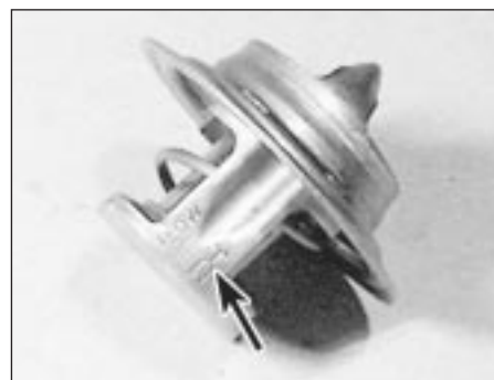
7.7 Thermostat direction of flow arrow
