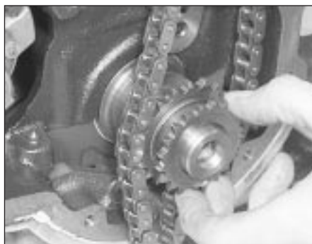
15.12 Sliding the double chain sprocket from the end of the crankshaft
