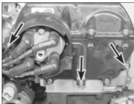
18.53 Upper timing chain cover securing stud locations (arrowed)
