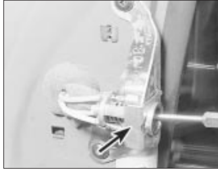
39.1b Pull out the clip (arrowed) to release the mirror control
