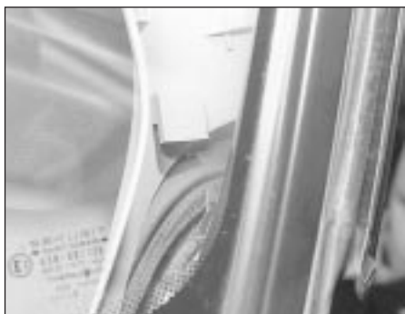
41.31b . . . and lower locating tab (viewed through windscreen)
