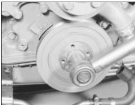
10.27a Unscrewing the vibration damper centre bolt
