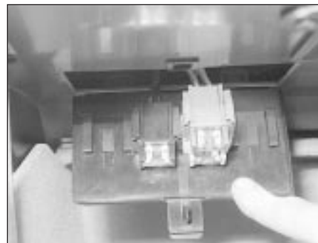
16.3 Auxiliary fuse box in the glovebox
