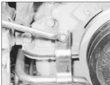
10.30 Coolant distribution pipe bracket
