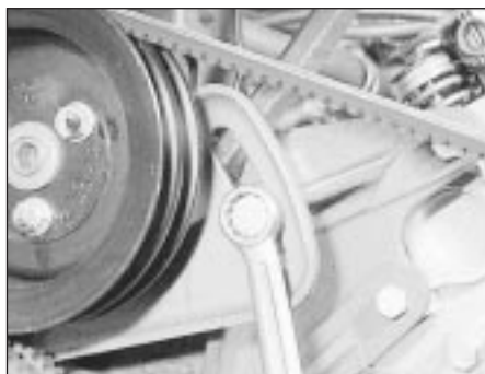
36.39b Power steering pump drivebelt tensioner bolt
