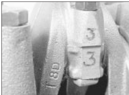
21.2 Big-end cap and connecting rod identification numbers
