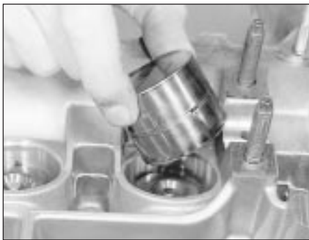
18.15 Withdrawing a cam follower
