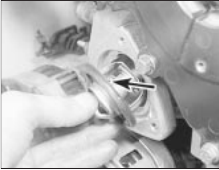
7.16 Thermostat relief valve (arrowed) positioned in the 12 o'clock position
