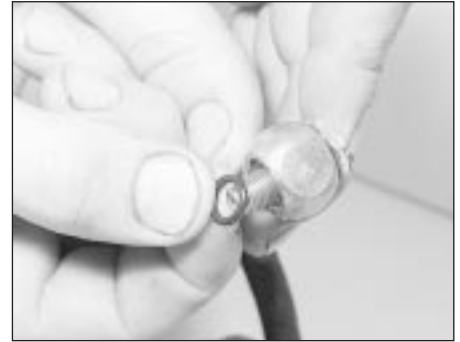
20.9 Fitting new sealing washers to a banjo union
