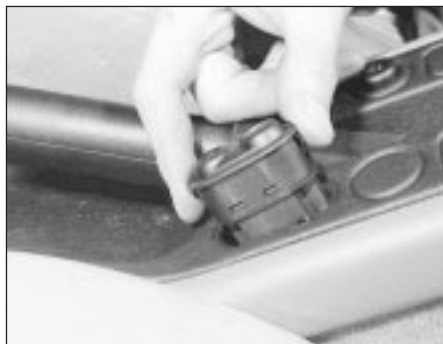
15.31 Removing a window operating switch
