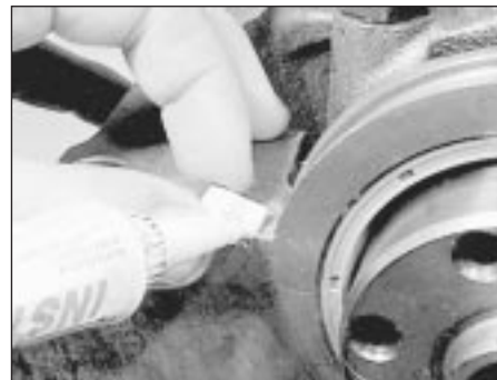
36.19 Fitting a sealing wedge to the rear main bearing cap
