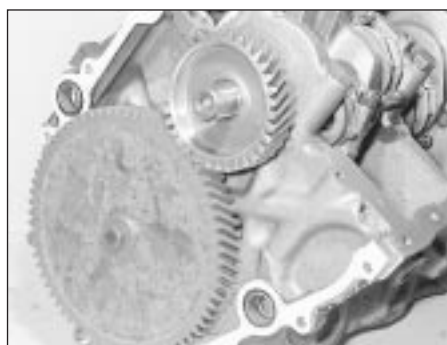
36.7a Timing cover gasket in position
