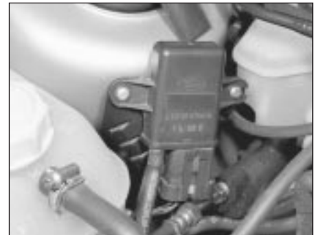
28.1 Manifold Absolute Pressure (MAP) sensor location - models equipped with a catalytic converter
