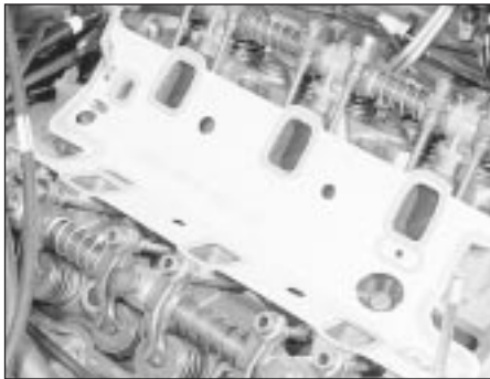
38.18a Inlet manifold gasket correctly located
