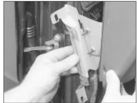
41.35b . . . then undo the screws and remove the bracket from behind the facia
