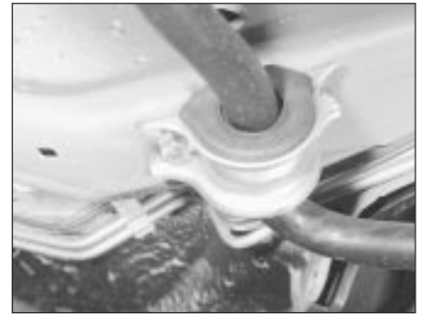
19.2 A front anti-roll bar clamp
