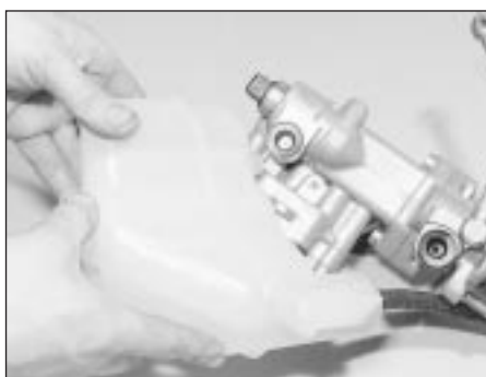
16.6 Removing the hydraulic fluid reservoir
