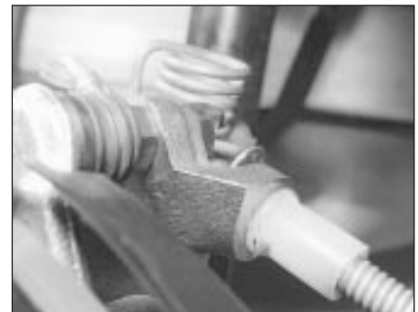
23.4 Handbrake cable outer attached to caliper bracket
