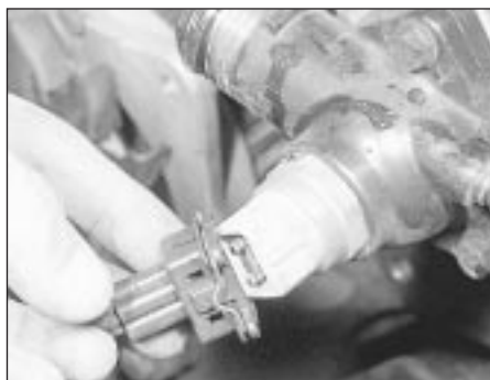
7.13 Disconnect the cooling fan switch wiring plug . . .
