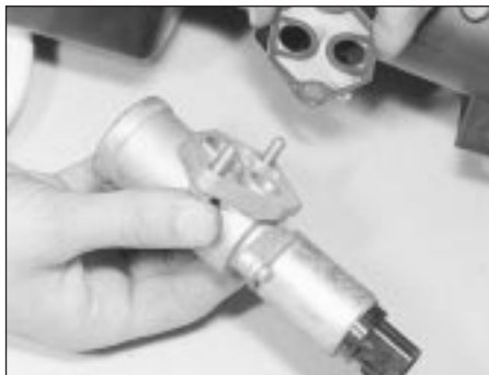
34.12 Withdrawing the idle speed control valve
