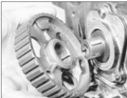
13.11 Removing the auxiliary shaft sprocket
