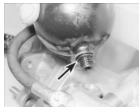
17.4 Removing the accumulator Note O-ring (arrowed)
