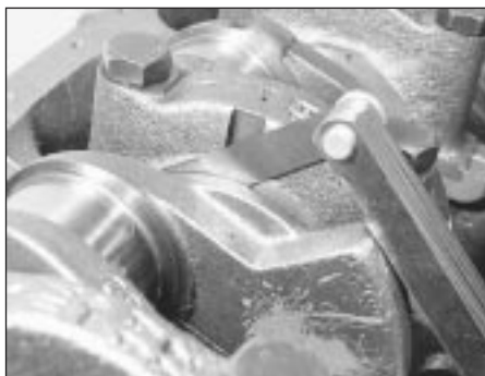
22.6 Checking crankshaft endfloat
