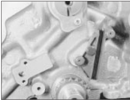
36.15 Crankshaft and camshaft key and slot alignment
