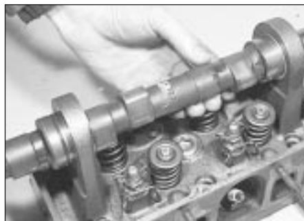
11.8 Removing the camshaft
