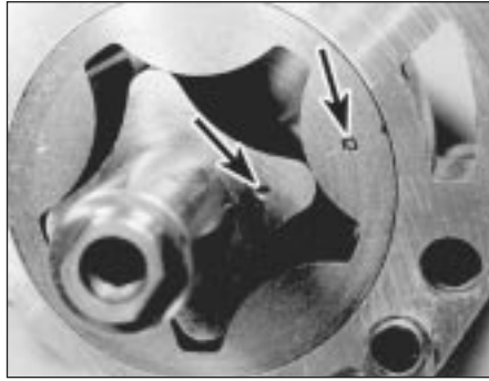
27.9 The punch marks (arrowed) on the oil pump rotors must face the pump cover
