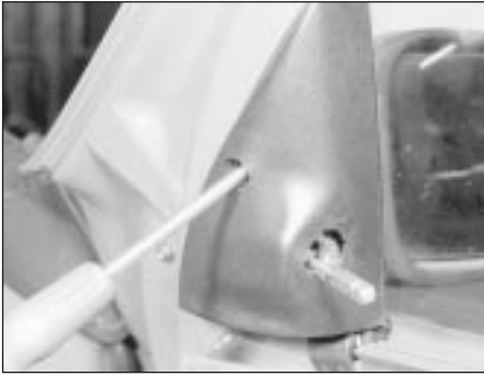
39.1a Removing the mirror mounting trim screw
