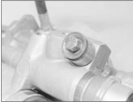
18.5 Hydraulic unit pump mounting bolt
