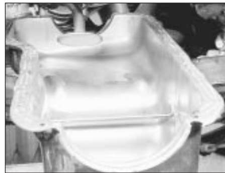
16.12 Removing the sump
