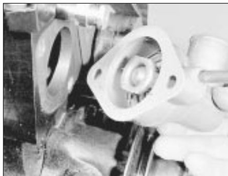
7.4 Removing the thermostat housing
