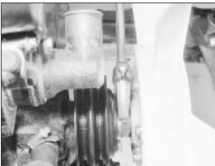
9.3b Undoing the viscous fan clutch nut
