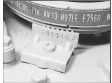
13.20 Crankshaft pulley notch set to the 12° BTDC position
