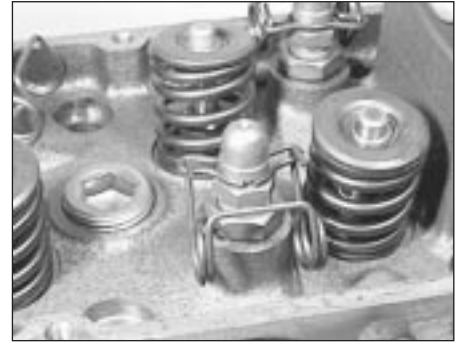
42.3 Cam follower ball-pins and spring clips fitted
