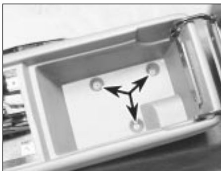
42.20a Centre console rear retaining screws (arrowed)
