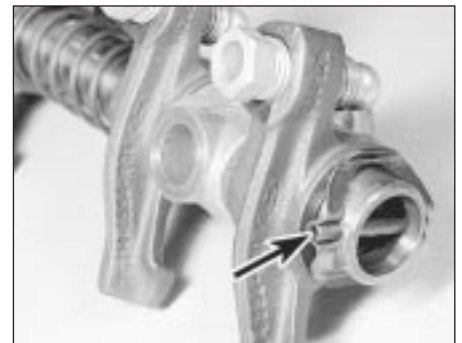
20.1 Rocker shaft roll pin (arrowed)
