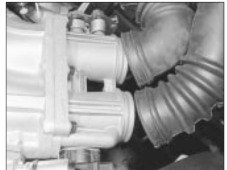
8.13 Disconnecting the air hoses from the throttle valve housing
