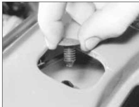
5.7 Pull out the plug to release the radiator top mounting
