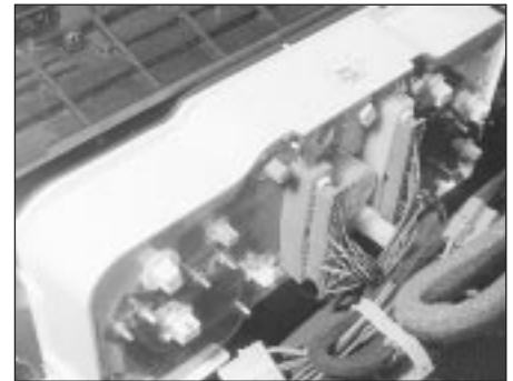
7.4a Instrument cluster viewed through windscreen to show multi-plugs
