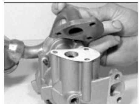
27.16a Removing the pick-up from the oil pump
