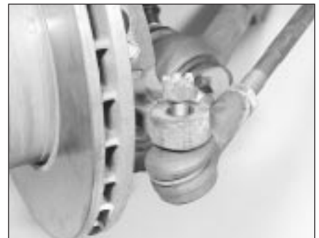
13.3 Track rod end balljoint nut unscrewed
