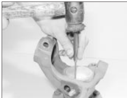
17.17 Seating the new dust cap
