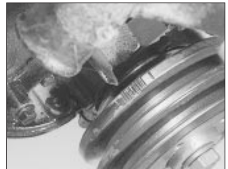
14.3a Timing marks and pointer Cast pulley shown
