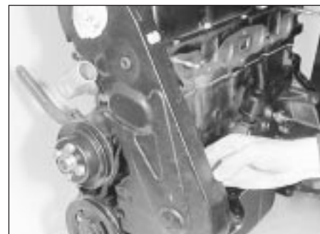
10.2 Removing the timing cover
