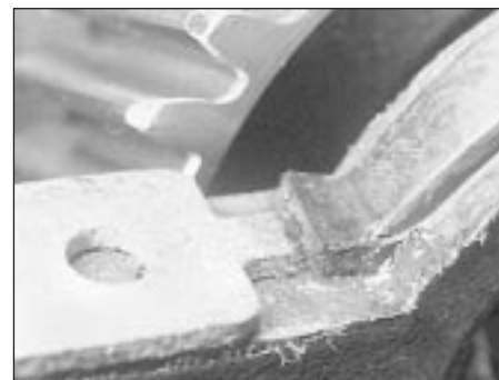
37.3 Slide the sump gasket tab into the seal cut-out
