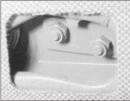
8.6 Tailgate hinge nuts are accessible through headlining
