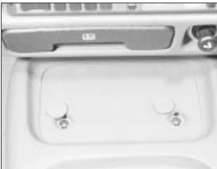
42.1 The two front screws which secure the low series console
