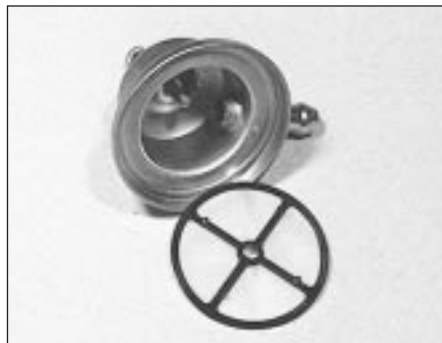
4.8b Fuel pump cover and filter screen
