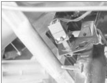
15.43 Stop-light switch fitted to brake pedal bracket
