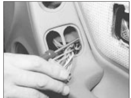
22.4b Access to the screw is through the window switch aperture
