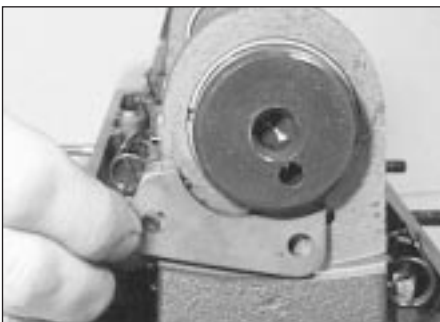
11.7 Removing the camshaft thrust plate
