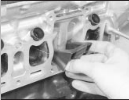
40.59 Removing a spark plug spacer from the cylinder head recess
