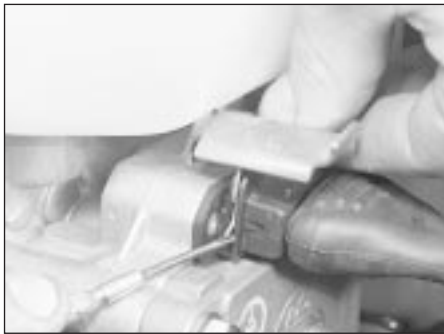
15.3a Disconnect the valve block multi-plug. Lift the clip and pull off the plug
