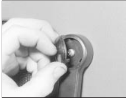
22.3 Prise the cap off the window winder handle to expose the screw
