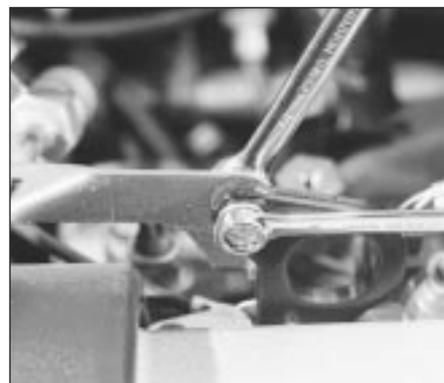
4.9B . . . unbolt the power steering high-pressure pipe . . .
