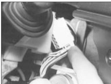
4.7 Disconnecting the multi-plug from the windscreen wiper multi-function switch
