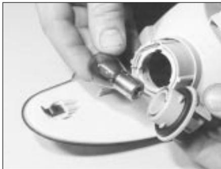
5.15 Removing the front direction indicator bulb
