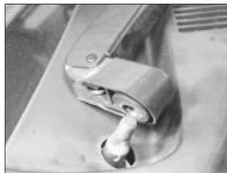
15.5 Removing the wiper arm from the spindle
