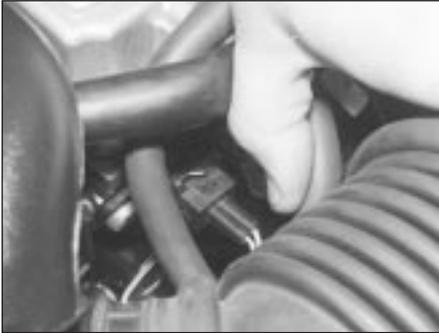
4.45 Camshaft position sensor is located at left-hand rear end of cylinder head
