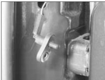
4.57B . . . and pull out the courtesy light switch
