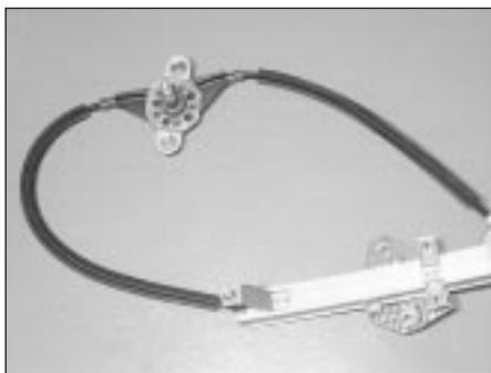
13.6D Rear door window regulator removed from the vehicle
