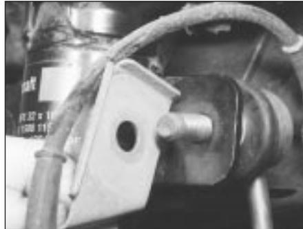
4.7 Removing the anti-roll bar link and ABS sensor wiring bracket
