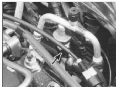
**12.33** Unplug pressure-regulating switch electrical connector (arrowed)
