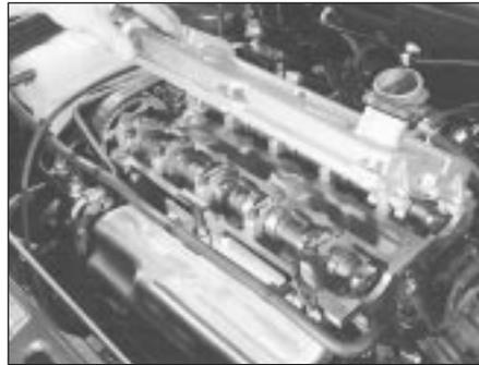
5.6 Removing cylinder head cover
