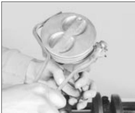
12.4A The piston ring grooves can be cleaned with a special tool, as shown here . . .
