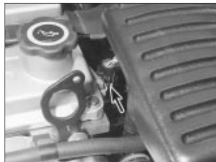
6.15 Location (arrowed) of coolant temperature sensor
