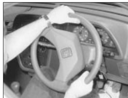
movement of the steering wheel, indicating wear in the column support bearings or couplings.
