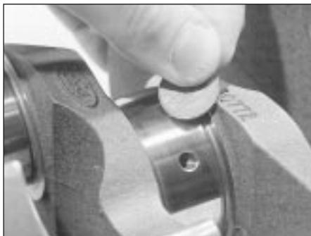
**13.3** Rubbing a penny lengthwise along each journal will reveal its condition - if copper rubs off and is embedded in the crankshaft, the journals should be reground
