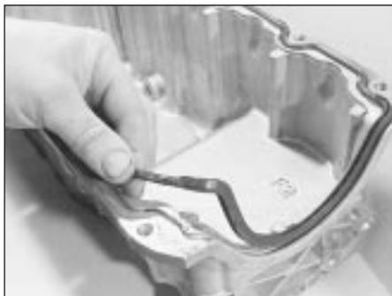
15.17 Ensure gasket is located correctly in sump groove
