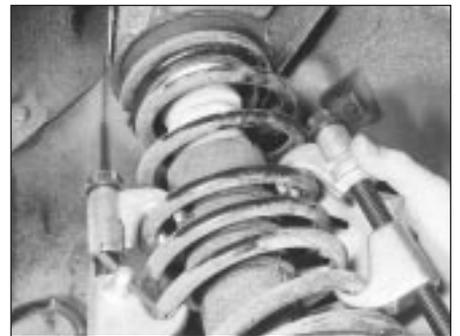
11.14 Removing the rear suspension strut
