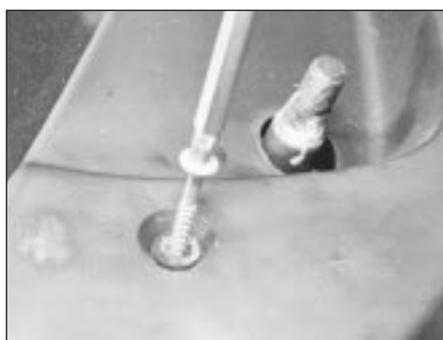
16.3B . . . and remove the upper retaining screws
