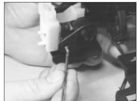
14.10 Pulling out the handle connecting rods
