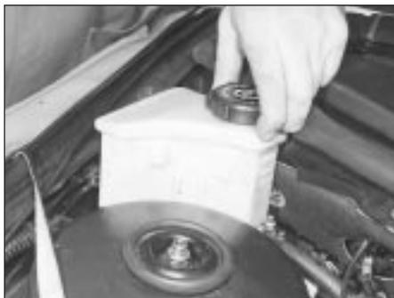
4.36A Unclip and lift power steering fluid reservoir - take care not to spill fluid . . .
