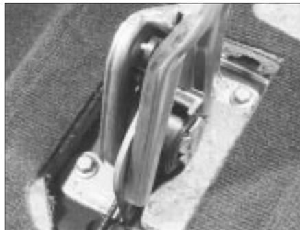
**26.6** Handbrake lever mounting bolts
