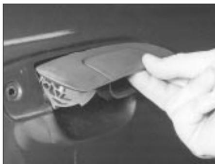
14.16 Removing the rear door exterior handle
