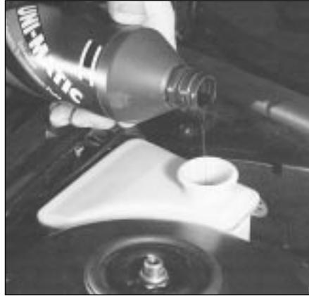
5.6 Topping-up the power steering fluid reservoir
