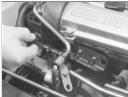
14.18A Remove cylinder head front . . .
