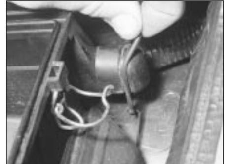
4.4 Remove rubber retaining band to withdraw air cleaner assembly
