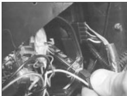
5.2B . . . and withdraw the headlight bulb
