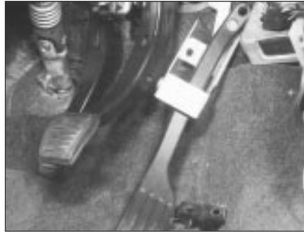
7.2 Removing the accelerator pedal assembly
