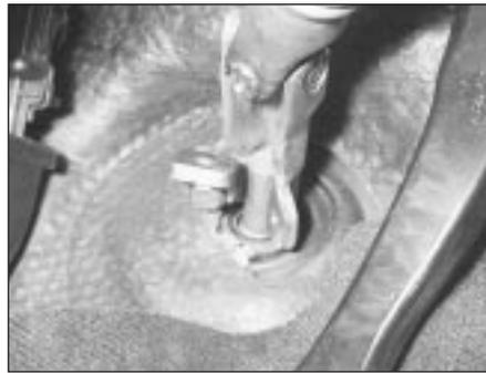
28.6B . . . and swivel the clamp plate around
