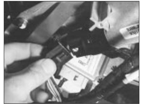
28.7A Disconnecting the multi-plug from the ignition switch
