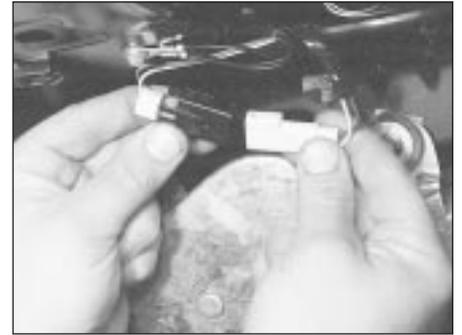
17.4 Disconnecting the tailgate wiper motor multi-plug
