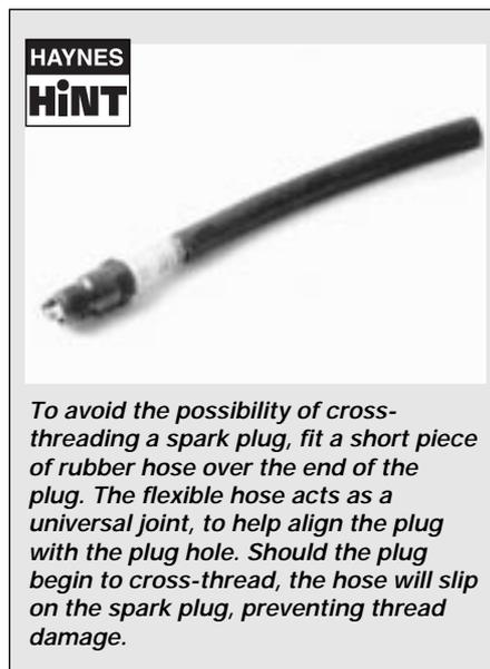
**To avoid the possibility of cross-threading a spark plug, fit a short piece of rubber hose over the end of the plug. The flexible hose acts as a universal joint, to help align the plug with the plug hole. Should the plug begin to cross-thread, the hose will slip on the spark plug, preventing thread damage.**
