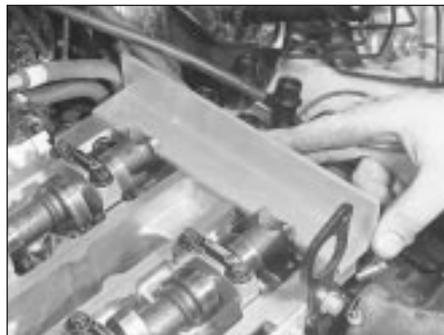
10.10 Fit camshaft aligning tool to ensure engine is locked with Nos 1 and 4 cylinders at TDC
