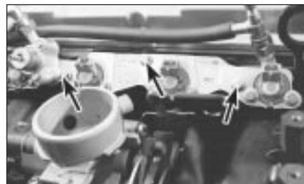
16.19A Unscrew bolts (arrowed) . . .
