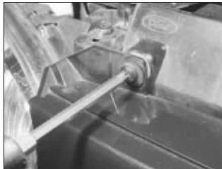
7.2 Removing a radiator grille mounting screw
