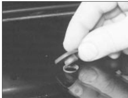
**22.12B . . . and prise out the rubber grommet**
