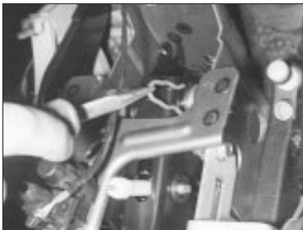
12.3 Removing the hairpin clip from the right-hand end of the brake pedal pivot shaft
