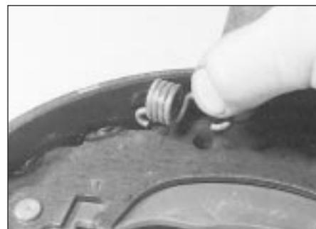
6.2M . . . and remove the small spring
