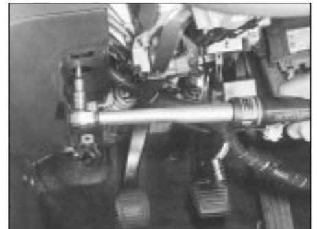
28.13 Tightening the steering column mounting bolts
