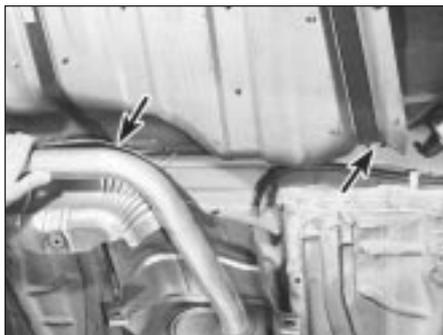
**10.8 Exhaust system must be lowered and heat shield removed to enable fuel tank removal - arrows show location of retaining strap front bolts**
