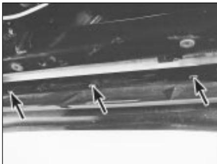
**28.11** Ensure radiator undershield is located securely in three clips at front edge (arrowed) when refitting
