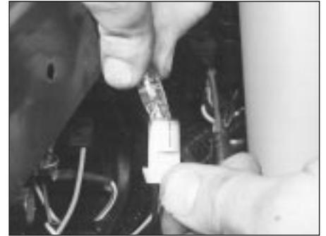
5.10 Pulling the wedge-type bulb from the bulbholder
