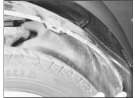
34.4 Removing a front wheel arch liner
