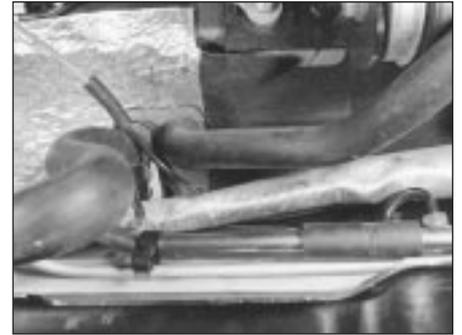
9.9A Coolant pipes to heater matrix must be disconnected . . .
