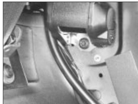
28.7B Rear seat belt reel mounting bolt
