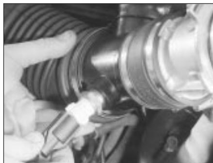
4.7 Unplugging intake air temperature sensor's electrical connector
