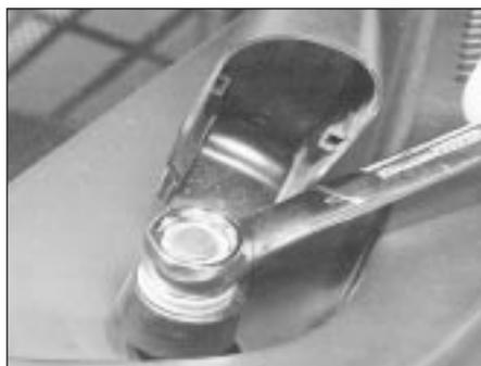
15.3 Loosening the wiper arm retaining nut
