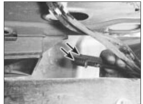
5.16 . . . unplug hoses (arrowed) from canister assembly . . .
