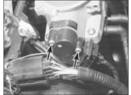
4.53 Throttle potentiometer is secured by two screws (arrowed)
