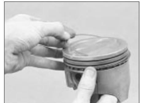
16.7A Installing the spacer/expander in the oil control ring groove
