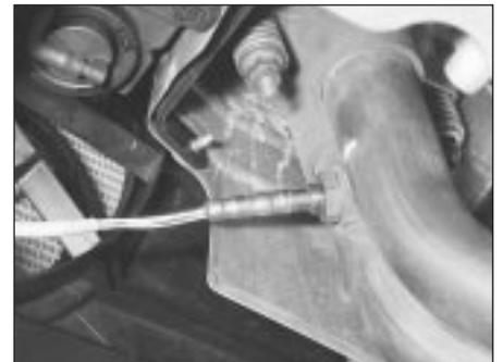
4.62 Oxygen sensor is screwed into pipe at right-hand rear end of exhaust system front downpipe . . .
