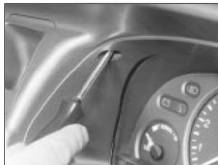
10.8A With the blanking covers removed, unscrew the concealed screws . . .
