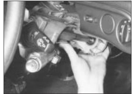
28.8B Removing the steering column
