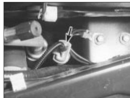
12.23 Unplug pressure-cycling switch electrical connector (arrowed)
