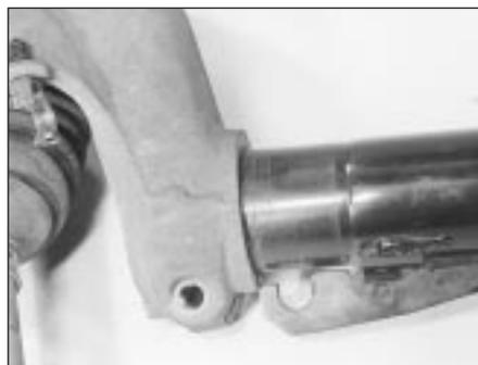
4.12B Releasing the knuckle from the strut
