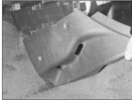
33.3B . . . and remove the heater side covers
