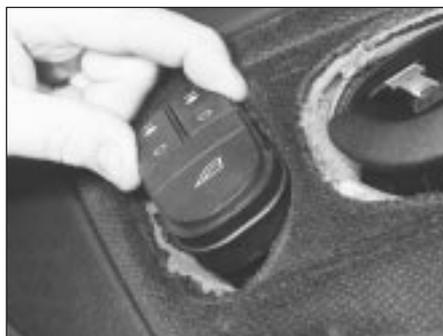
11.3A Remove the window operating switch . . .
