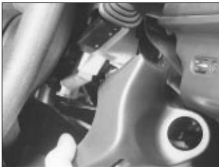
28.4C . . . and remove the lower shroud
