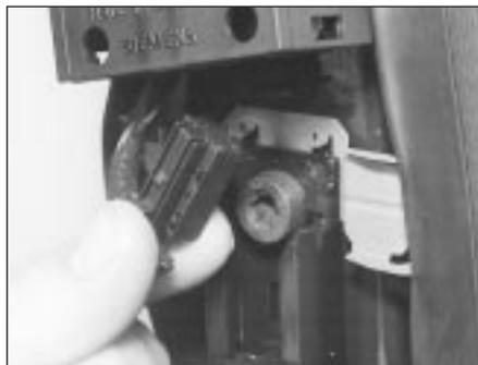
**20.3A Disconnecting a movement sensor multi-plug**
