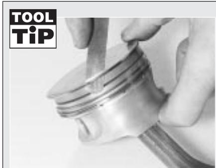
**If a piston ring removal tool is not available, the rings can be removed by hand, expanding them over the top of the pistons. The use of two or three old feeler blades will be helpful in preventing the rings dropping into empty grooves.**
