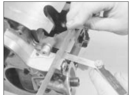
16.13 Check the oil pump is positioned correctly
