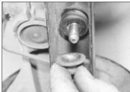
13.2B . . . remove the nut and rubber bush . . .
