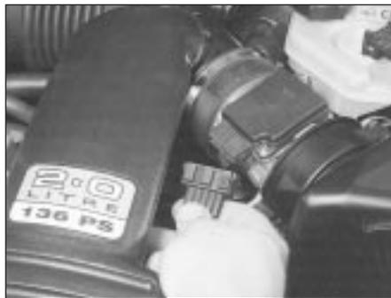
4.40 Unplugging the air mass meter's electrical connector . . .
