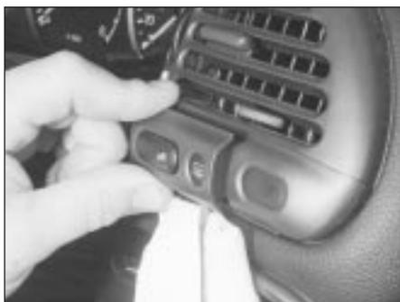
4.49 Prising out the heated rear window switch
