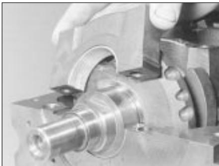
**17.7 Refit** the main bearing caps and tighten the bolts as specified
