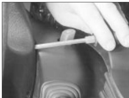
28.3 Unscrewing an air bag mounting bolt
