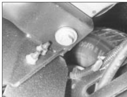
26.7B Rear suspension crossmember front mounting bolt
