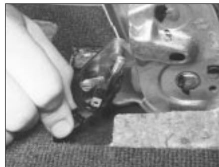
4.44 Disconnecting the multi-plug from the handbrake lever
