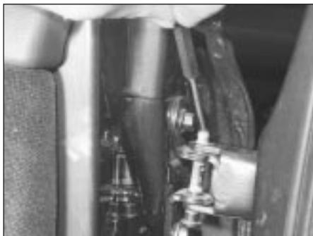
15.5A . . . then drive out the hinge pins . . .
