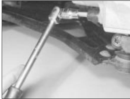
2.3C Using a 7 mm Allen key, unscrew . . .
