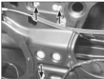
13.2C Window regulator mounting bolts - arrowed (rear door)
