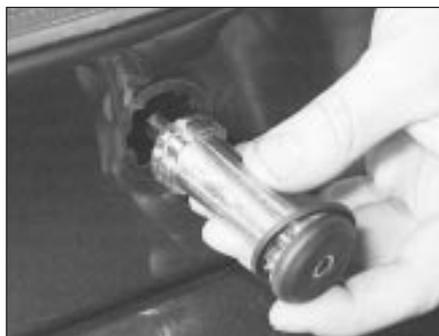
22.8A Removing the lock barrel . . .
