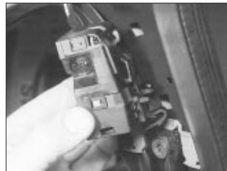
**20.3B Removing a movement sensor**
