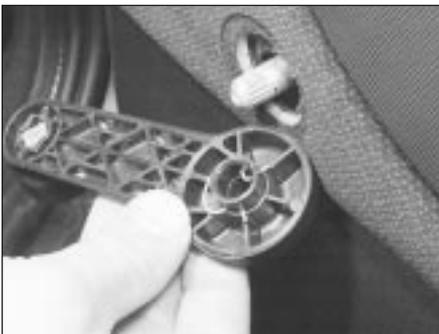
11.7B Withdrawing the window regulator handle
