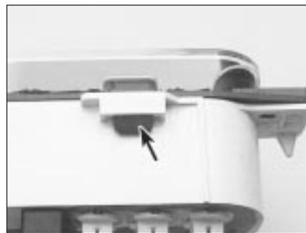
11.2 Bezel retaining lug on the instrument panel
