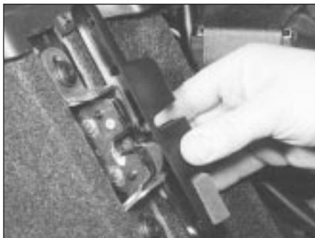
28.6B Removing the plastic cover from the rear seat lock
