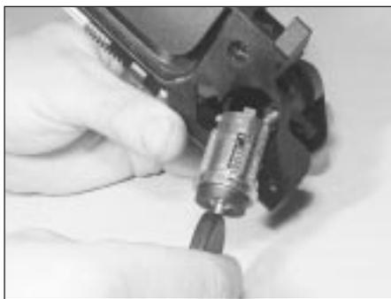
14.25 . . . and pull out the lock barrel
