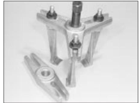
Three-legged hub and bearing puller
