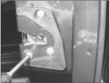
14.4A Unscrew the lock mounting bolts . . .
