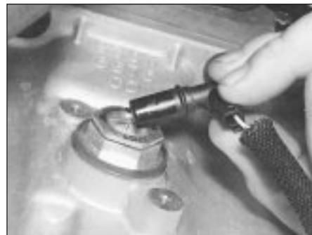
18.4 . . . disconnecting wiring from sensor
