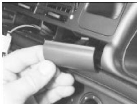
10.7 Removing a switch blanking cover
