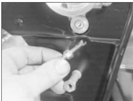
**10.19A** Fitting tensioner spring retaining pin
