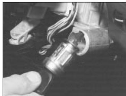
4.3B . . . and withdraw the ignition lock barrel
