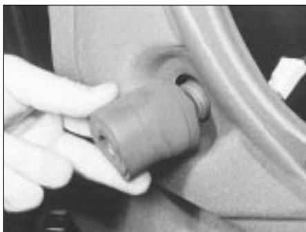
11.10 Removing the foam spacer
