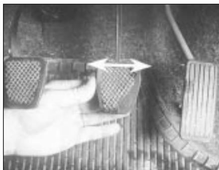
Check that the brake pedal is secure and in good condition. Check also for signs of fluid leaks on the pedal, floor or carpets, which would indicate failed seals in the brake master cylinder.
