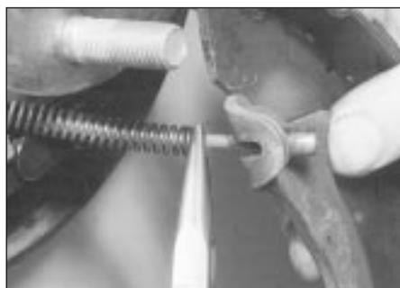
6.2K Pull the handbrake cable spring back from the operating lever on the rear of the trailing shoe. Unhook the cable end from the cut-out in the lever, and remove the shoe
