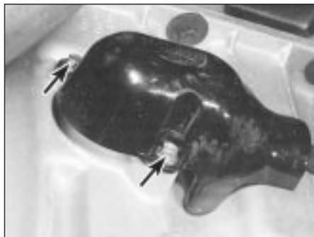
18.3 Remove screws (arrowed) to remove oil level sensor cover . . .
