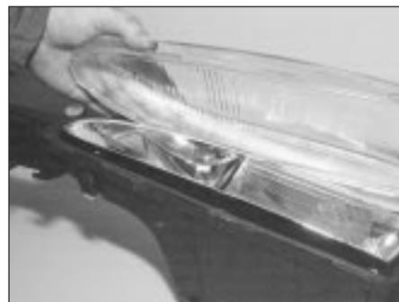
7.9B . . . and remove the headlight lens
