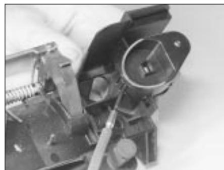
14.24 Prise out the barrel retaining tab . . .
