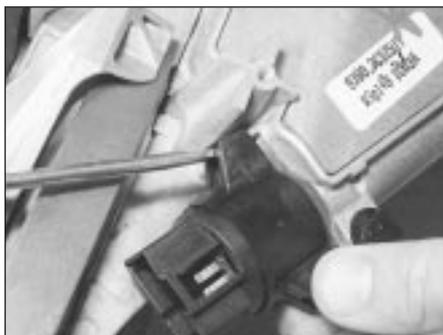
4.4A Release the retaining tab . . .
