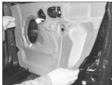
11.12 Removing the foam insulation
