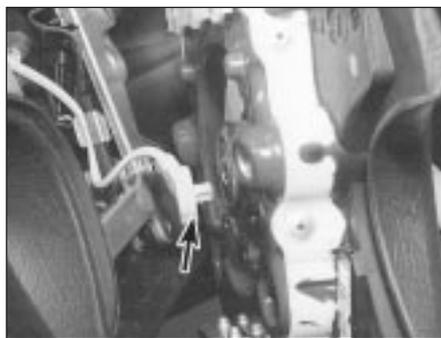
28.4 Disconnecting the air bag wiring multi-plug (arrowed)
