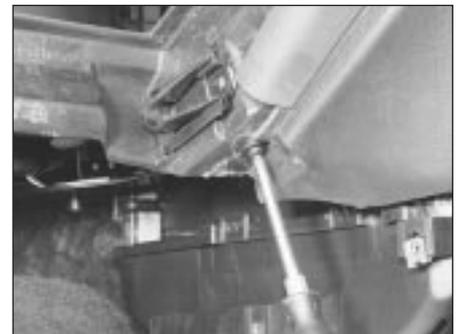
33.20D Facia mounting bolt near the heater
