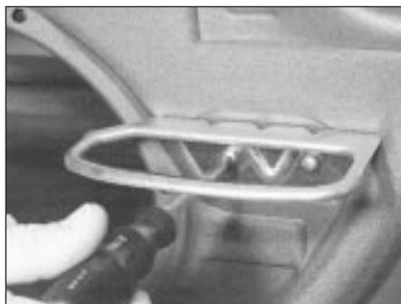
11.11 Removing the door pull bracket from a rear door
