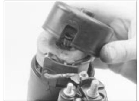
17.2C . . . and withdraw the end housing . . .
