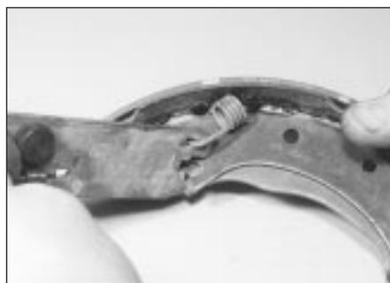
6.2L Unhook the automatic adjustment strut from the trailing brake shoe . . .
