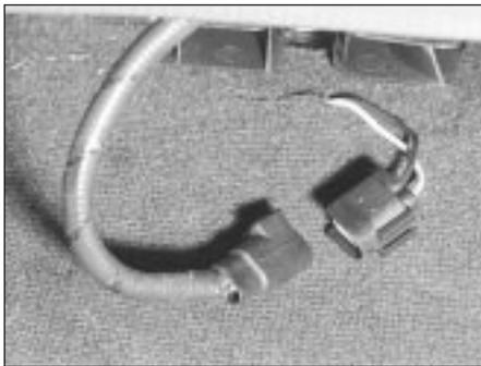
27.4 Disconnecting an electric seat multi-plug
