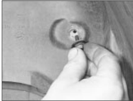
34.3 Removing a wheel arch liner retaining screw
