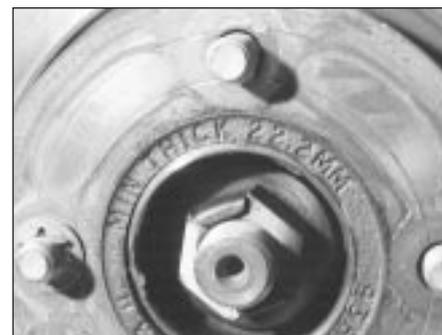
4.4B Disc minimum thickness marking
