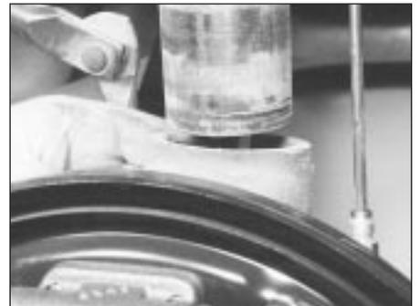
11.11 Separating the knuckle from the strut
