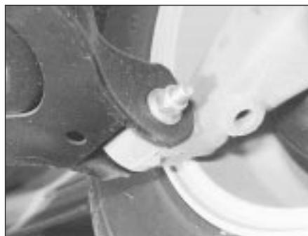
21.5 Rear lower arm-to-knuckle mounting bolt
