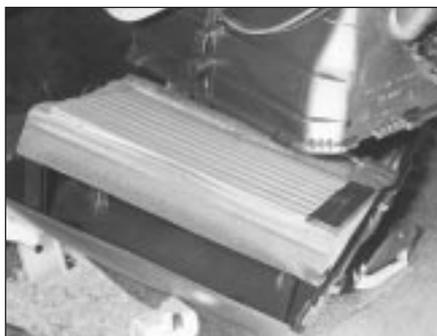
9.13 . . . heater unit's bottom cover, complete with matrix
