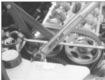
**10.25** Using forked holding tool while camshaft toothed pulley bolt is tightened
