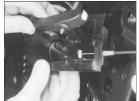
14.7A Removing the inner handle
