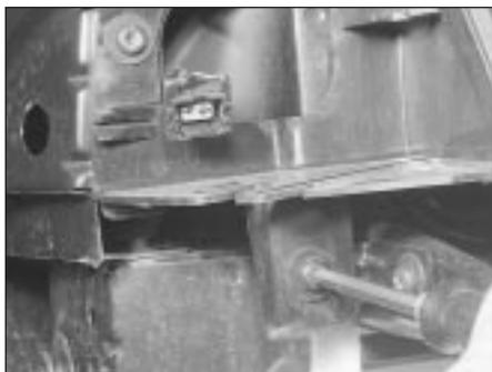
7.8A Unscrew the outer mounting screws . . .
