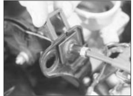
5.3 Removing clip securing accelerator cable to throttle housing bracket
