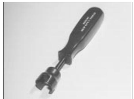
Brake shoe steady spring cup removal tool
