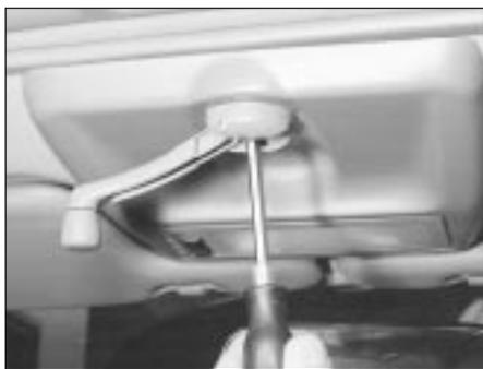
31.3 Removing the sunroof handle securing screw
