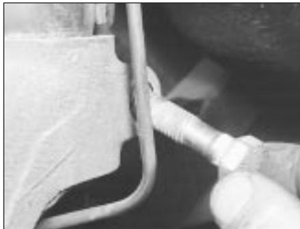
11.10B . . . and remove the knuckle-to-strut clamp bolt
