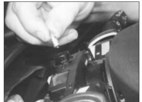
6.16B . . . and remove the bulb
