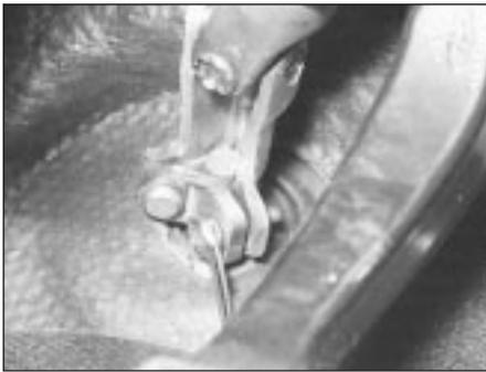
28.6A Unscrew the clamp plate bolt . . .
