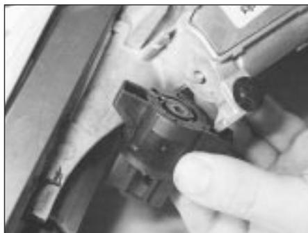
4.4B . . . and remove the ignition switch
