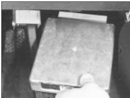
4.38 . . . then lift ECU to disengage it, and withdraw it
