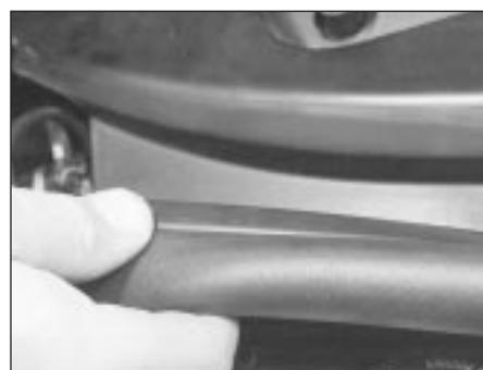
16.5 Removing the bonnet sealing strip
