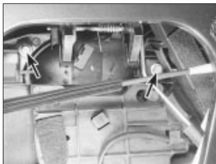
14.3A Remove the two bolts (arrowed) . . .
