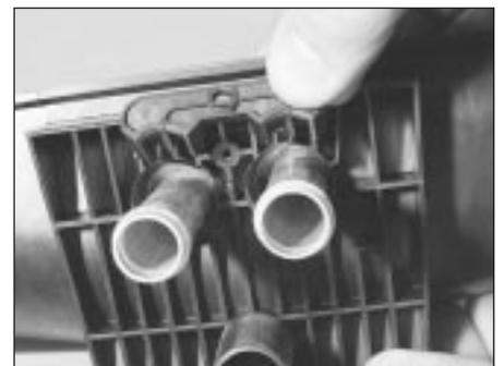
9.14 Remove clamp (one screw) to separate matrix from heater unit's bottom cover
