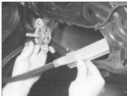
13.6C Removing the window regulator mechanism from the rear door
