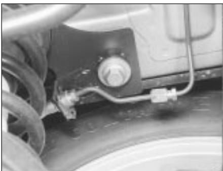
26.7A Rear suspension crossmember rear mounting bolt
