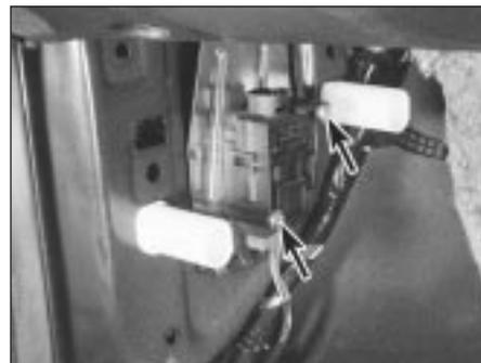
**13.3 Fuel cut-off switch retaining screws (arrowed)**
