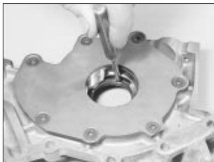
20.2 Driving out crankshaft right-hand oil seal
