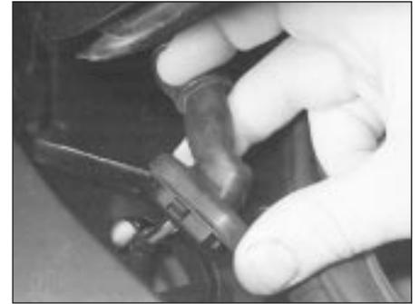
20.7 Removing the wiring loom rubber grommet
