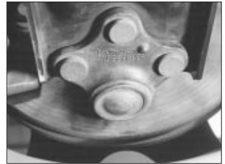
8.0 Original riveted front suspension lower arm balljoint
