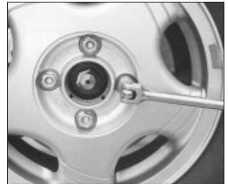
Slacken roadwheel nuts in diagonal sequence
