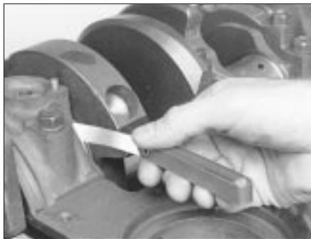
**10.3** Checking crankshaft endfloat with a feeler gauge
