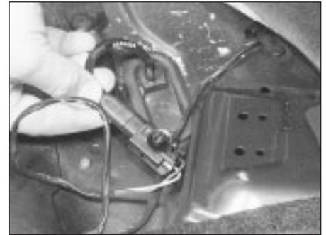
**21.12 Rear ABS sensor wiring multi-plug located beneath the rear seat**
