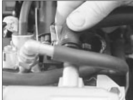
4.3 Disconnecting the crankcase breather hose from the cylinder head union
