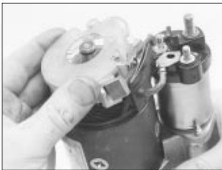
17.2G . . . lift off the plastic insulating plate . . .
