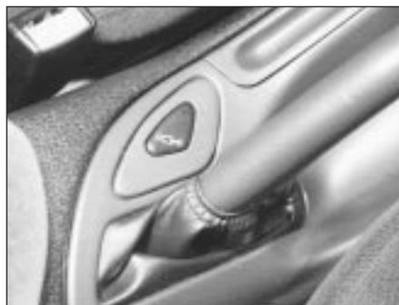
1.6A Adaptive damping switch located near the handbrake lever
