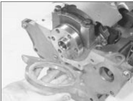
**20.15** Use new gasket when refitting left-hand oil seal carrier
