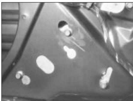
13.2B Electric window motor mounting bolts (front door)
