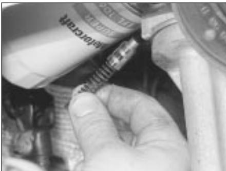
16.9B . . . to withdraw oil pressure relief valve spring and plunger
