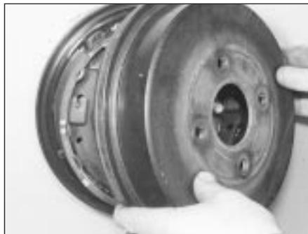
5.2B Removing a rear brake drum
