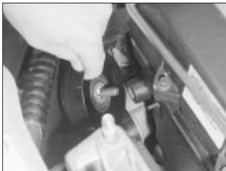
14.17 Unbolt auxiliary drivebelt idler pulley
