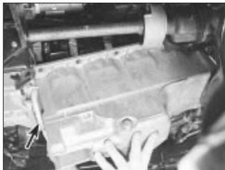
15.18 Engine/transmission lower adaptor plate (arrowed) must be refitted with sump
