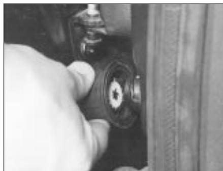
15.3 Disconnecting a door wiring connector
