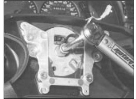
27.9 Tightening the steering wheel retaining bolt
