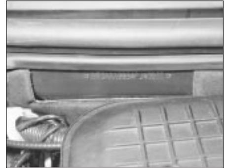
Vehicle identification number on engine compartment bulkhead
