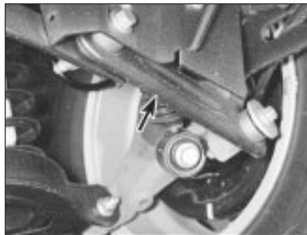
23.3 Front lower arm (arrowed)
