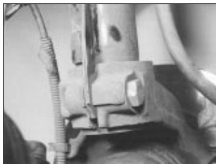
4.12A Steering knuckle-to-strut pinch-bolt
