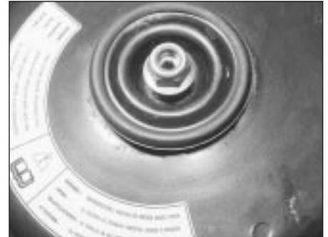
4.10 Front suspension strut upper mounting nut
