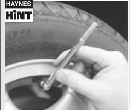
*Most garage forecourts have a pressure line which combines a gauge to check and adjust the tyre pressures, but they may vary in accuracy, due to general misuse and abuse. It therefore pays to carry a good-quality tyre pressure gauge in the vehicle, to make the regular checks required and ensure pressure accuracy.*
