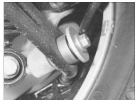
21.6 Front lower arm-to-knuckle mounting bolt
