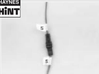
Whenever any wiring is disconnected, mark or label it as shown, to ensure correct reconnection . . .
