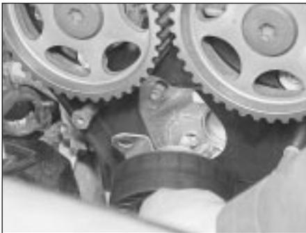
11.3 Removing timing belt tensioner
