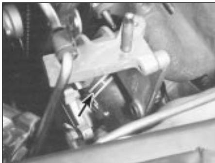
**8.8 Power steering system pump should be removed to reach water pump hose union (arrowed)**
