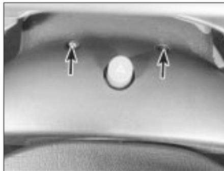
28.4D Upper shroud retaining screws (arrowed)
