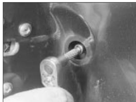
14.14B . . . and unscrew the handle mounting nuts
