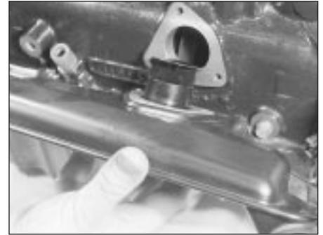
11.1C . . . unbolt crankcase ventilation system oil separator . . .
