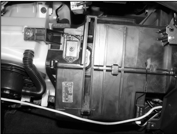
Slot where the pollen filters sit is easy to see and cut out with a Stanley knife
