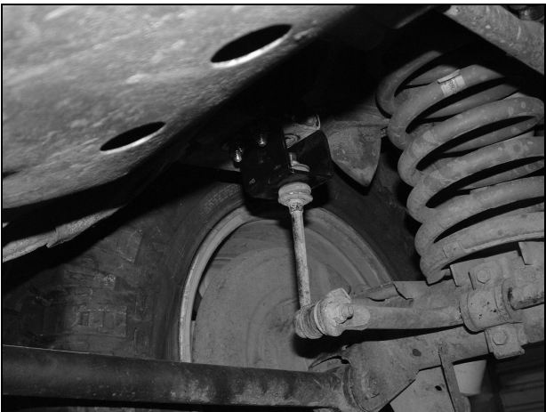
Right hand bracket installed
