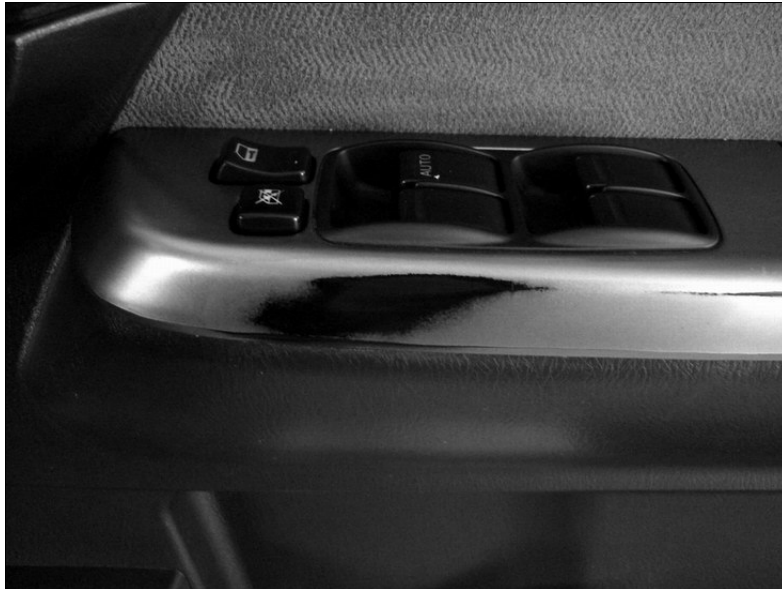
Worn door trim
