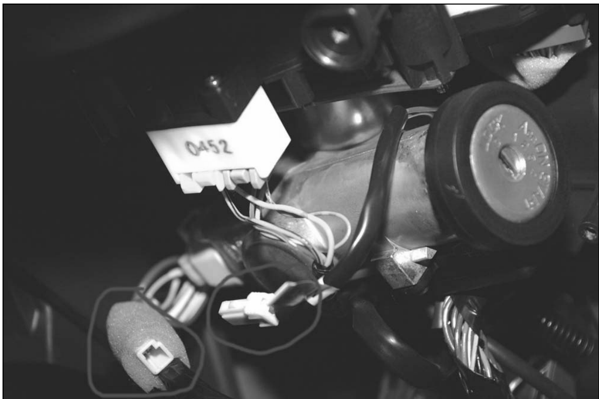
DIAGRAM OF 4.2 LITRE CONNECTOR THAT HAS BEEN UNPLUGGED
