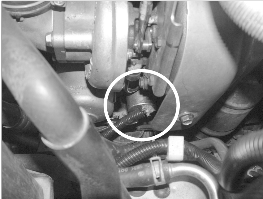
In this picture you can see the end of my oil pressure sender this is the position of pressure switch 1.
