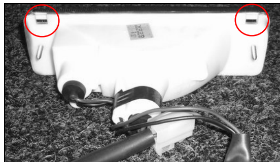
Vent holes are circled
