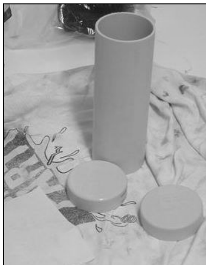
After cutting to length I sanded the tube and end caps ready for painting. Is much easier to do before assembling.
