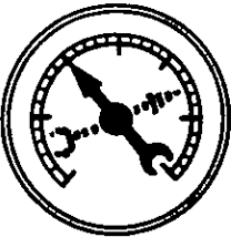
Weak Valve Spring. From 10 to 22 when accelerating engine, and becomes greater as increasing speed.
