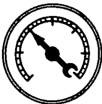
Late Timing of Valves. Remains steady between 8 to 15.
