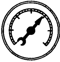
Normal Engine. Around 18 to 20 vacuum with slight fluctuation at idling speed.
