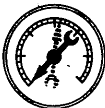
Choked Muffler. Normal at first, drops to zero and then builds up to 16.
