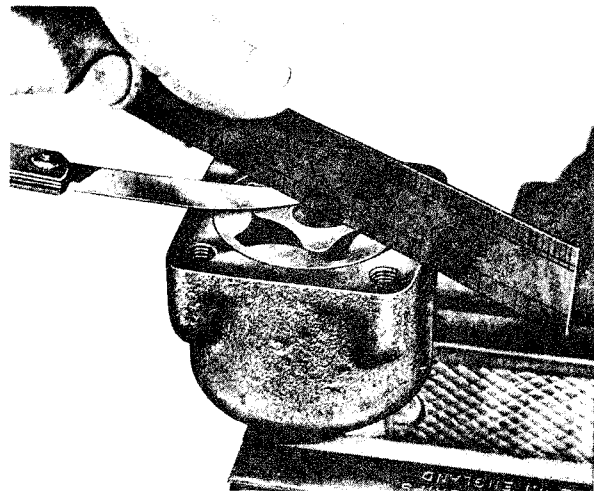
Checking Rotor End Clearance. L10
