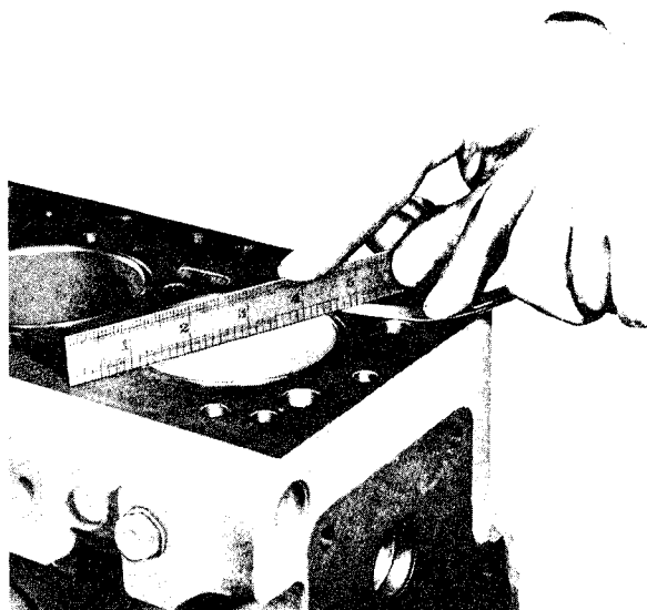
G2 Method of checking Liner protrusion.
