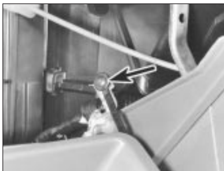
10.15 Glovebox damper retaining screw (arrowed)
