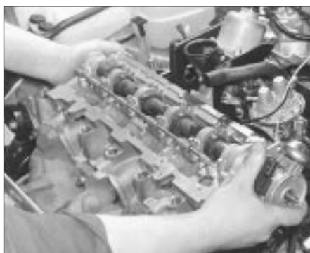
13.27 Refitting the cylinder head
