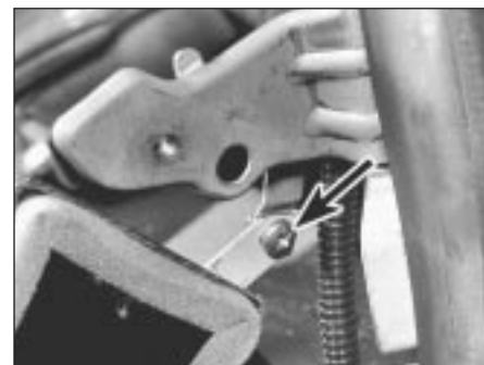
10.5a Undo right-hand duct retaining screw (arrowed) . . .
