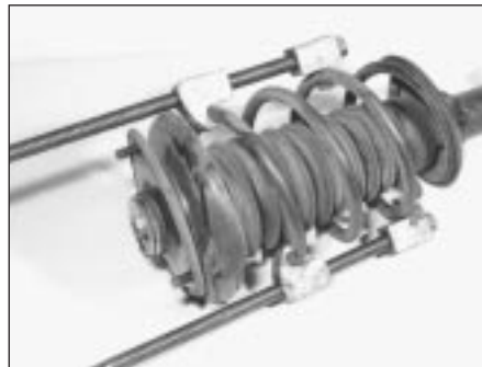
6.2 Compress coil spring with suitable pair of spring compressors . . .
