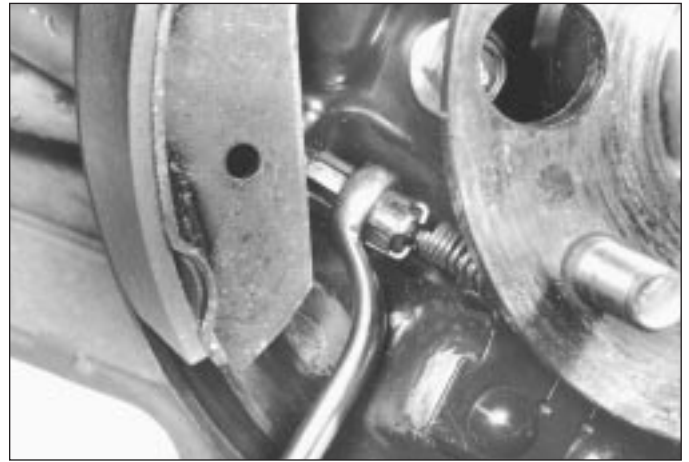
12.2a Using 12 mm spanner to compress handbrake cable retaining tangs
