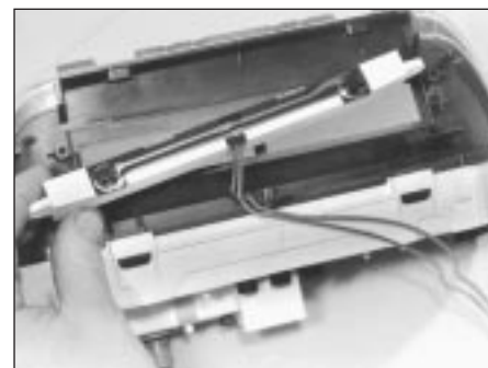
11.3 Removing instrument illumination panel
