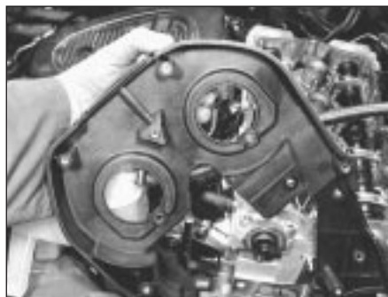
7.9c Removing timing belt upper left-hand (inner) cover - K16 engine
