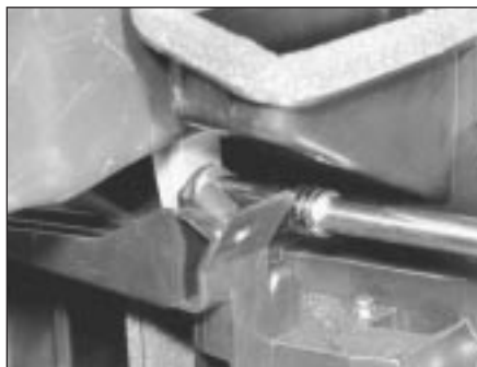
10.10b ... and remove heater retaining nuts
