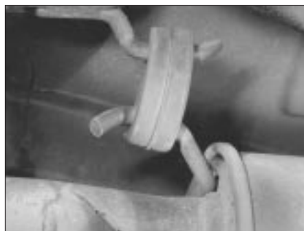
18.2 Exhaust system rubber mounting
