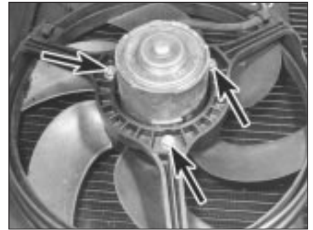
8.11 Cooling fan motor retaining nuts (arrowed)
