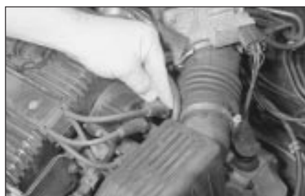
A Check that the distributor HT lead connections are clean and secure
