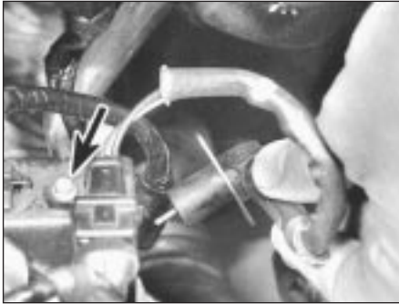
6.3 Removing crankshaft sensor (wiring lead screw arrowed)
