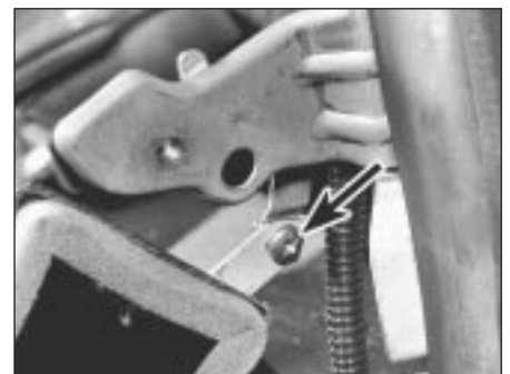
10.5a Undo right-hand duct retaining screw (arrowed) . . .
