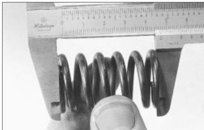
7.19 Measuring valve spring free length
