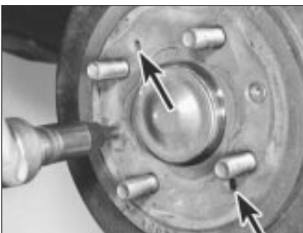
17.3 Removing brake drum retaining screws (jacking holes arrowed)
