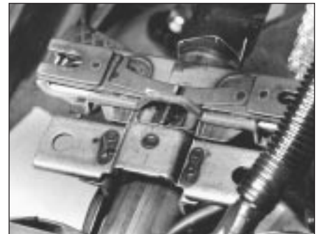
20.5 Fitted positions of upper mounting assembly components
