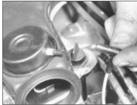
4.4 Disconnect vacuum pipe from control valve to check operation of system components
