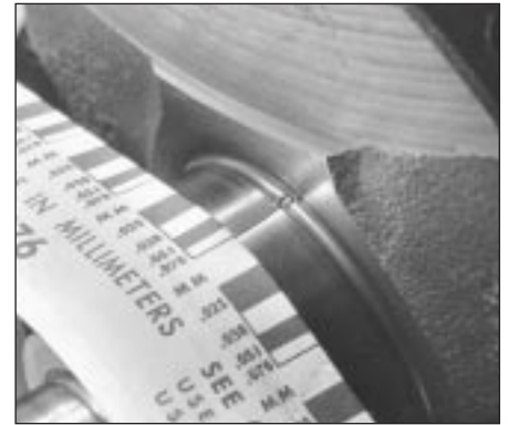
18.18 Using scale on Plastigauge envelope to check (at widest point) width of crushed Plastigauge
