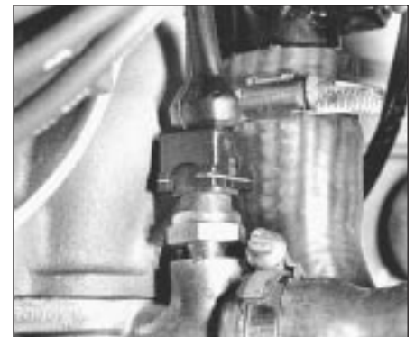
9.6 Coolant temperature gauge sender unit
