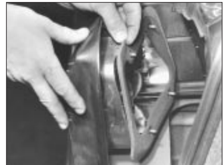
7.15 Withdraw rear lamp unit noting rubber seal
