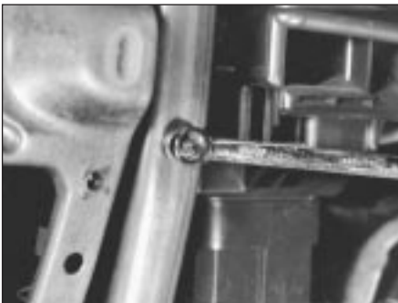
15.41a Undo inertia switch retaining nut . . .
