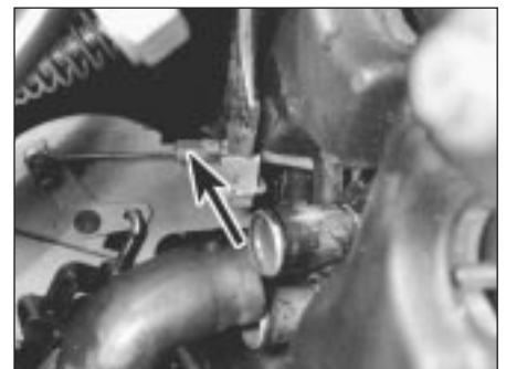
10.2c . . . and free heater valve cable from retaining clip
