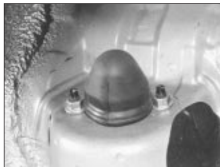
13.3 Remove luggage compartment side trim to gain access to strut upper mounting nuts - 414 models
