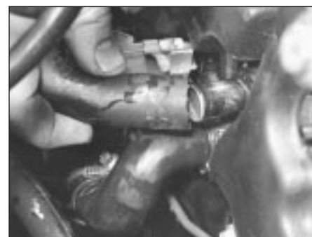
10.2b Disconnect heater feed and return hoses . . .
