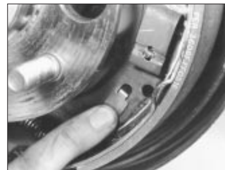
16.10 Ensure handbrake stop lever is correctly located
