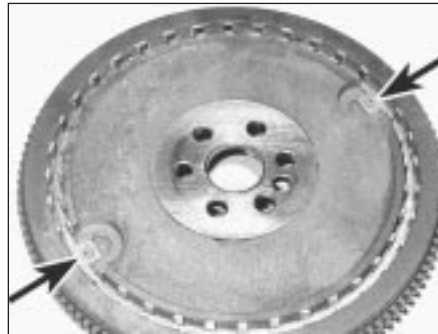
6.6 Reluctor ring-to-flywheel screws (arrowed)
