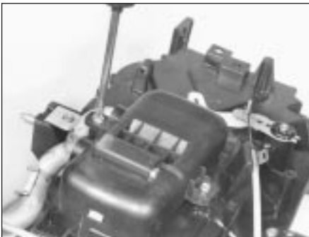
10.13a Undo two matrix cover retaining screws ...
