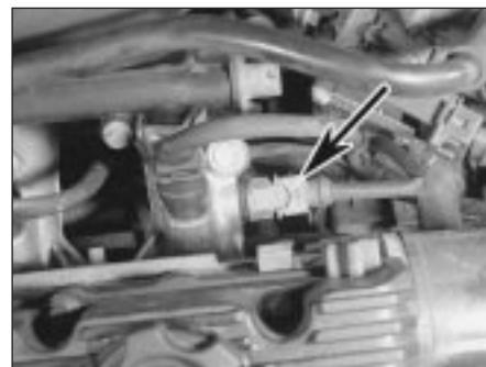
14.49 Intake air temperature sensor multiplug (arrowed)
