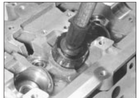
11.8 Use a valve-grinding sucker to extract hydraulic tappets
