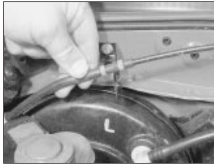
10.2 Releasing accelerator cable from retaining clip on engine compartment bulkhead
