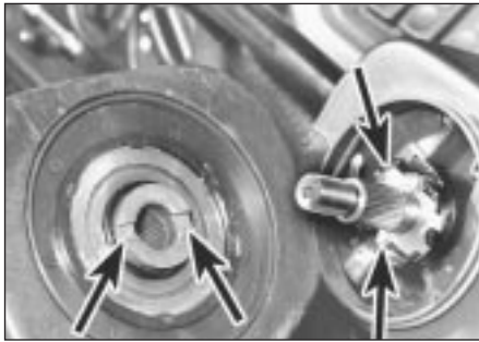
18.6a Ensure steering wheel cut-outs are correctly engaged with indicator cancelling cam tabs (arrowed) . . .
