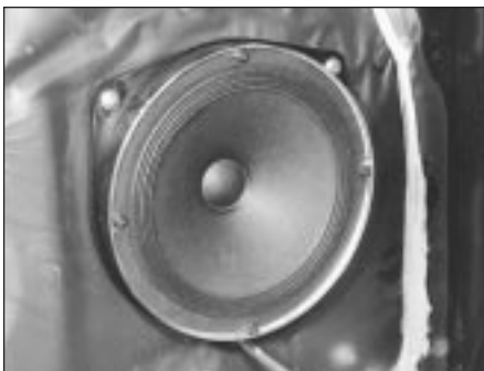
25.2a Slacken three retaining screws . . .
