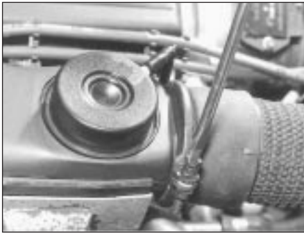
3.4 Slacken clamp to disconnect intake hose from air cleaner assembly metal intake duct
