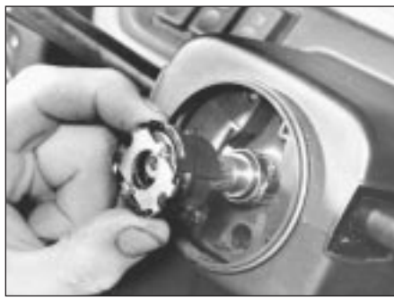
19.14 Ensure that indicator cancelling cam is correctly engaged with combination switch assembly
