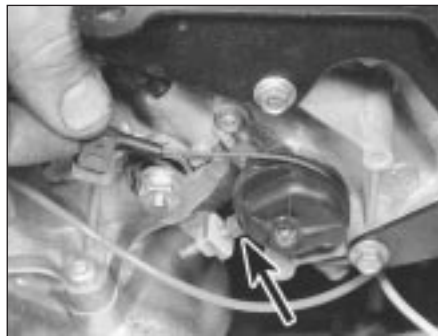
12.2 Releasing clip to disconnect choke cable from carburettor - fast idle adjusting screw arrowed
