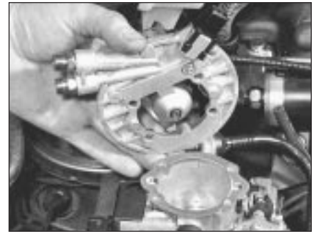
15.3b Remove injector housing from throttle body - noting gasket
