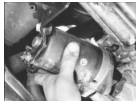
10.6c Removing the starter motor
