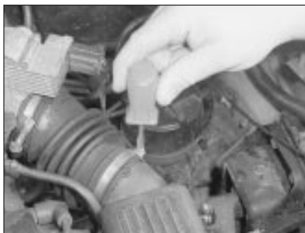
3.2 Releasing throttle housing-to-air cleaner securing clips
