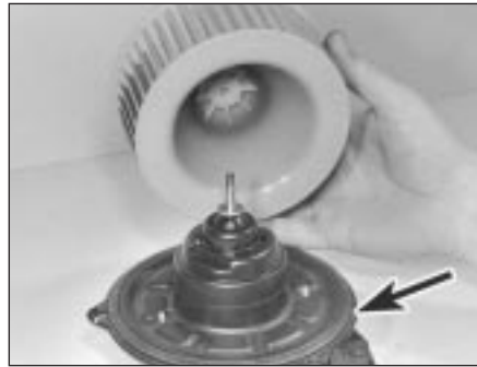
10.20e . . . and lift off fan (seal arrowed)
