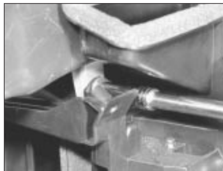
10.10b ... and remove heater retaining nuts
