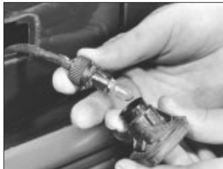
5.16 ... then withdraw lamp and pull out bulbholder
