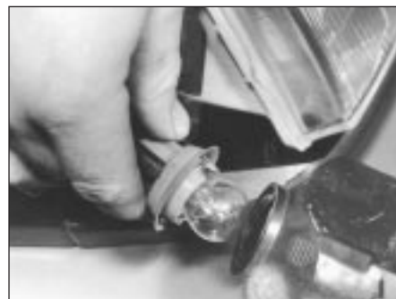
5.12 ... then withdraw indicator lamp and twist bulbholder free
