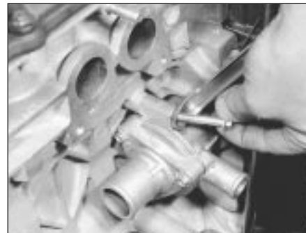
6.4a . . . unscrew dipstick tube retaining bolt . . .
