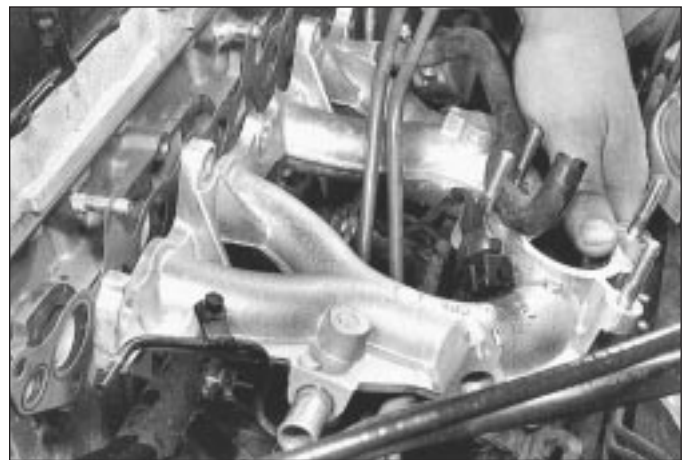
17.6b Remove inlet manifold and withdraw gasket
