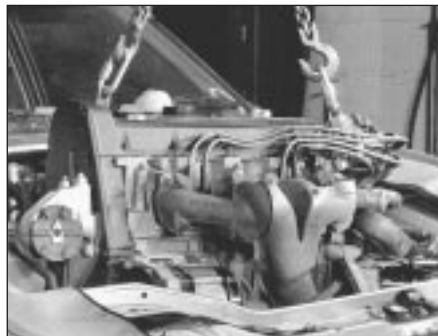
4.34 Lifting out engine/gearbox unit
