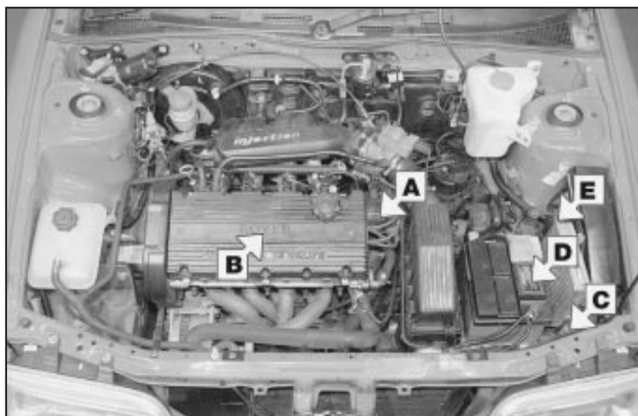
D Check the security and condition of the battery connections
