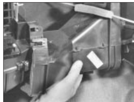
10.4 Remove blower motor-to-heater unit duct
