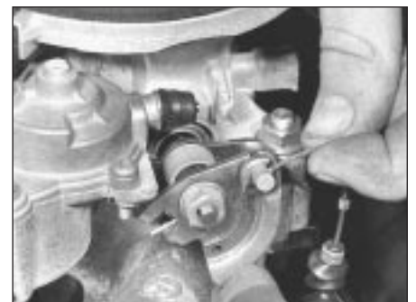
11.2 Disconnecting accelerator cable from throttle cam pulley
