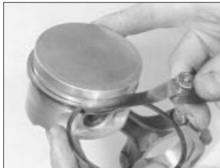
13.5a Measuring piston ring-to-groove clearance
