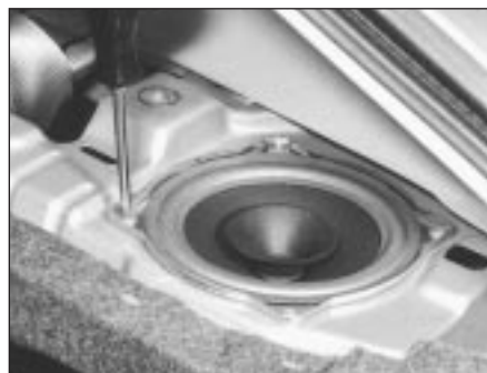
25.5 Rear speakers are retained by four screws - 214 models
