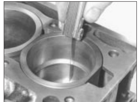
13.5b Measuring piston ring end gap
