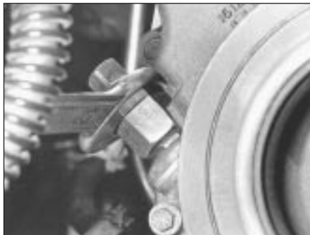
16.4 Unscrewing oil pressure relief valve threaded plug
