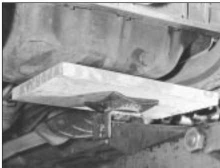
19.7a Use trolley jack with wooden spacer to adjust height of engine/gearbox unit
