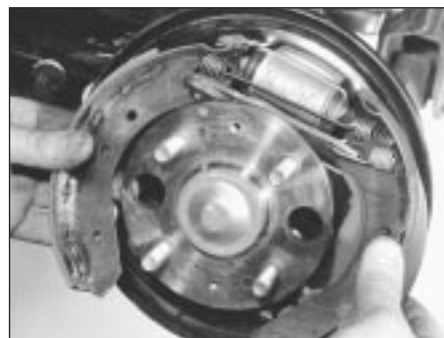
16.5d . . . and manoeuvre shoe and adjuster strut assembly away from backplate
