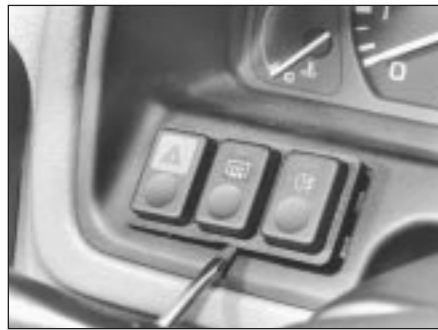
10.2a Carefully prise left-hand switch assembly out of instrument panel shroud ...
