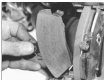
11.4 Removing pads with springs and shims
