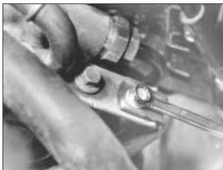
25.2b Remove outlet pipe bracket retaining bolt . . .
