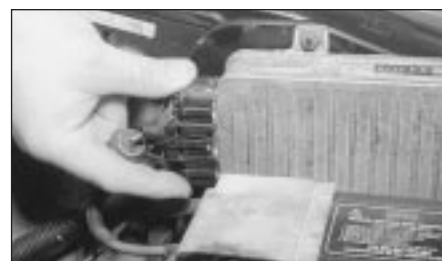
E The ECU wiring plugs may cause problems if dirty or not properly connected
