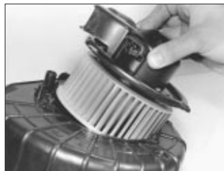
10.20c Undo motor retaining bolts and withdraw motor from unit
