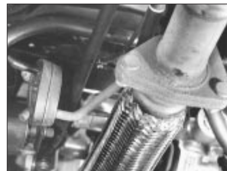
18.7 Front pipe-to-intermediate pipe flange joint and mounting rubber
