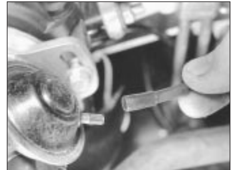
5.3 Disconnecting vacuum pipe from distributor vacuum diaphragm unit
