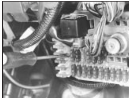
14.7a Release left-hand fuse panel . . .
