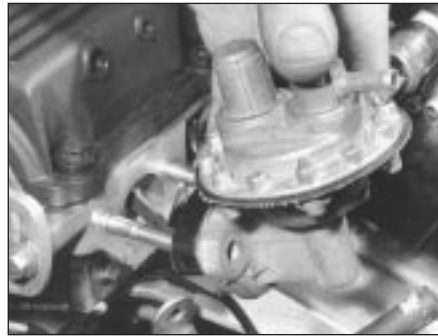
6.5 Removing fuel pump and insulating block
