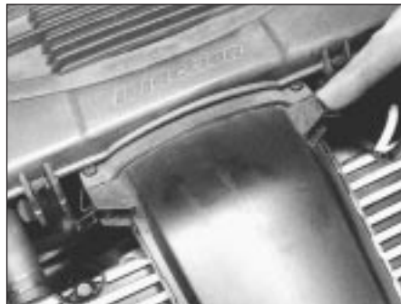
3.1 Releasing clips to separate intake duct from air cleaner
