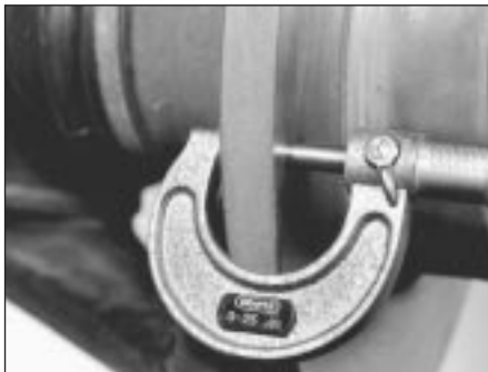
13.3 Using a micrometer to measure brake disc thickness
