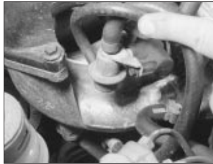
14.25 Fuel pressure regulator location - alloy inlet manifold
