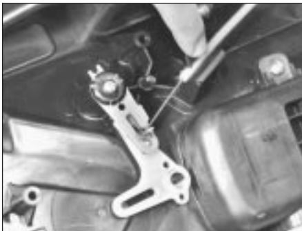
12.2a Disconnect control cables from heater unit . . .
