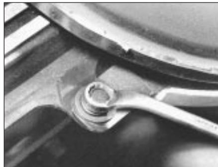
4.4 Unfastening intake duct-to-support bracket retaining bolt
