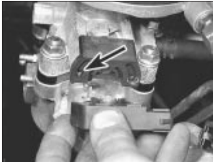
15.19 Ensure potentiometer tongue engages correctly with throttle lever (spacer arrowed)
