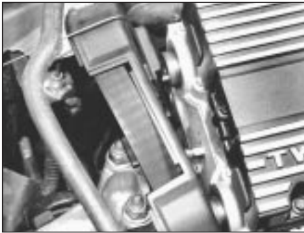
11.9 Secure partly-removed timing belt upper left-hand (inner) cover clear of cylinder head - K16 engine
