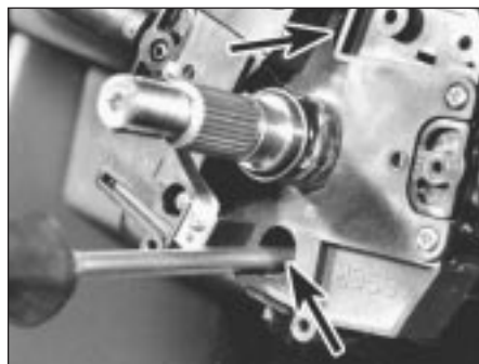
19.5 Combination switch assembly is retained by two screws (arrowed)
