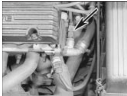
14.53 Coolant temperature sensor multiplug (arrowed)
