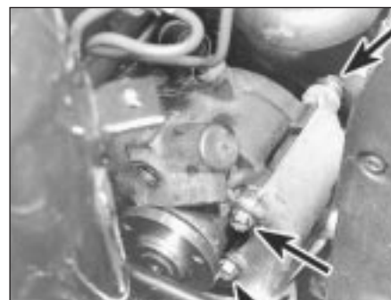
25.5a Unscrew power steering pump mounting bolts (three arrowed) . . .
