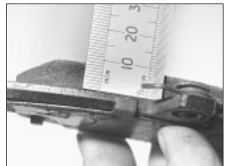
11.5 Measuring thickness of brake pad friction material
