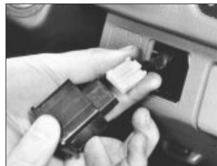
4.19b ... and disconnect wiring connectors
