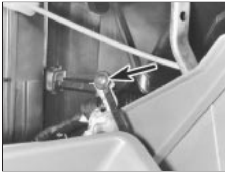
10.15 Glovebox damper retaining screw (arrowed)
