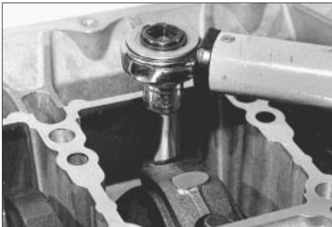
19.17a Tighten connecting rod big-end bearing cap bolts to specified torque wrench setting (first stage) . . .
