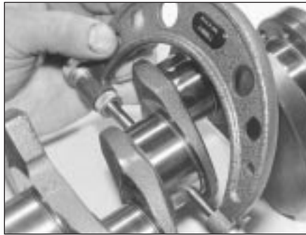
14.8 Measuring crankshaft journal diameter
