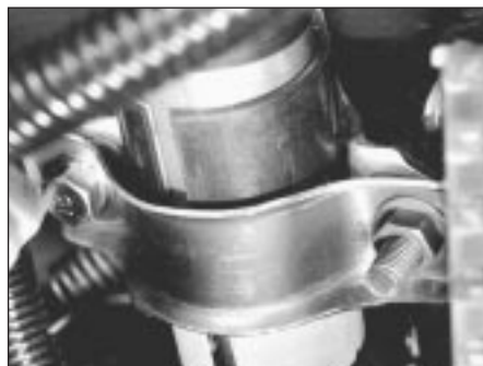
19.9 Steering column lower mounting clamp components
