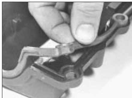
5.12a Ensure seal is correctly seated in cylinder head cover groove . . .
