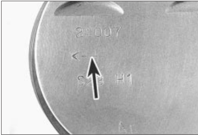
19.15a Arrow or FRONT marking (arrowed) on piston crown must point to timing belt end of engine
