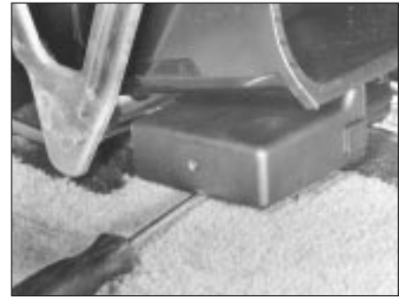
3.15a Use a screwdriver to release relay module retaining clip . . .
