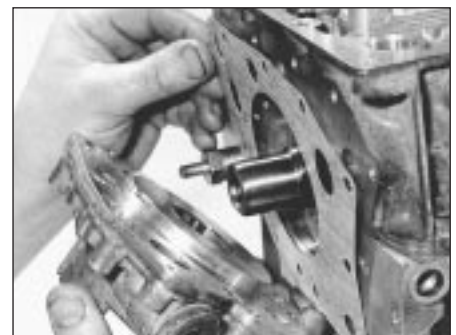
18.31a Use grease to stick new gasket in place when refitting oil pump
