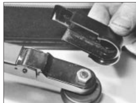
23.3 Removing cover to reveal tailgate wiper arm spindle nut
