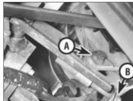
8.9b . . . and lower adjusting arm bolt (A) then rotate adjuster bolt (B) to slacken drivebelt tension
