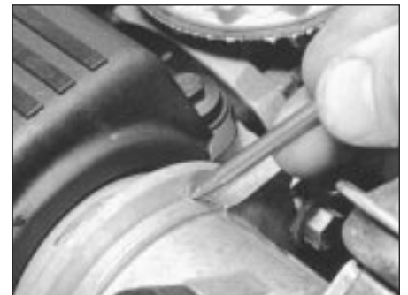
5.5 Making alignment marks on distributor body and cylinder head
