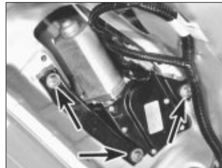
23.7 Tailgate wiper motor mounting bolts (arrowed)
