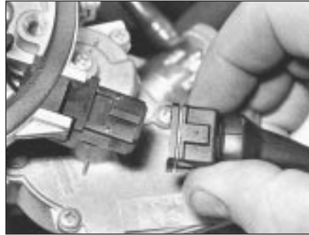
15.2 Disconnecting wiring connector from injector housing
