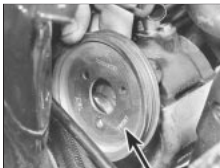
25.4b . . . and withdraw pulley. Note FRONT mark on pulley face (arrowed)
