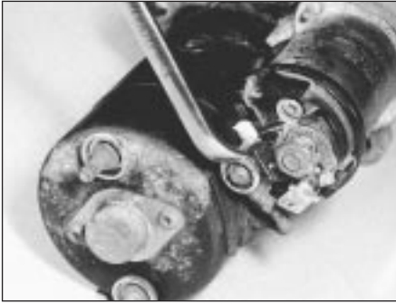
11.14 Unscrew nut and disconnect starter motor lead from solenoid terminal
