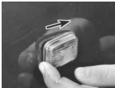
5.15 Push indicator side repeater lamp to right ...
