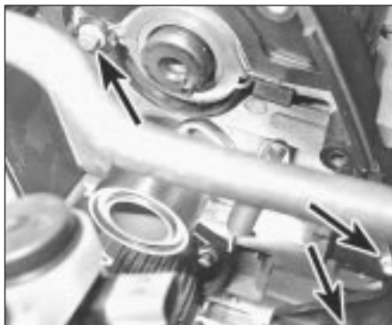
7.9a Timing belt upper left-hand (inner) cover fasteners (arrowed) - K8 engine
