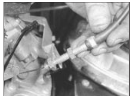
9.2 Disconnecting accelerator cable from carburettor
