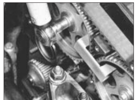
9.23b Locking camshafts in position with fabricated tool - K16 engine
