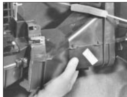
10.4 Remove blower motor-to-heater unit duct
