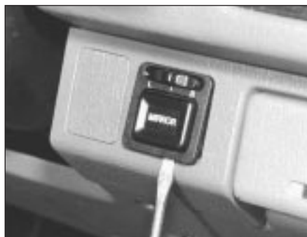
4.19a Carefully prise fascia switches out of position ...
