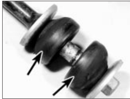
9.5 Renew tie bar mounting bushes if damaged (arrowed)
