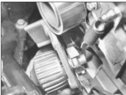
7.5 Removing the coolant pump
