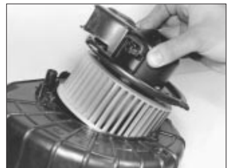
10.20c Undo motor retaining bolts and withdraw motor from unit
