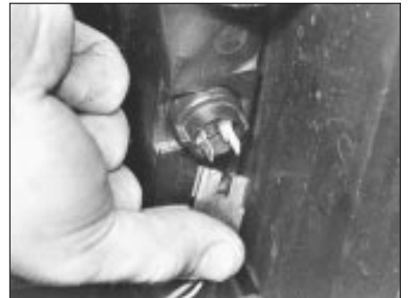
5.4b Disconnecting wiring connector from radiator switch
