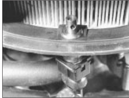
15.28 Remove air cleaner metal intake duct to gain access to intake air temperature sensor
