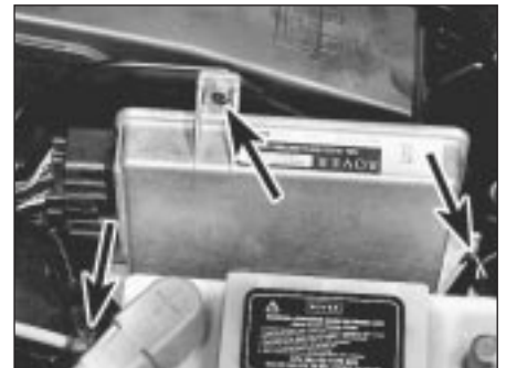
15.21b . . . then undo ECU mounting nuts (arrowed) and remove unit
