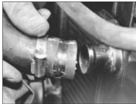
5.6a Slacken clips and disconnect top hose from radiator . . .
