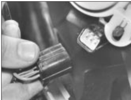
7.4 Disconnecting headlamp wiring connector
