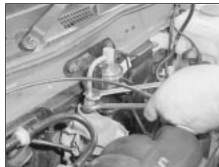
5.3 Loosening fuel filter pipe union
