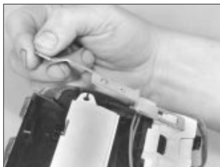
11.2b ... and remove upper mounting brackets from instrument panel
