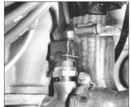
9.6 Coolant temperature gauge sender unit
