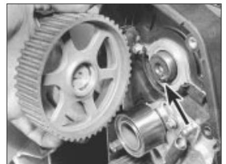
9.12 Removing camshaft sprocket (roll pin arrowed) - K8 engine
