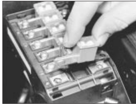
3.10b . . . then undo retaining screws and remove fusible link
