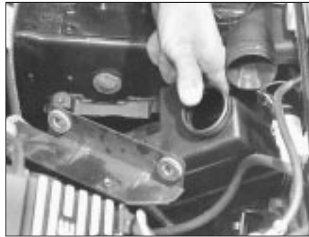
3.6b . . . then remove resonator
