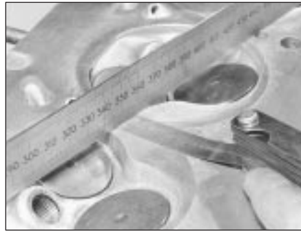
7.6a Checking a cylinder head gasket surface for warpage
