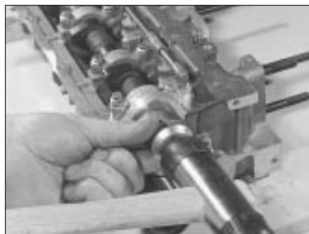
11.31 Fitting a new camshaft right-hand oil seal - K8 engine
