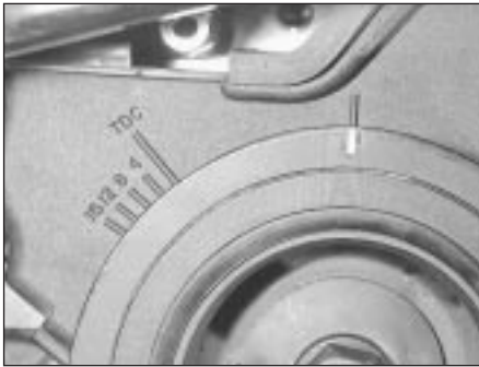
8.6 Crankshaft pulley mark aligned with timing belt lower cover mark at 90° BTDC
