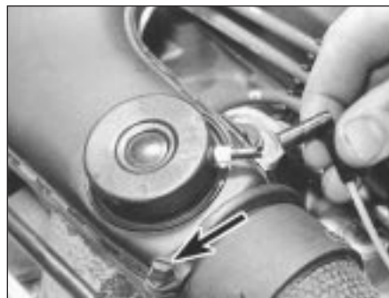
4.11 Disconnecting vacuum pipe from air temperature control valve - intake hose-to-metal intake duct securing clamp (arrowed)
