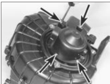
10.20a Remove motor cover retaining screws (arrowed) . . .
