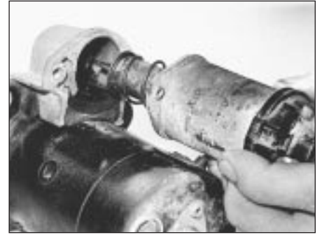
11.16 . . . then release solenoid plunger from lever and remove assembly from motor
