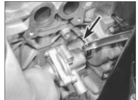
6.4b . . . and withdraw thermostat housing (O-ring arrowed) - inlet manifold removed for clarity
