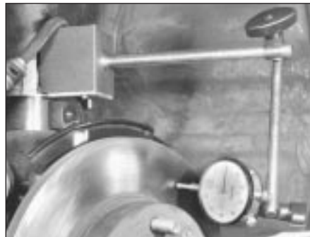
13.4 Using a dial gauge to check brake disc run-out
