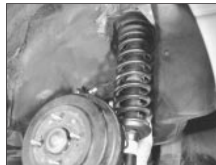
13.4 Removing rear suspension strut
