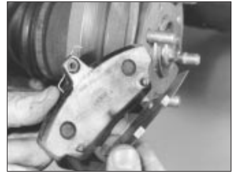
11.9 . . . and fit shims on pads
