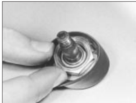
23.4a Unscrew wiper spindle retaining nut . . .
