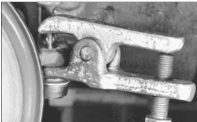
28.4 Using a universal balljoint separator to free track rod balljoint from swivel hub
