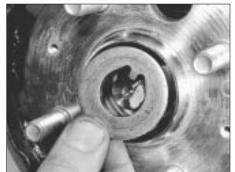
11.9b . . . and washer, ensuring its tooth engages with stub axle groove
