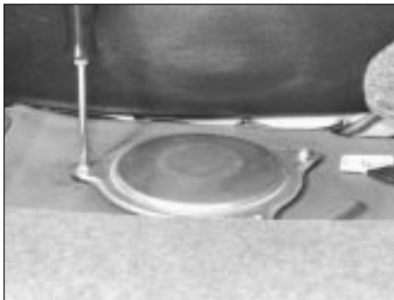
7.4 Undo three screws to remove fuel gauge sender unit access cover
