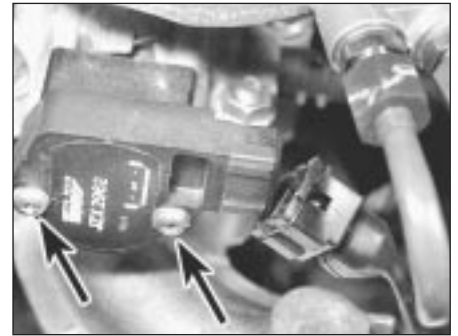
15.17 Disconnecting throttle potentiometer wiring connector (mounting screws arrowed)
