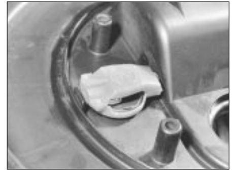
4.9 Thermac switch is clipped into air cleaner assembly
