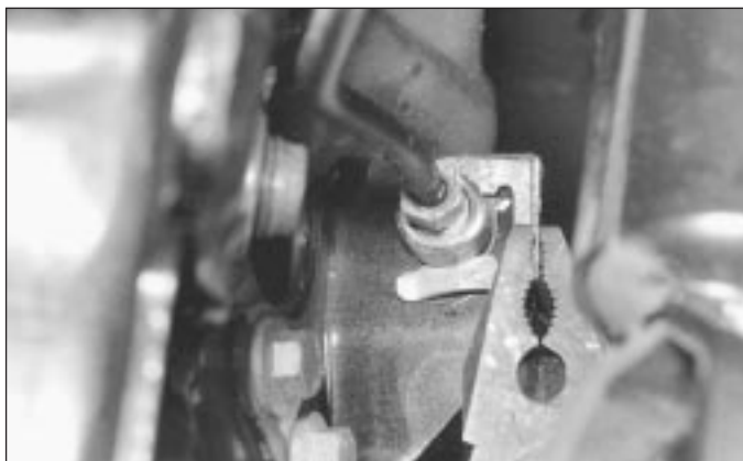
16.3 Remove retaining clip and free brake hose from trailing arm
