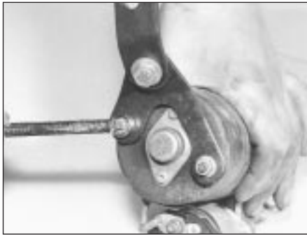
11.2 Undo retaining nuts and remove support bracket from starter motor
