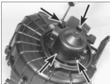
10.20a Remove motor cover retaining screws (arrowed) . . .
