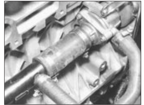
6.10 Thermostat housing and coolant hoses refitted
