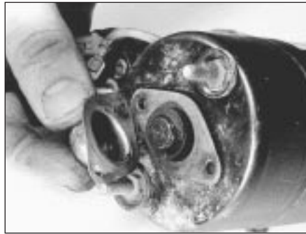
11.3 Remove cover to gain access to armature C-clip
