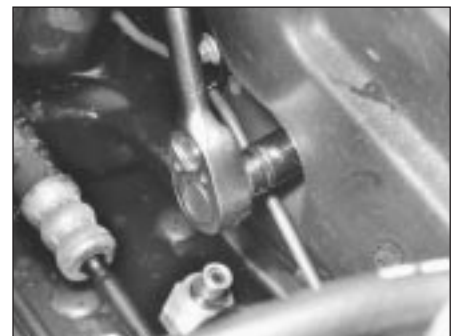
10.2d Slacken and remove heater unit lower mounting nut
