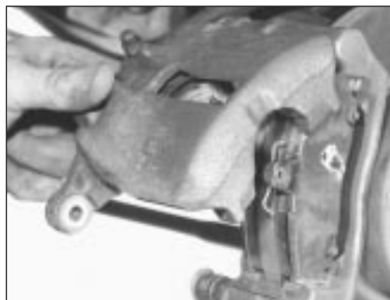
11.2b . . . and pivot caliper away from disc
