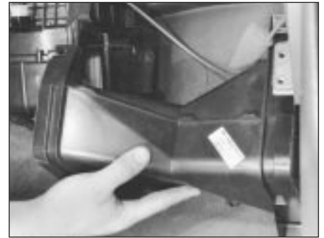
10.17 . . . then remove blower motor-to-heater unit duct
