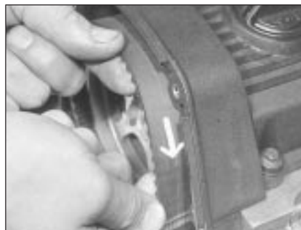
8.13 Mark direction of rotation of timing belt before removal
