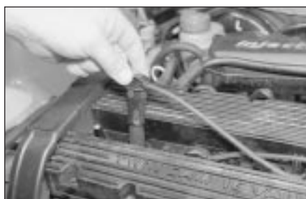
B Check that the spark plug HT lead connections are clean and secure - cover removed
