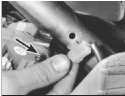
10.7a Release wiring connector from steering column support bracket and remove fusebox nut (arrowed)
