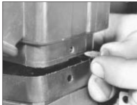
10.9 Remove retaining stud and disengage rear heater duct sleeve from heater unit
