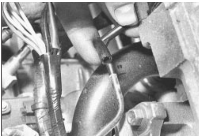
17.6a Ensure all vacuum pipes and hoses are disconnected
