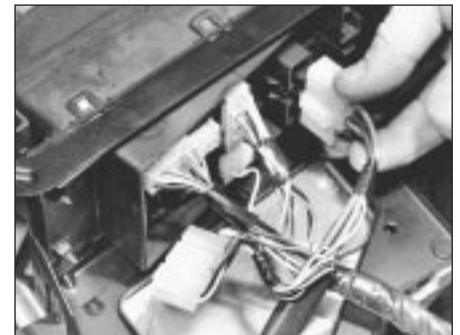
4.11a Disconnecting engine harness wiring connectors from underside of fusebox . . .
