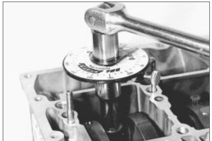
19.17b . . . then use angular torque gauge to tighten bolts through angle specified (second stage)
