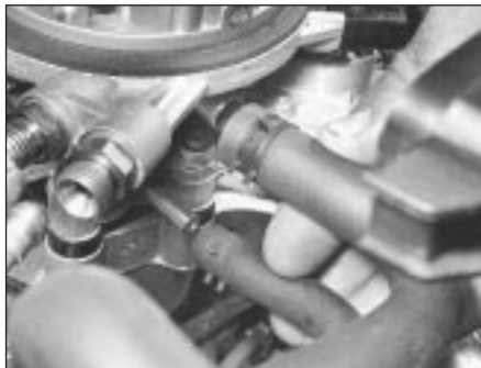
13.7 Disconnecting breather hoses from throttle housing
