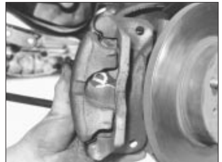
13.6 Removing caliper assembly
