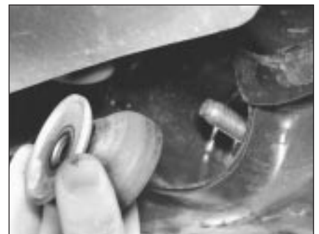
9.7 . . . then refit tie bar to subframe and install second mounting bush and flange washer
