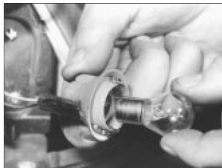
5.13 Indicator bulbs are of bayonet type
