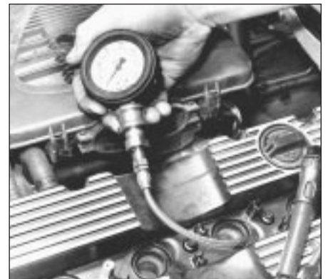
3.4 Measuring compression pressure
