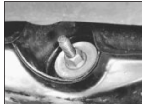
9.3 Tie bar retaining nut is accessed from front of subframe
