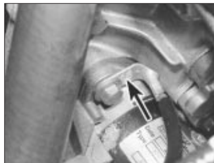
10.6b Starter motor upper mounting bolt and earth strap (arrowed) - viewed from above
