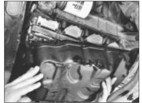
14.9 Removing the sump
