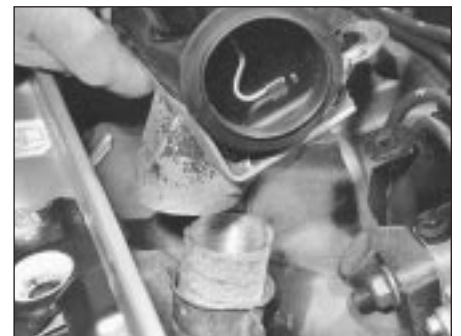
4.12 Do not lose hot air intake connector hose when removing air cleaner metal intake duct
