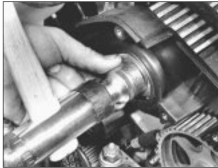
10.4 Fitting a new camshaft right-hand oil seal - K16 engine
