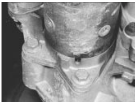
10.6a Starter motor lower mounting bolts viewed from underneath
