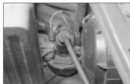
C Check that the ignition coil HT and LT lead connections are clean and secure
