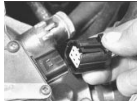
15.12 Disconnecting stepper motor wiring connector
