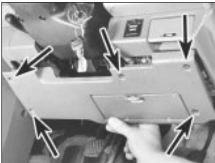
14.6 Remove retaining screws (arrowed) and withdraw right-hand lower fascia panel
