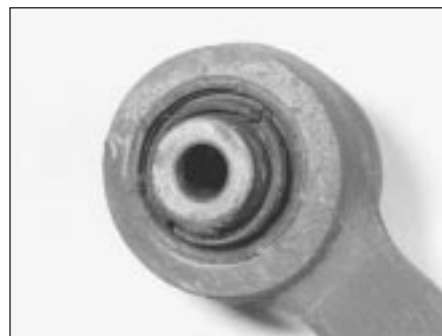
15.7 Examine lateral link bushes for signs of wear and renew if necessary
