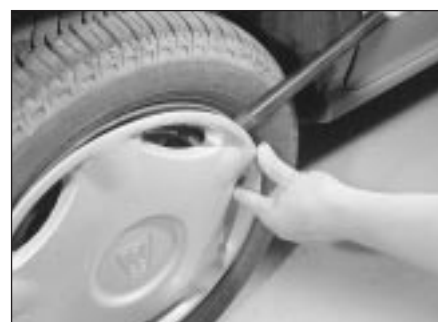
3 Remove the trim to expose the wheelnuts
