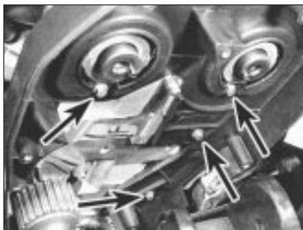
7.9b Timing belt upper left-hand (inner) cover fasteners (arrowed) - K16 engine
