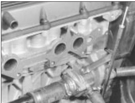
16.13a Fit a new manifold gasket . . .
