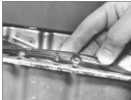
14.12 Sump gasket pegs must engage with sump mating surface holes
