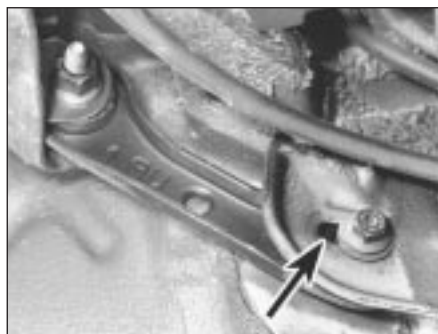
15.3 Front lateral link to body mounting bolt (arrowed) is slotted to permit rear wheel alignment
