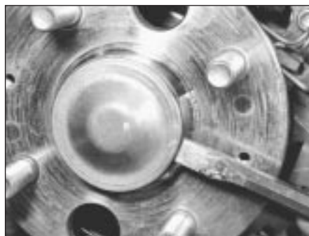
11.2 Prise off centre cap to gain access to rear hub nut
