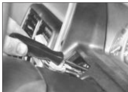
10.5a Instrument panel shroud lower retaining screws are accessed through switch apertures
