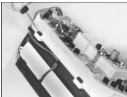
11.6 Release retaining clips and separate instrument panel case and cover
