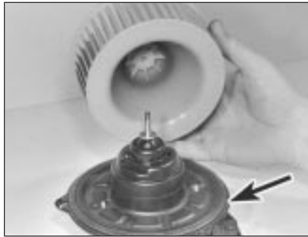
10.20e . . . and lift off fan (seal arrowed)
