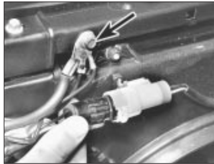
5.4a Disconnect cooling fan wiring connector then remove earth lead retaining bolt (arrowed)
