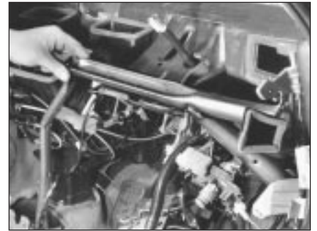
10.7b Remove mounting bolts and manoeuvre steering column mounting bracket out of position
