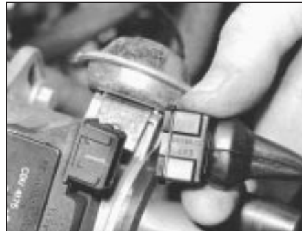
5.2 Disconnecting wiring connector from ignition amplifier module
