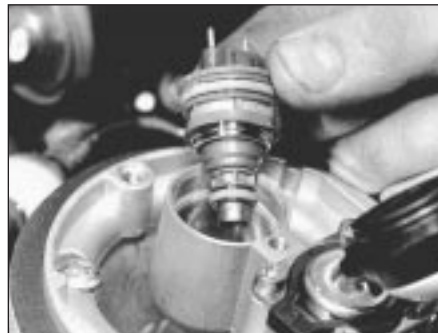
15.8b . . . and withdraw injector
