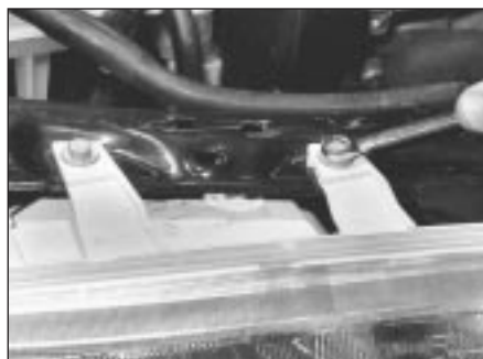
7.3b . . . and two headlamp retaining bolts
