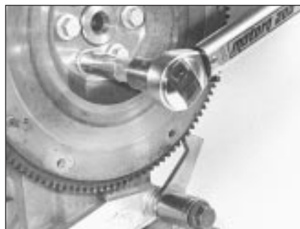
18.30c Use fabricated tool to lock flywheel while slackening or tightening flywheel bolts
