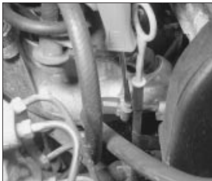
16.16 Releasing coolant hose from inlet manifold
