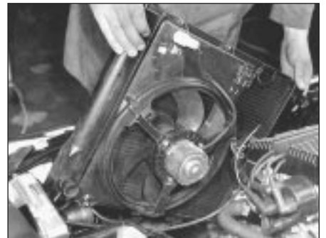
5.7c . . . and manoeuvre radiator out of engine compartment
