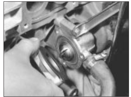
6.1 Thermostat can be removed without disturbing housing if inlet manifold is first removed
