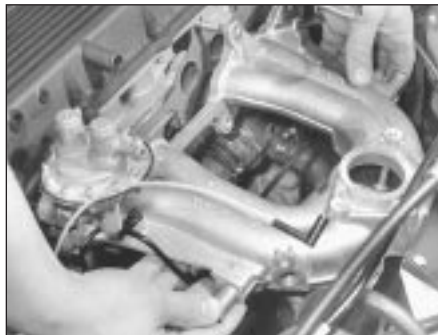
16.13b . . . and fit inlet manifold - less carburettor
