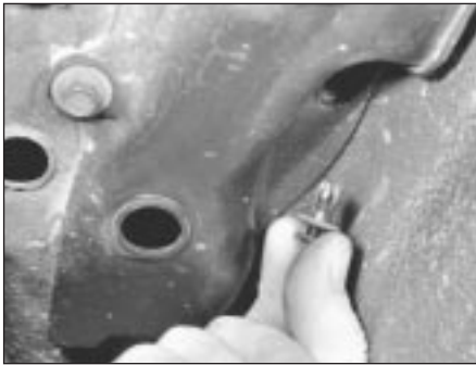
8.3 Removing cover retaining bolt (arrowed) and screw retaining plugs
