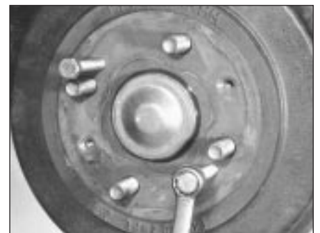
17.4b Brake drum can be drawn off hub by using two 8 mm bolts
