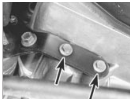
10.5 Starter motor support bracket-to-gearbox bolts
