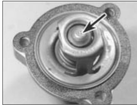
6.8 Note temperature specification stamped on thermostat end
