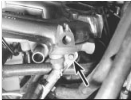
16.11a Inlet manifold support stay upper end bolt (arrowed)
