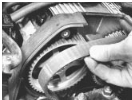
8.16 Refitting timing belt - K16 engine
