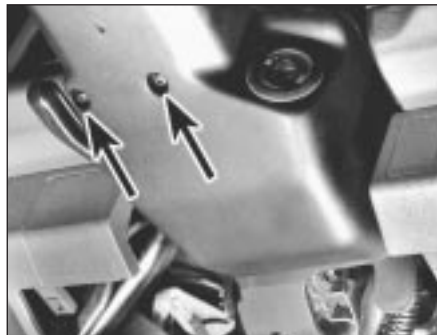
19.3b . . . undo lower shroud retaining screws (arrowed) . . .
