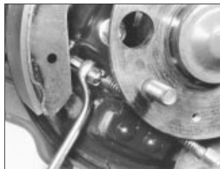
24.6 Using a 12 mm spanner to compress cable outer retaining tangs
