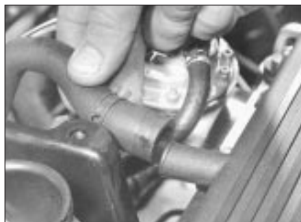
5.3a Disconnecting breather hose from cylinder head cover - K8 engine
