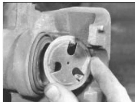
11.3 Removing circular shim from caliper piston
