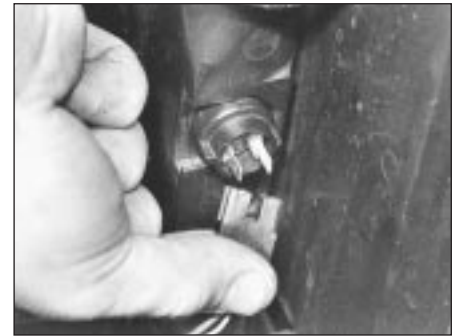
5.4b Disconnecting wiring connector from radiator switch
