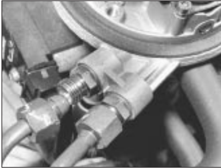
15.1 Disconnecting fuel feed and return pipes from injector housing
