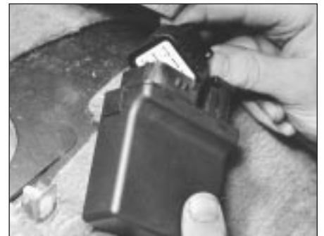
3.15b . . . then slide module out of position and disconnect its wiring connectors
