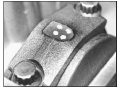
9.9 Mark big-end bearing caps before removal - No 4 cylinder cap shown
