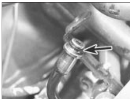
25.7 Always renew outlet pipe O-ring (arrowed)
