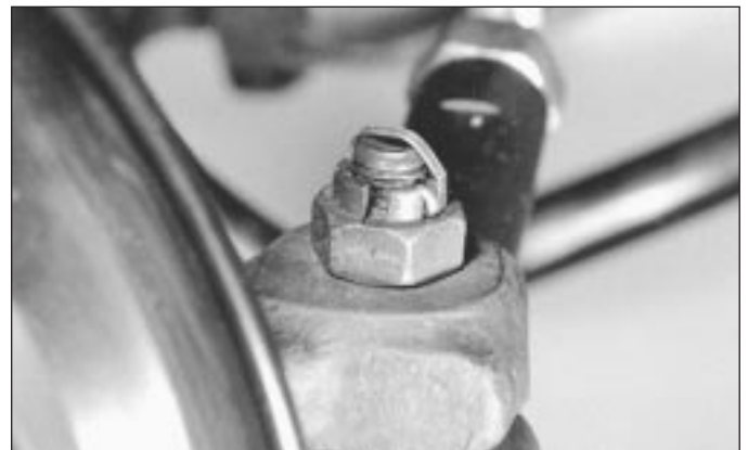
28.9 Secure balljoint retaining nut in position with new split pin
