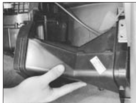
10.17 . . . then remove blower motor-to-heater unit duct
