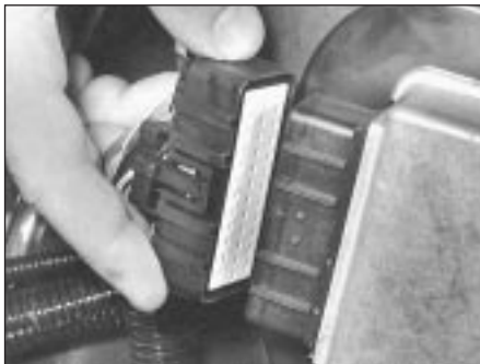
15.20 Disconnect wiring connector . . .
