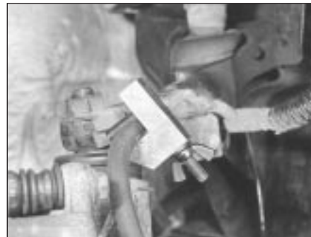
8.1 Using a brake hose clamp to minimise fluid loss
