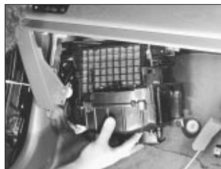
10.19b . . . and remove unit from behind fascia
