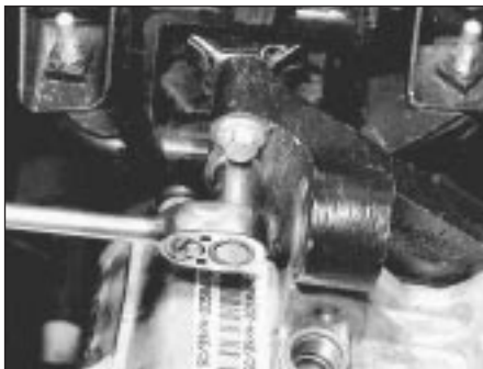
19.18 Slacken and remove gearbox bracket-to-mounting bolts . . .
