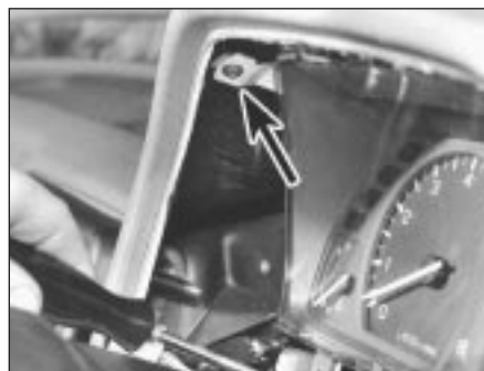
10.6a Remove instrument panel upper (arrowed) and lower retaining screws ...
