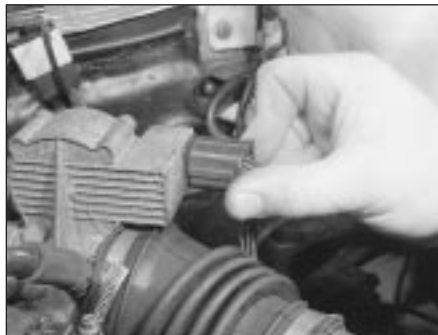
16.6 Disconnecting stepper motor multiplug
