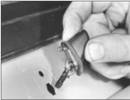
21.5 Removing tailgate washer jet - 214 models
