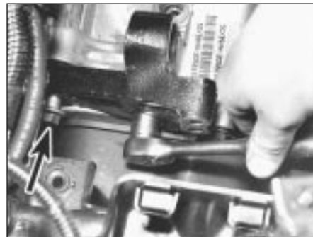
19.19c Gearbox bracket is retained by two bolts (one arrowed)
