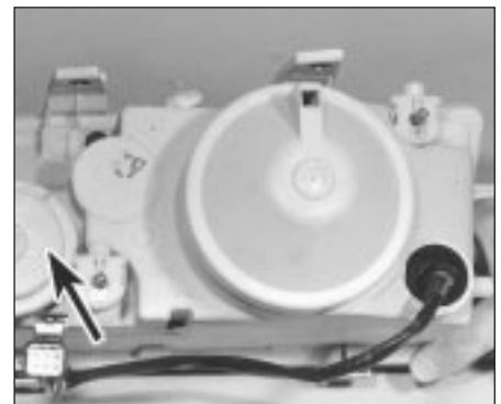
5.2 Remove large circular cover to access dip/main beam bulb and sidelamp bulbs and smaller cover (arrowed) to access individual main beam bulb
