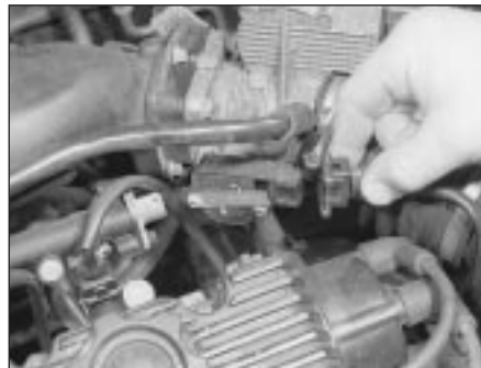
14.35 Disconnecting potentiometer multiplug - alloy inlet manifold
