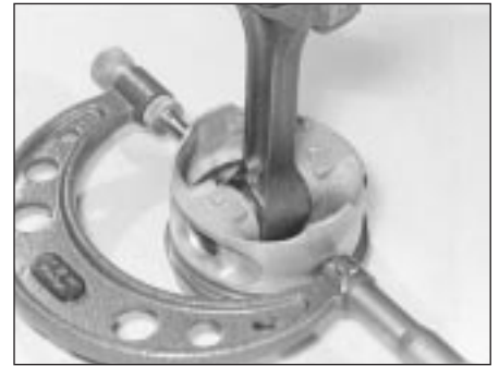
13.1 Measuring piston diameter
