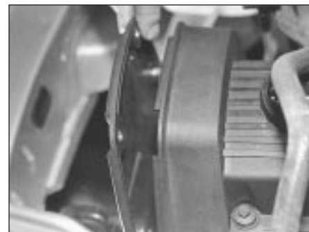
7.10 Ensure timing belt upper right-hand (outer) cover engages correctly with cylinder head cover - K8 engine
