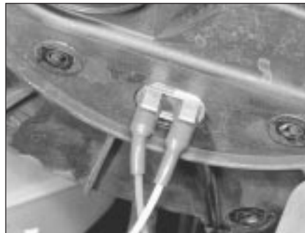
3.2 Note colour-coding of thermac switch vacuum pipes before disconnecting
