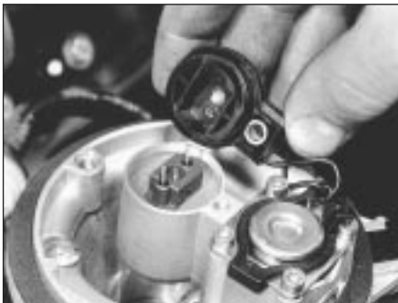
15.8a Remove screw then lift off injector connector cap . . .
