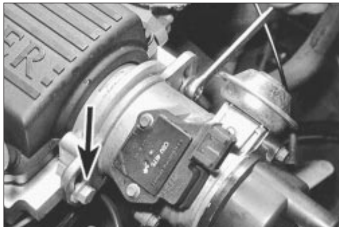
5.6 Unscrew distributor mounting bolts (remaining bolt arrowed) . . .
