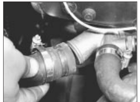
5.6b . . . and engine coolant elbow
