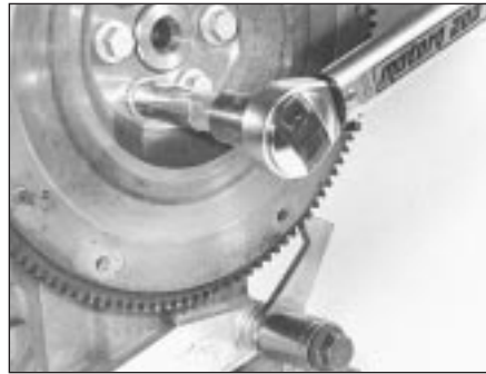
18.2 Using fabricated tool to lock flywheel in position
