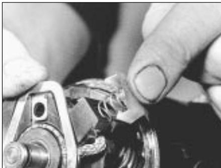
11.6b . . . remove brush spring caps and springs . . .
