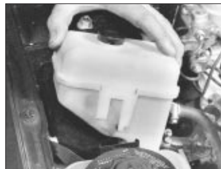
25.3 Removing power steering fluid reservoir from retaining clamp
