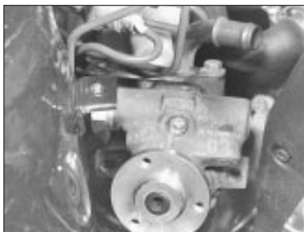
25.5b . . . and remove pump
