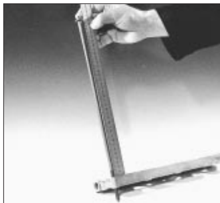
9.16 Checking length of cylinder head bolts
