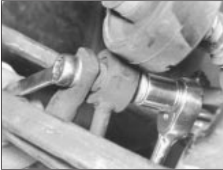
7.4 Slacken and remove anti-roll bar-to-connecting link bolts
