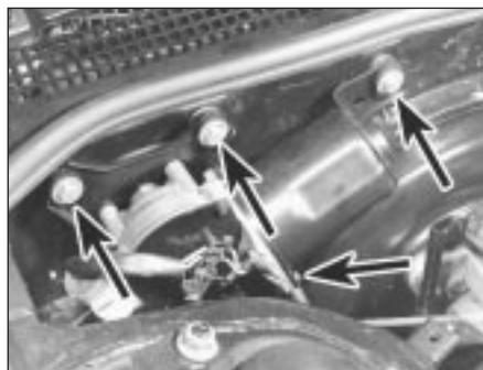
22.6 Windscreen wiper motor mounting bolts (arrowed - lower bolt hidden)
