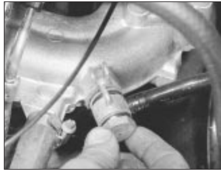
4.5 Ensure hose union locating pin is correctly located between lugs on inlet manifold
