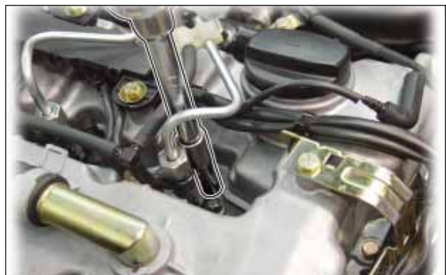
Glow plug wrench - special service tool (10 mm) Part No.: Y99220132B
