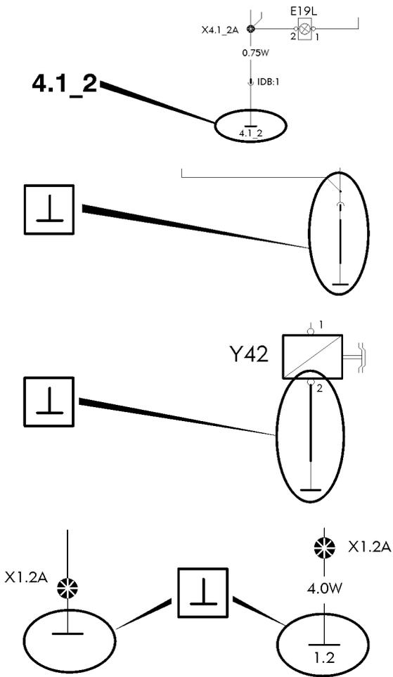
Earth connection point 4, earth connection 1 and wire 2.
