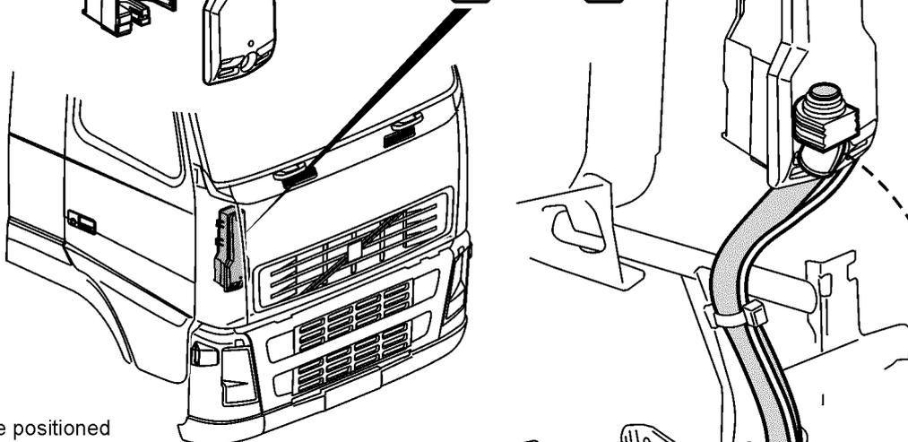
Wires must always be positioned in the lower channel of the bracket.
