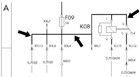
Conductor on circuit card.
