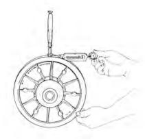
To correct spring tension displace spring end accordingly.
