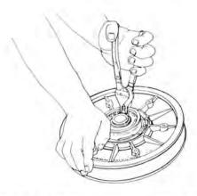
Check sliding half bushing wear, replace bushing if wear is excessive.
