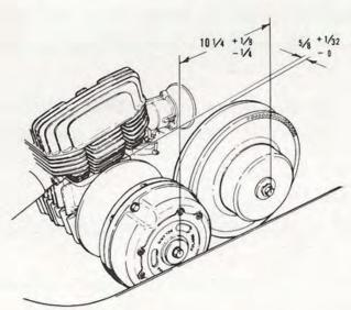
After alignment, you should very carefully start the engine, accelerate the machine to get the belt to the top of the drive clutch and make certain the belt is running in a straight line. Clutch center distance and alignment should be checked weekly or immediately after a belt is replaced.
