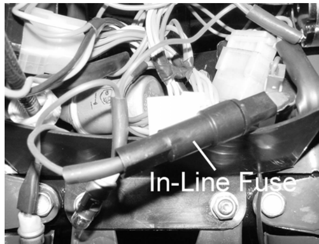
The #1 in-line fuse is located behind the headlight.
