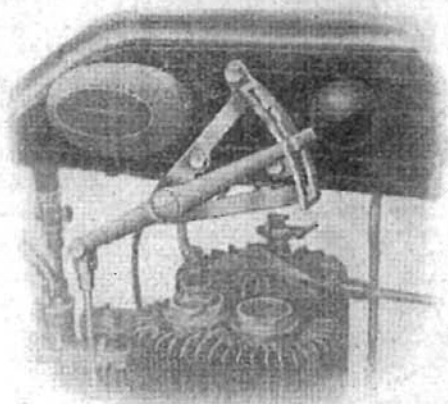
THE A.J.S. PATENT CHANGE SPEED LEVER.
