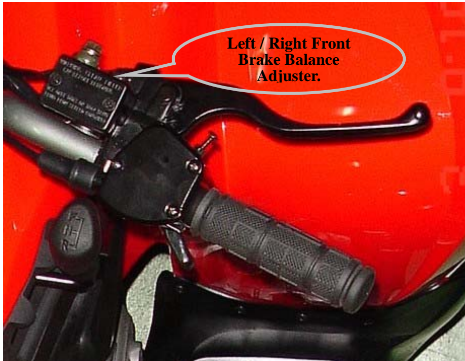
(STEP.5) The brake balance adjuster on right lever.
