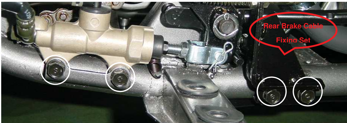
STEP.2) Take off the rear brake fixing set and the bolt of brake pump.
