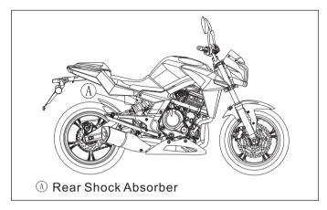
The rear shock absorber can be adjusted by changing the spring preload and rebound damping force for various riding and loading condition.
