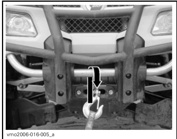
TYPICAL - FRONT ATTACHMENT LOCATION
