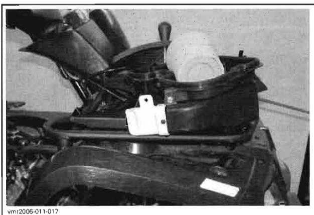
AIR FILTER HOUSING AND PLACE IT ON FRONT RACK (ON RENEGADE MODELS, REMOVE IT COMPLETELY)
