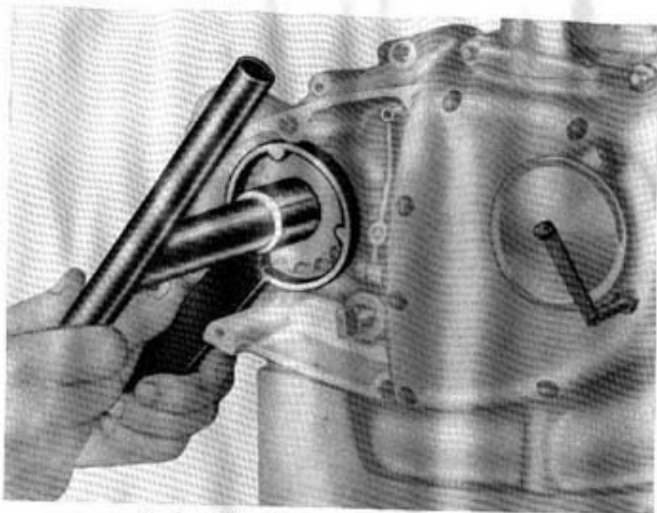
5 - Gear-holding key for tightening the pinion nut
