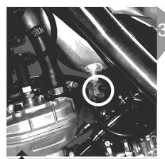
The fuel tap should be in a vertical position for normal working. Forwards, reserve; downwards, the supply valve is open; and towards the rear, the valve is closed.
