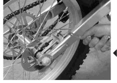
To eliminate any air trapped in the brake circuit, the shoes are fitted with air bleeds.
