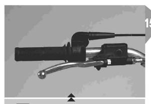
9) The throttle should be cleaned and oiled regularly especially after washing the motorbike with water at highpressure.
