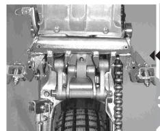
Periodically, the joints of the lower part of the rear suspension should be cleaned, the adjustments checked, and lubricated.
