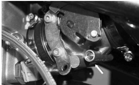
The throttle body has an idling regulation screw (arrow) that acts on the air channel in the by-pass.
