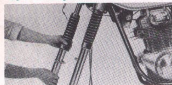
Fig. 5-27. Installing the front fork into the steering
