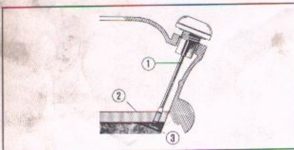
① Level gauge ② Upper limit ③ Lower limit Fig. 4-74. Oil level
