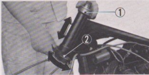
① Steering head top thread ② Steering stem Fig. 5-37. Check of stem operation
