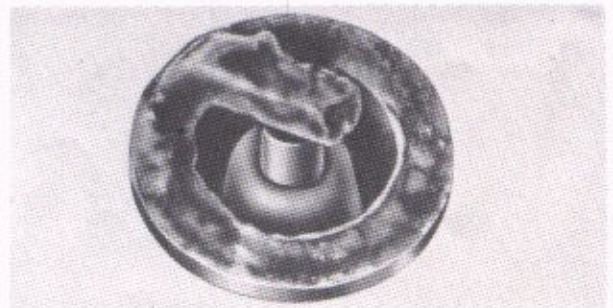
Fig. 6-24. Sooty condition (dry)
