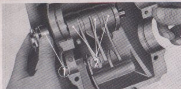
① Gear shift drum ② Gear shift forks Fig. 4-113. Removing the gear shift drum
