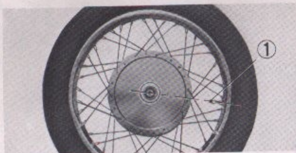
① Valve stem Fig. 5-89. Valve angle
