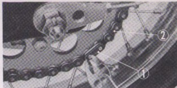
① Drive chain joint clip ② Drive chain Fig. 5-126. Removing the drive chain joint
