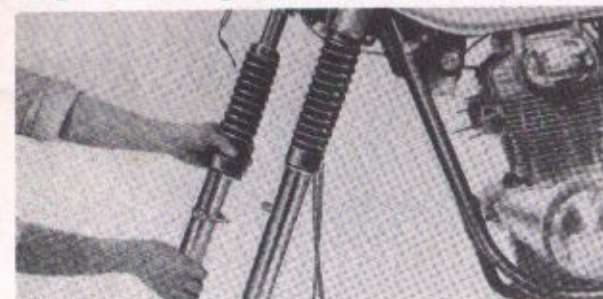
Fig. 5-27. Installing the front fork into the steering
