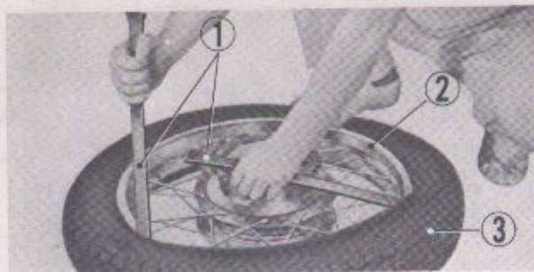
① Tire lever ② Rear wheel rim ③ Rear wheel tire Fig. 5-131. Removing the rear wheel tire
