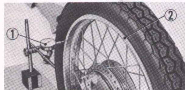
① Dial gauge ② Front wheel rim Fig. 5-84. Measuring rim runout
