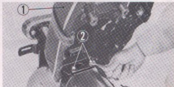
① Seat ② 8 mm hex. nuts Fig. 5-51. Removing the seat
