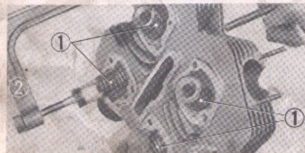
① Valve springs ② Valve assembly and disassembly tool Fig. 4-16. Removing the valve
