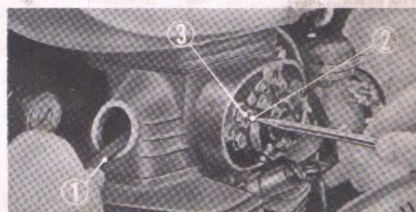
① Thickness gauge ② Rocker arm pin
