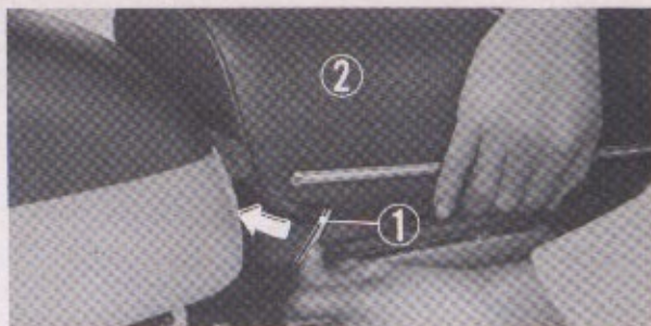
① Seat latch lever ② Seat Fig. 5-50. Unlatching the seat latch lever
