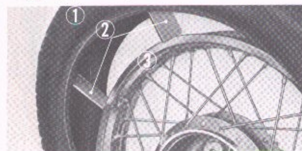
① Rear wheel tire ② Wood spacer piece ③ Rear wheel rim Fig. 5-134. Inspecting the inside of tire
