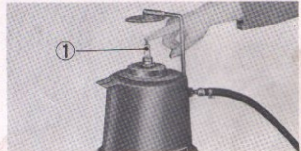
① Spark plug Fig. 6-27. Spark plug cleaning
