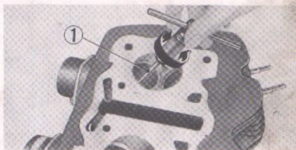
① Reamer Fig. 4-36. Performing reaming
