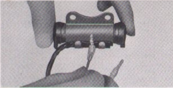
Fig. 6-20. Short-circuiting of the condenser
