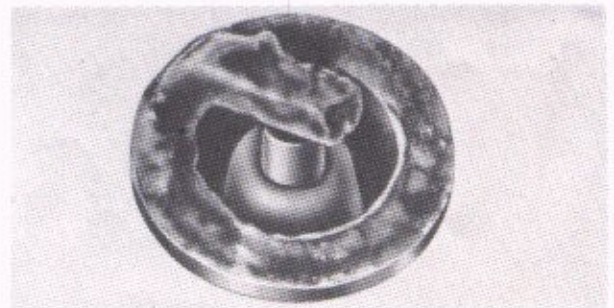
Fig. 6-24. Sooty condition (dry)
