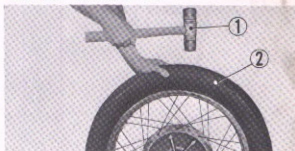
① Wooden hammer ② Front wheel tire Fig. 5-88. Tapping around the tire
