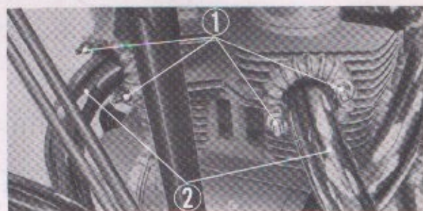
① 6 mm hex. nut ② Exhaust pipe Fig. 5-59. Installing the exhaust pipe
