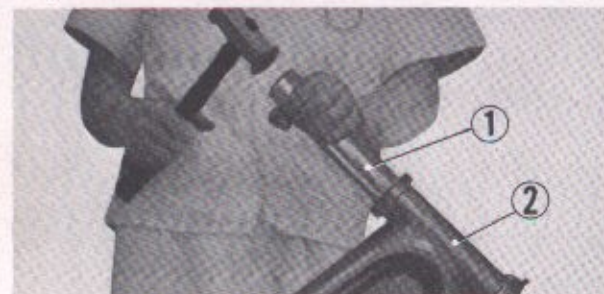
① Wooden drift ② Head pipe Fig. 5-47. Removing the ball race
