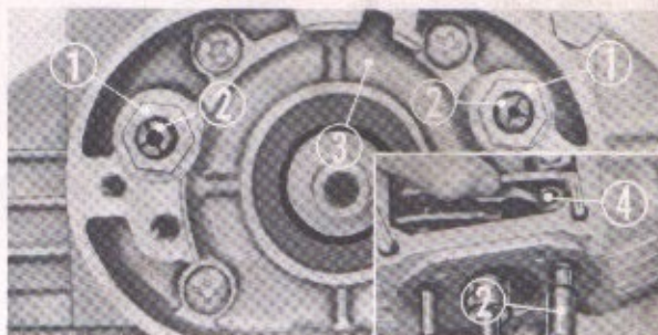
① Rocker arm pin lock nuts ② Rocker arm pins ③ Side cover ④ Rocker arm
