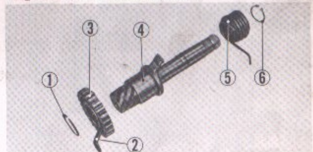
① 25 mm circlip ② Friction spring ③ Kick starter pinion ④ Kick starter spindle ⑤ Kick starter spring ⑥ 18 mm circlip Fig. 4-120. Component parts of kick spindle
