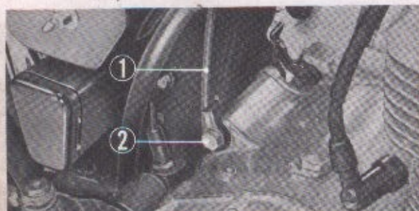
① Battery ground cable ② Engine hanger bolt Fig. 4-5. Installing the battery ground cable
