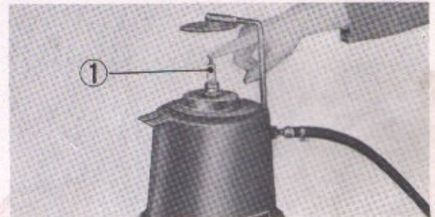
① Spark plug Fig. 6-27. Spark plug cleaning
