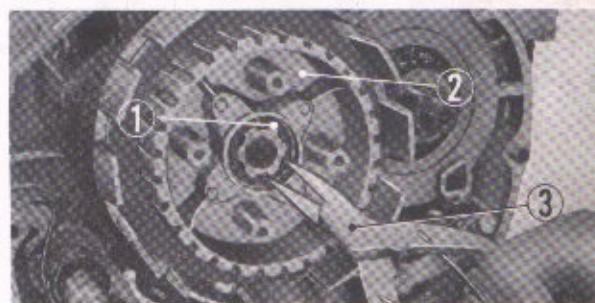
① 25 mm circlip ② Clutch center ③ Pliers Fig. 4-70. Removing the clutch center
