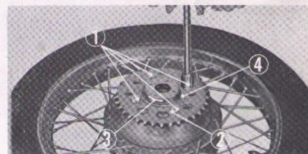
① 10 mm thin nuts ② 10 mm tongued washer ③ Final driven sprocket ④ 69 mm external circlip Fig. 5-128. Removing the final driven sprocket
