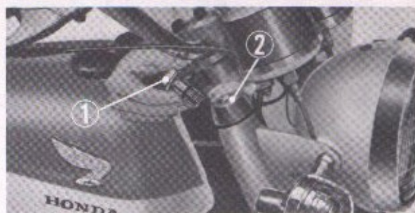
① Front fork bolt ② Oil filler opening Fig. 5-21. Removing the front fork bolt
