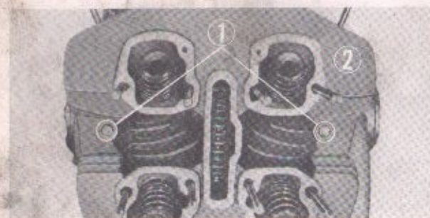
① 6 mm hex. bolts ② Cylinder head Fig. 4-15. Removing the cylinder head
