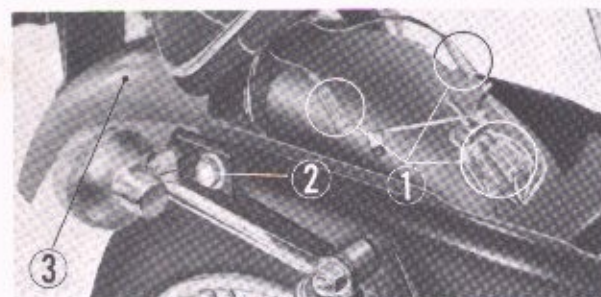
① Lead connector ② Rear winker setting bolt ③ Rear fender Fig. 5-65. Removing the rear fender
