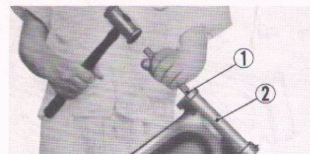
① Ball race driving tool ② Head pipe Fig. 5-48. Driving the ball race
