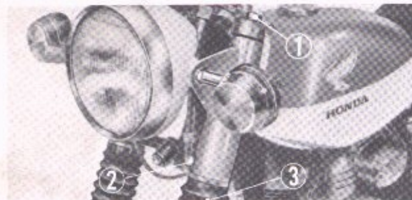
① Front fork bolt ② 8 mm hex. bolt ③ Front fork assembly Fig. 5-18. Removing the front fork assembly
