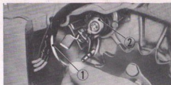
① Neutral lead connection ② Neutral switch Fig. 4-92. Removing the neutral lead connection
