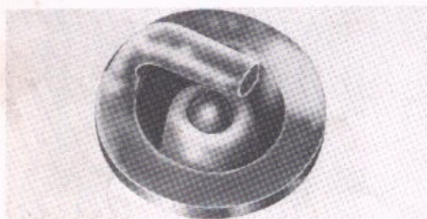
Fig. 6-23. Excessively burnt condition
