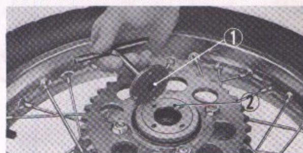
① Bearing retainer tightening wrench ② Bearing retainer Fig. 5-129. Removing the bearing retainer
