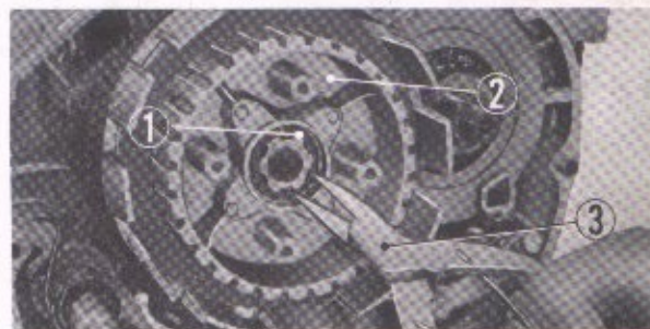
① 25 mm circlip ② Clutch center ③ Pliers Fig. 4-70. Removing the clutch center
