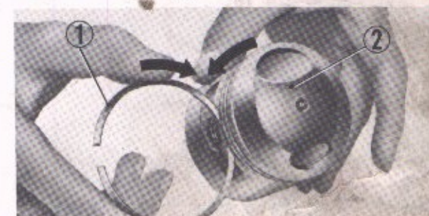
① Piston ring ② Piston Fig. 4-54. Rolling the piston ring in the piston groove
