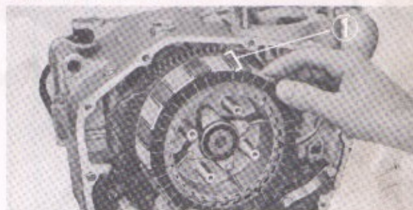
① Clutch plate and friction disks Fig. 4-69. Removing the clutch plates and friction disks
