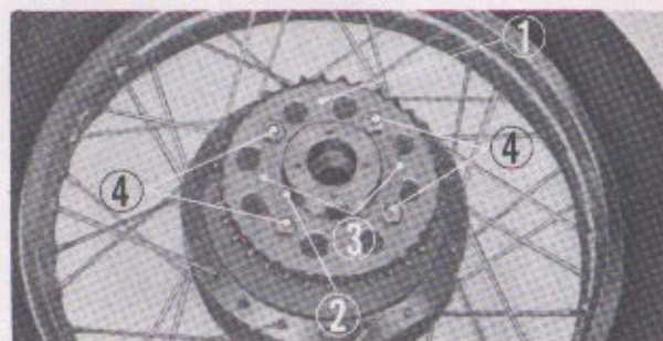
① Final driven sprocket ② 69 mm external circlip ③ 10 mm tongued washer ④ 10 mm thin nut Fig. 5-136. Assembling the final driven sprocket
