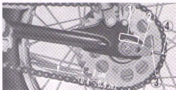
① Reference mark ② Drive chain adjuster ③ Lock nut ④ Drive chain adjusting bolt Fig. 5-139. Adjusting slack of drive chain
