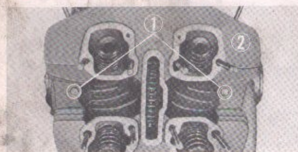
① 6 mm hex. bolts ② Cylinder head Fig. 4-15. Removing the cylinder head
