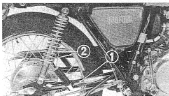
Fig. 2-14 ① Rear fork ② Rear shock absorber
