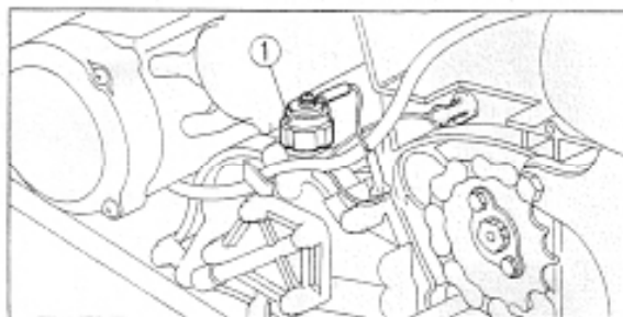
Fig. 5-43 ① Oil pressure control switch
