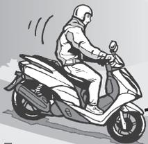
Close the throttle and apply the front and rear brakes together.
