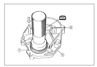
Apply SUPER GREASE A to the lip of the oil seal
