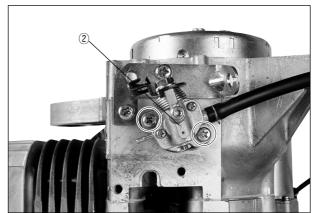
● Install the reed valve gasket ①, intake pipe gasket ② and intake pipe ④ with reed valve ③ to the crankcase.
