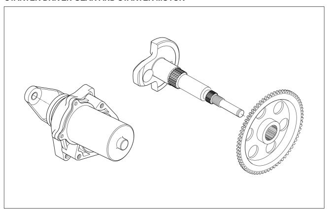
● Install the starter driven gear ① over the left crankshaft end.
