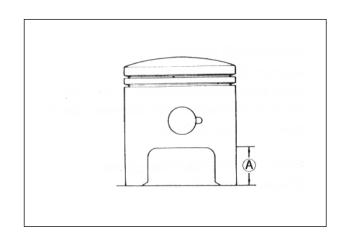
As a result of the above measurement, if the piston-to-cylinder clearance exceeds the following limit, overhaul the cylinder and use an oversize piston, or replace both cylinder and piston. The measurement for the bore diameter should be taken in the intake-to-exhaust port direction and at 20mm from cylinder top surface.
