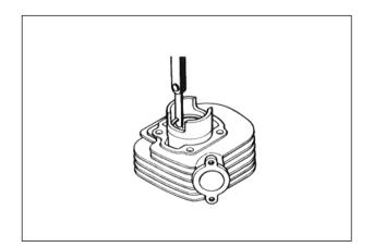
As the piston ring wears, its clearance increases reducing engine power output because of the resultant blow by through the enlarged clearance. Here lies the importance of using piston rings with the clearance within the limit.
