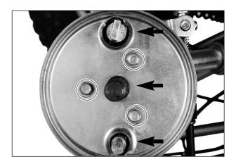
• Install the front brake drum and tire.
