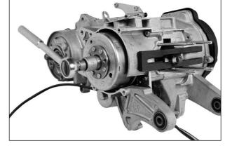
Remove the magneto rotor with the special tool.
