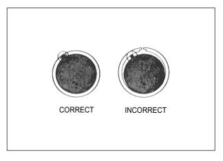
Apply engine oil on the piston pin and install the piston to the conrod.
