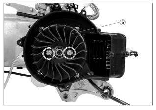
• Install the cooling fan cover ① .
