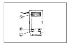
• Remove the bearing © with the special tool.
