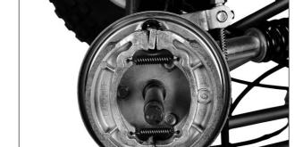
Remove the brake cam lever.
