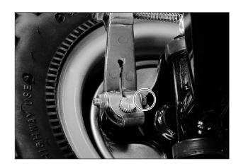
Remove the front brake plate.
