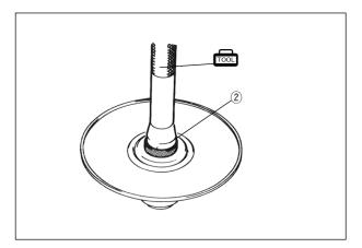
● Install the new oil seals (④, ⑤) to the movable driven face ③ with the special tool.
