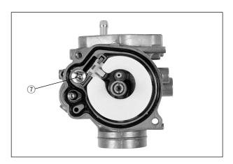
• Install the thermoelement assembly.
