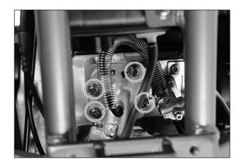
• Disconnect the oil hose from the oil pump.
