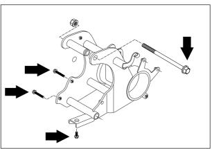
Remove the sprocket mounting flange by removing the nut.
