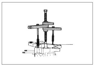
• Remove the crankshaft with the special tool.
