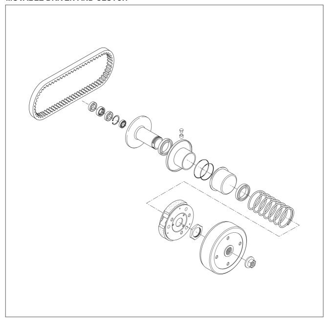
● Install the bearing ② in the fixed driven face ① with the special tool.
