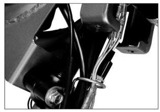
Remove the steering head cover bracket and handlebar by removing the mounting bolts.
