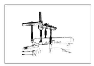
Remove the bearings, oil seals and bushing.
