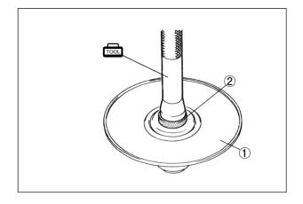
• Install the circlip ①.
