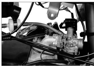
■ Remove the carburetor by loosening the mounting bolts ④ .
