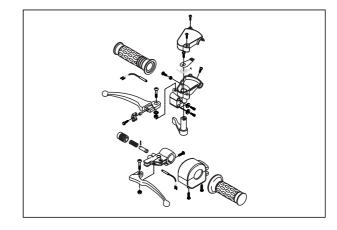
Remove the front brake cables.
