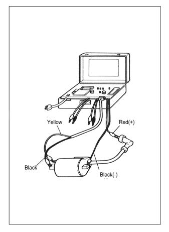
• Check the ignition coil with the pocket tester.
