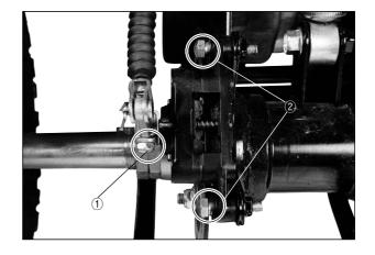
Remove the rear caliper lever return spring .
