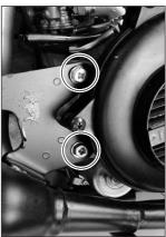
• Remove the engine ground lead wire ①.
