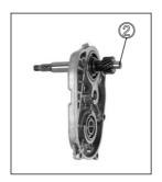
● Apply **BOND 1215** at the hatched area shown in the illustration and install the gear box cover ③ on the crankcase.
