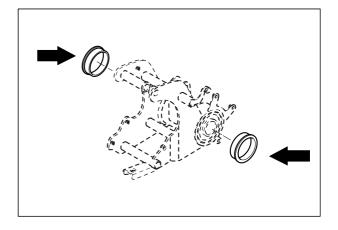
Remove the right and left bearings and spacer.
