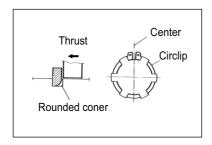
Install the new bearing ⑦, ⑧ to the gear box cover⑨ with the special tool.
