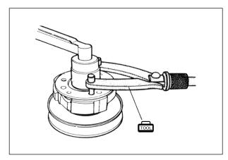
• Insert the V-belt between the driven faces as deep inside as possible while pulling the movable driven face all the way outside to provide the maximum belt clearance.
