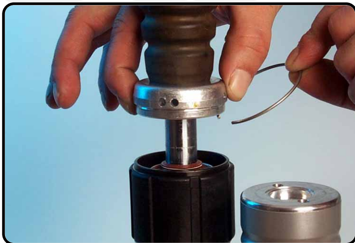
Assemble the springring.
