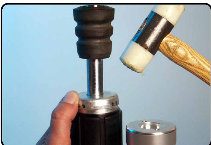
Tap the cap into the tube.
