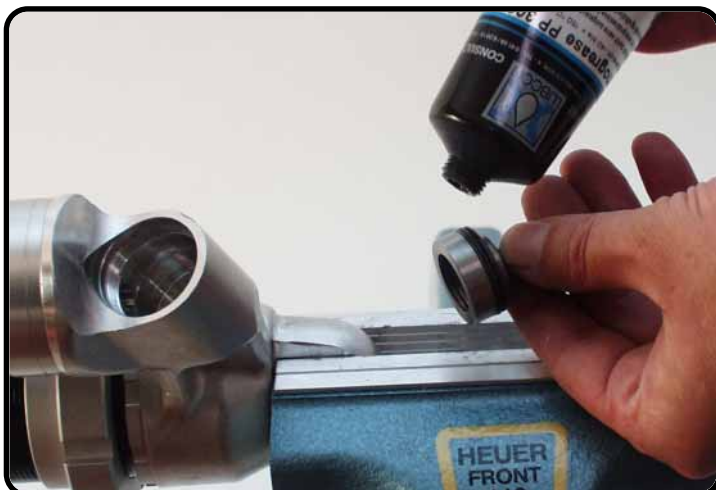
Wet the O-ring of the piston MCC with T158.
