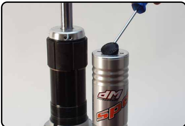
Disassemble the rubber cap.
