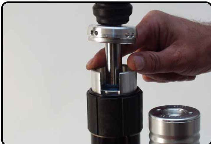
Push the adaptor DU-bush downwards.
