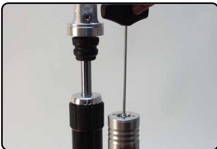
Unscrew slowly the nitrogen plug (size 4) to release the pressure.
