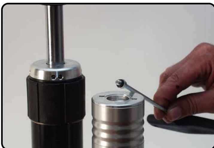
Nitrogen plug with O-ring.
