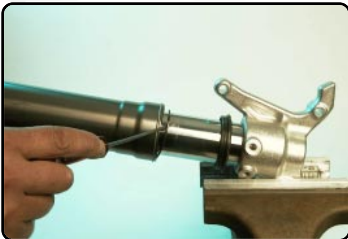
Disassemble the circlip.
