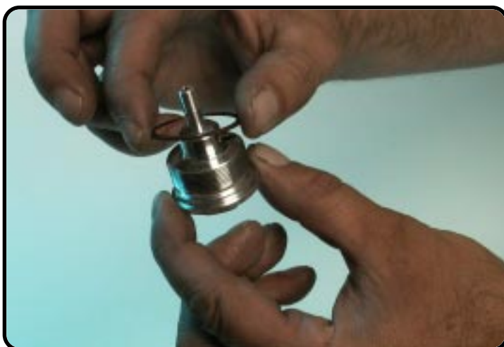
Remove the copper washer.
