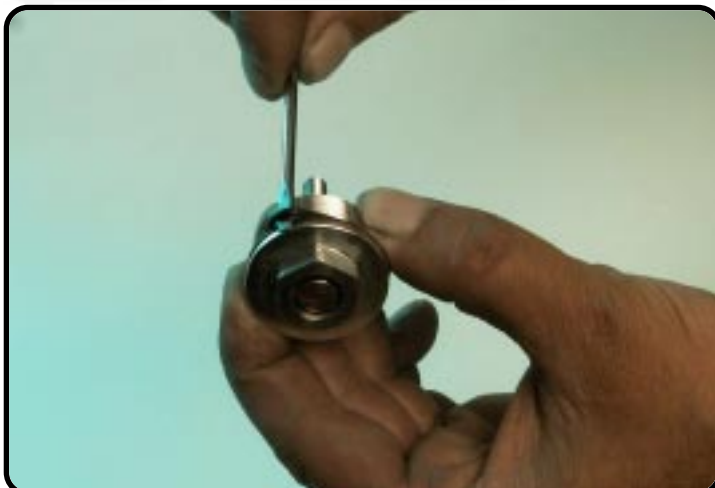
Disassemble the O-ring.
