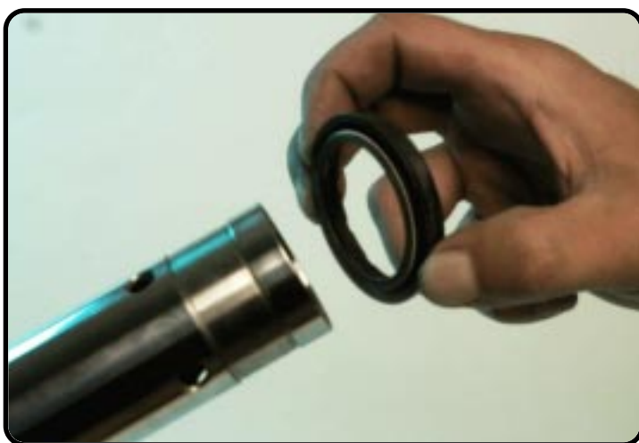
Remove the dust wiper.
