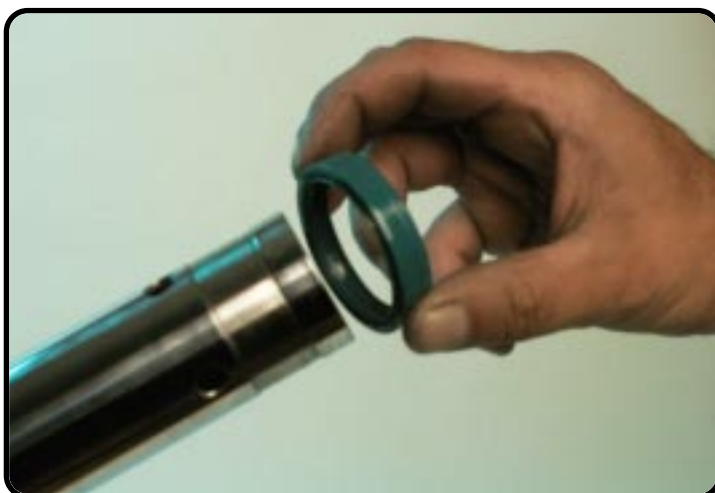
Disassemble the oilseal. Pay attention to the assembling direction!!!
