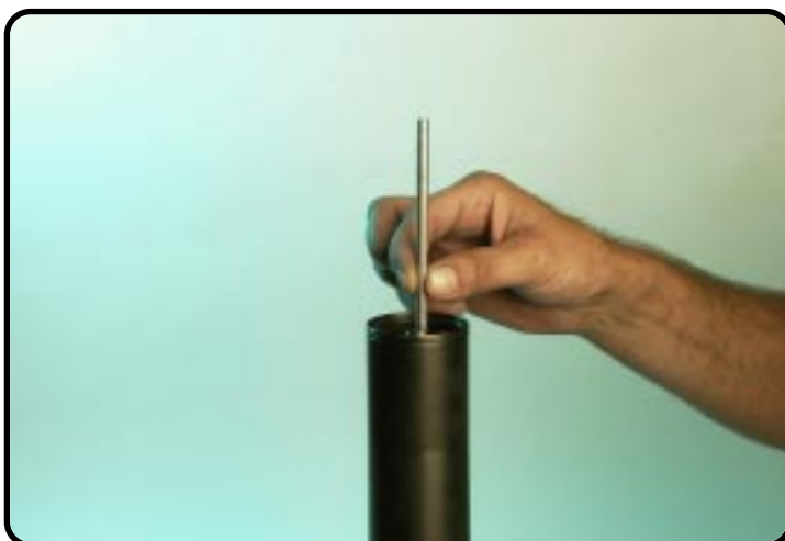
Remove the adjustment tube with the O-ring.
