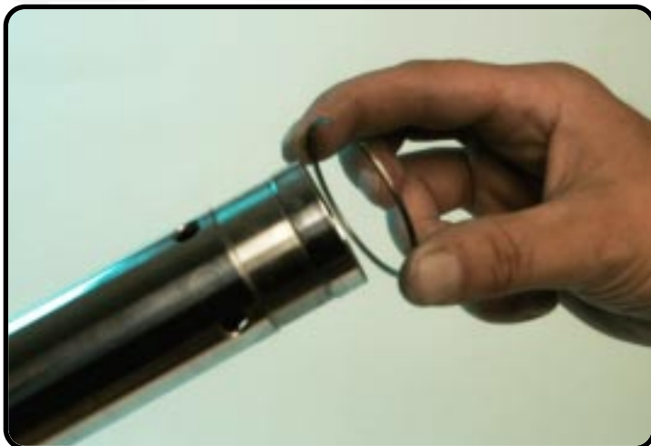
Remove the circlip.
