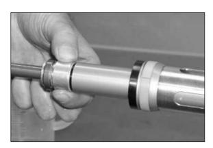
Screw on the screw bushing.
