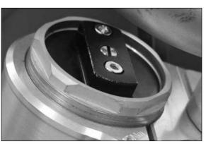
NOTE: The maximum riding height is the level of the second groove!
