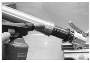
– Heat the surface of the outer-tube near the oil seal to a temperature of  $\pm~50^{\circ}\text{C}.$
