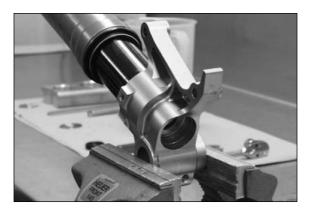
Remove the closed cartridge 2 complete.
