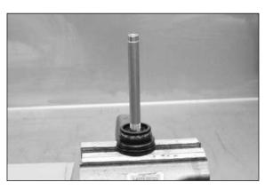
Place the screw-cap in the vice according to the picture.
