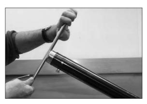
Loosen the inner-tube.
