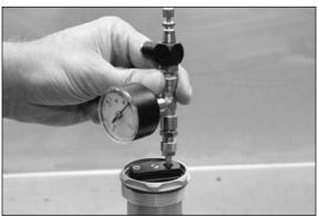
Remove the protecting cap 6 of the needle and stick the needle through the middle of the filling rubber plug.
