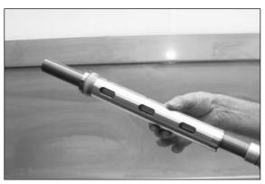
Slide the tube on the tube of the cartridge. Pay attention to the assembling direction!
