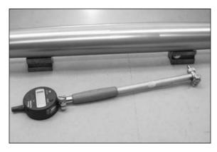
Micrometer for measuring the diameter of the running surface of the outer-tube.
