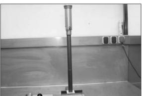
Clamp the tube in the clamping block at the level of the screw sleeve.
