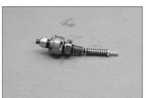
Assemble the adjustment needle in the tap rebound.
