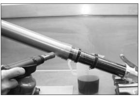
Heat the outer-tube to a temperatur of approx. 50°C at the level of oil seal chamber of the outer-tube.
