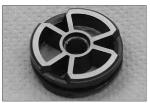
Compression piston, check-valve setting side shown.
