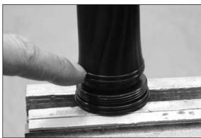
Assemble the membrane in the groove of the screw-cap.
