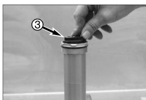
Screw the screw-cap in the membrane holder 3.
