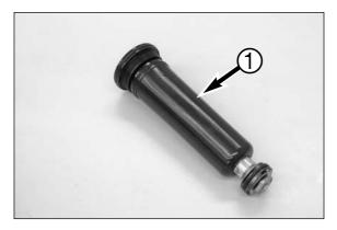
If the membrane • does not have the right shape (see photo), open the membrane at the groove in the screw cap and press the membrane into the right shape with a small amount of compressed air
