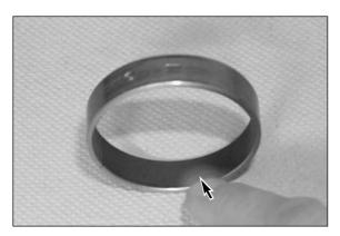
Replace the DU-bush of the outer-tube if the surface is feeling rough.
