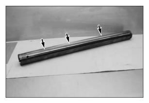
Inspect the outside running surface of the inner-tube on scratches, wear and tear.
