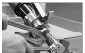
Screw the rebound adjustment holder from the nut, (Size 19 and
