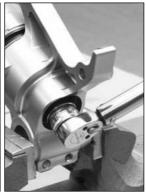
Screw the rebound adjustment adaptor 6 into the axle-clamp and tighten it to a torque of 30 Nm.
