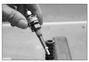
Screw the tap rebound with needle and spring out of the piston rod.
