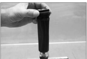
Screw the membrane on the tap compression.
