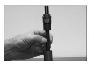
Pull the piston rod out of the tube.
