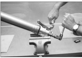
Tighten the rebound adjustment adaptor against the contra nut 2 to a torque of 30 Nm.
