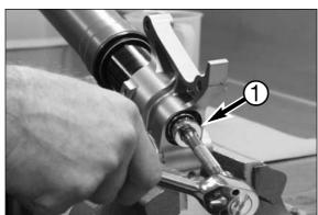
Unscrew the rebound adjustment holder • out of the axle-clamp, (Size 19).
