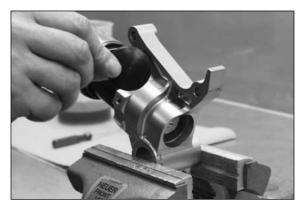
Remove the rubber cap out of the axleclamp.
