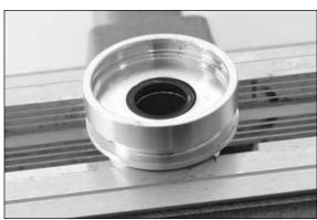
Assemble in correct order the back-up rings and quad ring!!! See \_ disassembling.
