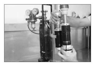
Close the tap and pull the Allen key of the nitrogen charging device out of the nitrogen filling plug.
