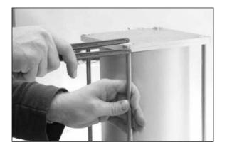
Place the oil reservoir on the front lid and remove the nuts from the rear lid using tool T103. Hold the threaded rod while unscrewing the nuts, to avoid the rods from piercing the front sticker of the oil reservoir.
