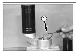
– Remove the O-ring  ${\ensuremath{\bullet}}$  inside the shock absorber housing out of the groove.
