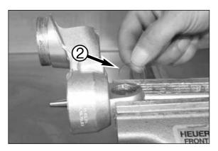
– Disassemble the other spring ring **2**.
