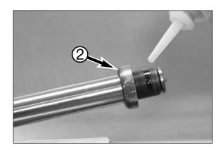
Wet the thread of the piston rod with T 132.
