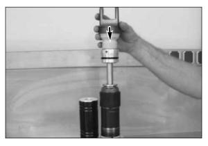
Assembling the shock absorber - Assemble the piston rod "complete" into the tube.
