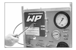
Place back the filling plug using a torque wrench. The filling plug \_ has to be fastened with a torque of 10 Nm.
