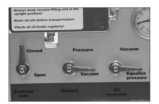
As soon as the pressure has been reached, the lever damper can be moved to the Vacuum position.
