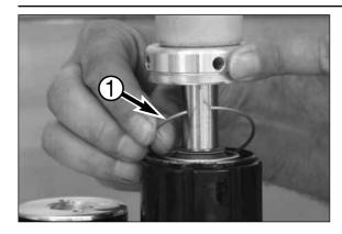
– Assemble the spring ring  ${\ensuremath{\bullet}}$  first with the closed side into the groove.
