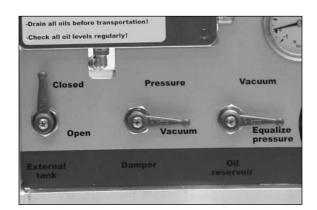
When the pressure gauge has reached 0 bar, the lever Damper can be moved to Pressure.
