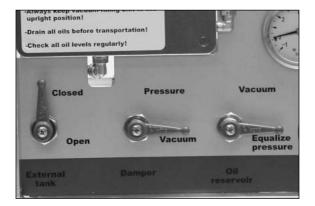
As soon as the vacuum gauge reaches the specified pressure, in this example 4 mbar, the lever Oil reservoir should be moved to Pressure equalize.
