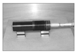
Measure the inner diameter at both ends and in the center of the pipe.
