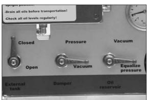
When the correct pressure has been set, press knob of pressure regulator down and release the pressure by moving lever Damper to the Vacuum position.
