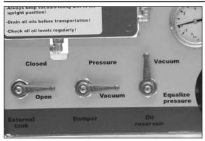
When the pressure gauge reaches 0 bar, the lever Oil reservoir can be moved to Vacuum and the lever External tank must be moved to Open position, this will start the 2nd cycle of vacuum.
