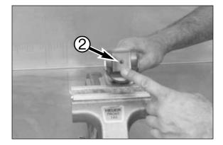
Assemble the rubber plug 2 into the mounting fork.
