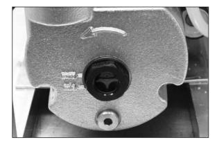
The oil level of the vacuum pump should never exceed max level and should never be lower than the min level. Keep the oil level close to the max level to ensure good function and cooling of the pump.
