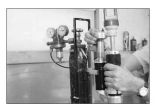
Place the shock absorber in the Nitrogen charging device and ensure that the Allen key is fitting in the nitrogen filling plug.
