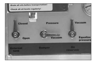
This will start the forcing of oil into the damper, you will see the pressure gauge move to the pressure that has been set earlier, in this case 3 bar.
