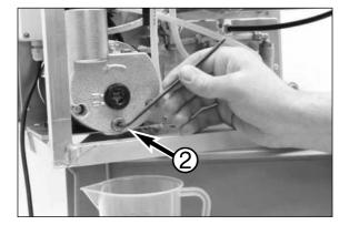
For draining the vacuum pump-oil, unscrew the draining plug 2 and let the oil flow into a measuring cup. When the oil is drained, place back the draining plug.
