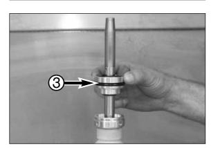
– Slide carefully the adaptor DU-bush  $\ensuremath{\mathfrak{G}}$  over the tool on the piston rod.
