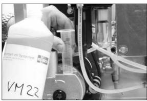
Fill up the vacuum pump with oil to the max. level on the level indicator. Only use Busch Vm22 vacuum pump oil! Place back the \_ filling plug.
