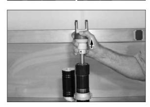
Pull careful but firmly the piston rod "complete" out of the tube.
