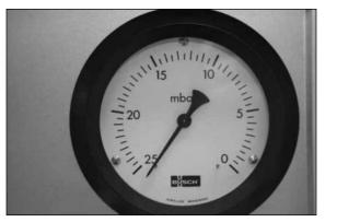
As soon as the pressure reaches 25 mbar the vacuum gauge will also start moving to a lower pressure.
