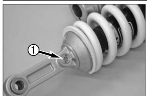
Adjusting the position of the compression and rebound damping Rebound damping:
