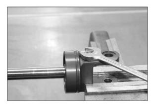
Unscrew the screw cap ① of the rebound adjustment.
