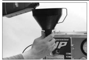
Fill the oil reservoir until the level indicator reaches max. level. \_ Place back the filling plug using a torque wrench. The filling plug has to be fastened with a torque of 10 Nm. The vacuum-filling unit should always be in the upright position, to avoid oil spreading trough the entire system! This will cause serious damage to the vacuum filling device. Only use oil approved by WP Suspension!
