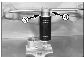
– Screw the nitrogen reservoir on the shock absorber housing and tighten it with T 145S 0 and T 125S 0.
