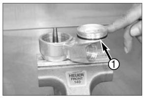
– Place the new O-ring  ${\color{black}\bullet}$  in the groove of the shock absorber housing.
