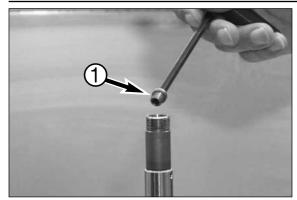
Remove the seat ① - does not apply to SXS/SMR
