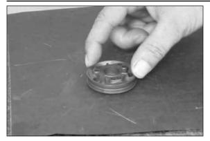
Polish the surface of both sides of the pistons on a flat plate with sandpaper 600.
