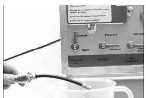
Let the oil run out of the reservoir. When there is no more oil flowing, disconnect the filling adapter.
