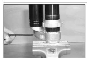
Unscrew the oil filling plug for about two turns. (size 5) This wil help you later by removing the piston rod "complete" out of the shock absorber!
