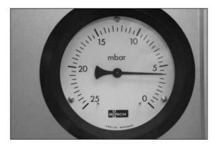
As soon as the vacuum gauge reaches the specified pressure, in this example 4 mbar the lever External tank should be moved to Closed position and the lever Oil reservoir should be moved to Equalize pressure.
