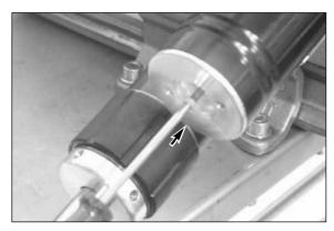
Push the separation piston with T 107S to the correct position, the O-ring must have a distance for about 10 mm from the screw cap.
