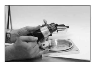
Grease the O-ring of the rear lid with special O-ring grease (PP300) T158.
