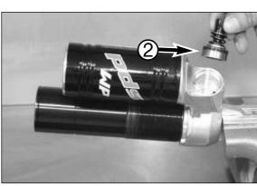
Turn the oil filling plug ③ out of the shock absorber housing (AH, Größe 5).
