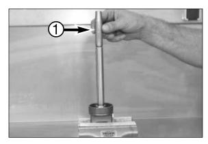
– Place assembling tool T 1215  ${\ensuremath{\textcircled{}}}$  on top of the piston rod.
