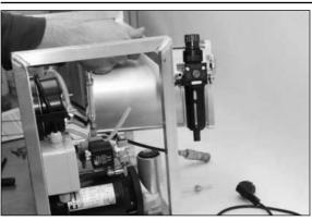
The oil reservoir can now be taken out of the frame trough the backside of the installation. Guide the damper connector pipe to avoid kink.
