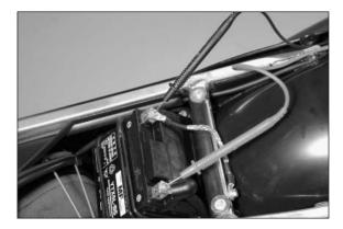
**Regulator rectifier output** – measure the voltage with the measuring leads of the peak voltage adapter 584.29.042.000 directly on the poles of the vehicle battery:
