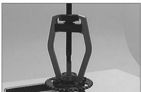
Use the puller tool 590.29.033.000 to extract the grooved ball bearing <sup>(G)</sup> from the camshaft (see photo).
