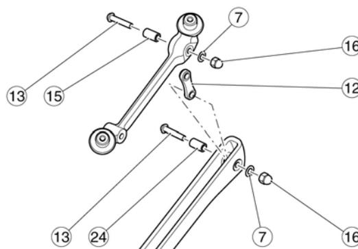
**Locking torques (N\*m)****M6 Electric windshield supports retainer 12 Nm**
