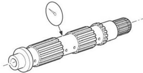
Check transmission gears for signs of pitting and wear and replace damaged gears if necessary.
