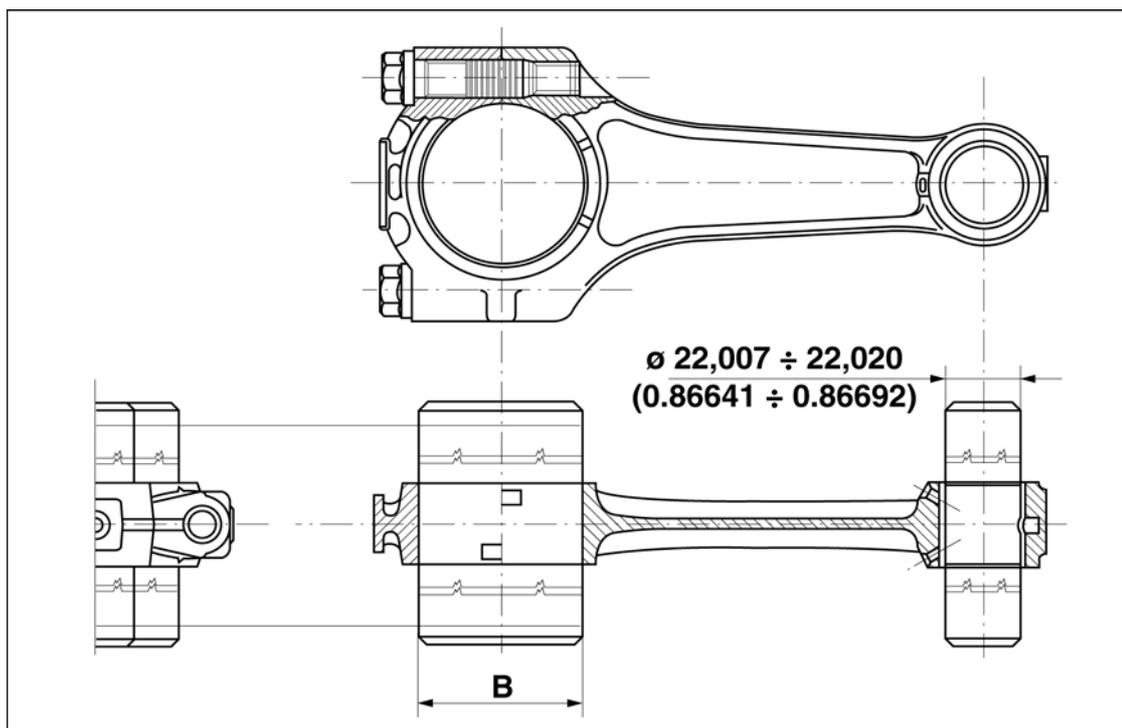
**CONNECTING ROD BEARING THICKNESS**
