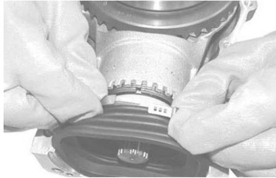
Screw the clamp with the specific pliers.
