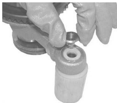
Remove the sealing rings (2) and (7) with a screwdriver.
