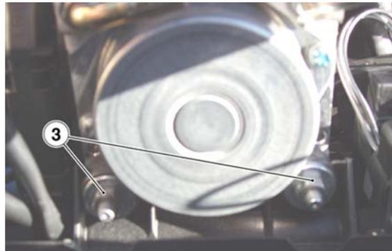
The braking system must be purged every time 'sponginess' is found in the main system, i.e. outside the ABS control unit. In this occurs, purge the system as usual. If air has stopped in a pipe section between the control unit and the front callipers, try to make it go out the reservoir by extending the brake callipers plungers. The four nipples (1 - 2) in the ABS control unit should be unscrewed only when the unit is replaced.
