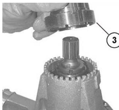
Assemble the sealing ring (3) to the ring nut (2) with the buffer CA715855 (see F.1) and a hammer.
