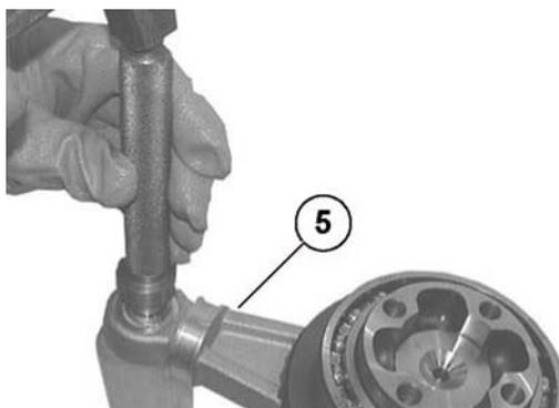
Fit the stop ring (3) in the support (5) with suitable pliers.
