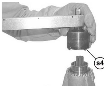
Remove the ring nut (2) and remove the sealing ring from the ring nut.
