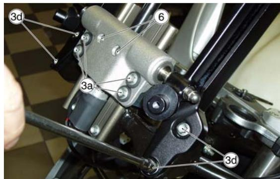
To carry out the tightening, proceed as follows and remember to make sure that after being lifted, the plate (5) always comes down freely (without being forced):
