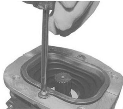
Fit the cap with the washer.
