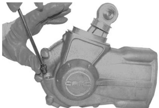
Assemble the cap with the clamps.
