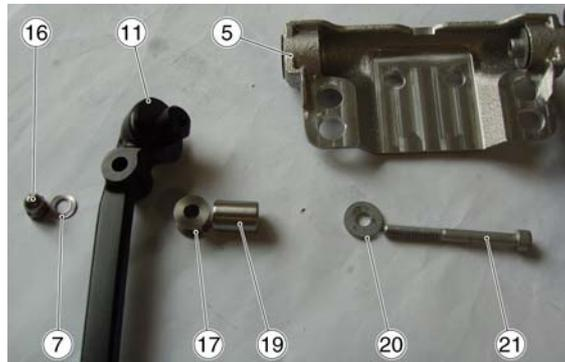
**Locking torques (N\*m)****M6 Electric windshield supports retainer 12 Nm**
