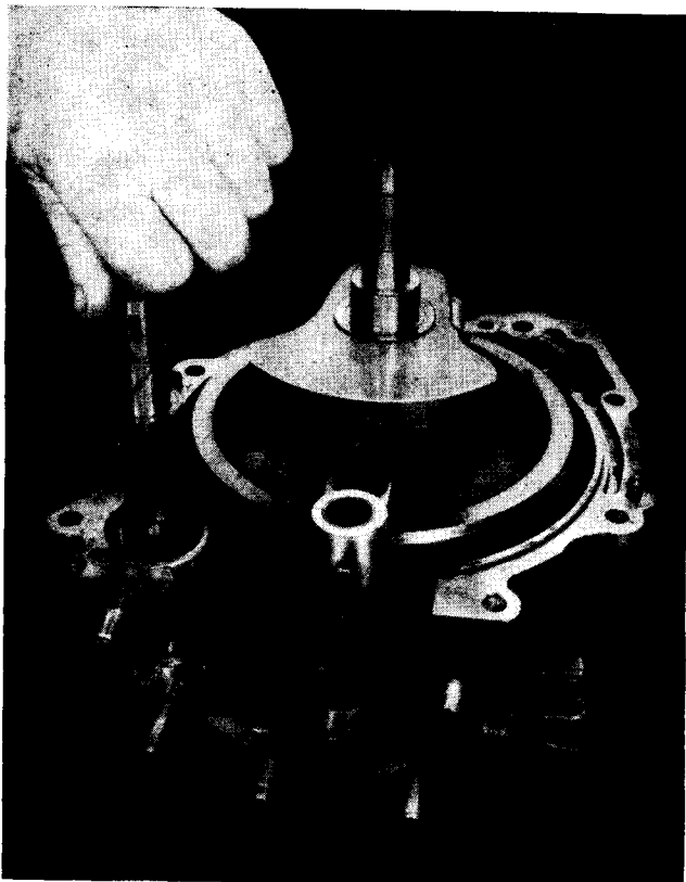
FIG. 16 Extracting the Camshaft
