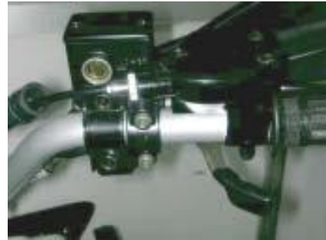
Acceleration cable/ Front & rear brake lever pivot
