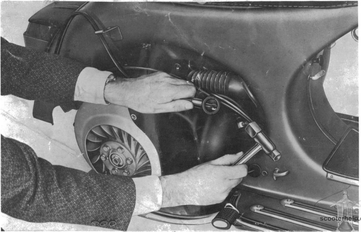
Fig. 15 - Dismantling spark plug
