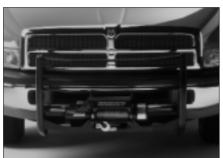
Warn Winch and Mounting Kit (shown on Ram Pickup)
