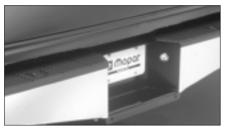
Drop-style Step Bumper with Hitch Ball (shown on Ram Pickup)
