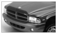
Bug Deflector with Fender Shields (shown on Durango)
