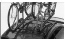
Permanent Roof Rack (shown on Neon)
