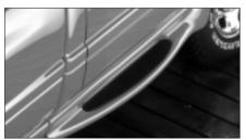
Molded Side Step with Ground Effects on Regular Cab (shown on Ram Pickup)
