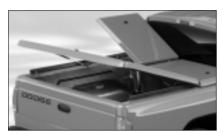
Gull Wing Style Tonneau Cover (shown open on Dakota Quad Cab™)
