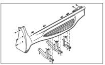
Side Step with three-bracket support per side
