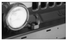
Tow Hooks mounted on OE bumper (shown on Wrangler)
