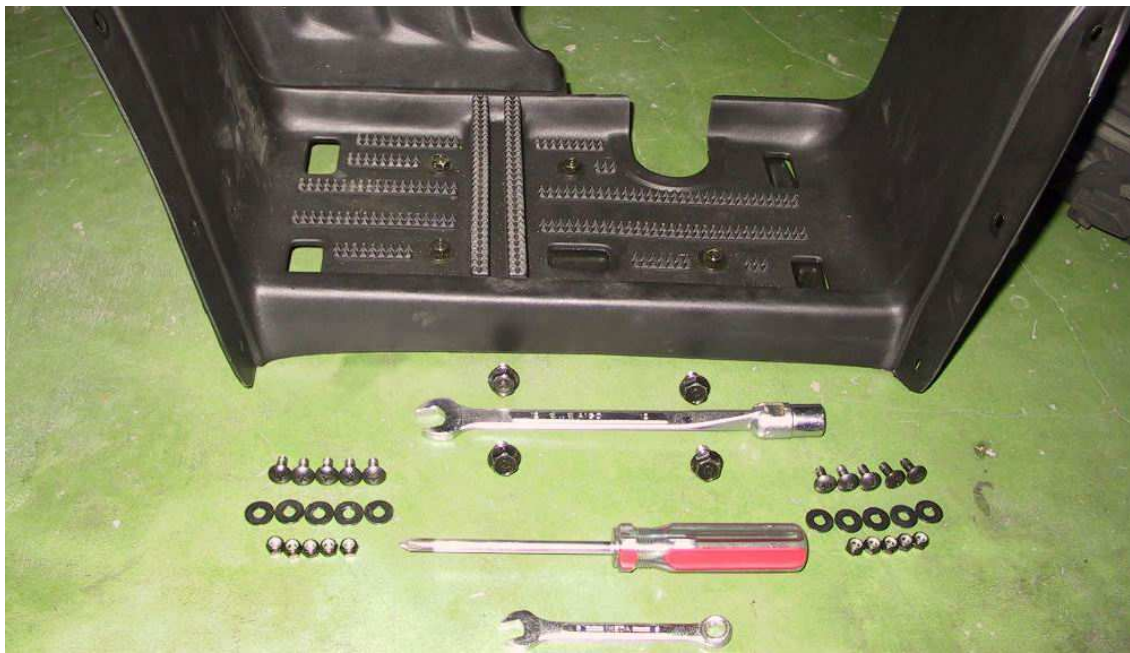
STEP.1) Take off the right side footwell for adjustment.
