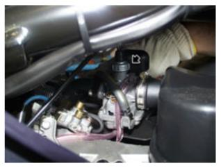
Remove the gas cable from the carburettor.
