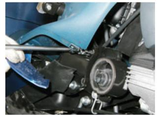
Working from the left, unscrew and remove the nut (2).
