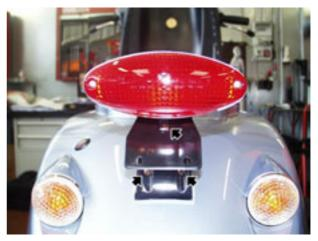
Unscrew and remove the rear fixing bolt for the engine cowling.
