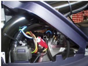
Release the clamp and disconnect the fuel supply piping.
