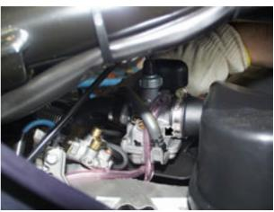
• Release the clamp and disconnect the vacuum pipe
