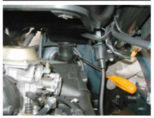
Unscrew and remove the four fixing screws for the tank.
