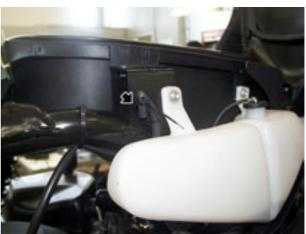
Remove the battery, fuel tank, and carburettor breather pipes from the guide eyelet.
