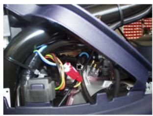
Release the hose clamp that fixes the carburettor to the filter casing.
