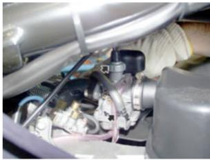
• Remove the gas cable from the carburettor.
