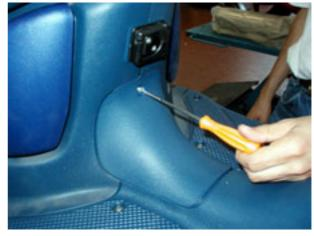
Working on both sides, unscrew and remove the four lower fixing screws for floor panel.
