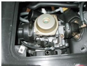
Release the clamps and disconnect the fuel supply and vacuum pipes from the fuel pump.
