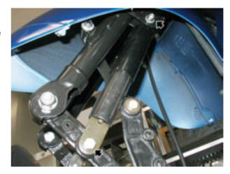
To proceed with removing the fork, remove the superstructure.
