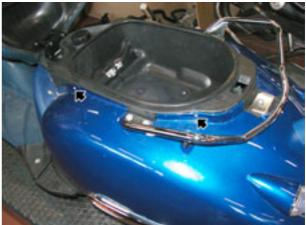
Working on both sides, unscrew and remove the two fixing screw for the front engine cowling.
