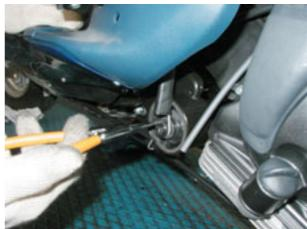
Unscrew and remove the rear fixing screw for the left underpanel.
