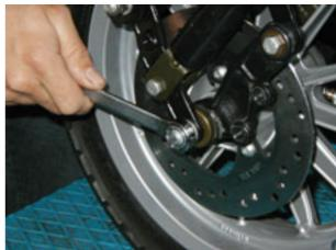
Take note of the position of the speedometer transmission in order to be able to refit it correctly.
