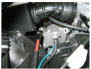
• Disconnect the spark plug cap.
