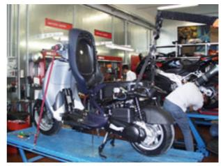
Unscrew and remove the lower bolt that fixes the shock absorber to the engine.
