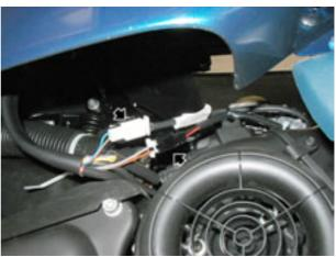
Release the clamp on the carburettor and disconnect the fuel pipe.
