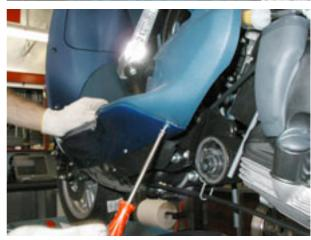
Unscrew and remove the lower fixing screw for the silent-block support plate
