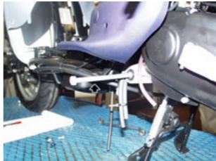
• Remove the engine, complete with the central stand and rear wheel.
