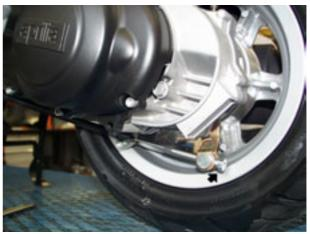
Unscrew the screw (1) and remove the brake cable seal hose clamp.
