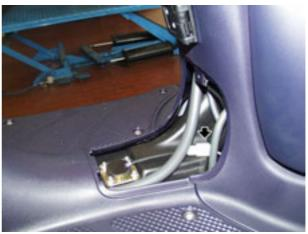
Release the retention hose clamp and remove the fuel tank breather pipe.
