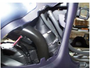
Unscrew and remove the four fixing screws for the tank
