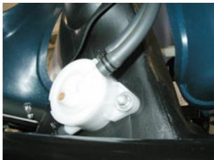
Release the lower hose clamp on the upper tank.
