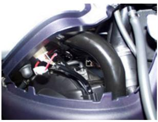
Release the clamp and disconnect the mixer oil pipe.
