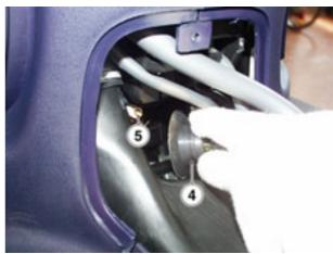
Disconnect the three connectors (pick-up, starter motor and power) from the ignition unit.
