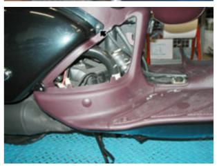
Unscrew and remove the two screws that fix the reflector to the support.
