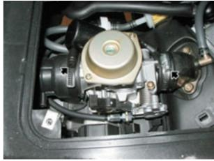
Disconnect the automatic starter and heater connectors
