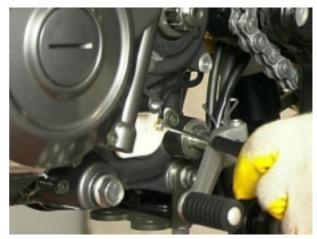
• Fit the cable guides and tighten the screw with washer.
