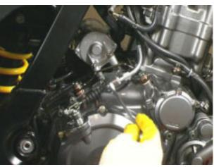
• Disconnect the clutch cable from its lever.
