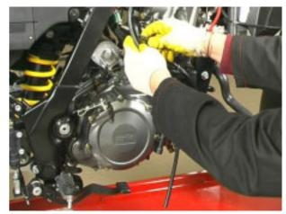
Connect the engine temperature sensor connector.
