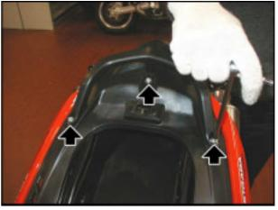
Working on either side, loosen and remove the front screw.
