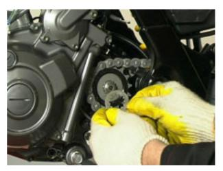
Remove the chain from the sprocket and remove the sprocket.
