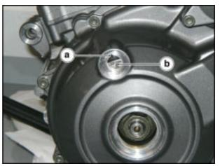
**NOTE** To set piston at TDC in the compression stroke, align reference "I" on camshaft gearwheel to the fixed reference on the cylinder head.
