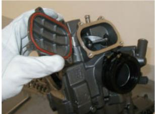
Loosen and remove the four screws and remove the exhaust tappet cover.
