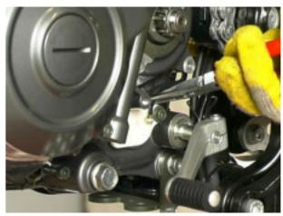
Loosen the ties and disconnect the tube from the air box.
