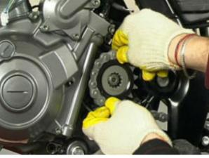
• Fit the safety washer and tighten the nut.
