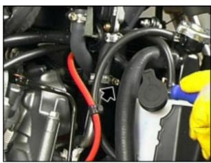
Slide out the tube from the throttle body.
