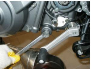
Loosen and remove the three oil filter cover screws.
