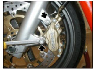
Unscrew the wheel shaft nut, collect the washer.
