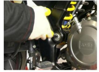
Set the ring nut to the centring bush and tighten it.
