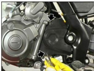
• Remove the sprocket cover.
