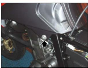
• Disconnect the fuel pump connector.
