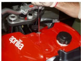
Release and remove the two side screws (one on each side).
