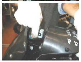
The right bracket stays on the vehicle because wiring is routed inside it. Release and remove the two outer screws.
