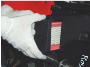
• Remove the air filter from its mount and clean the filtering element.
