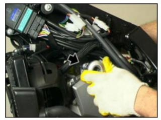
Loosen and remove the two lower screws, collect the washers.
