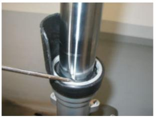
Unclamp the sleeve from the vice and remove the damper rod with bottom buffer.
