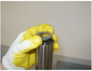
• Install the spring preload spacer.
