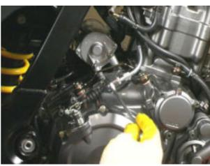
Connect the starter motor power cable.
