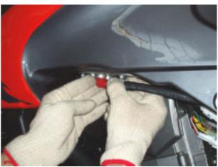
• Release and remove the fuel tank front screw.
