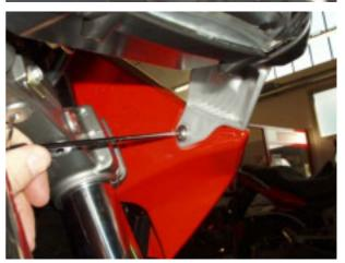
Unscrew and remove the outer screw.
