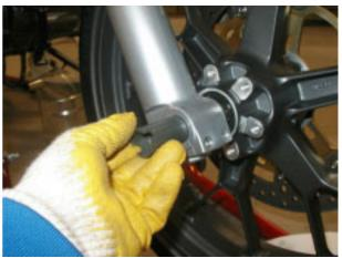
Support the stanchion and loosen the three screws securing stanchions to bottom yoke.
