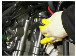
• Connect the clutch cable to its lever.
