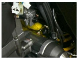
Loosen the nut and slide out the clutch cable from its housing.
