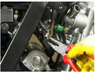
• Tighten the secondary air system tube tie.
