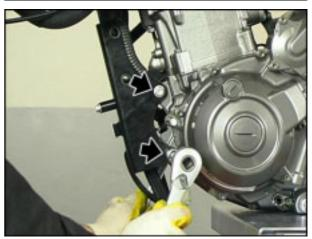
Remove the engine front support.
