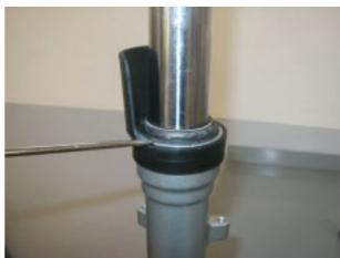
• Pull up the dust seal to remove it.
