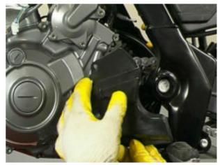
Fit and tighten the two screws with spacers.
