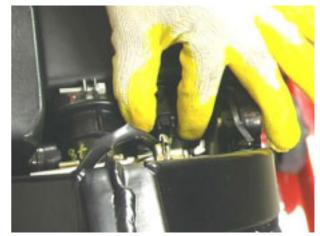
Fit the hose and tighten the clamp.
