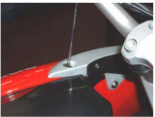
Release the headlight wiring connector.
