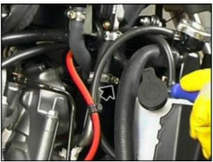
Connect the spark plug cap
