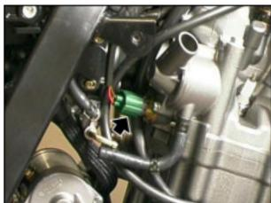
Fit the tube to the throttle body.
