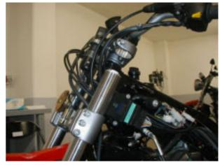
Take the stanchion in position and tighten the screw securing stanchion to top yoke.
