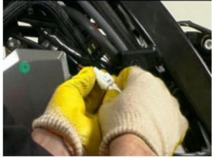
• Refit the clamp to fuel vapour recycle hose.
