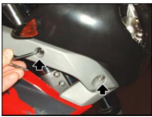
The left bracket stays secured to the headlight. Release and remove the two inner screws.
