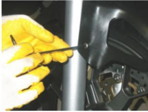
• Tighten the two mudguard shell screws.
