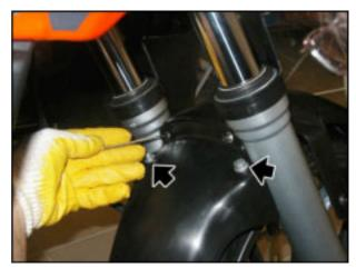
Working on either side, loosen and remove the screw securing the front mudguard shell.
