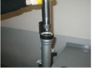
damper rod. Change any component which is badly worn or damaged.
