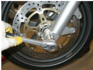
Working on either side, partially loosen the wheel shaft pinch bolts and completely loosen the wheel shaft.
