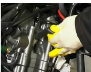
Loosen the secondary air system tube tie.
