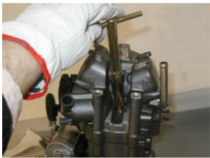
Release and remove the timing reference screw (3) and crankshaft screw (4).
