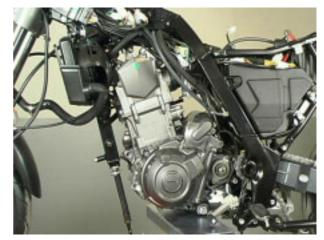
Set the throttle body in the intake manifold and tighten the clamp.
