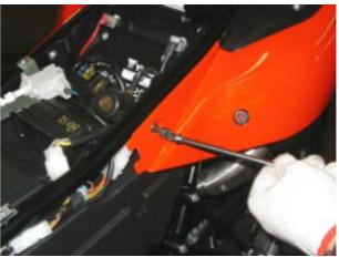
Working on either side, loosen and remove the top screw.
