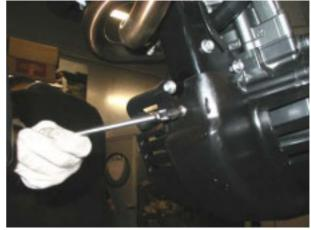
Release and remove the sump guard rear screw.
