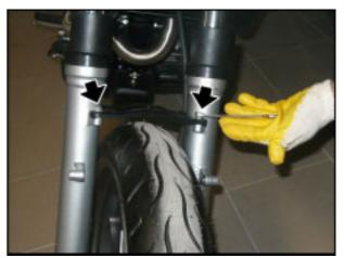
• Fit the rear mudguard shell and tighten the two screws.
