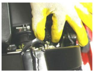
Remove the clamp from "fuel vapour recycle" hose.
