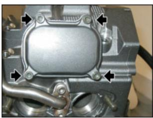
• Install the intake tappet cover and tighten the four screws.
