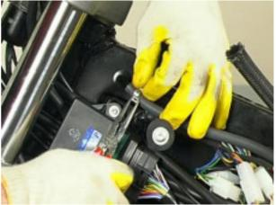
Remove the air box connector.
