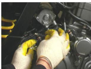
• Fit the clutch cable in its housing and tighten the nut.
