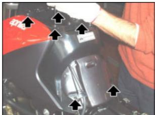
Release and remove the two screws on motor for opening the glove compartment, raise it and disconnect the connector.
