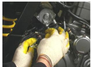
Disconnect the spark plug cap.
