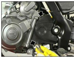
Fit and tighten the screw.
