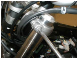
• Support the stanchion and loosen the three screws securing stanchion to bottom yoke.
