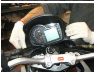
Disconnect the instrument panel connector.
