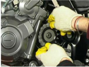
Loosen and remove the screw, collect the washer and slide out the cable guides.
