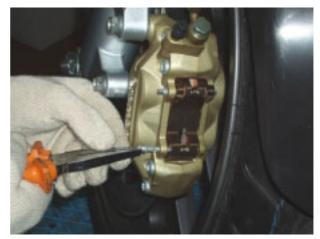
Remove the vibration damper.
