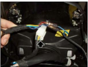
Remove the headlight together with left mount.
