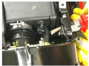
Remove the tie from wiring.
