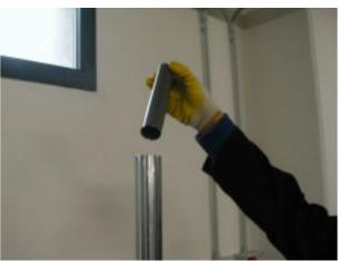
• Start the plug onto stanchion tube, be careful not to damage the O-ring. Tighten the plug to the specified torque.
