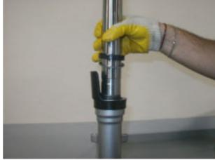
Fit the snap ring from inside the sleeve, using a screwdriver.
