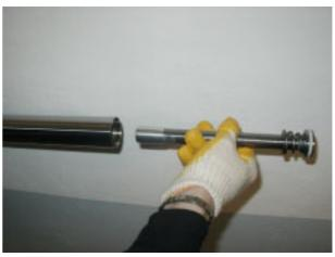
• Install the tube to the sleeve, fit the shim and oil seal in the relevant seats in the sleeve.
