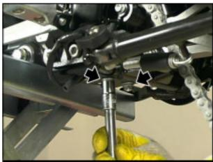
• Loosen the ties and remove the intake manifold.
