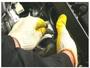
Loosen and remove the screw and disconnect the ground cables.
