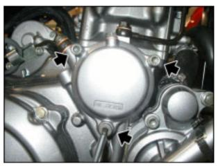
Remove the oil filter cover with gasket, collect the Oring.
