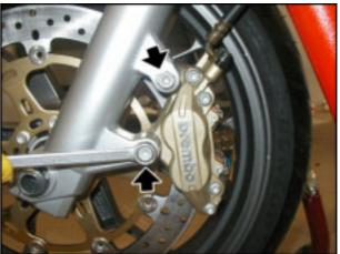
Fit the fork plate and tighten the two screws.
