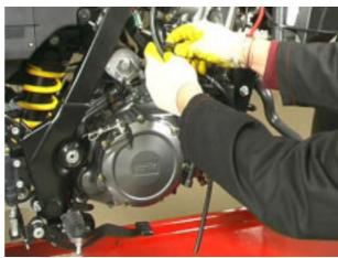
Remove the tie from wiring.
