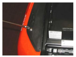
Working on either side, loosen and remove the two rear bottom screws.
