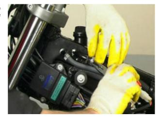
Remove the clamp and slide off the hose.
