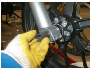
Tighten the wheel shaft clamp bolts to the right.
