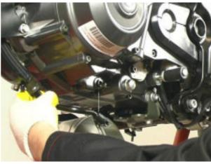
Loosen and remove the two screws, collect the spacers.
