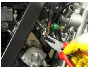
Disconnect the engine temperature sensor connector.
