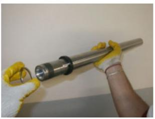
Install the damper rod with bottom buffer to the tube.
