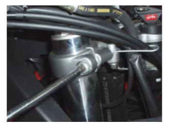
Remove the nut from the steering tube.
