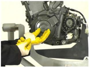
Using the suitable special tool (no. 8140850), loosen and remove the flywheel cover giving access to the timing reference.
