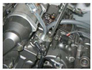
Release the clamp and remove the oil tank breather hose.
