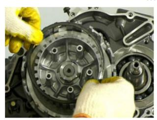
Install the thirteen clutch plates, position them correctly.
