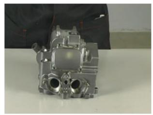
Working on either side, remove the tappet cover, collect the O-ring.
