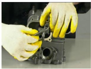
• Using the suitable puller, remove the intake rocker arm shaft.
