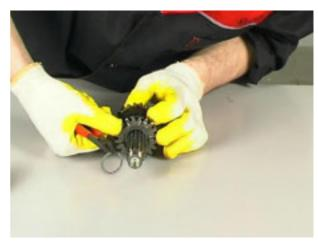
• Fit the safety washer, the spacer, the retainer and install the fifth speed gear
