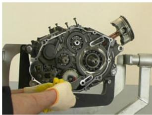
• Remove the circlip and the oil pump gear.
