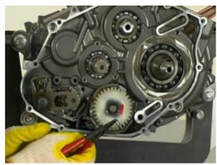
Unhook the spring and remove the complete gearbox shaft stop lever.
