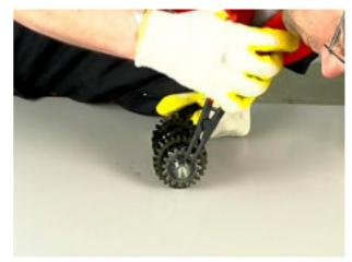
Remove the second-speed gear.
