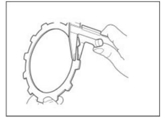
Driving plate thickness 1: 2.90-3.10 mm (0.114-0.122 in.) Service limit: 2.80 mm (0.110 in.) Driving plate thickness 2: 2.92-3.08 mm (0.115-0.121 in.) Service limit: 2.80 mm (0.110 in.) Driving plate thickness 3: 2.90-3.10 mm (0.114-0.122 in.) Service limit: 2.80 mm (0.110 in.)
