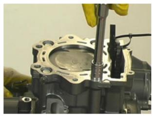
Tighten the two screws.
