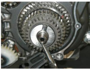
Install a new lock washer and nut.
