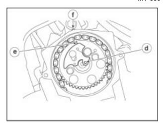
If these references are not aligned, correct by repeating the same indicated operations; restart from installation of the camshaft gearwheel.
