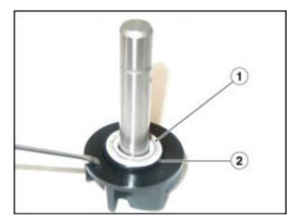
Remove the water pump seal using a small screwdriver.
