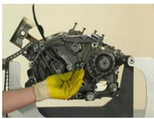
Remove the timing chain from crankshaft.
