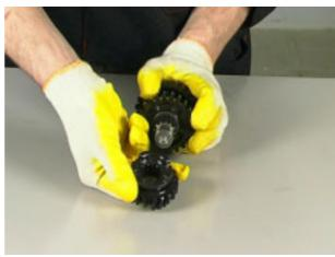
Remove the circlip.
