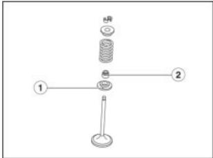
• Install the valve spring.
