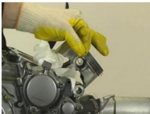
• Using the puller for piston gudgeon pin (no. 8600388), remove the gudgeon pin.
