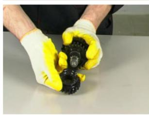
Install the first speed gear and washer.
