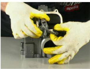
Install the bearing snap ring.
