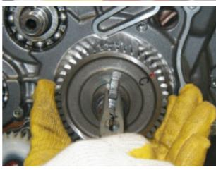
• Install the primary drive driving gear.
