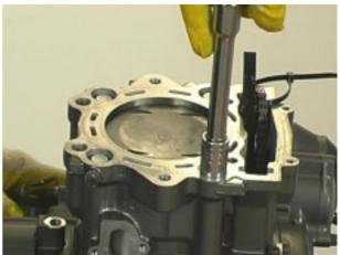
Release and remove the two screws.
