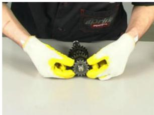
Remove the safety retaining washer.
