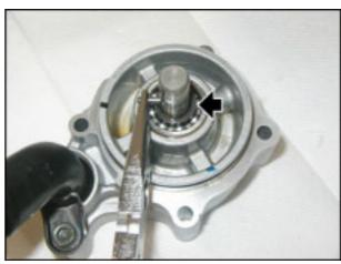
Remove the rotor shaft assembly.
