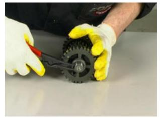
Remove the first-speed gearwheel and collect the washer.
