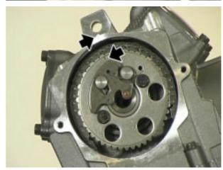
Loosen and remove the two screws and remove the timing chain tensioner.
