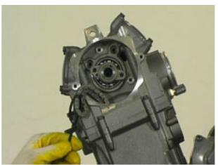
Loosen and remove the four stud bolts in the order shown and collect the washers.
