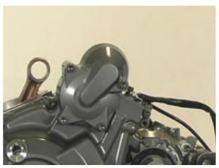
• Correctly fit the four screws and tighten in a cross sequence.
