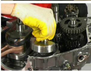
Remove the gearbox shafts assembly.
