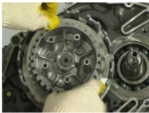
Straighten the lock washer, fit the universal clutch locking tool (tool no. 8600391), loosen and remove the clutch hub nut and collect the lock washer.
