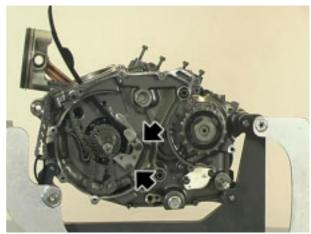
Remove the rear chain slider.
