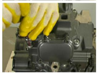
• Tighten the two lower bolts to the specified torque.
