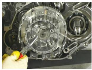
Using clutch locking tool (no. 8600391), tighten clutch hub nut to the specified torque
