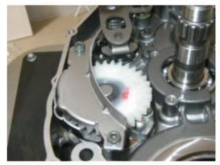
• Remove the safety snap ring (1) and the oil pump gear (2).
