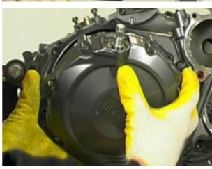
• Tighten the screws in a cross pattern.
