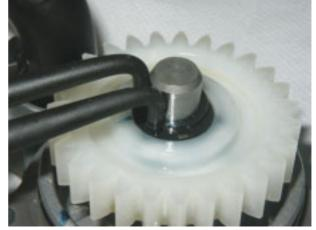
Remove the crankshaft gear.
