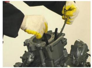
Release and remove the two screws.
