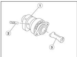
• Install the camshaft upward.
