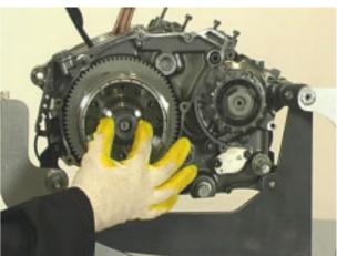
Tighten the nut to the specified torque.
