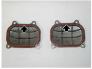
Working on either side, tighten the four screws of both covers
