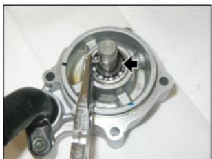
Install the rotor shaft gear with marking facing out (in view).
