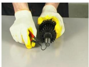
Remove the third-speed gearwheel and collect the safety washer.
