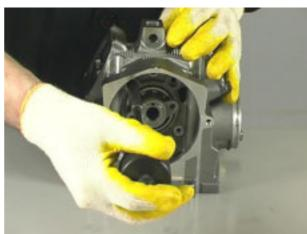
Remove the exhaust rocker arm.
