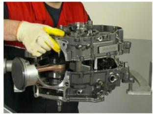
Tie the gearbox shafts with rubber bands.
