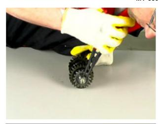
**NOTE** Ensure that the sharp edge (a) of circlips (2) is on the opposite side with respect to safety washers (1) and relevant gears.
