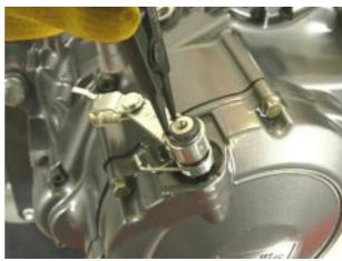
Install the spring to the release lever.
