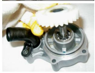
Install a new circlip.
