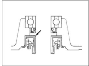
• Remove the oil seal (3) and the bearing (4);
