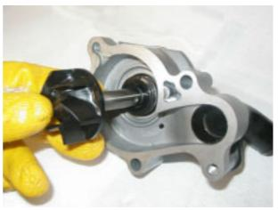
• Remove the support (1) and rubber dampener (2) from the rotor, using a screwdriver for flathead screws.
