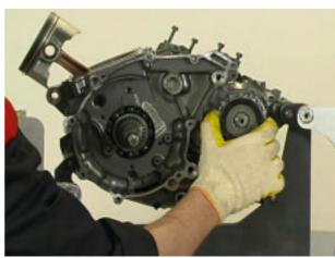
Remove the circlip.
