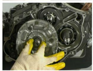
Remove the clutch housing.
