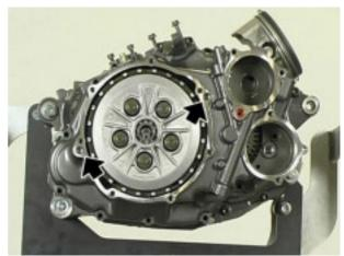
Change the gasket and install the right casing.
