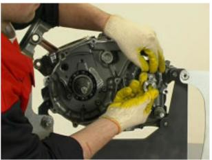
Remove the front chain sprocket.
