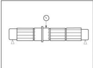
Check drive gears for wear and pitting and change faulty gears, if necessary.
