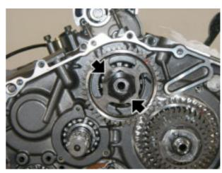
Loosen and remove the balancer driven gear nut, collect the washer.
