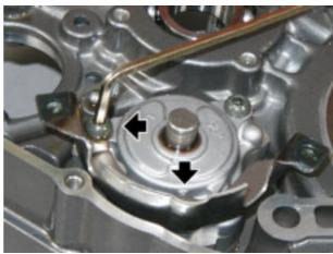
• Remove the oil baffle plate, collect the O-ring.
