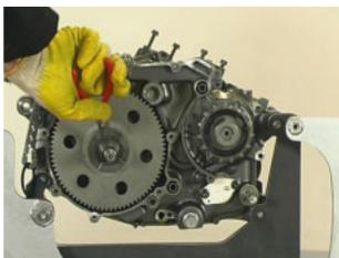
Install the flywheel, pay attention to the correct positioning of the key in its seat.
