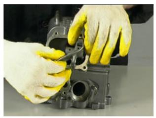
Using puller (no. 8140848), install the intake rocker arm shaft.
