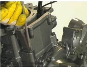
Change the seal, tighten the two screws and secure the cooling system fitting.
