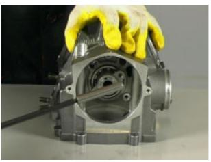
Remove the intake rocker arm.
