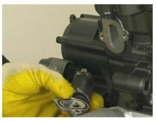
Loosen and remove the four stud bolts in the order shown and collect the washers.
