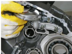
• Remove the oil pump unit, collect the two O-rings.
