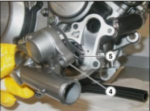
• Release and remove the two screws.
