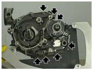
Install the complete selector shaft.
