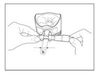
Calculate gudgeon pin to gudgeon pin hole clearance, change gudgeon pin and piston as a set if reading is out of allowed tolerance.
