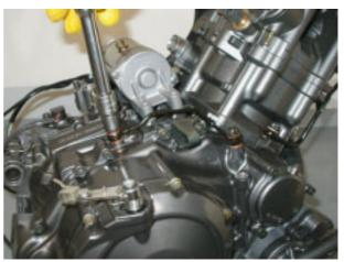
Loosen and remove the two screws and remove the starter motor.
