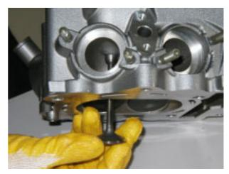
• Install the valve spring seat (1) and seal ring (2).
