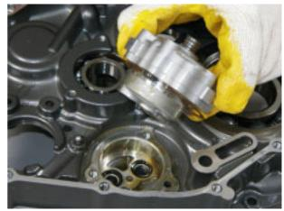
Fit the filter and secure it tightening the three screws.
