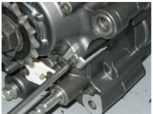
Remove the hose, collect the dowel and the snap ring.
