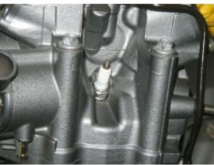
Loosen and remove the two screws and remove the secondary air hose, collect the metal gasket.
