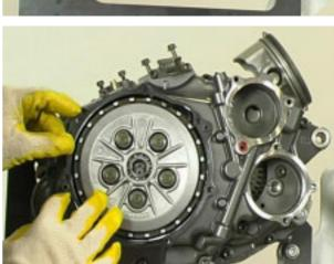
Install the clutch casing.
