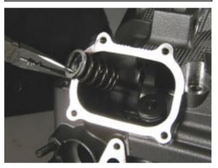
• Install the valve spring retainer.
