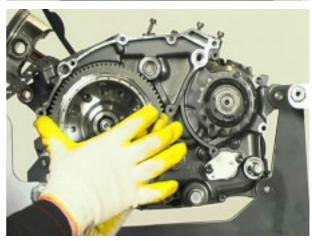
Set the piston locking tools (no. 8600840) and flywheel tools (no. 8140838).  $\label{eq:constraint}$
