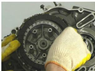
Remove the clutch damper spring and its housing.
