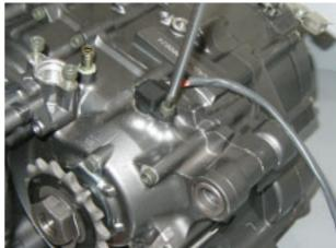
• Loosen the screw and disconnect the neutral sensor.
