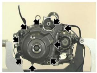
Remove the flywheel cover with gasket, starter motor idle gear, four dowels and two O-rings.
