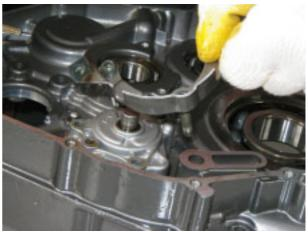
Tighten the two screws.
