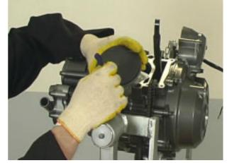
Remove the gudgeon pin circlip.
