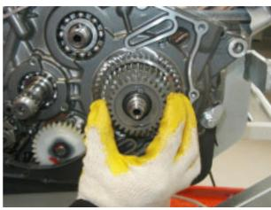
Remove the primary drive driving gear.
