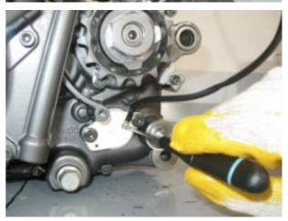
Loosen and remove the screw and remove the cable guide.
