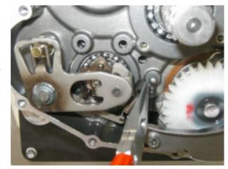
• Working on generator side, remove the snap ring.
