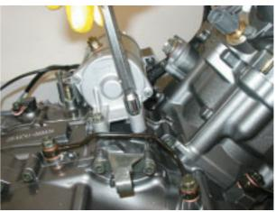
Release the clamp and remove the crankcase breather tank hose.
