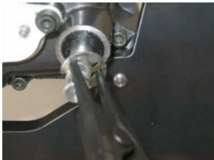
Working on clutch side, remove the gear shift selector and collect washer and oil seal.
