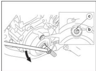
**NOTE** Ensure reference "I" (e) on gearwheel matches fixed reference (f) on the cylinder head.
