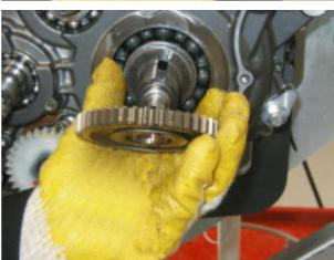
Install the key with rounded surface up.
