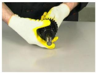
• Install the third speed gear and safety washer.
