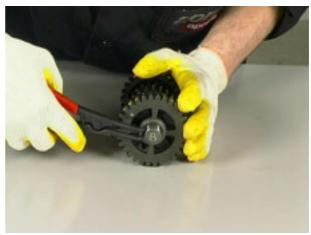
**NOTE** Ensure that the sharp edge (a) of circlips (2) is on the opposite side with respect to safety washers (1) and relevant gears.
