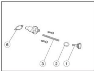
• Install the spring (3) and chain tensioner threaded plug (1), tighten plug to the specified torque.
