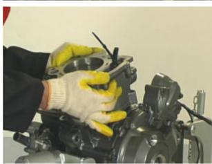
Collect the centring dowels and the seal.
