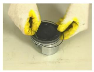
• Fit the piston and install the gudgeon pin.
