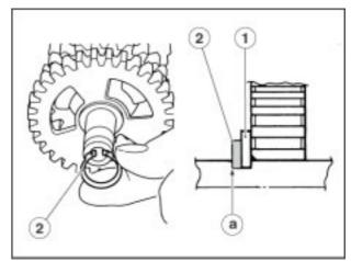
**NOTE** Install circlips so that both edges are at the centre of every groove.
