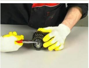
Remove the fifth-speed gear and collect retainer, spacer and safety washer.
