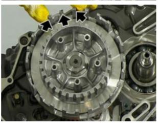
Install the damper spring seat and the spring, with "OUTSIDE" reference outward.
