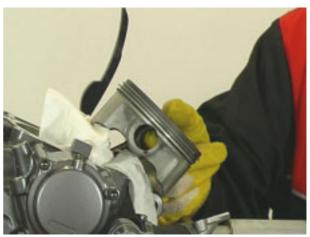
Remove the top ring, the second ring, and the three scraper rings.
