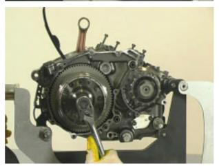
Position the two front and two rear dowels with O-rings to the crankcases.
