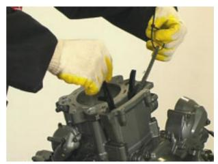
Install four new washers with rounded surface up.
