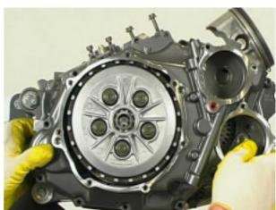
Correctly fit the screws and tighten in a cross sequence.
