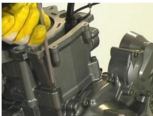
Remove the cylinder, pay attention not to damage the chain and the piston.
