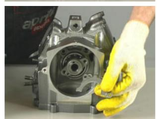
Using the suitable puller (no. 8140848), remove the decompression shaft.
