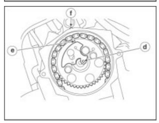
• Ensure reference "I" (e) on gearwheel matches fixed reference (f) on the cylinder head.
