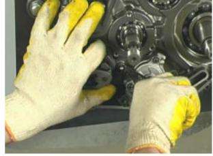
Insert the circlip.
