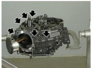
Use the connecting rod locking tool (no. 8600840) and the crankcase puller (no. 8140853) and separate the two crankcase halves.
