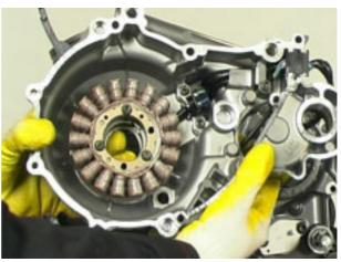
• Correctly fit the nine screws and tighten in a cross sequence.
