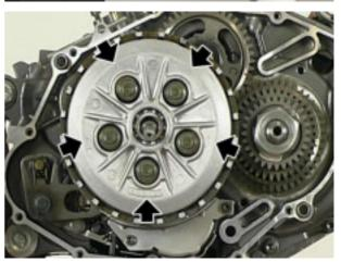
Remove the pressure plate, collect disengagement shaft and pushrod.
