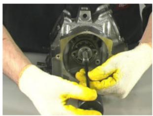
• Using the suitable puller (no. 8140848), remove the exhaust rocker arm shaft.
