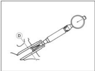
Calculate valve stem to valve guide clearance (G) as follows:
