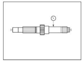
With a dial gauge and a centring device, measure secondary shaft runout, change the shaft if reading does not comply with recommended values.
