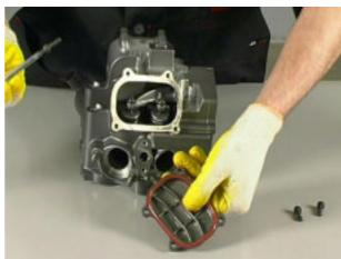
Loosen and remove the two adjuster screws.
