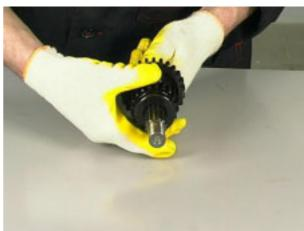
• Remove the circlip and then the second-speed gearwheel, collect safety washer and seal.
