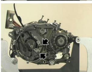
• Fit the timing chain to crankshaft.
