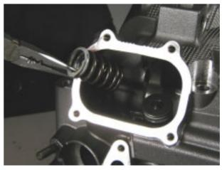
• Remove the valve stem oil seal (1) and valve spring seat (2).
