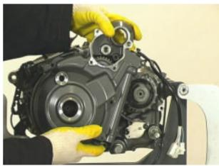
Undo and remove the flywheel nut.
