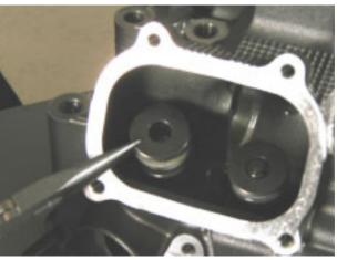
Remove the valve spring.
