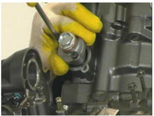
Hold the flywheel nut with a wrench, loosen and remove the two screws on the camshaft gearwheel.
