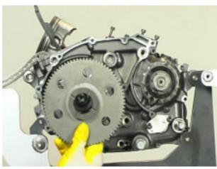
Fit the key into the crankshaft.
