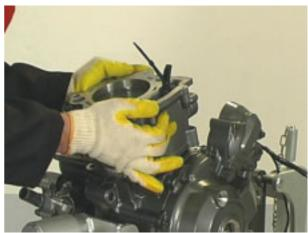
• Install the timing chain guide (exhaust side).
