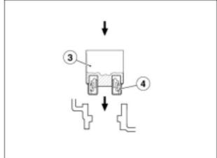
**NOTE** Before refitting the rubber damper, apply an emulsified solution to the outer surface to help installation, see (LUBRICANT TABLE).
