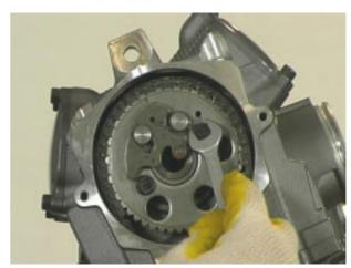
Remove the camshaft gearwheel.
