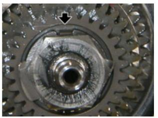
Insert key and counter shaft driven gear.
