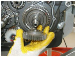
Install the water pump driving gear.
