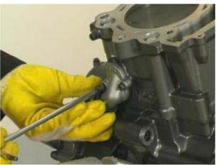
• Remove the cooling system union, collect the seal.
