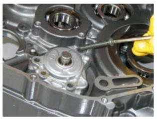
Loosen and remove the three screws and remove the filter.
