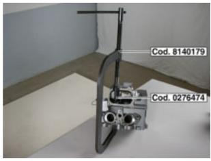
· Remove the valve spring retainer.
