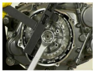
• Remove the clutch hub and collect the thrust washer.
