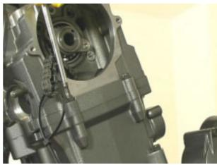
Remove the cylinder head, pay attention to the timing chain and to the decompression system since it is free to move in its housing.
