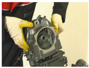
• Collect the seal and the two centring dowels.
