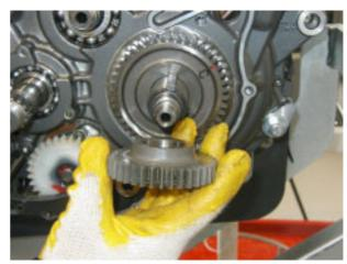
• Remove the balancer driving gear and remove the key.
