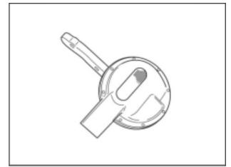
Check oil delivery tube for damage. Change the part, if necessary.
