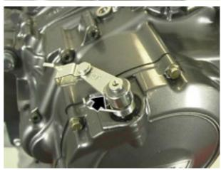
Fit the circlip.
