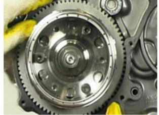
Set the starter motor idle gear.
