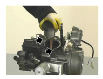
Lubricate the piston, the piston rings and the cylinder with engine oil.
