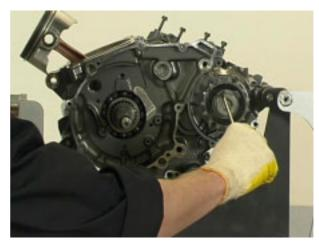
• Undo and remove the nut and collect the washer.
