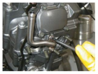
Remove the oil delivery hose, collect the O-ring.
