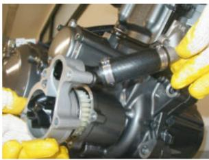
Release and remove the clamps.
