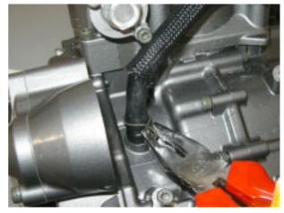
Loosen and remove the screw and remove the speed sensor.
