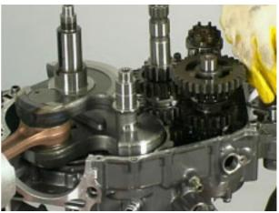
• Install the right casing to the left casing, tap with a mallet, if necessary.
