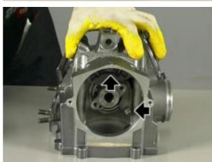
Remove the bearing snap ring.
