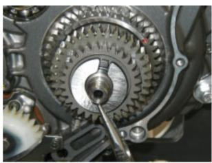
Remove the water pump driving gear.
