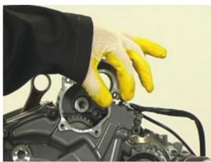
• Install the torque limiter cover with a new gasket.
