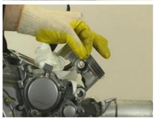
Install a new cylinder gasket.
