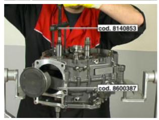
Tap the crankcases lightly with a hammer to separate the crankcases. After they become separated, remove both tools.
