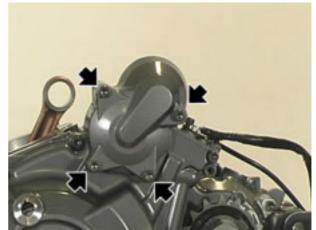
• Remove the cover together with torque limiter.
