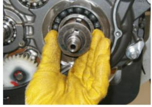
Install counter shaft driving gear.
