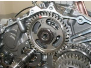
• Remove the driven gear and collect the key.
