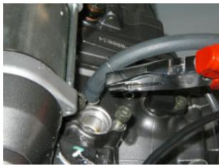
Loosen and remove the two screws, remove the oil hose and collect the four washers.
