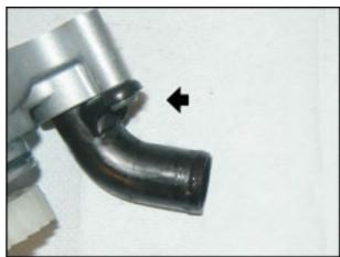
• Install the water pump breather hose (1) and water jacket joint (2).
