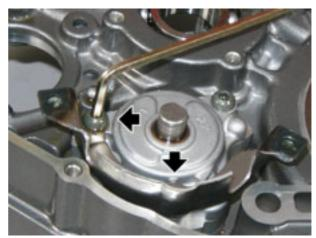
• Install the oil pump gear (2) and change the safety snap ring (1).
