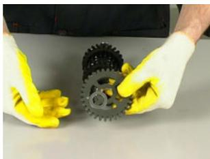
• Remove the fourth-speed gearwheel.
