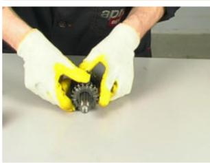
Remove the circlip.
