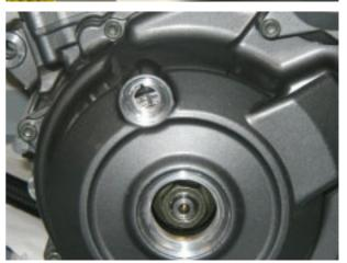
Release and remove the two screws.
