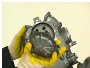
• Ensure that reference mark "I" on camshaft gearwheel matches cylinder head fixed reference mark.
