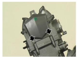
Remove the gearwheel inspection cover, collect the seal.
