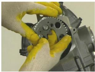
• Fix the timing chain with a tie.
