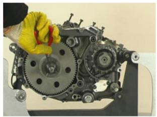
Remove the starter clutch and the roller bearing.
