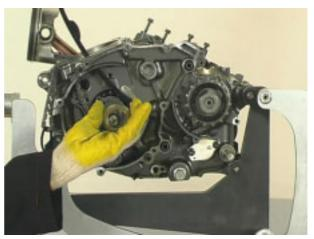
Release and remove the two screws.
