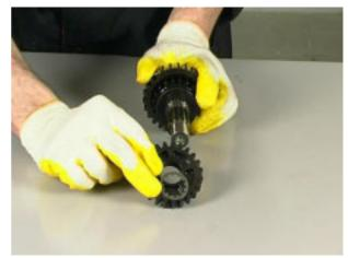
Remove the fifth-speed gearwheel.
