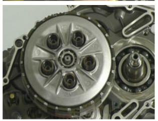
Tighten the screws with washers to the specified torque.
