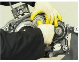
• Fit the flywheel cover complete with stator.
