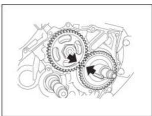
• Tighten countershaft driven gear nut to the specified torque.
