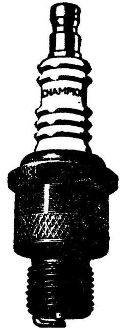
*Fig. 4. The sparking plug*
