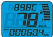
In main screen, press the **Adjust button** to switch from odometer, Trip A, and Trip B..
