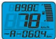
Press the **Adjust button** one time, and then the odometer will switch to **trip A**
