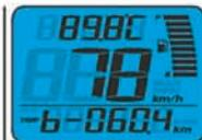
Press the **Adjust button** one time, and then the odometer will switch to **trip B**.
