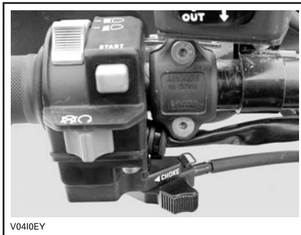
CHOKE LEVER IN THE OFF POSITION
