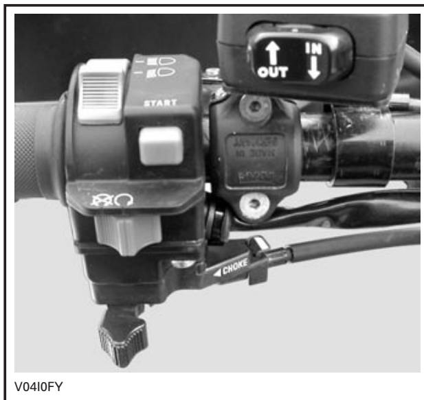
CHOKE LEVER IN THE FULL CHOKE POSITION
