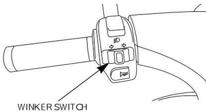
If this switch is turned on when the main switch is in an ON position, the winker will operate.
