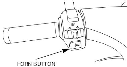
The horn is sounded if the horn button is pressed when the main switch is in an ON position.
