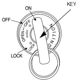
1. ON.... Starts engine. Key can not be pulled out.(Headlight ON)
