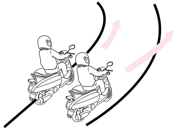
The centrifugal force increases in inverse portion to the radius of a curve and in portion to the square speed. Decelerate prior to entering the curved way to reduce the centrifugal force.
