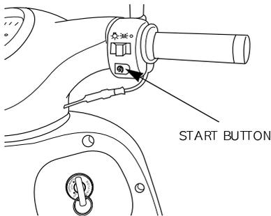
The engine is started pressing this button when pressed in a state where the main switch key is placed to an ON position and the brake lever is pulled.
