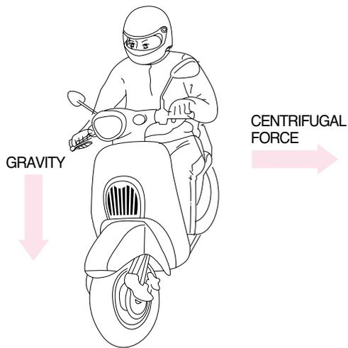
The basic principle of turn is balancing using the centrifugal force which makes vehicle go outside and the gravity which makes vehicle fall inside.
