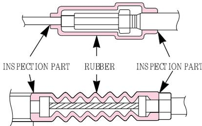
Check the installing condition of rubber boots daily. After adjusting the free play of throttle grip, never forget to place the rubber boots to the original position.
