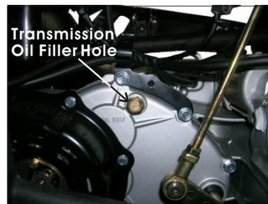
1. Place an oil catch pan under the unit directly below the transmission box.
