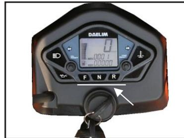
The instrument panel has three lights that correspond to the transmission shifter shaft position.
