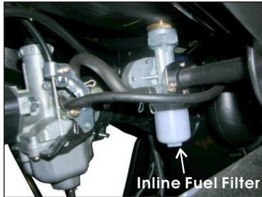
The filter should be replaced every 600 hours of operation and at the start of each season.
