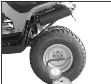
It is important to inspect your tires and wheels for damage and wear before each riding session. Inspect each tire for cuts, tears and punctures. Inspect the wheel rim for dents and separation of the wheel from the tire bead.
