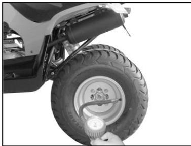
It is important to inspect your tires and wheels for damage and wear before each riding session. Inspect each tire for cuts, tears and punctures. Inspect the wheel rim for dents and separation of the wheel from the tire bead.
