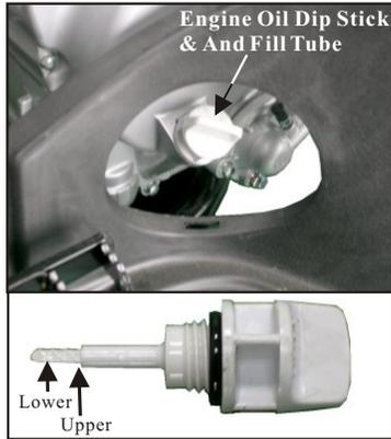
Your ATV uses automotive type engine oil to lubricate the engine. The engine oil dip stick is located on the right hand side of your engine below the transmission shifting lever.
