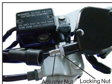
The cable should be adjusted to allow for  $\frac{1}{8}$ " free travel before the throttle engages the carburetor throttle slide. Slide the adjuster cover down the cable to uncover the adjuster assembly. To adjust the cable's free travel, loosen the locking nut of the cable adjuster, and turn the adjuster nut until there is  $\frac{1}{8}$ " free travel in the lever. Tighten the locking nut to secure the adjusting nut. Slide the cover back over the adjuster assembly.
