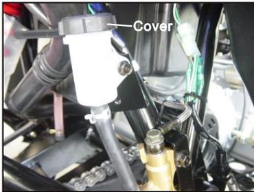
Fill the reservoir to 1/8" from top with Dot-3 SAE-J 1703 grade brake fluid.
