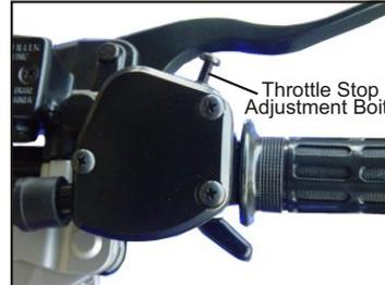
To increase the throttle's travel, thus increasing the maximum speed, turn the throttle stop bolt counter clockwise. To decrease the throttle's travel, thus decreasing the maximum speed, turn the throttle stop bolt clockwise.
