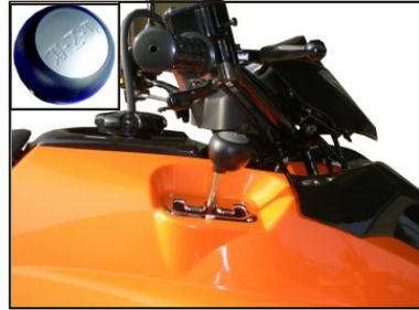
Your ATV is equipped with a fully automatic C.V.T. transmission and has forward and reverse gearing. A transmission shifting shaft is located on the right hand side of your vehicle. The shifter has three positions "F" Forward, "N" Neutral and "R" Reverse.
