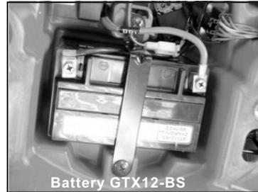
When reinstalling the battery, be sure to connect the red cable to the positive (+) terminal and the black cable to the negative (-) terminal.
