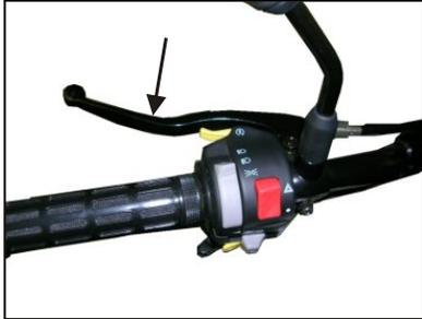
pressure to your front brakes so that the wheels lock up, stop turning, and causing a loss of steering control. If the front wheels lock up, and stop turning, lightly reduce the pressure on the front brake lever until they unlock and start to turn.
