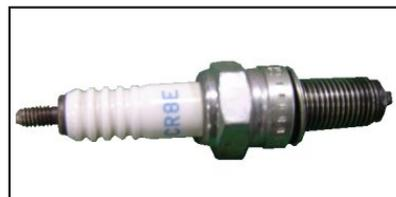
Replace spark plug at the beginning of each season with a replacement plug **NGK-CR8E**. Disconnect spark plug wire. Clean dirt from around spark plug base with brush or compressed air. Remove spark plug with spark plug wrench. Set the spark plug gap on the new plug to 0.023". Install the new plug screwing it in finger tight and then use the plug wrench to screw the plug in another  $\frac{1}{2}$  turn. Inspect the spark plug wire for cuts, nicks or other damage. Replace as needed.
