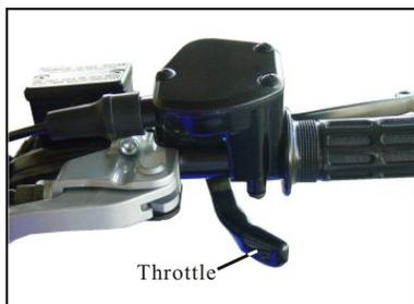
The throttle lever is located beside the right-handbar grip and is operated by using the right-hand thumb. The lever is spring loaded and will return to the idle position when you remove your thumb from the lever. To accelerate the unit, simply press the lever forward to open the throttle slide in the carburetor. To slow the unit, reduce the pressure on the lever or remove your thumb and the throttle will return to the idle position automatically.
